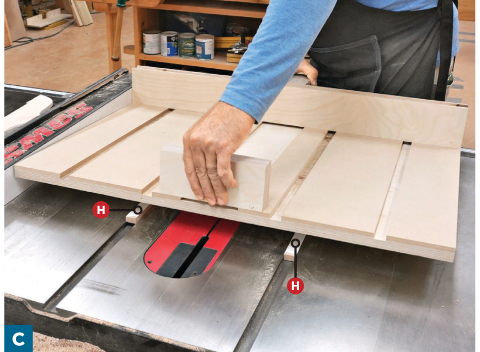
With the back edge of the sled aligned with the back of the saw table and the side of the sled against the fence, carefully lower the sled onto the runners (D).
