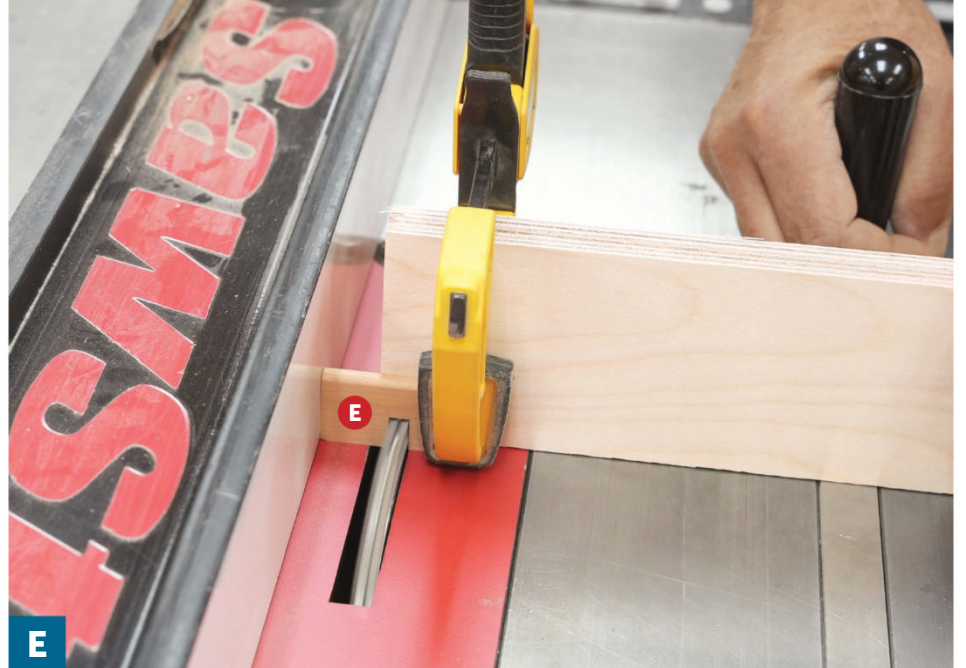
E With a 1/4" dado blade in the tablesaw, test the rip-fence position by notching test pieces the same length as an end key (E) to center the notch on the workpiece. Then notch each end key.
