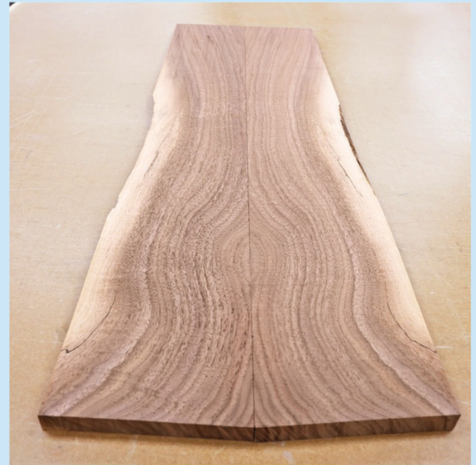
Resawing the board into thinner pieces and gluing the jointed edges together creates a symmetrical pattern.
