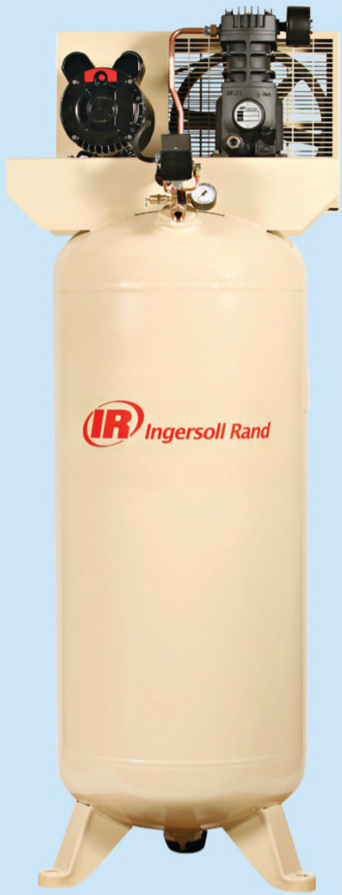
The 60-gallon tank of this 3-hp compressor provides air to spare. It stands 67" tall and requires 220-volt power.
