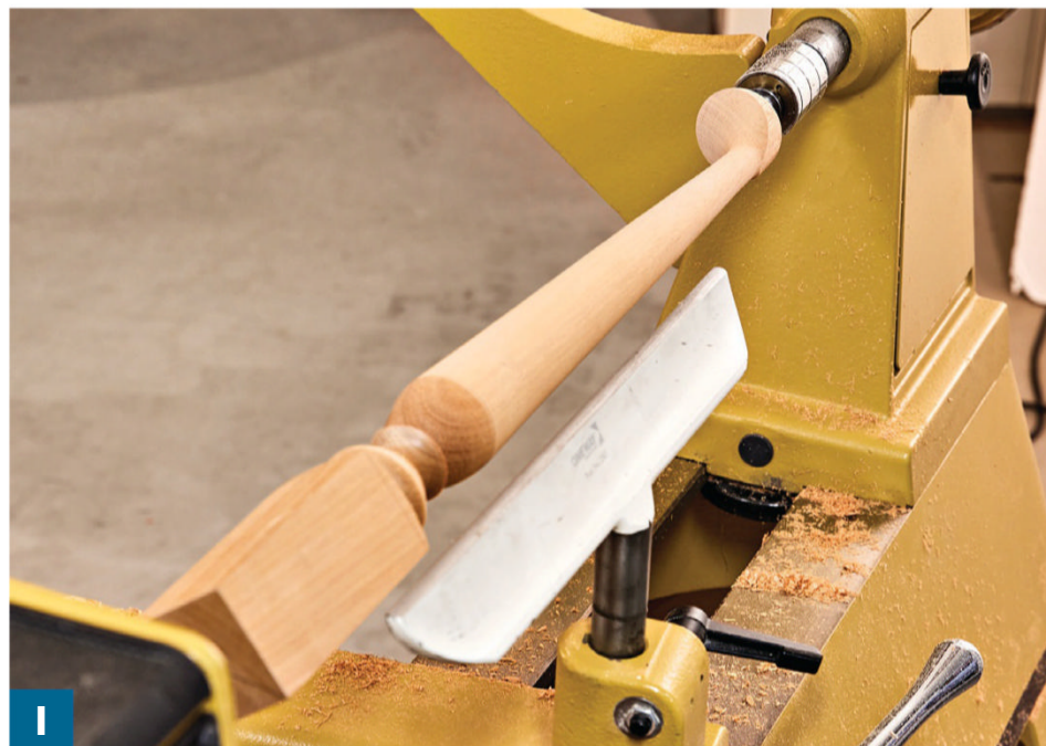
I The completed leg needs only light sanding. Remove the tool rest and hold long strips of sandpaper taut and avoid contact with areas turned on a different axis.
