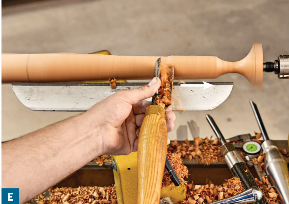
E Start the taper near the ankle where there is more material to remove. Begin each successive cut closer to the calf and make longer cuts to the ankle.
