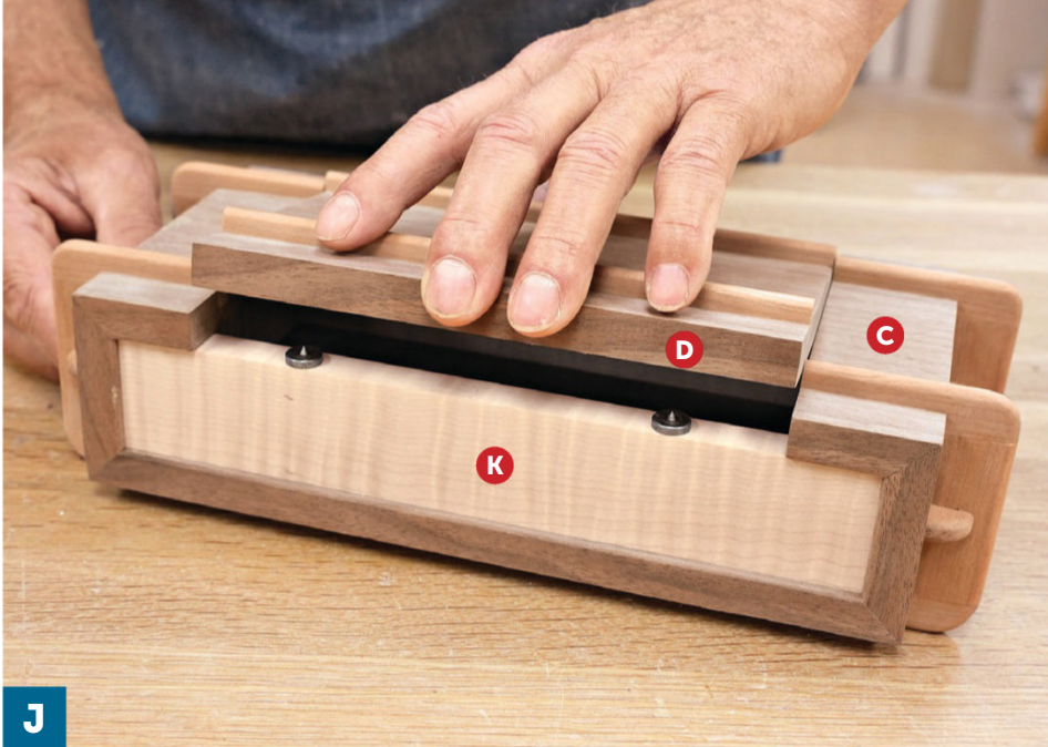
Place a dowel center in each hole in the box back (K). Position the lid (D/G) flush with the front of the top cladding (C), then pivot the lid down and press it firmly against the dowel centers.
