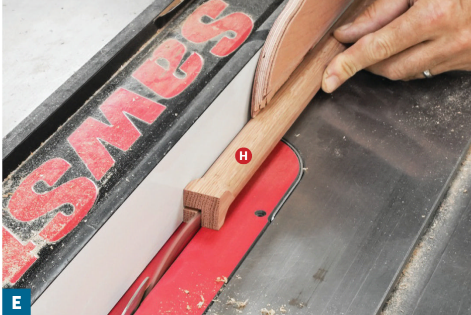
Cut a 1/2" rabbet 1/2" deep in each of the legs, using a pushblock to keep the squared ends of the legs tight against the fence and saw table. Cut the rabbet in two passes.
