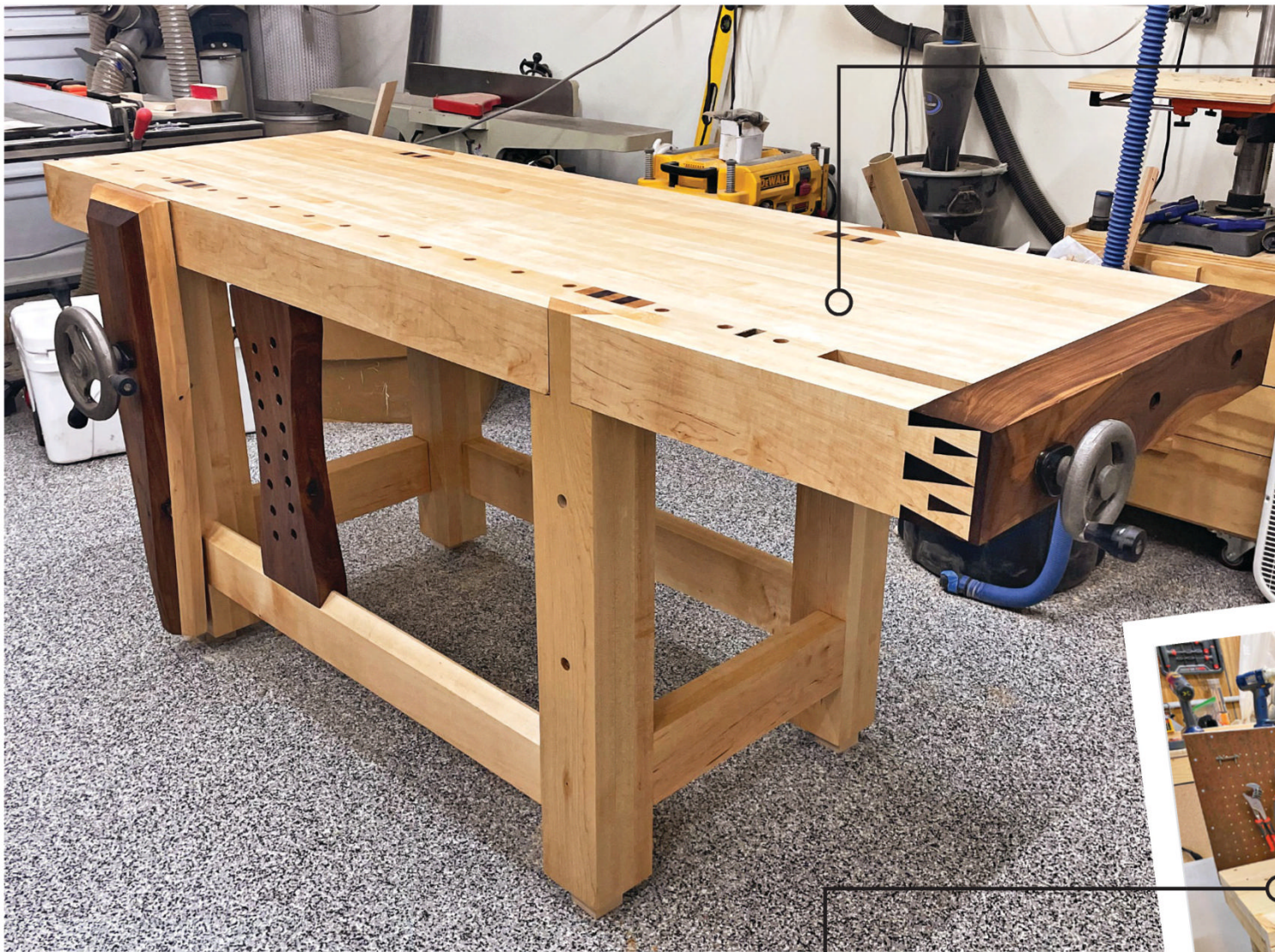
It took CALEB WYATT of Buckeye, Arizona, about nine months to build this workbench. He used hard maple with walnut accents. He built the vises using hardware from benchcrafted.com .
