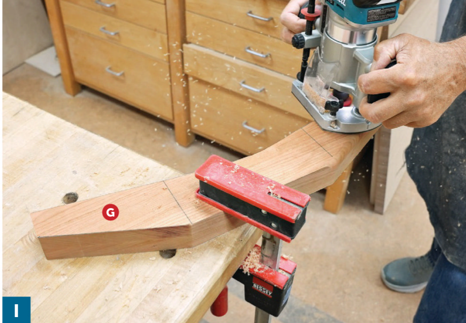
The extra-long foot blanks allow you to safely clamp the workpiece while sawing and routing the feet (G) to shape. Cut the feet to length after completing all the shaping and sanding.
