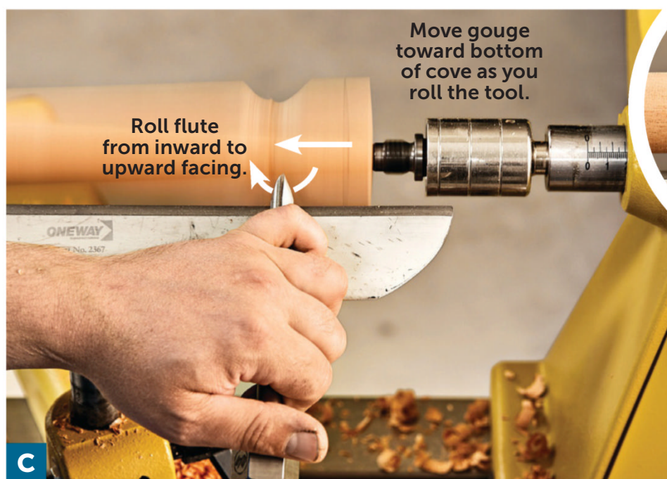
C Start with the gouge flute closed and facing the direction of the cut. Lift the handle to engage the cutting edge, then roll the flute open and raise the handle farther until you reach the center of the cove.
