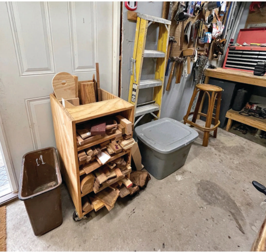
A simple, plywood cart keeps cutoffs contained and accessible for use in smaller projects like toys and kitchen utensils. Casters make the cart easily mobile.
