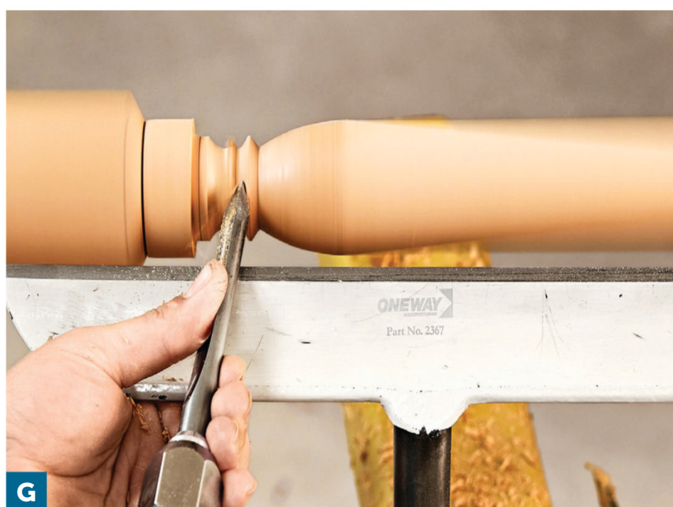
G As when cutting the cove for the ankle, begin on one side and work down to the center, then work from the opposite side. Increase the width and depth of cut until you reach the final dimensions.
