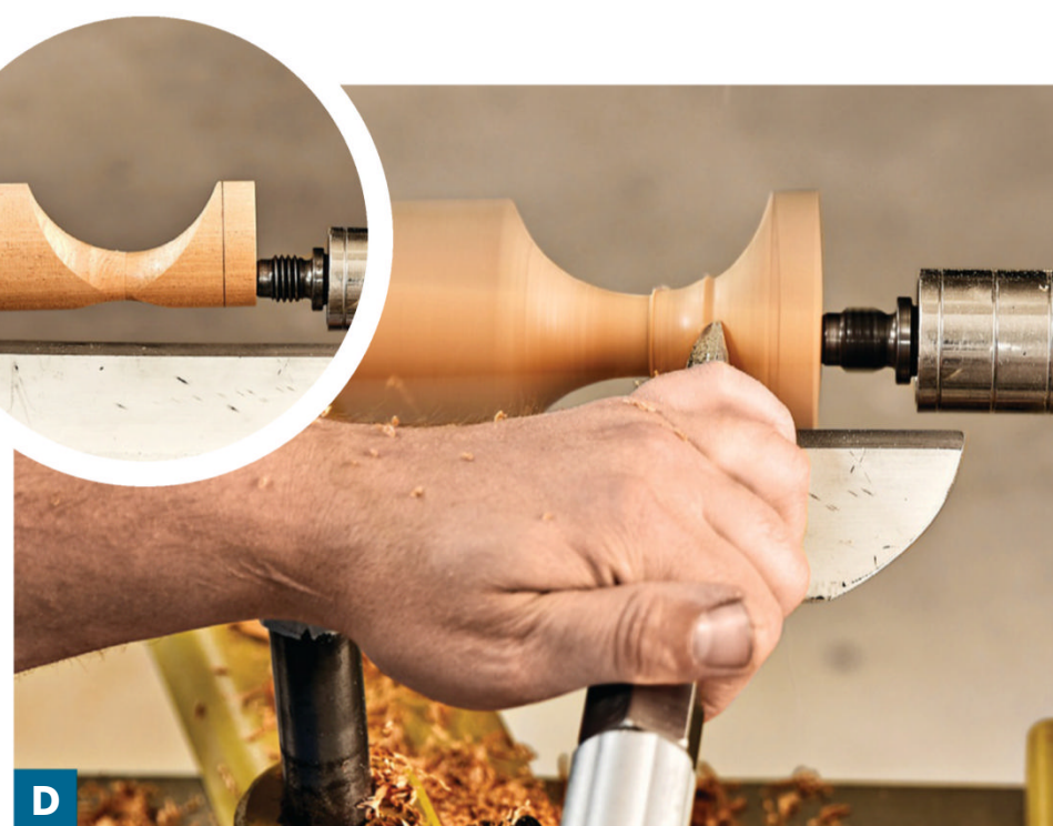
D Work from one side of the cove to the center, then from the other side to the center. Make each successive cut deeper and wider until the final cut reaches from the toe to the ankle (inset).
