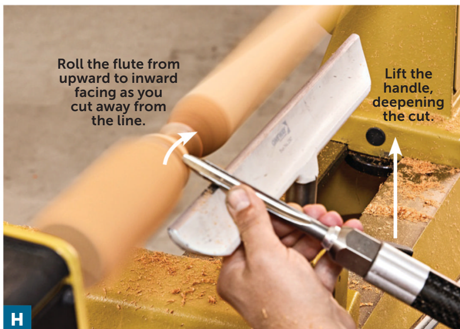
H Forming a bead is the opposite action of cutting a cove. Begin with an open flute just off the centerline, then roll the tool closed as you lift the handle and cut away from the line.
