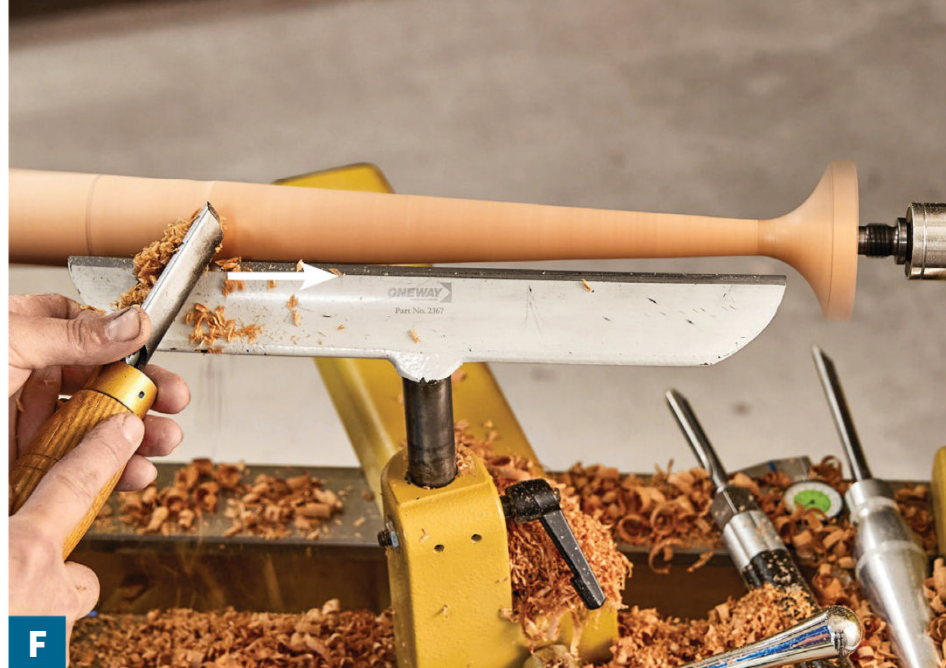
F For a clean final cut along the taper that needs minimal sanding, skew the gouge to face the direction of the cut. Move at a slow and steady pace.
