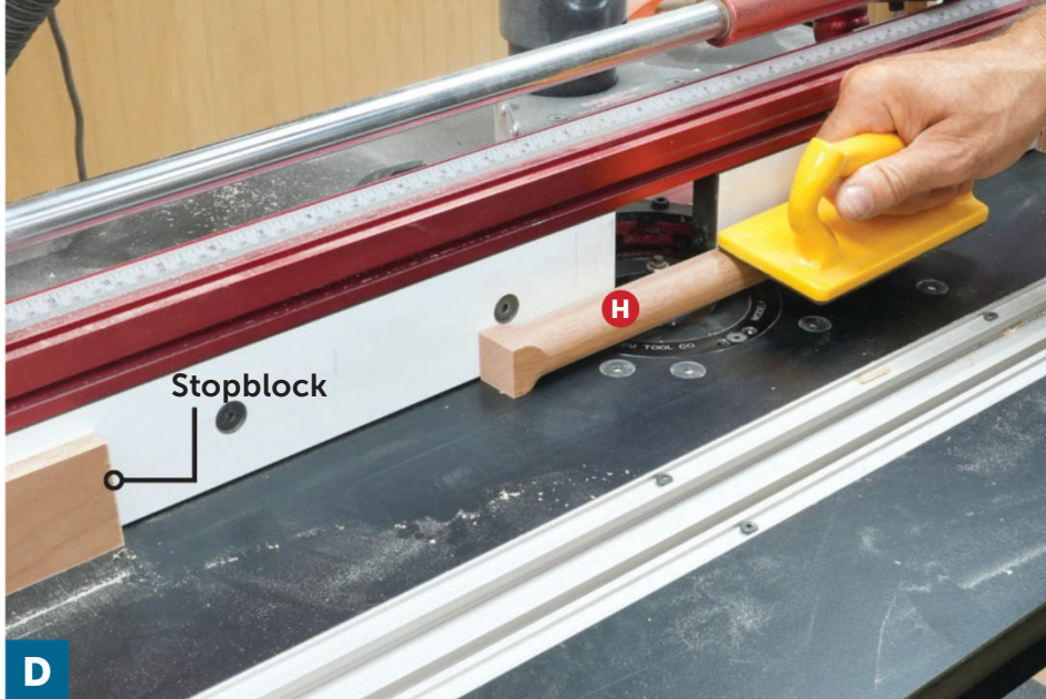
Align the marks with the center of a 1/2" round-over bit to set blocks for your starting and stopping point on the legs (H). Then rout all four corners of each leg, using a pushblock to guide the legs.
