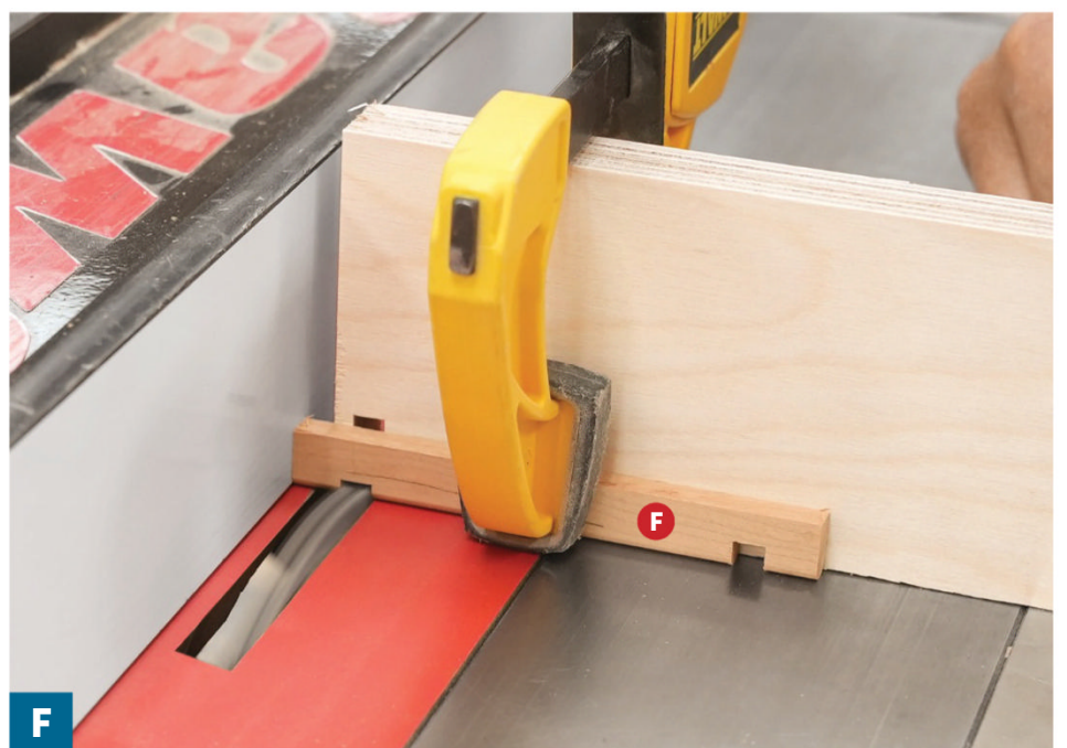
F Lower the dado blade and reposition the rip fence to cut the notches in the handles (F) 3/8" from each end. Notch one end, flip the workpiece end for end, and notch the other end.
