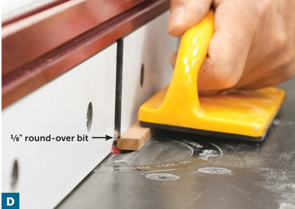
D Set the router-table fence flush with the bearing of the bit. Rout both faces of the key and handle blanks along one edge to create a bullnose profile.
