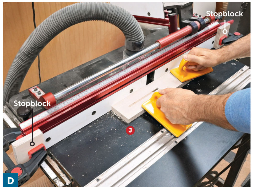
Rout the fence base (J) slot in multiple passes, raising the bit between each pass. Use stopblocks to ensure the starting and stopping points stay the same.
