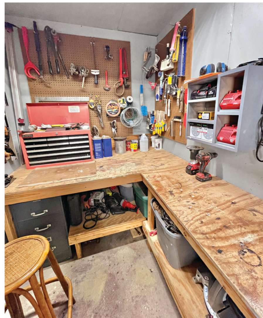
A wall-mounted charging station also holds sanding discs. The area below the bench houses portable power tools, a file cabinet for table saw accessories, and a bin filled with electrical supplies.
