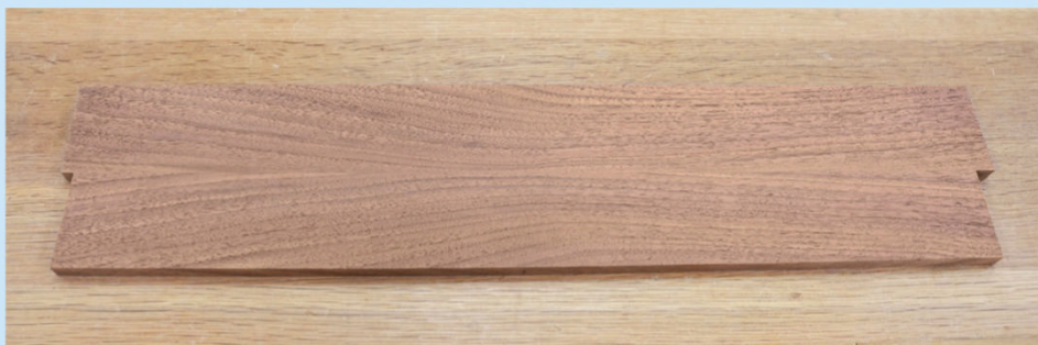
Rip each resawn board to one-half the width of the finished blank—in this case, 2½" for a 5" blank. Glue the jointed edges together, aligning the grain pattern as closely as possible for a mirror match.
