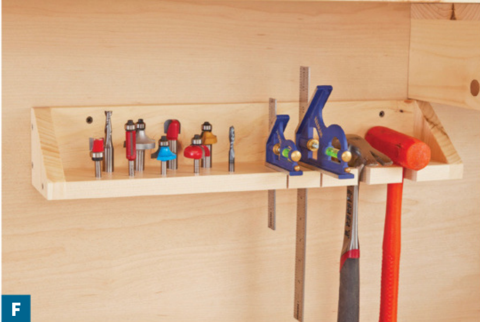
F Cut slots to accept squares, hammers, and chisels. Drill stopped holes \frac{3}{8} " deep to fit the shanks of router and drill bits, or through holes for screwdrivers. Or leave the shelf whole for odds and ends.
