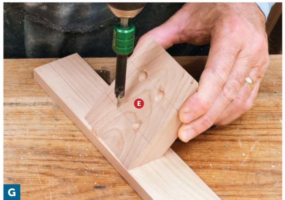
After the bit bites into the wood, raise the corner block to rest on its beveled end. Keeping the bit perpendicular to the bench, drill through the block.
