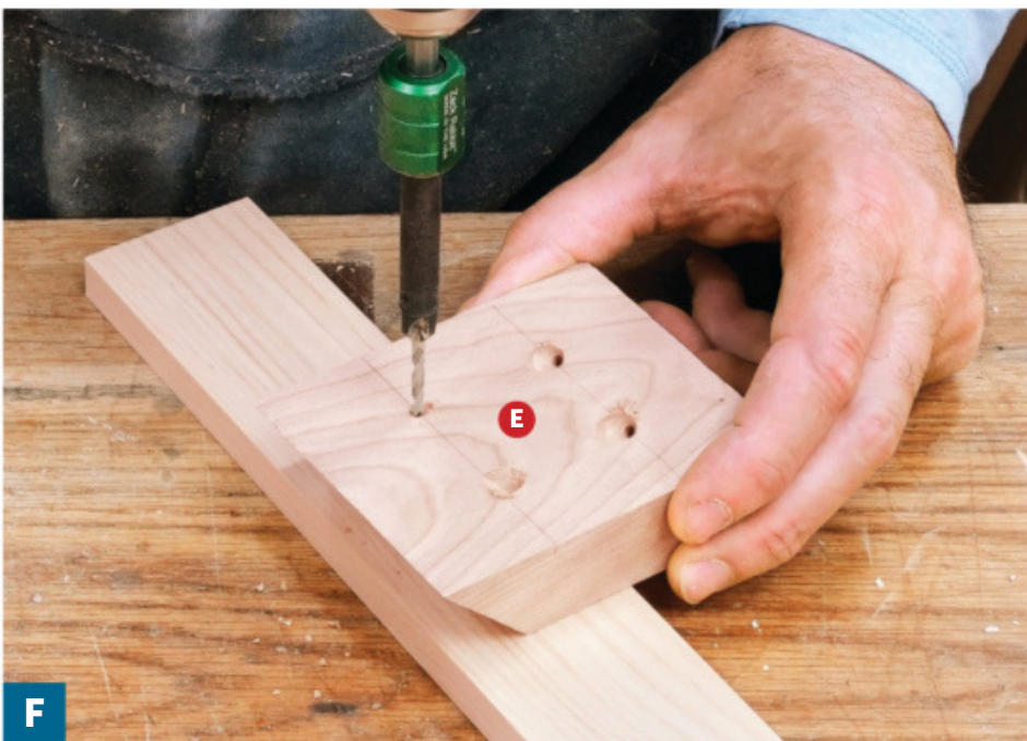
Rest the corner block (E) on a scrap backer block. Start drilling at the marked locations with the bit perpendicular to the face of the corner block. Drill no more than \frac{1}{8} " deep.
