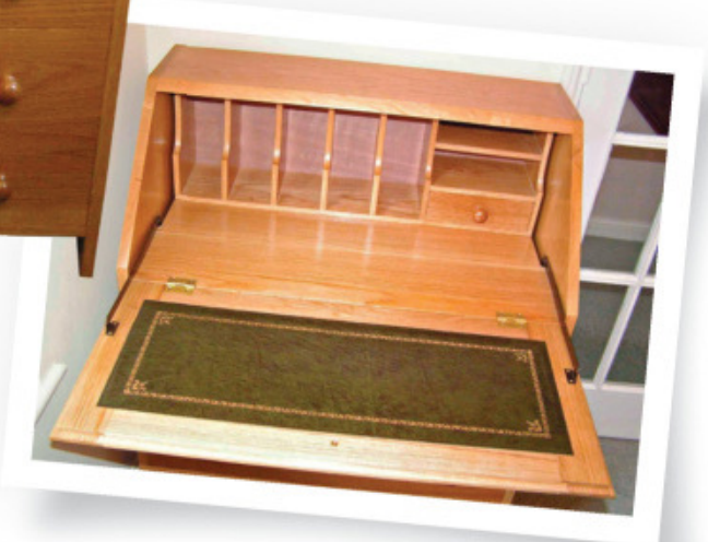
● KEVIN GOOSMAN of Dorridge, England, used American white oak to build this desk. The drawers were constructed with dovetail joints. He turned the handles and made the storage compartments inside. The desk includes mechanisms to automatically extend salvaged lopers (runners) to support the drop-down writing surface. He built the frame using mortise-and-tenon joints.
