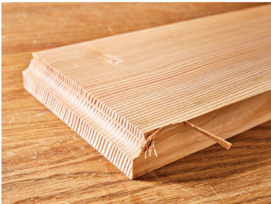
Routing end grain tends to tear out the wood along the adjoining edge as the router bit exits the cut, particularly in woods that are prone to splintering, such as this Douglas fir.
