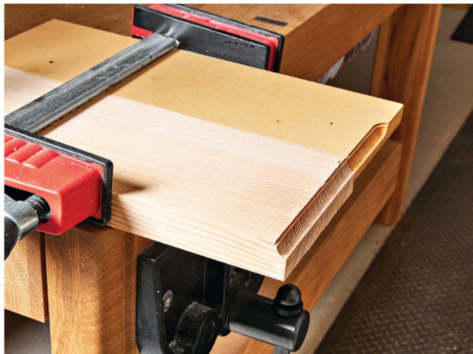
Prevent tear-out by clamping a backer board to the edge of the workpiece and routing into it as you make the cut. The backer board supports the wood fibers of the workpiece.
