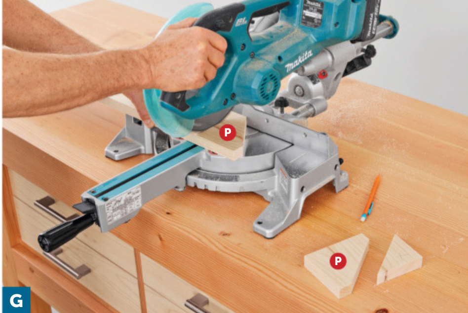
G After miter-cutting the end of the blank, crosscut a shelf end (P) from the blank. Reset the saw to 38°, miter-cut again, leaving the squared tip, and repeat the process to make each shelf end.
