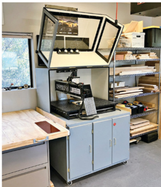
Henry built a cabinet to house his Shark CNC machine. The hinged top with 4" dust port makes it easy to access and tames the noise when closed. The base holds accessories like bits and tools.
