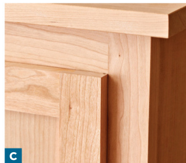
C If the opening is relatively square, size the door for a tight fit. This makes it easier to fit the door, while still providing enough extra material for trimming.
