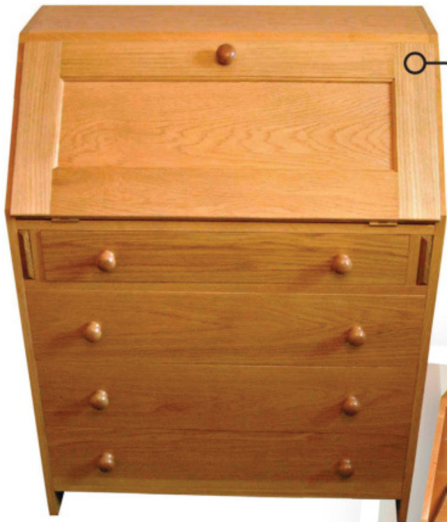
● KEVIN GOOSMAN of Dorridge, England, used American white oak to build this desk. The drawers were constructed with dovetail joints. He turned the handles and made the storage compartments inside. The desk includes mechanisms to automatically extend salvaged lopers (runners) to support the drop-down writing surface. He built the frame using mortise-and-tenon joints.
