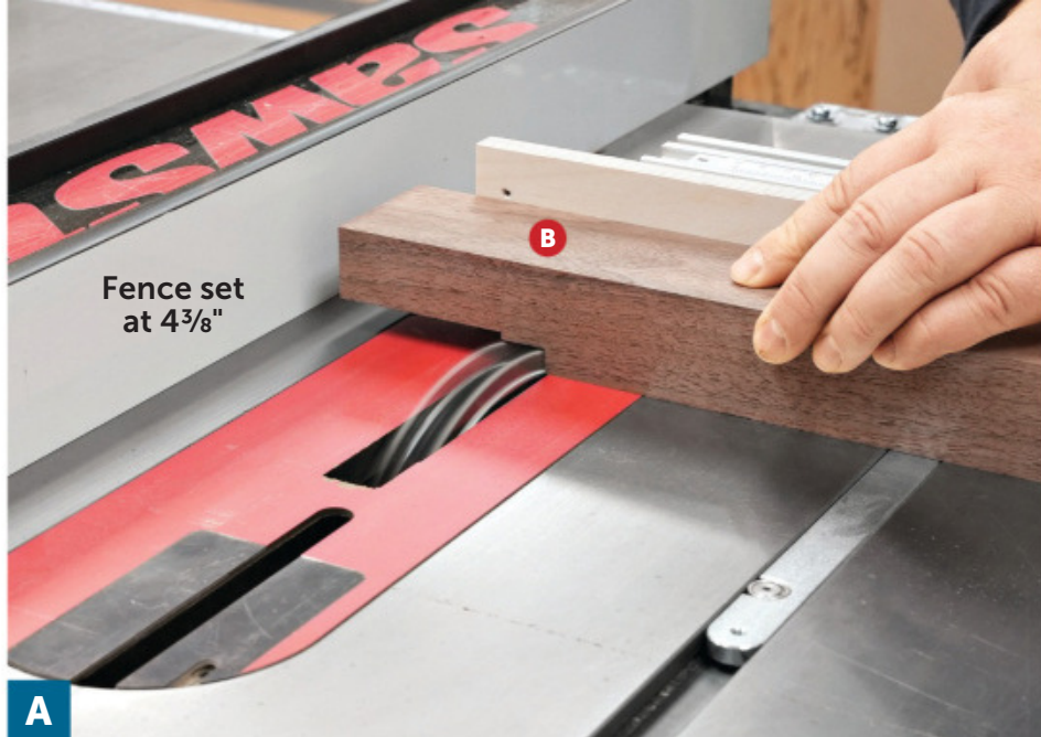
A Raise the dado blade to \frac{1}{2} " above the table and set the rip fence as a stop. Using an auxiliary fence on the miter gauge, rabbet one end of the rear infill (B) in multiple passes.
