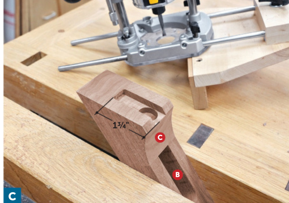
Using a router equipped with a fence and \frac{1}{4} " spiral upcut bit, rout the \frac{5}{16} "-deep slot for the adjuster. Rout one edge, then the other, and then remove the waste in the center of the slot.
