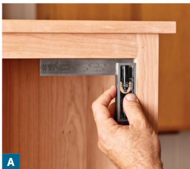
A Before checking the door opening for square, place the cabinet on a stable, flat surface and install the back of the cabinet (if you haven't already).
