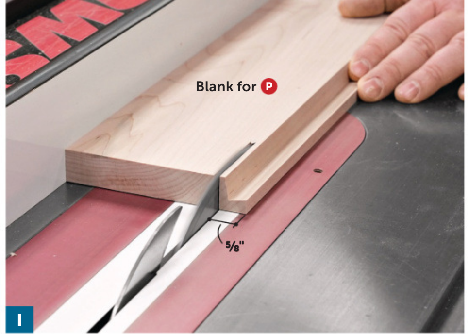
Adjust the tablesaw fence to leave a \frac{5}{8} "-wide strip on the left side of the blade, then ripcut the seat strip to width.
