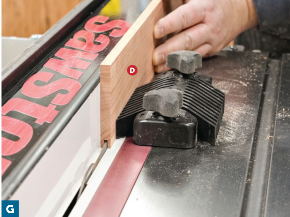
G Adjust the blade height to \frac{3}{8} " and run both faces of five of the slats against the fence to cut a centered groove.
