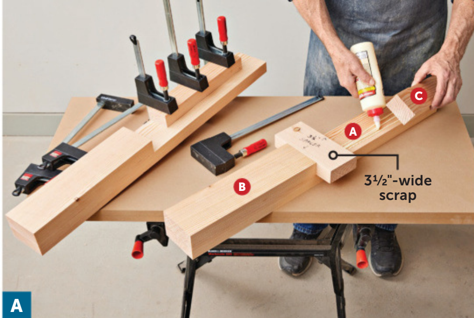
A Cut a 3½"-wide scrap to help position the upper leg spacer (C). Note that the legs mirror each other. Remove the scrap after clamping the spacer so the scrap doesn't get glued in place.
