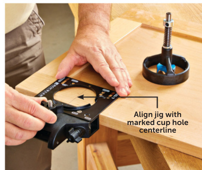
The Rockler jig requires you to measure and mark the location of the cup hole on the door stile, then align the jig with your mark and tighten the clamping knob. The drill guide fits over a raised rim on the base.
