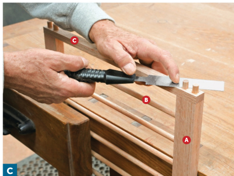
C Glue in extra-long dowels to reinforce the butt joint between the divider rails (A) and the divider stiles (C). Cut the dowels using a flush-trim saw. Sand the stiles smooth.
