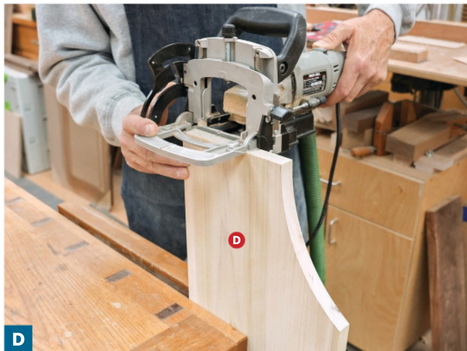
Lay out biscuit slots in the case sides (D), top (E), and bottom (F). Make sure to create mirror images for the sides, cutting the slots on the inside face of each piece.
