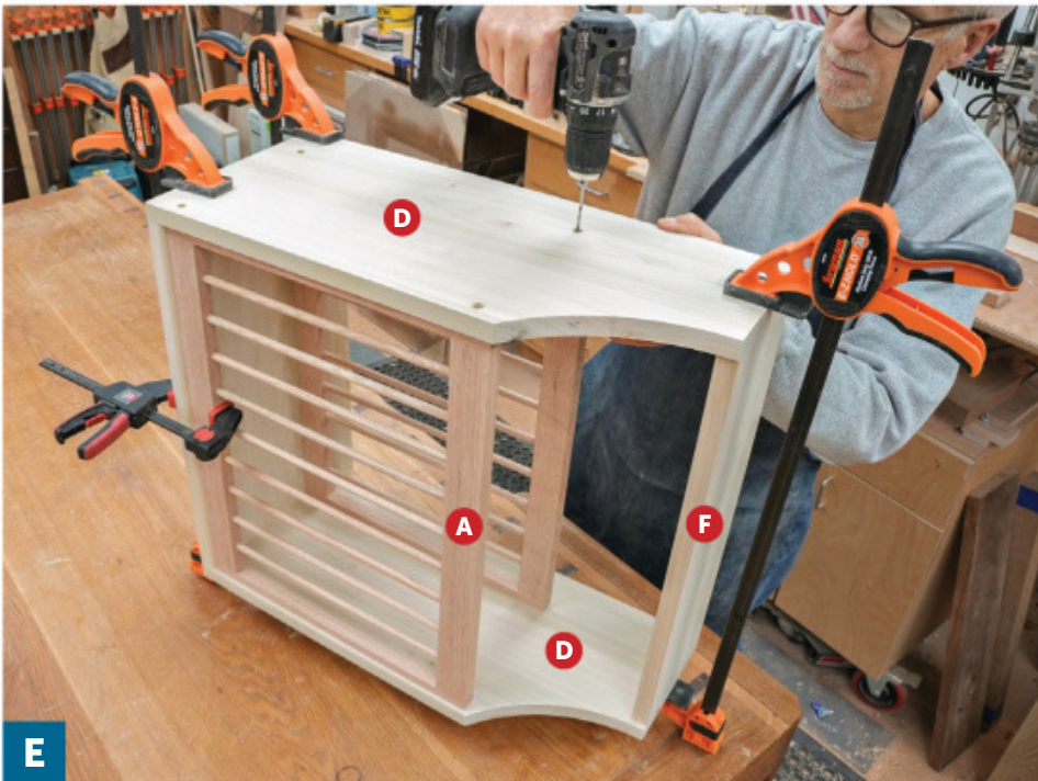
Counterbore screw holes in the case sides to join the divider assemblies, paying careful attention to the offset distances of the dividers from the front and back edges of the case.
