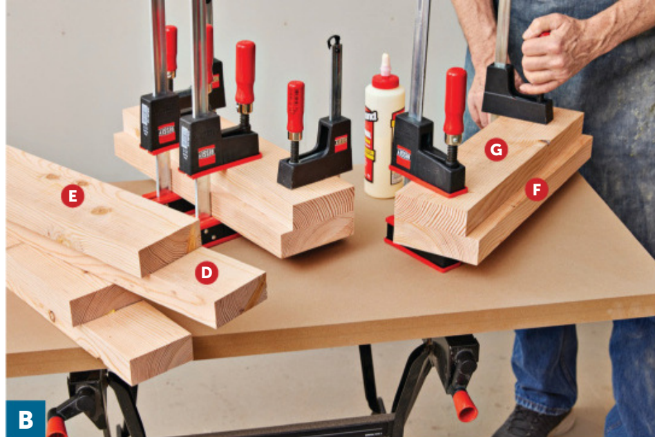
B Make sure the bottom edges of the fillers and rails remain aligned as you clamp the pieces together. Holding the pieces by hand for a minute before clamping allows the glue to grab, reducing slippage.
