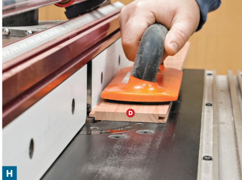
H Install a straight bit in the router table and gradually remove material from both sides of each tongue until it fits well in a slat groove.
