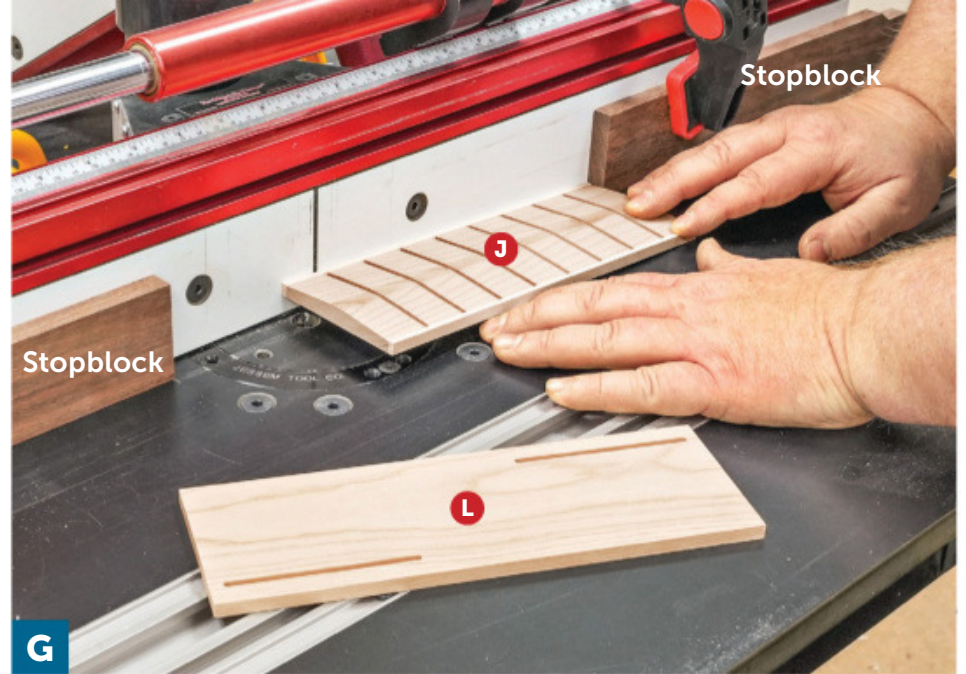
G Using a pair of stopblocks clamped to the fence, carefully lower the workpiece onto the spinning \frac{1}{8} " spiral bit and rout stopped grooves in opposite corners of the floor (L) and roof (J).
