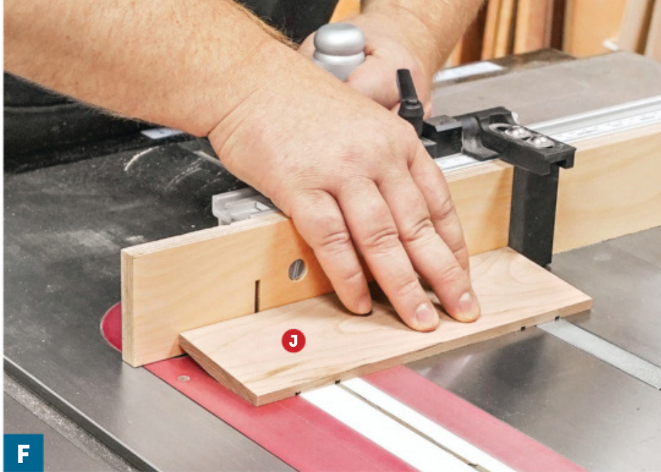
F Hold the beveled faces of the roof (H) flat on the tablesaw to cut the kerfs on the top. Use a stop to position the kerfs, flipping the roof end for end between cuts and then repositioning the stop.
