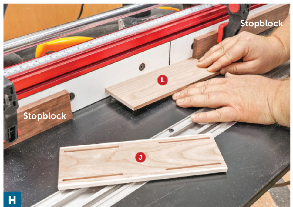
H Reposition the stopblocks to rout the grooves on the opposing corners. To rout the grooves for the doors, reposition the fence and stopblocks.
