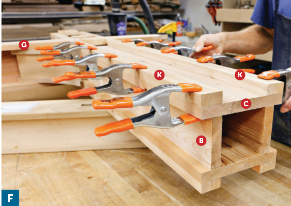
Clamp the trim (J, K) flush with the edges of the sleeve sides (C) and against the arms (G).
