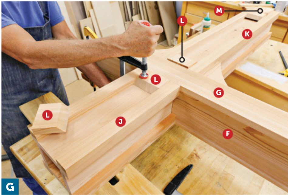
Glue short fillers (L) on all four faces on the upper portion of the sleeve, and only on the side faces on the lower portion.
