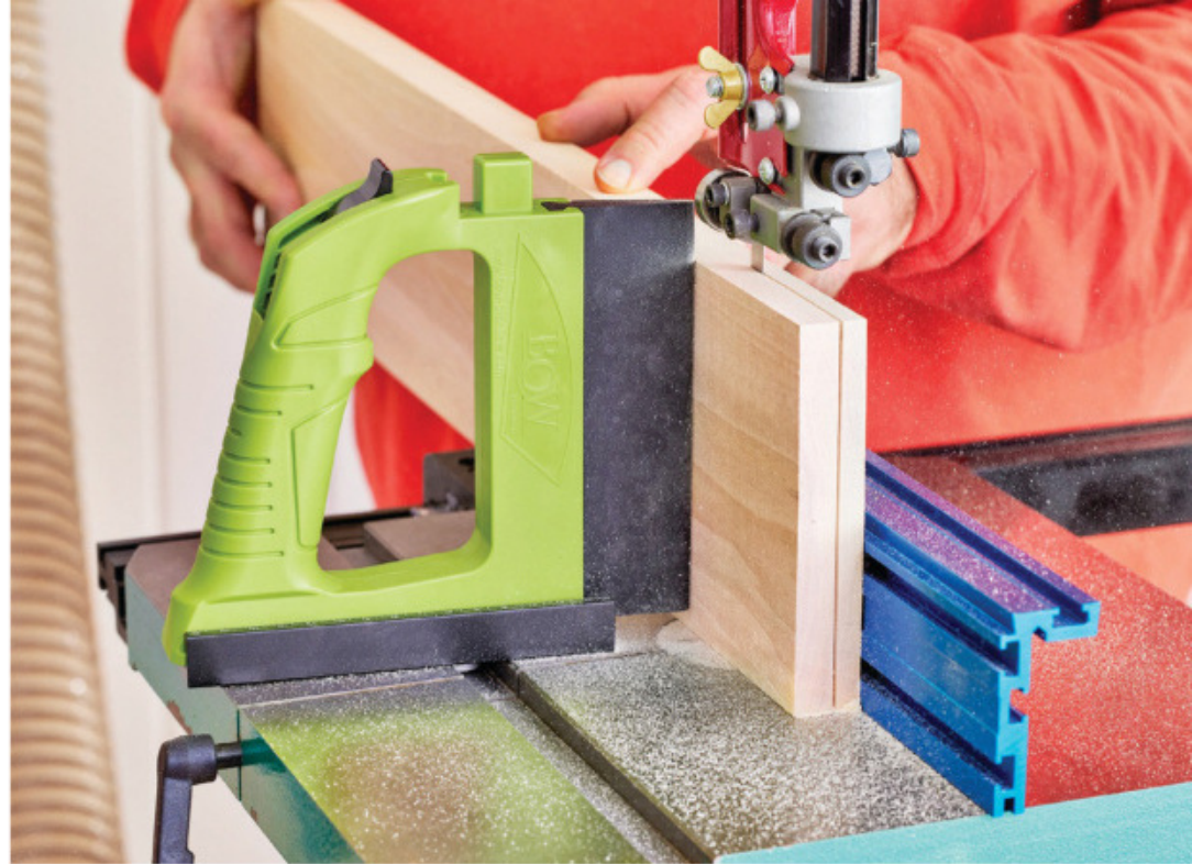
This tall featherboard by Bow Products is designed specifically for resawing at the bandsaw. A 6" flexible silicone feather provides pressure across the entire face of the board.
