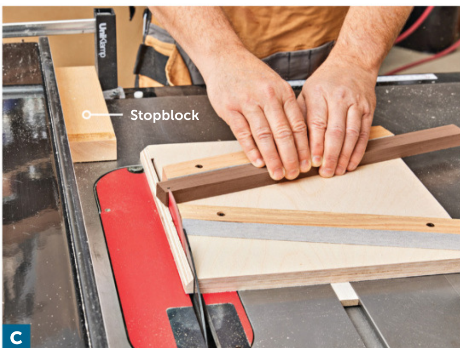
C Trim your first segment blank using the rear sled fence. This cuts the end at 15°. This first cut doesn't require the stopblock.
