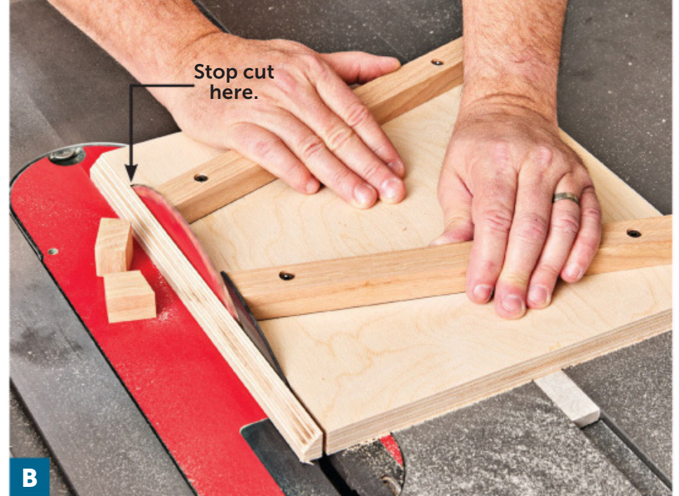
B Raise the blade to cut through the fences, and then cut a kerf in the base. Stop the cut just beyond the rear fence.
