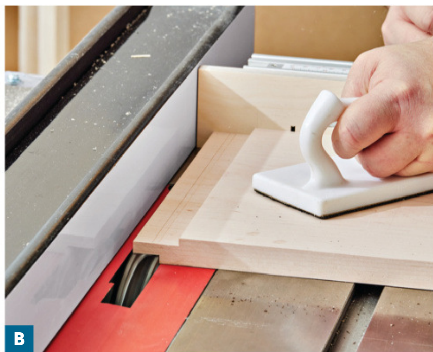
B Set your fence to cut the tenon to proper length. Cut the cheek on one side, making multiple passes. Then flip the panel over and cut the cheek on the other side.
