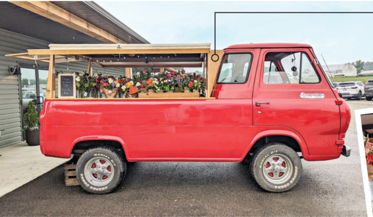
After his daughter bought a 1967 Ford Econoline to promote her flower arrangements at events, MARK BEACHY of Sugarcreek, Ohio, built out the cap on the back as a display area. White oak construction and several coats of spar varnish make the rack beautiful and durable.
