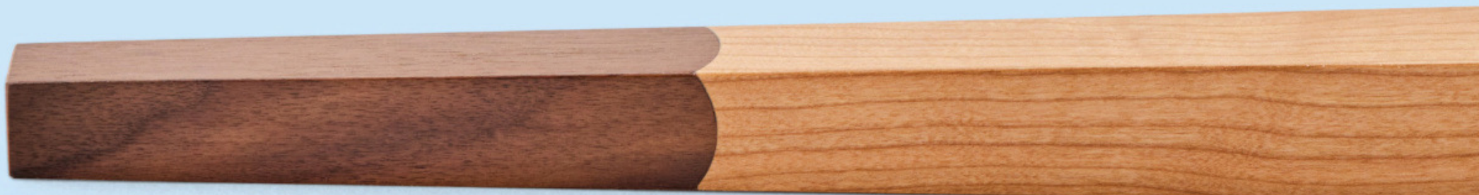
Glue the sock assembly together around the tenon. Then slide the assembly into place.
