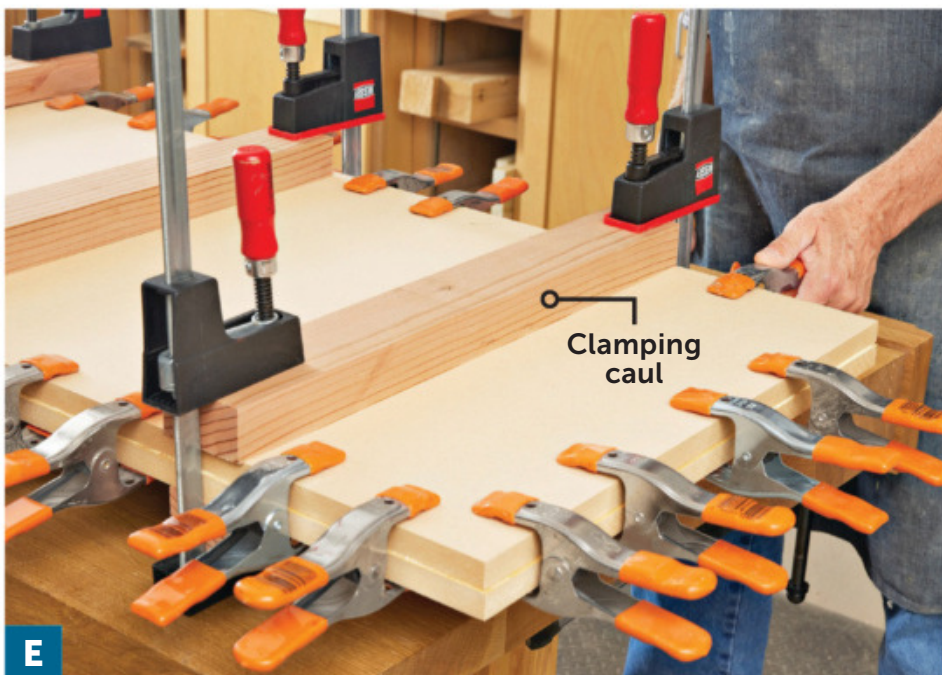
Use a roller to spread glue evenly on the face of one MDF blank, then clamp the two blanks together to form the benchtop (M). Clamping cauls apply pressure to the center of the panels.
