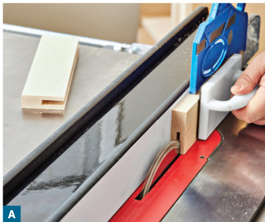
A Center a \frac{1}{4} " stacked dado blade on the end cap stock and cut the groove. For our dense maple, we made a pass with a regular blade first to remove some waste and make it easier to complete the groove.
