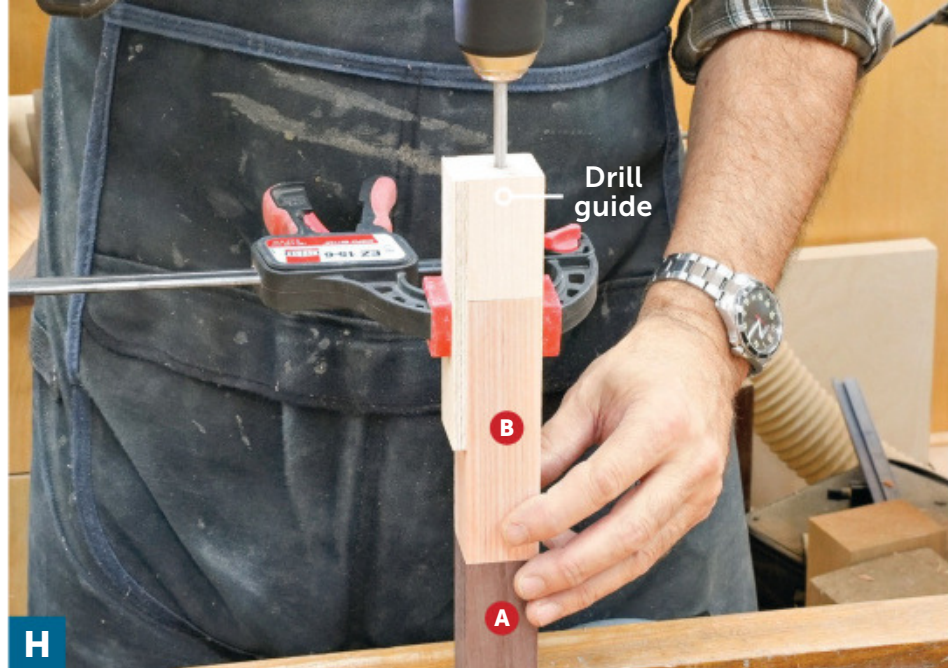
H At the drill press, make a drill guide by drilling a \frac{1}{4} " centered hole through a block of scrap sized to match the leg. Add a cleat to align the guide with the leg. Then drill a centered hole in the end of each leg.
