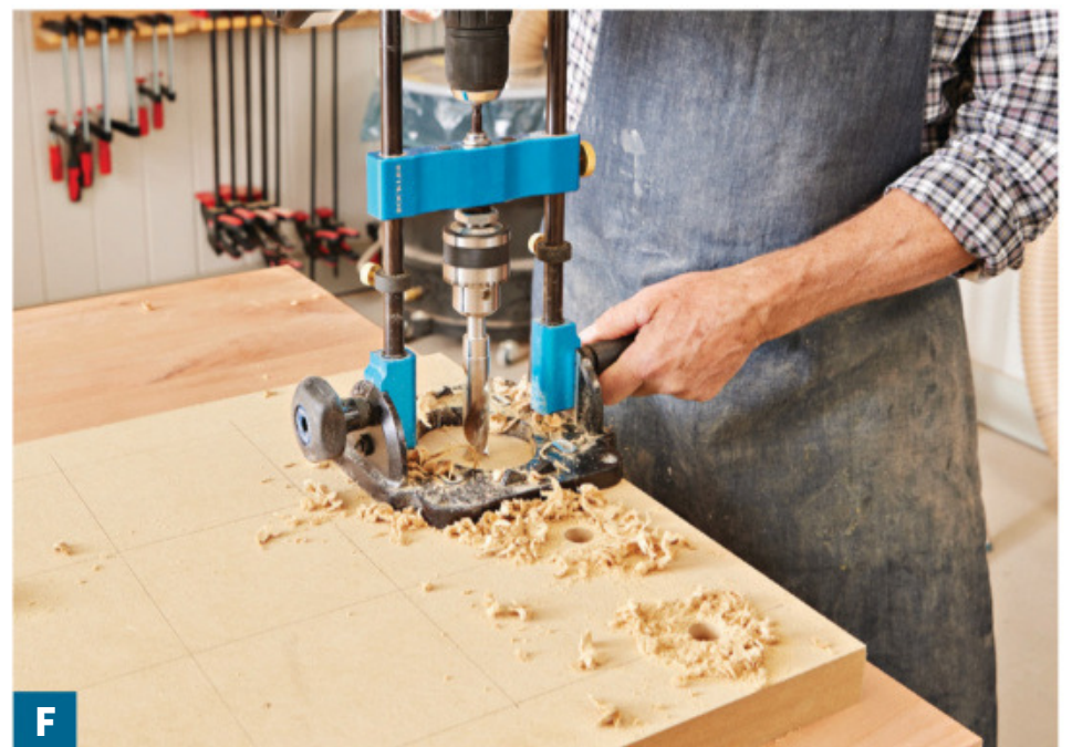
A portable drilling guide makes drilling perpendicular bench-dog holes quick and accurate. We used a \frac{3}{4} " brad-point bit from Lee Valley that cut more quickly and cleanly than others we tried.
