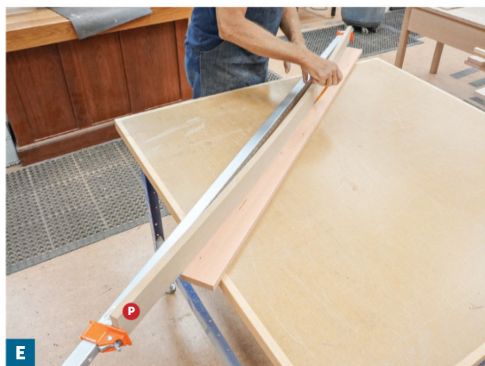
E To create the curve for the face-frame bottom rail (P), flex a piece of \frac{1}{4} " plywood or hardboard between the layout points, or squeeze a piece of \frac{1}{2} " or \frac{3}{4} " MDF in a long bar clamp.
