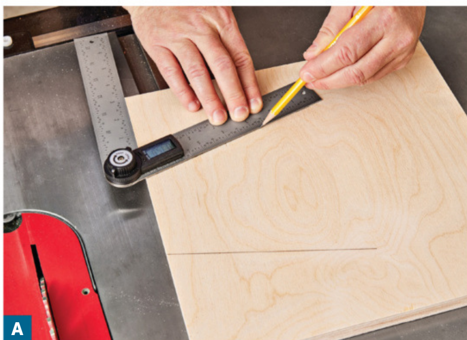
A Lay out the fence locations at opposing 15^\circ angles from one edge of the base. A digital angle finder provides accurate measurement.
