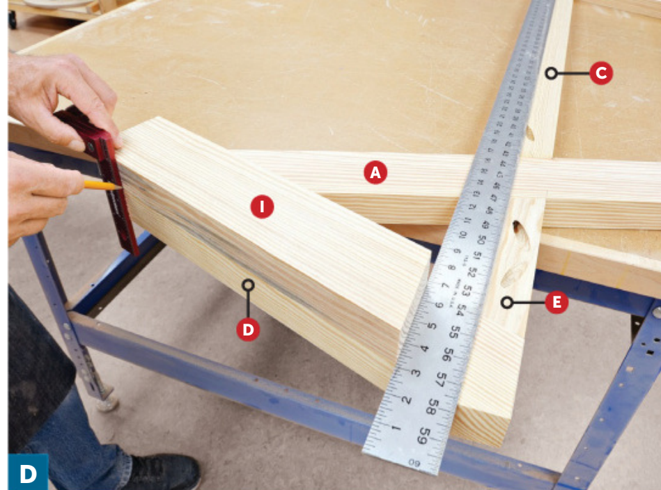
Miter one end of the inner frame seat leg (I) and butt it against a straightedge in order to mark the part for length.
