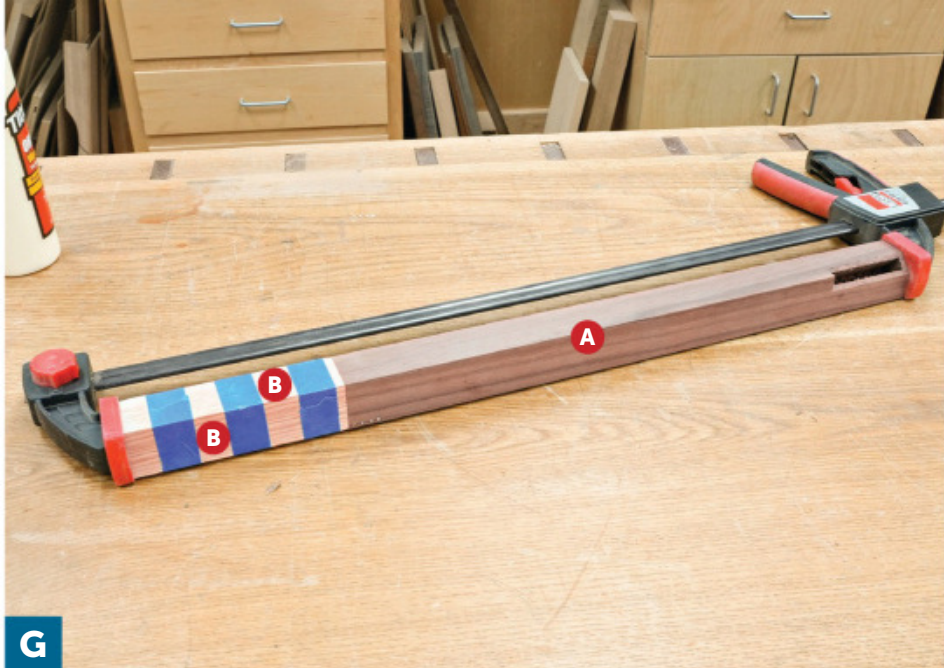
G Use several strips of painter's tape to hold the sock assembly against the faces of the core and light pressure from a bar clamp to hold it against the shoulders while the glue sets up.
