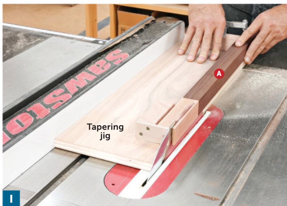
I Using the tapering jig, taper all four sides of each leg, rotating the leg after each cut. Finish-sand the legs after tapering to remove any saw blade marks.
