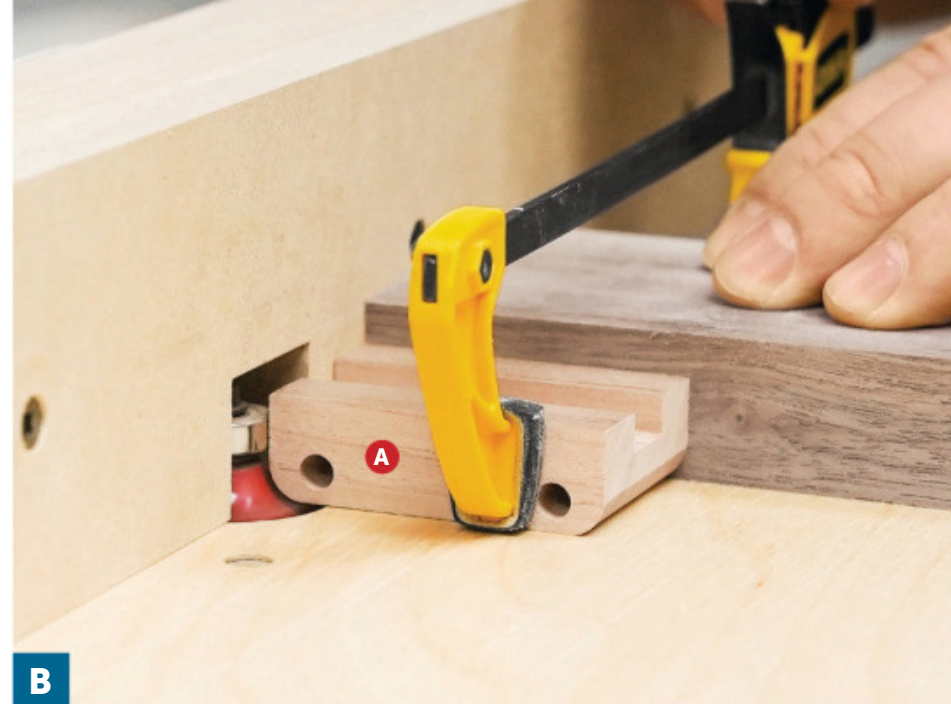
B Install a \frac{1}{4} " round-over bit in the router table. Clamp the truck frames to a backer block to keep your fingers away from the bit and prevent tear-out as you rout across the grain.
