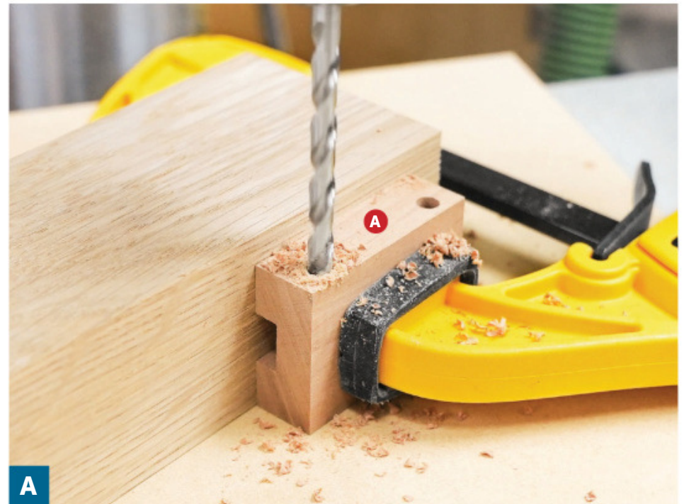
To ensure straight holes for the axle pegs, clamp the truck frames (A) to a backer block on your drill-press table, then drill \frac{1}{2} "-deep holes using a \frac{7}{32} " brad-point bit.
