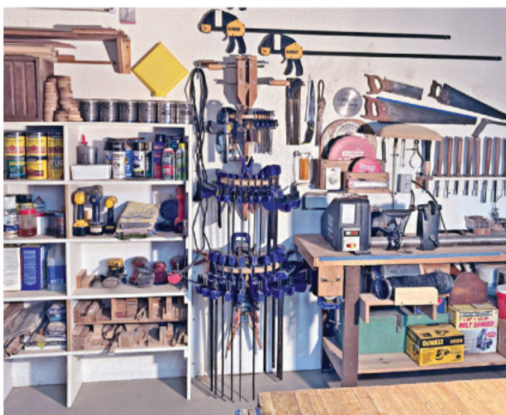
OSB-lined walls simplify attaching racks for hand tools, and other accessories. The semicircular clamp rack reduces their storage area.
