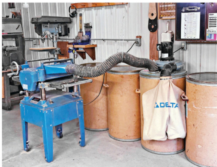
Roger's drum-mounted dust collection system easily handles large volumes of chips and dust from the planer.
