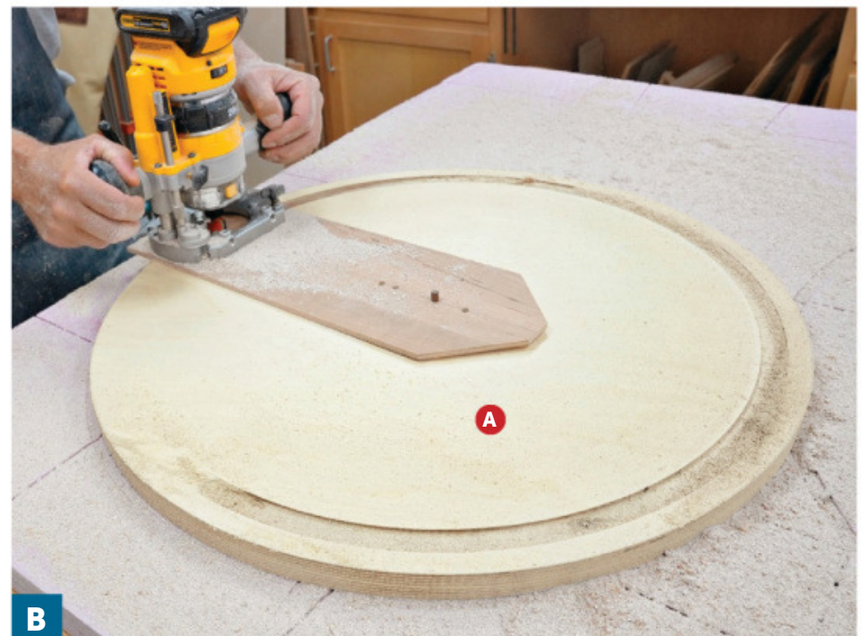
B Make multiple passes to rout a groove \frac{1}{2} " deep at a diameter to fit the rim of your dust-collection drum.
