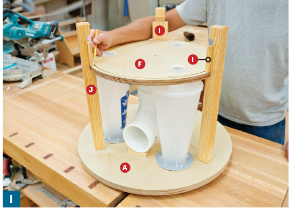
I Space the legs (J) evenly around the bottom (F). Dry-fit the cleats (I) and mark the centerline of each cleat onto the bottom. You will align the window seams on these marks later.
