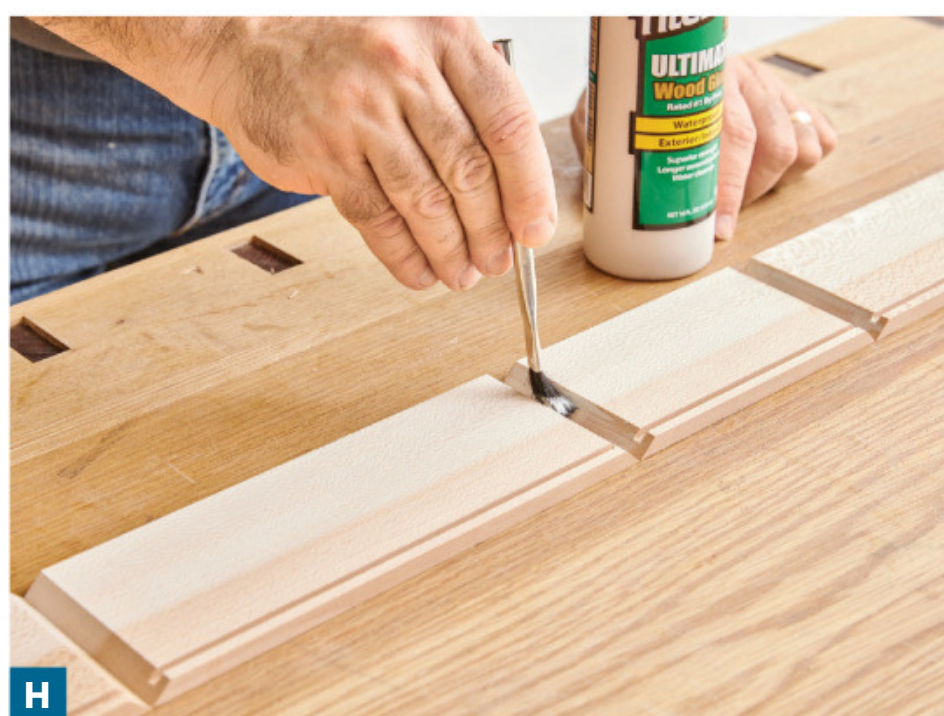
H Flip the taped box-side assembly over and apply glue to the miter joints with a glue brush. Use a sparing amount of glue to avoid excessive squeeze-out.
