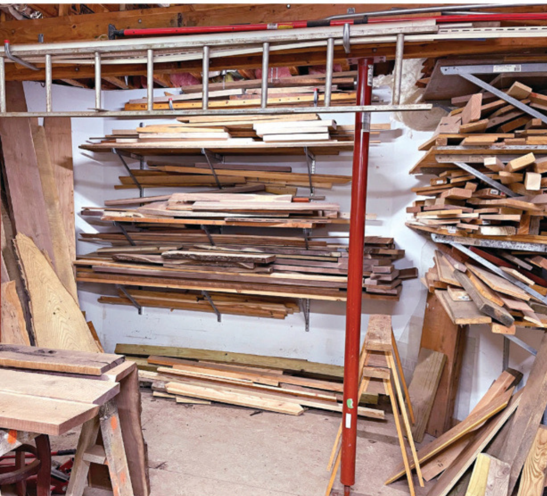
In a recessed area tucked into one corner of the shop, heavy-duty shelf brackets provide storage for lumber and cutoffs.
