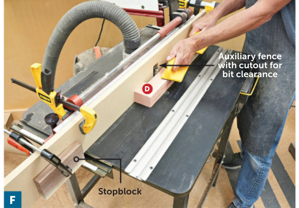
Install a \frac{3}{4} " flush-trim bit in the router table. Attach stopblocks to a long auxiliary fence to set the starting and stopping points of the cut. Position the fence \frac{1}{2} " behind the face of the bit to make a \frac{1}{2} "-deep cut.
