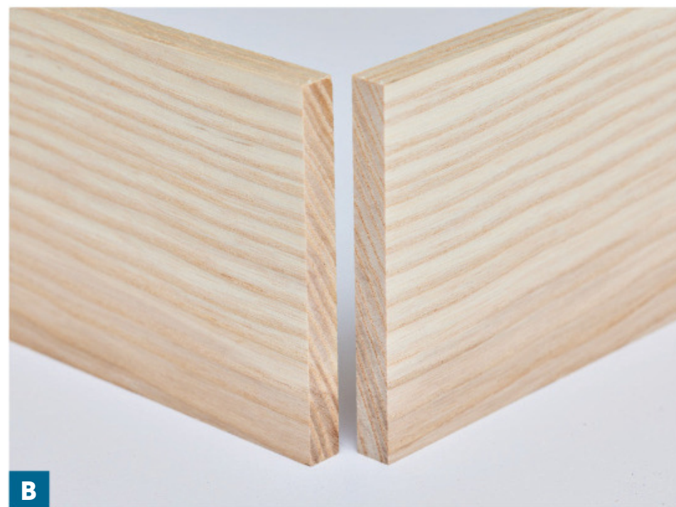
The end grain of plainsawn or riftsawn boards runs diagonally. Due to the kerfs created during resawing and mitering, the grain pattern shifts slightly, resulting in a close, but not-quite-perfect, match.
