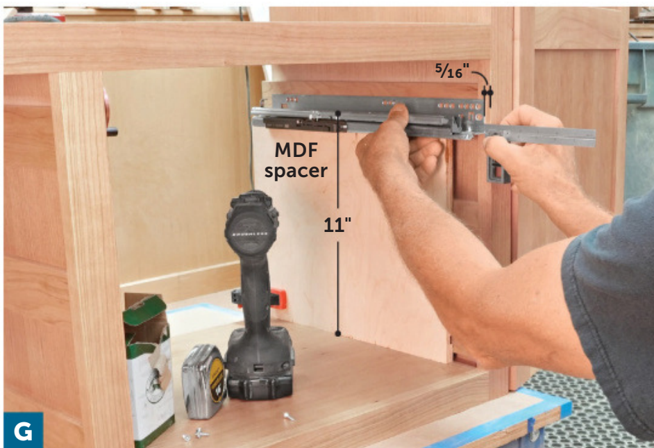
Use the scrap pieces you cut earlier to locate the upper two sets of drawer slides. The lower slides simply rest on the case bottom. Mount the slides \frac{5}{16} " back from the front of the face frame.
