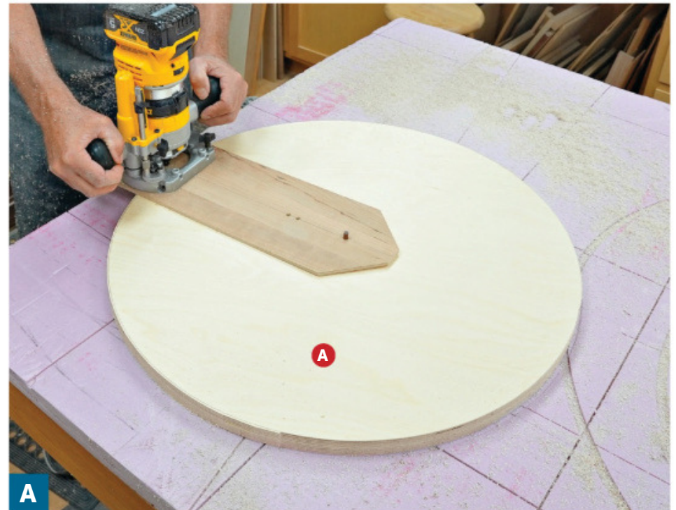
Mount your plunge router to a trammel and install a straight bit. Then trim the laminated lid (A) blank to 23 3/4" diameter.
