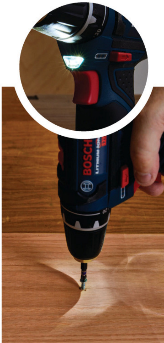
LEDs mounted near the drill base, such as the DeWalt ( left ) create smaller shadows than LEDs mounted beneath the clutch like the Bosch ( right ). LED power ranged from disappointingly dim to helpfully bright.
