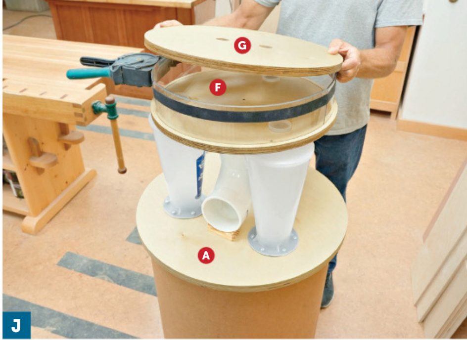
J Adjust tension on the band clamp to help align the windows with the groove in the top (G).
