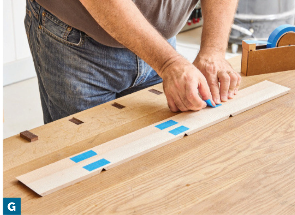
G Lay the box sides out in order, end to end with the outside faces up. Place painter's tape across the joints to act as hinges when gluing the box together.
