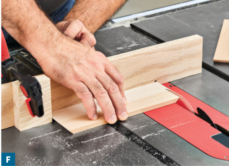
F Once all the pieces are mitered at one end, set up a stopblock to miter the other end and ensure that opposing sides of the box are identical in length.
