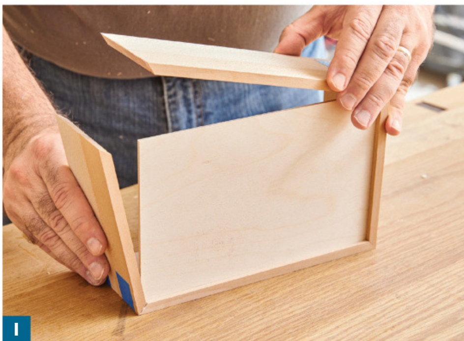
I Fold the taped sides around the bottom of the box and add tape to the last corner of the box to hold it together. Check that the miter joints line up at each corner.
