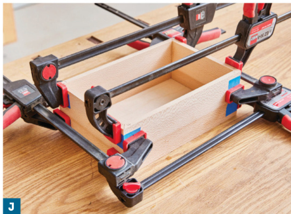
J The painter's tape should provide enough clamping pressure while the glue dries. But if the box is slightly out of square, apply clamps to pull the corners square.
