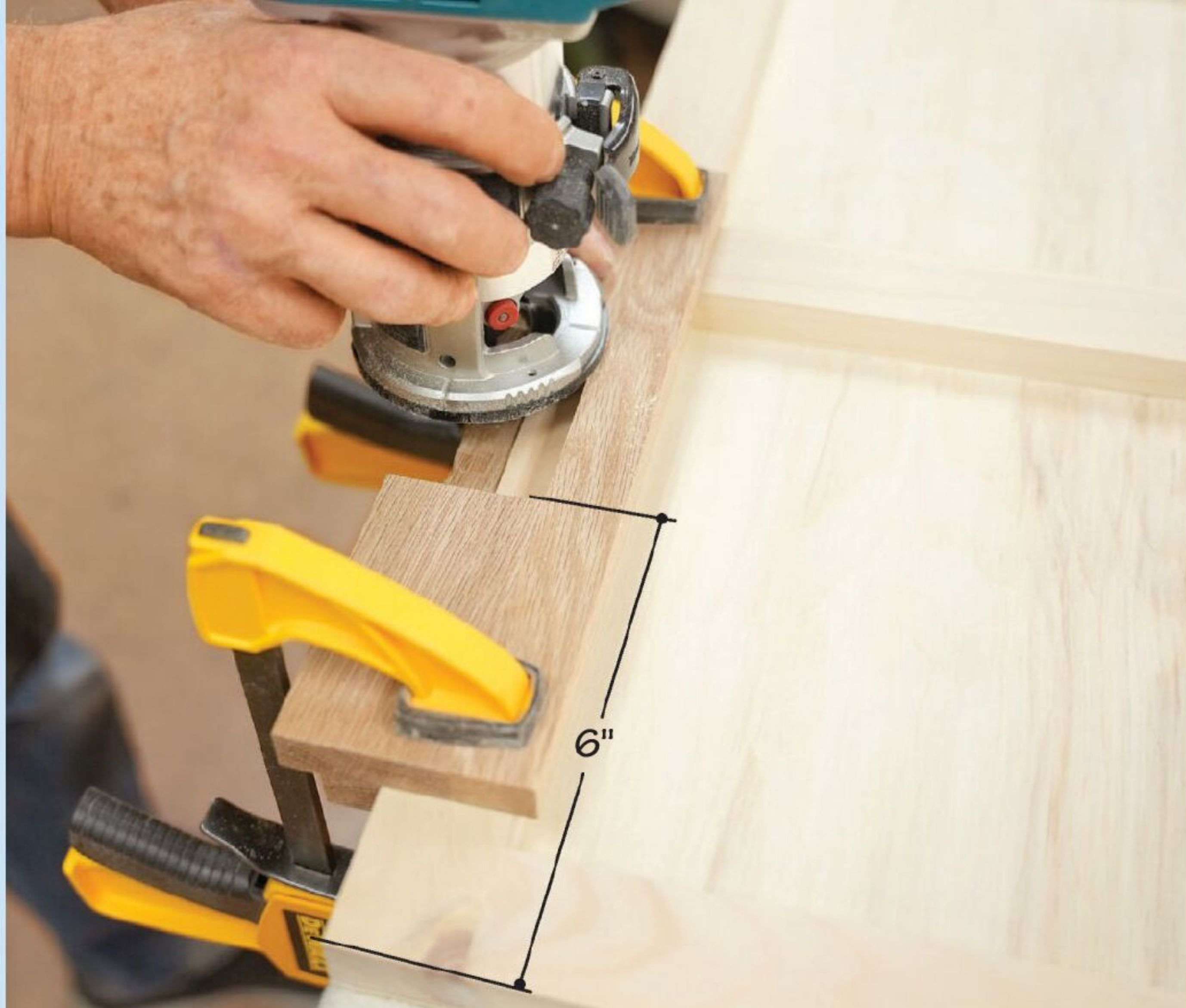
Clamp the hinge-mortising jig on the lid layout lines. Remove the waste using a 1/2" hinge-mortising bit set to cut the thickness of the hinge leaf. Transfer the hinge locations to the case and repeat.
