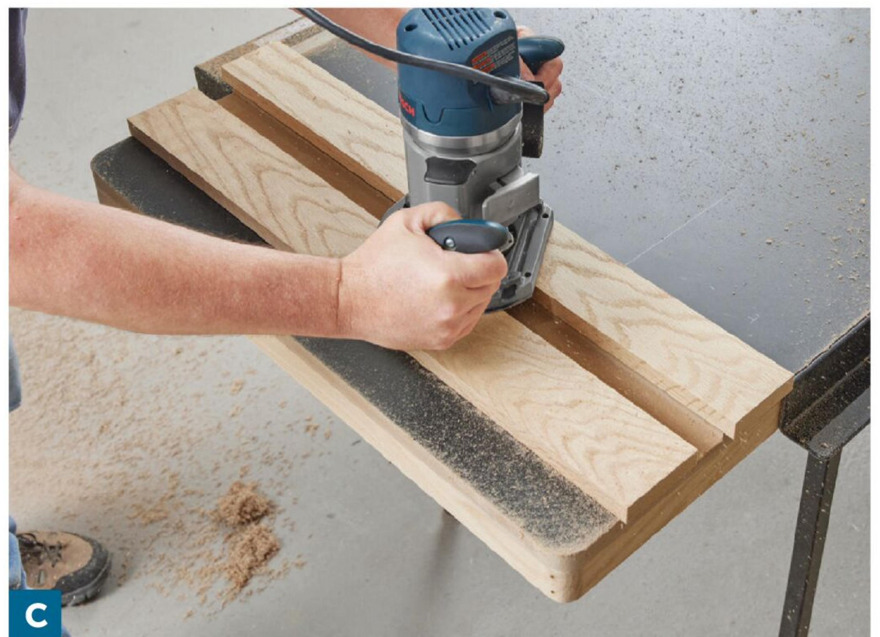
C Rout using a ½" dado-cleanout bit [Sources] . Make a pass along one guide, then work your way across to follow the other guide. Cut the groove in a couple passes to the final depth required for your track.
