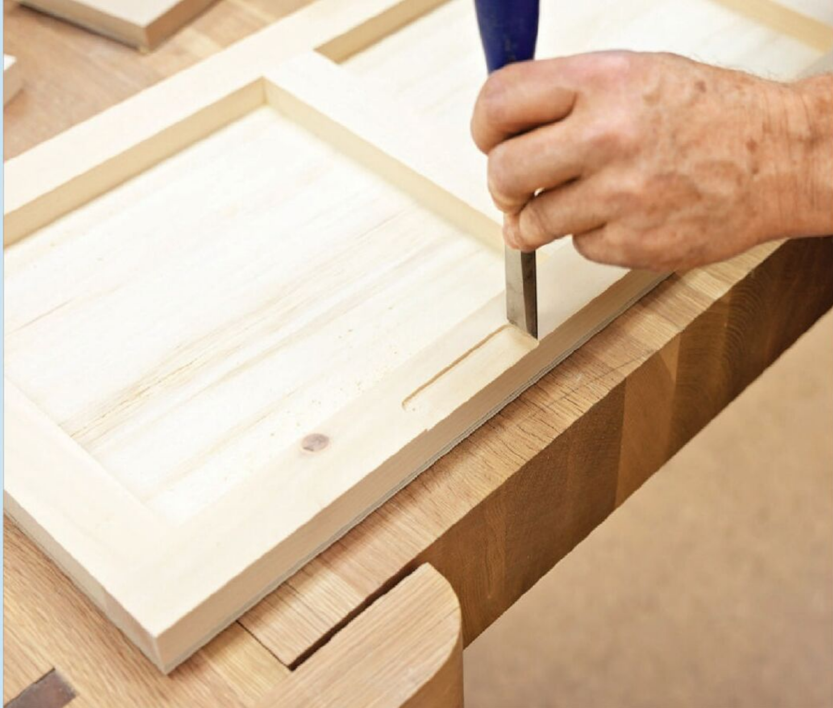
After routing the hinge mortises in both the lid and case, square up the corners of the mortises with a chisel, using the edges of each mortise as a guide.
