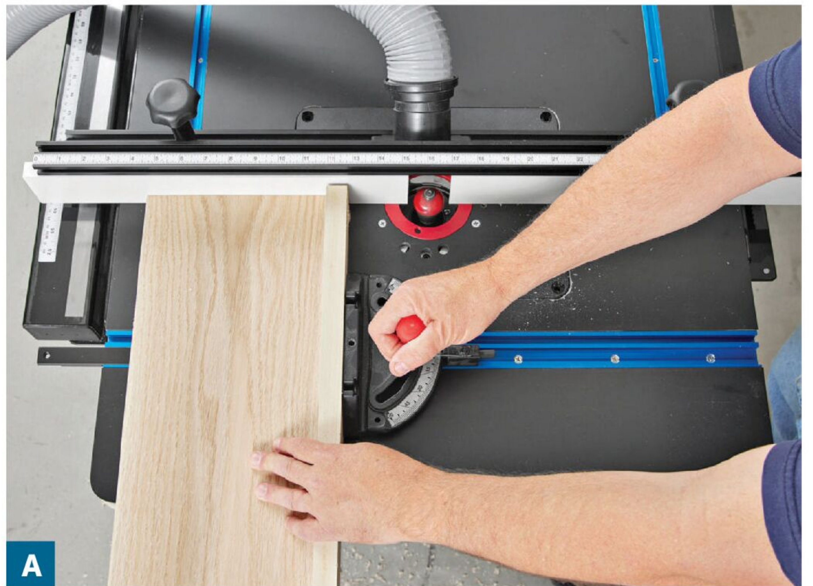
A Make your tabletop long enough to protrude beyond the ends of the fence rails so the miter-gauge bar can travel past the table edge without interference.
