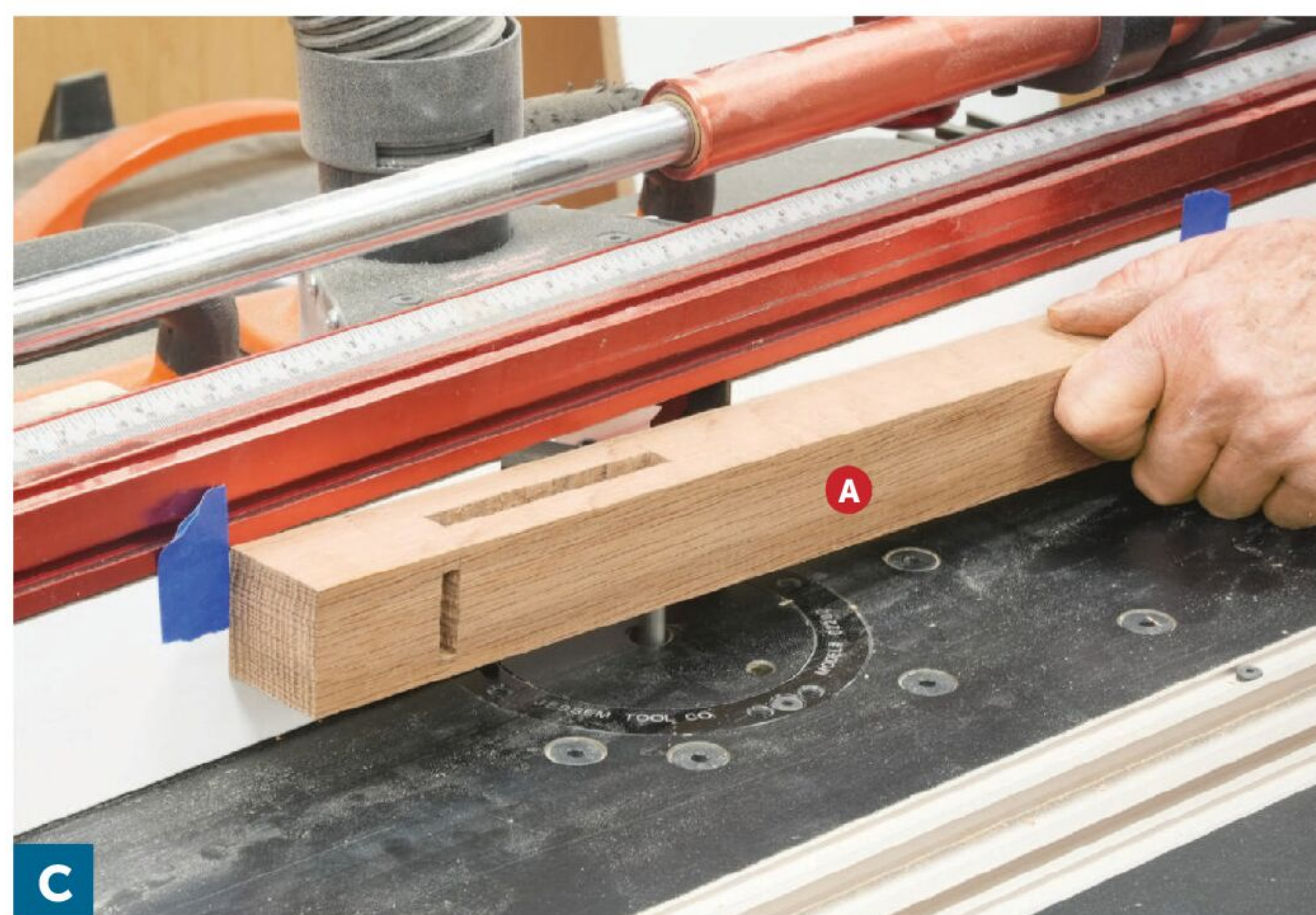
Position the fence to center the groove on the leg (A) and use masking tape to indicate start and stop points for the groove. Lower the leg onto the spinning bit, and rout the groove in one pass.
