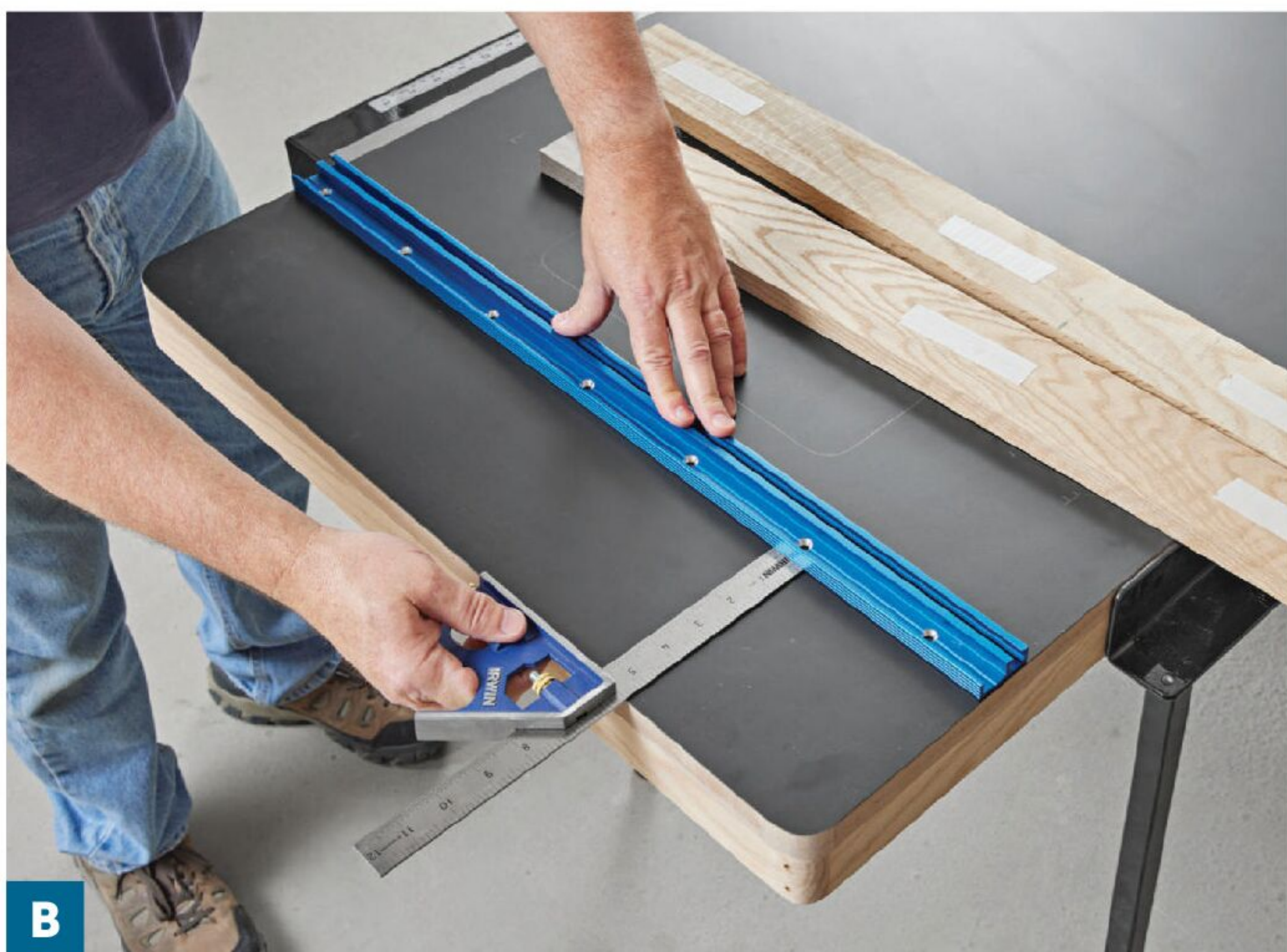
B Determine the distance from the table end to the miter-gauge track, then use a combination square to accurately position the track. Hold the track in place with a couple small pieces of double-faced tape.
