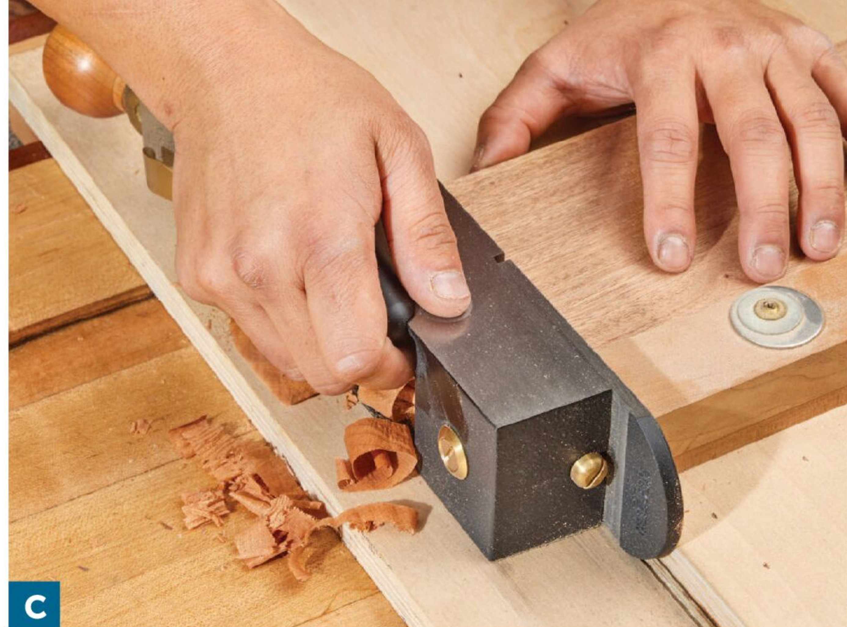
C Finesse the fit of the drawer front in the opening using a plane and shooting board on the end grain while checking the fit often.
