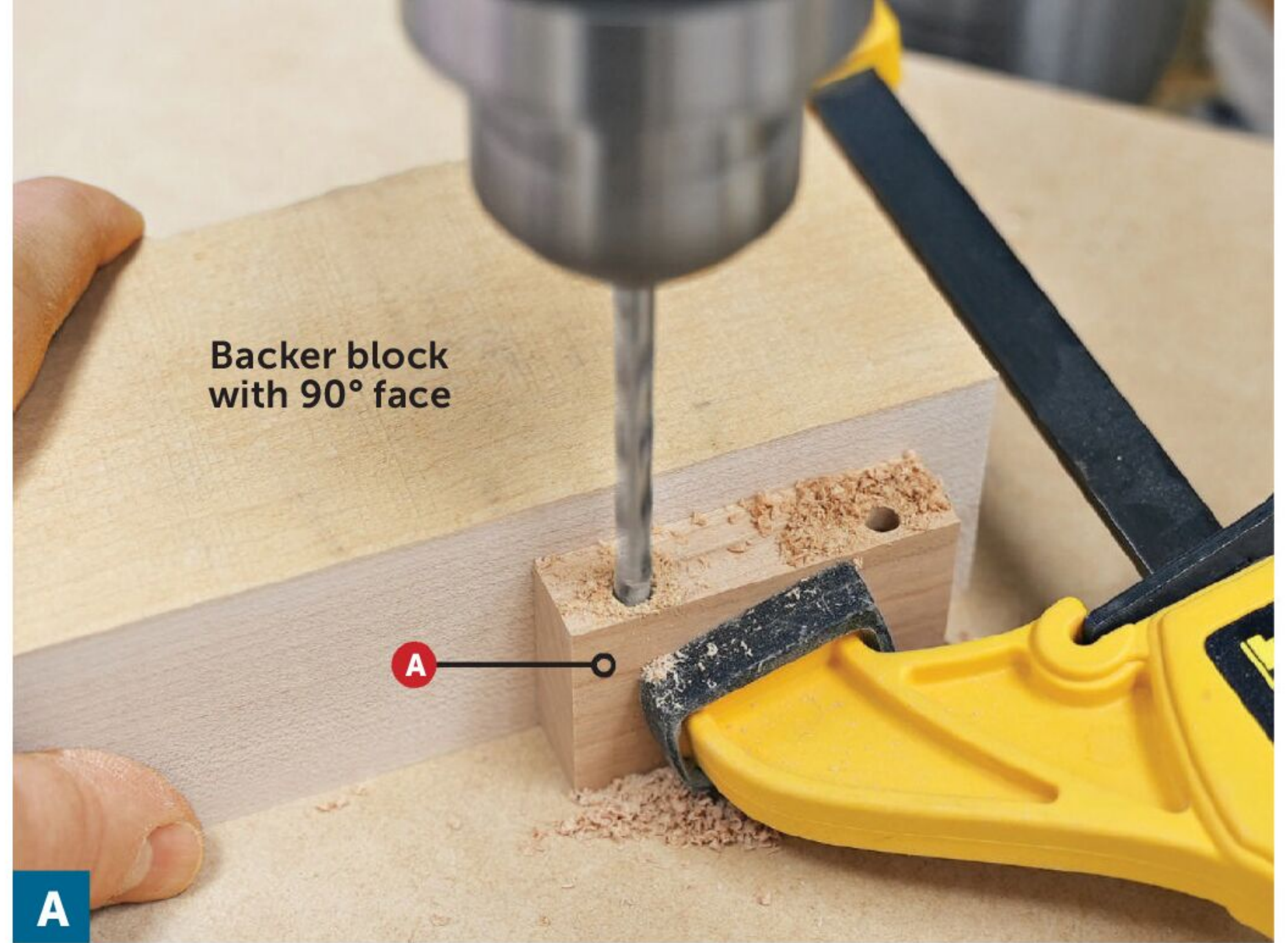
To ensure straight holes for the wheel axles, clamp the steering frame (A) against a backer block, then drill the holes at the drill press using a sharp brad-point bit.
