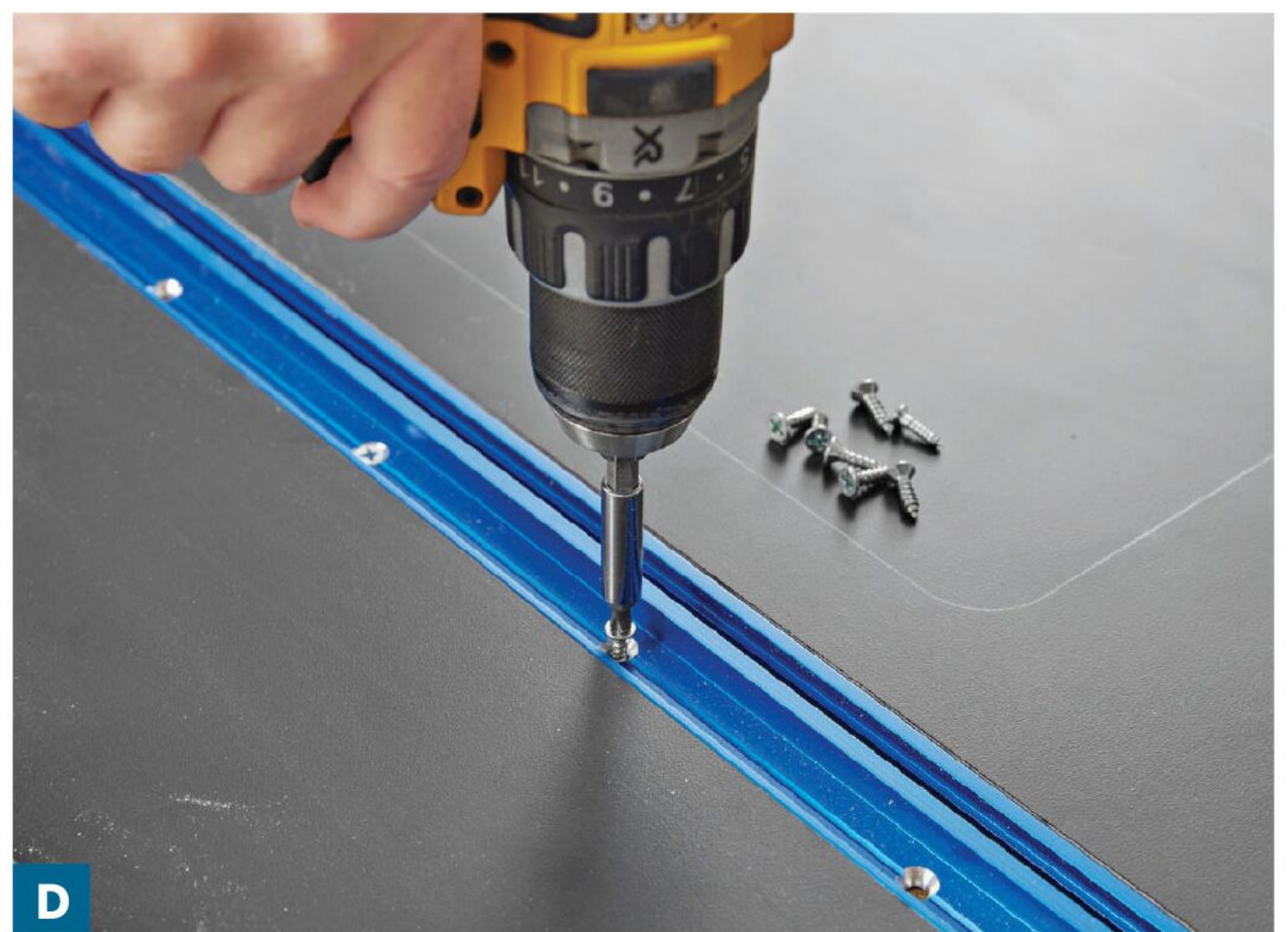
D Use a file to slightly ease the cut edges of the laminate, then screw the track in place. With MDF, you won't need pilot holes, but take care not to over-drive the screws and strip out the MDF.
