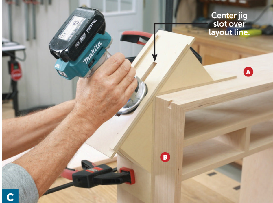
C Rout a set of dovetail slots in each corner of the case using a compact router. A shop-built jig clamped to the case guides the router as you mill each slot.
