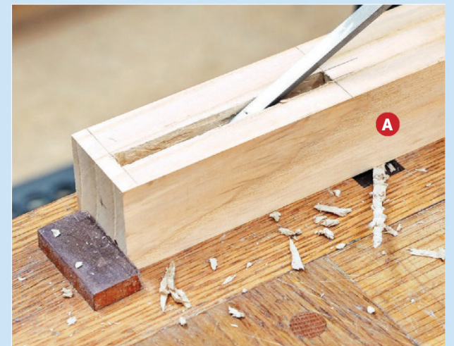
Use a \frac{1}{4} " chisel to clear out the bottom of the mortise. Position the chisel at an angle, with the bevel-edge down, and work from the center toward each end.
