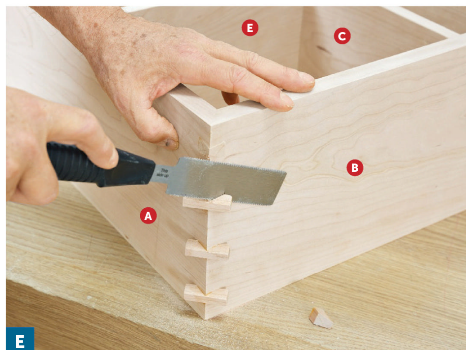
E Use a flush-cut saw to trim away the bulk of the dovetail key waste, taking care to avoid chipping out the key near the miter. Then sand the keys flush with the surface of the case.
