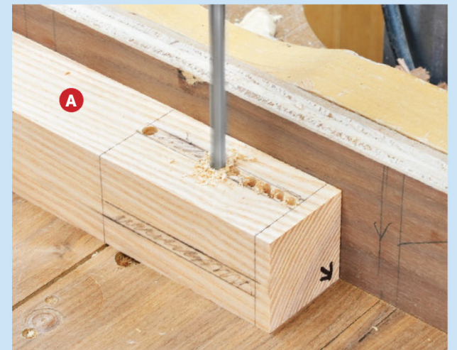
Remove the bulk of the waste between the ends by drilling overlapping holes as close as the bit will allow. Repeat the process for the remaining mortises.
