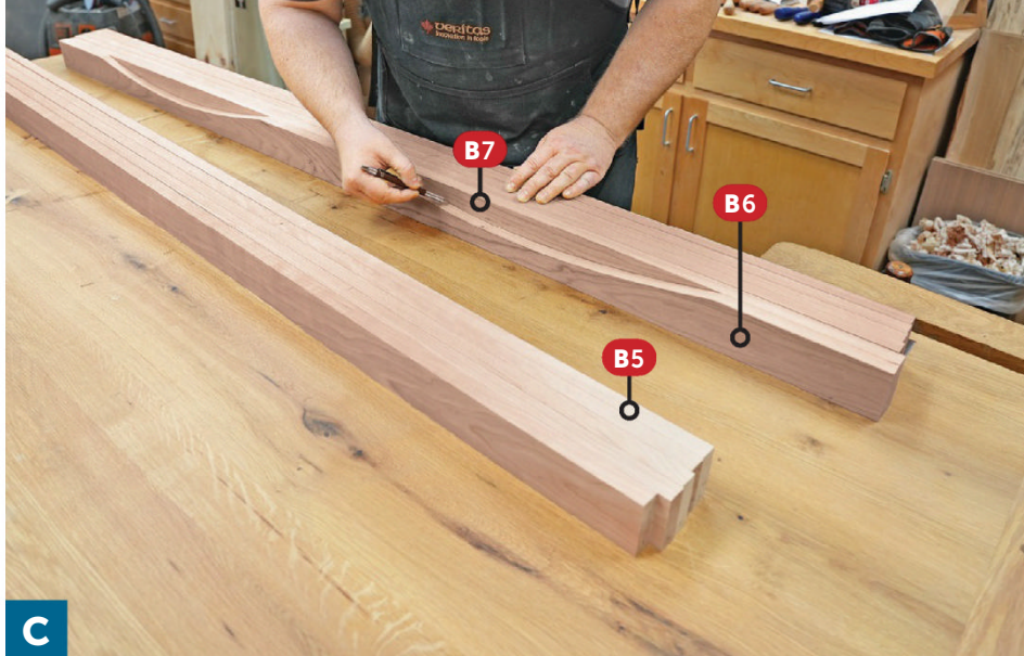
C Align the ends of seat rail B6 with seat rail B5 and trace the cutouts. Then align B6 with B7 and trace again.
