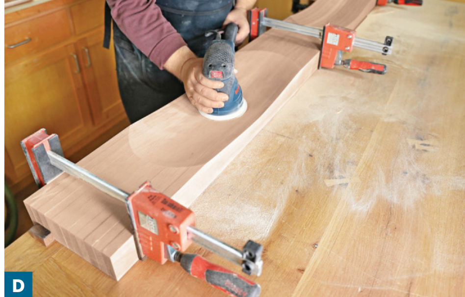
D Remove the saw marks with an orbital sander and 80-grit sandpaper, then sand up to 220 grit. We sanded the last few grits by hand.
