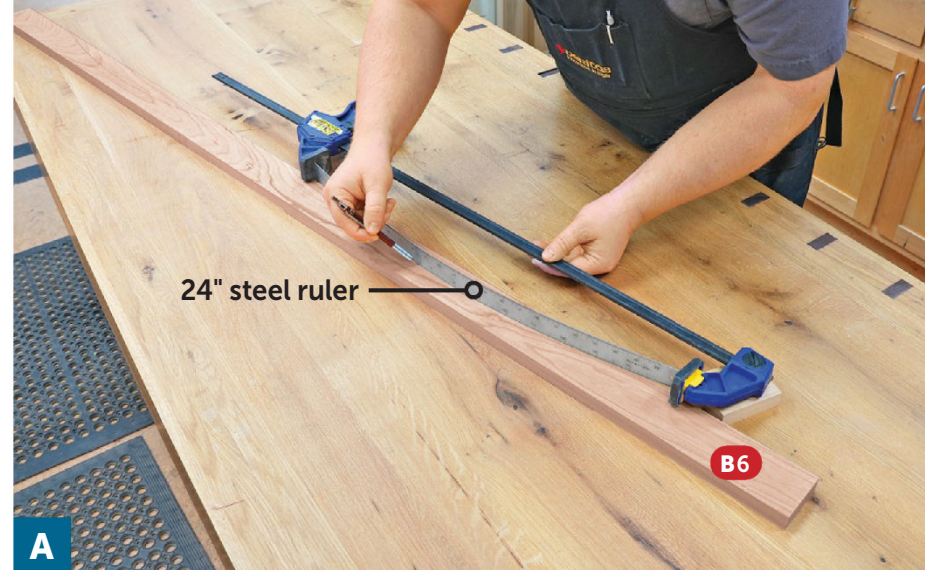
After marking reference points for both seat cutouts on the center seat rail (B), connect the dots by tracing along a fairing stick or steel ruler flexed in a clamp.
