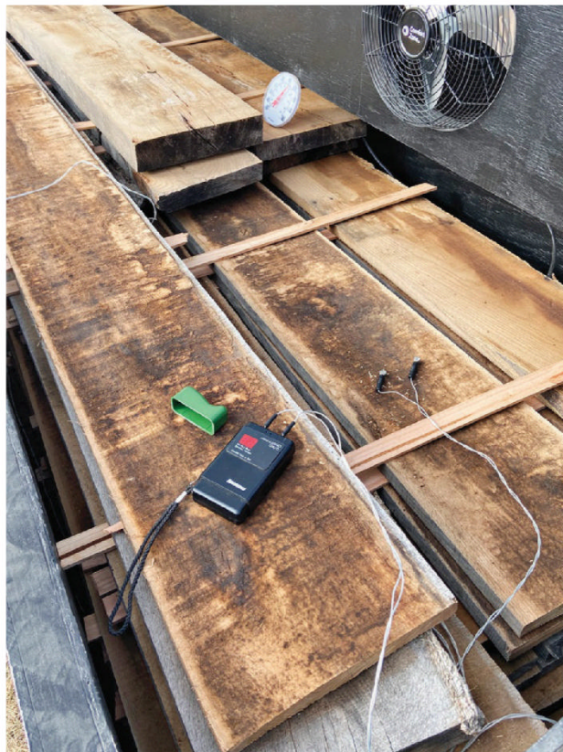
By sinking multiple sets of probes into boards in this solar kiln, we could attach the meter and get readings at different levels without having to unstack the boards.
