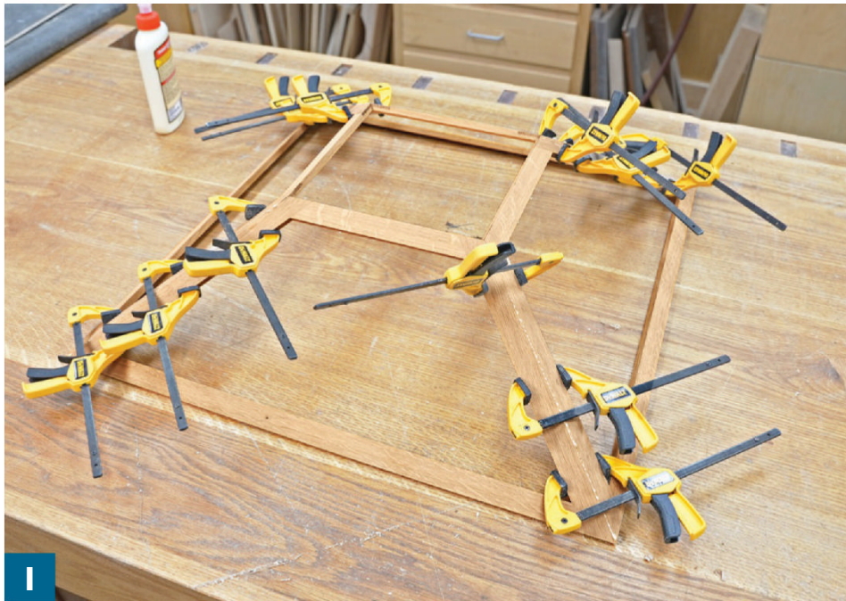
Keeping the top and bottom edges aligned, glue and clamp the frames, working on one corner at a time.
