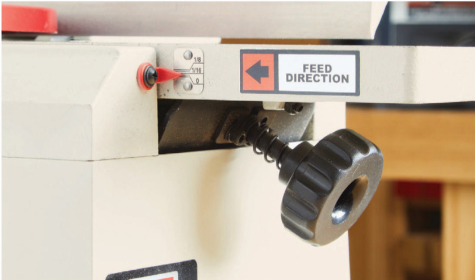
The Jet and Delta's depth gauges use 1/8" (actual-size) scales with few increments. They're tricky to set precisely, and there's no lock to ensure that the setting holds.
