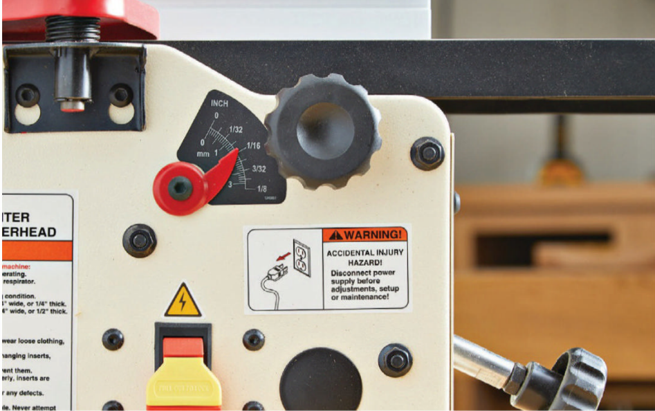
Ten of the test jointers use this indicator that magnifies the 1/8" cut depth capacity across a much larger scale. Few people will likely need its difficult-to-distinguish 0.1 mm increments, though.
