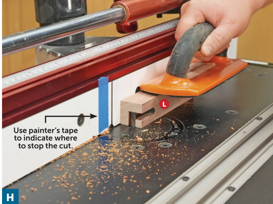
H Using a \frac{3}{8} "-diameter spiral upcut bit, rout the first mortise in all four legs (L). Then reposition the fence to rout the second mortise.
