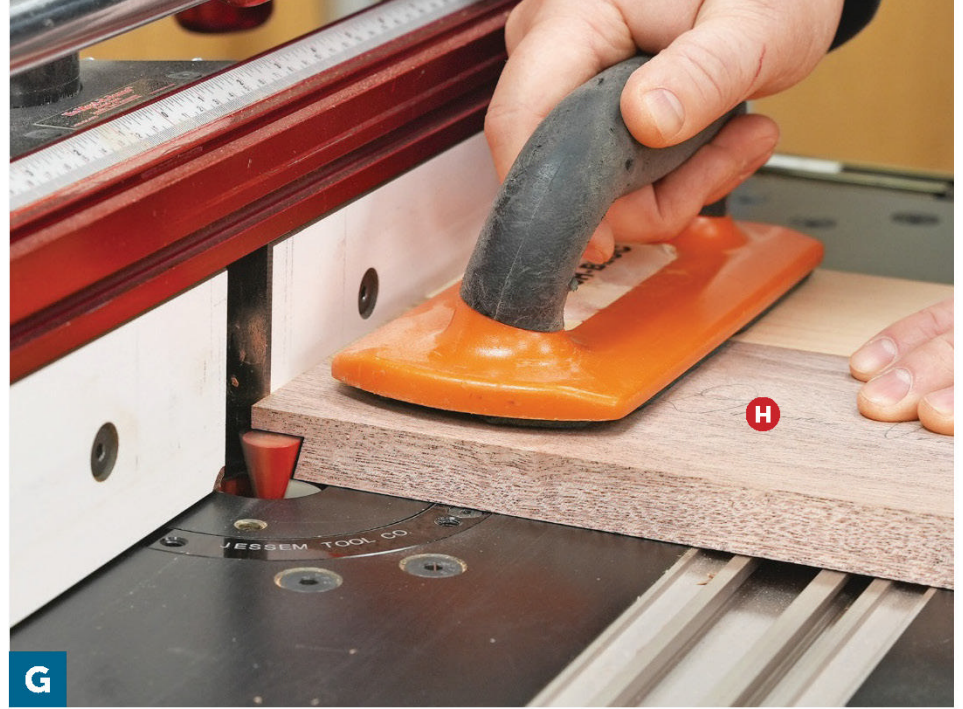
Position the router-table fence to expose \frac{5}{8} " of the router bit, then rout a rabbeted dovetail on each end of the drawer front (H).
