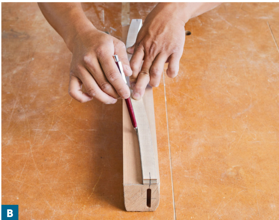
B Trace the outline of the template on the top face of the workpiece. This helps you visualize the position of the template, which will be hidden under the workpiece, as you cut.
