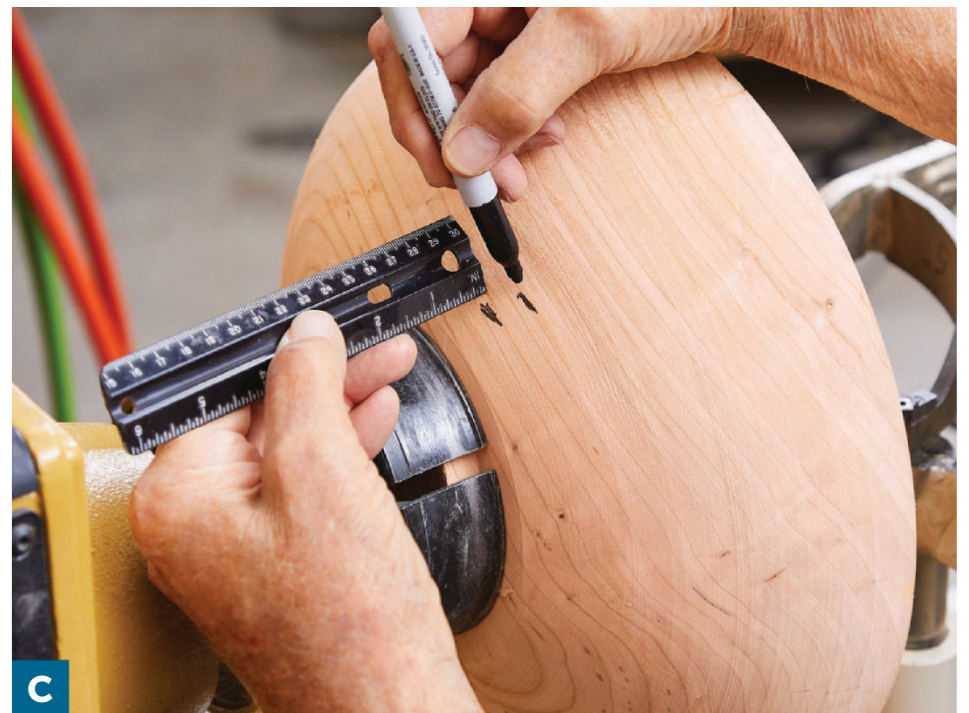
C Start from the bottom of the bowl blank (where the chuck jaws contact the tenon shoulder) and mark the thickness of the largest bowl. Then mark the kerf allowance ( \frac{3}{8} " for our aftermarket cutter).
