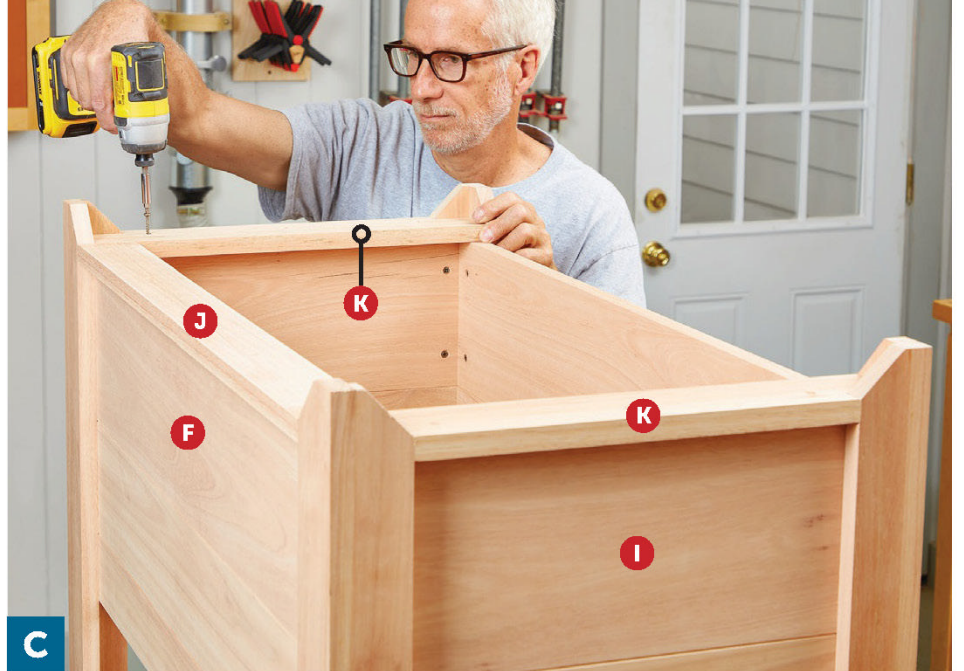
Screw the supports (J, K) to the bottom edges of the box assembly (F/I), flush with the outside faces of the legs.
