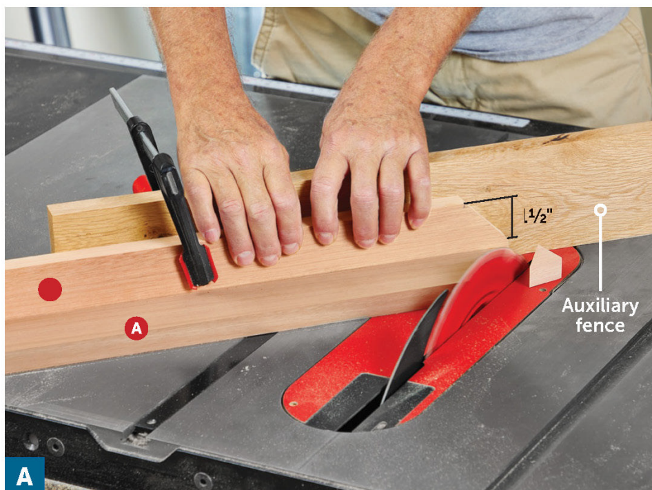
Adjust your miter gauge to 45° and cut the first taper. Then, rotate the miter gauge in the opposite direction to cut the other side.
