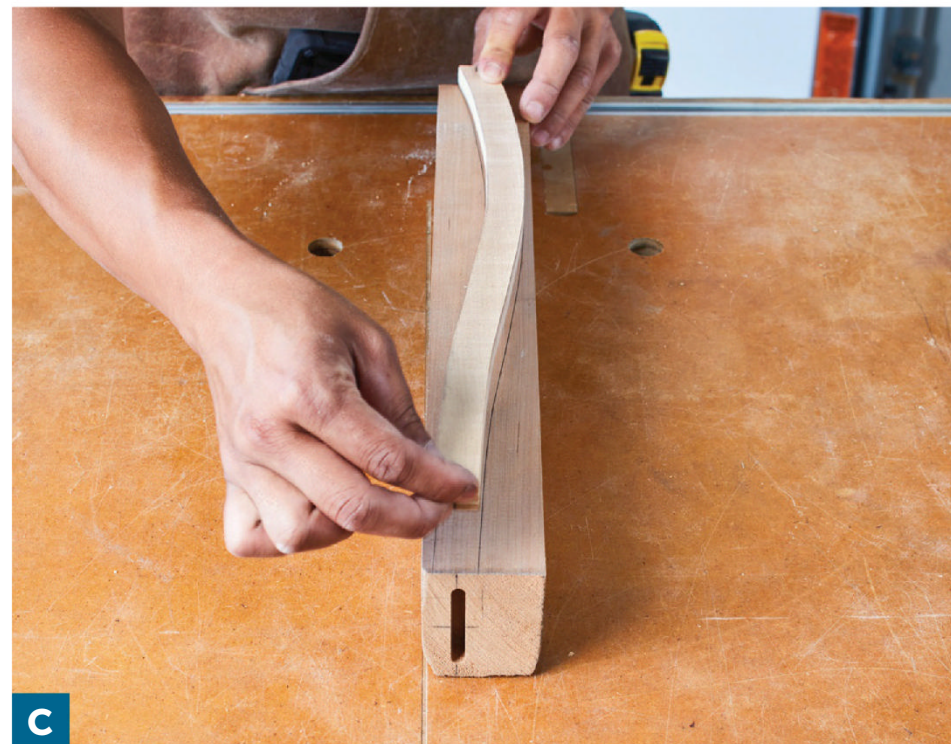
C Turn the workpiece over with the opposite face up. Then attach the template. Note that the template has to be flipped to mirror its position on the first face.
