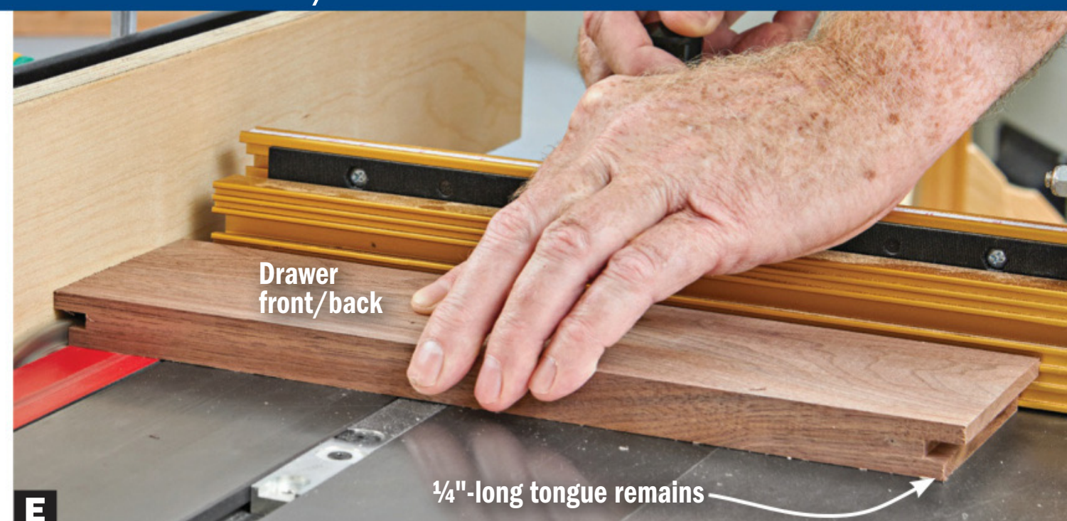
E Install an auxiliary rip fence and lower the blade to about \frac{3}{8} ". Cut away a portion of the lower tongue, leaving a tongue that fits the dado in a drawer side. Repeat for the back. Sand all parts and assemble.
