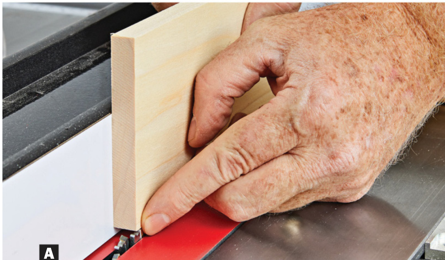
A With a dado stack and auxiliary fence in place, position the rip fence so the amount of exposed blades equals the thickness of the drawer side.
