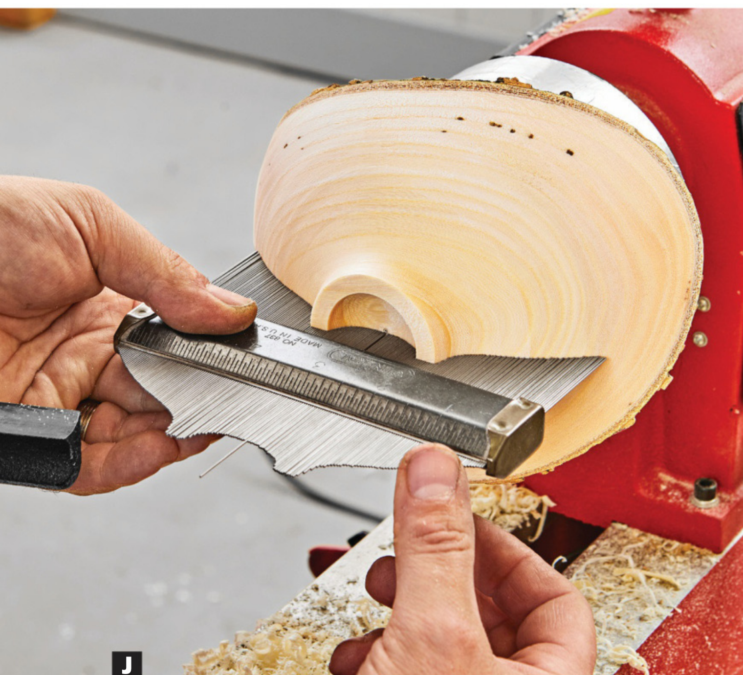
J After hollowing within the tenon, mark the center, reset the profile gauge, and retract the center pin.
