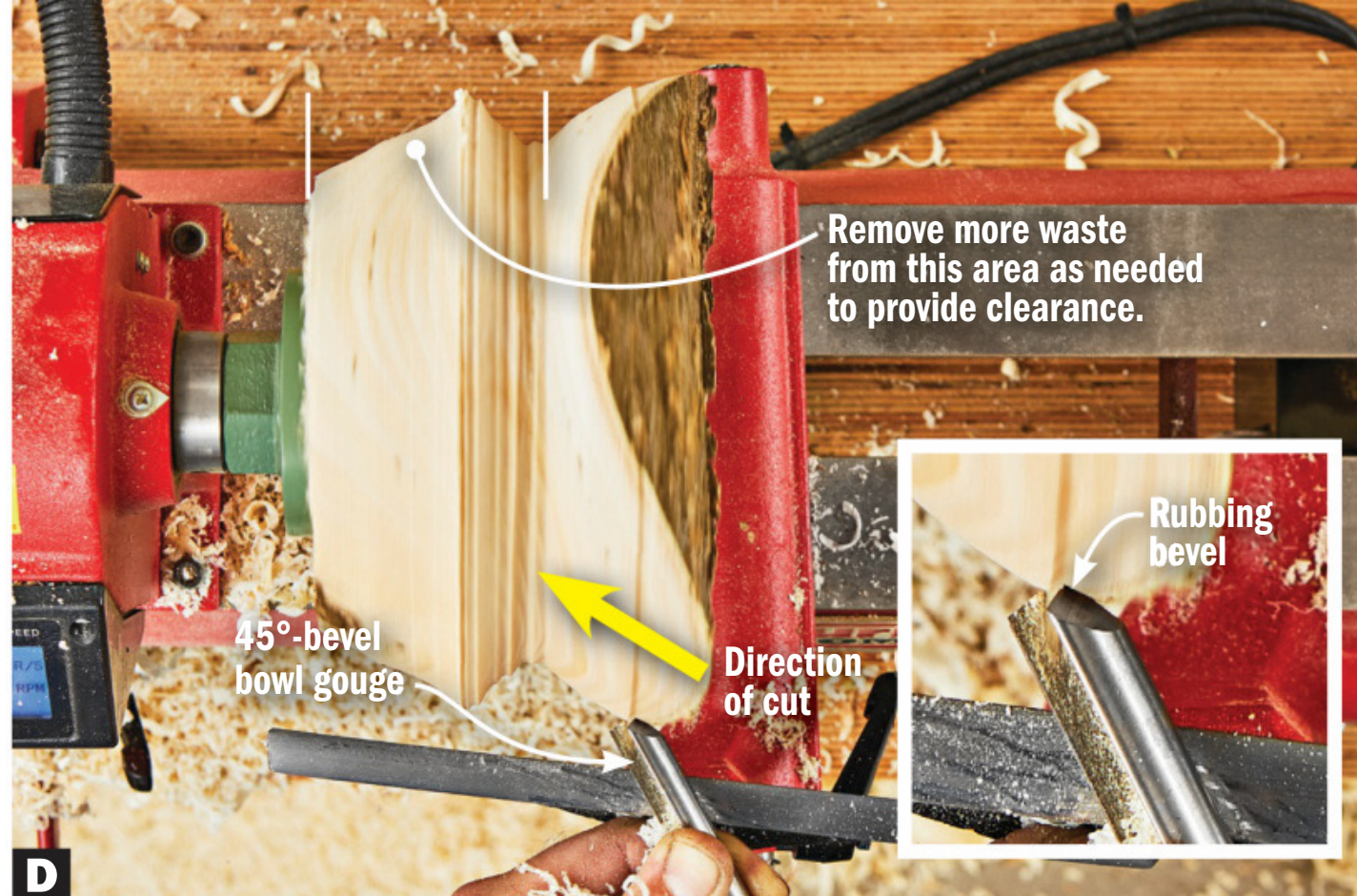
D Make push cuts from the rim to the bottom of the bark line. Cutting against the grain in this fashion prevents tear-out along the bark edge.
