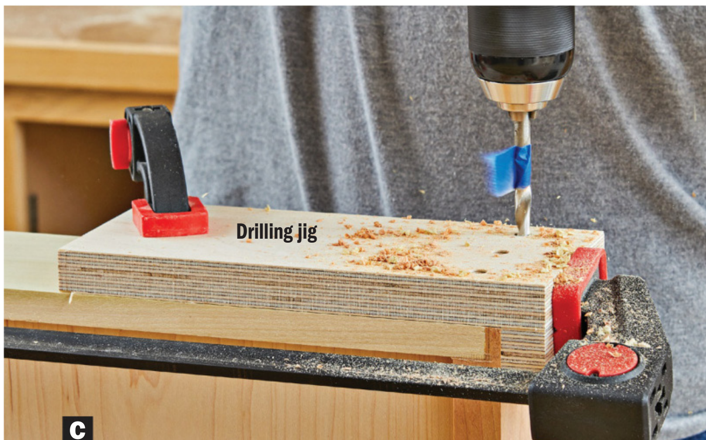
C Make a drilling jig to locate the dowel holes, clamp it to the drawer and drill the holes. Use a stop collar or masking-tape flag to set the drilling depth.
