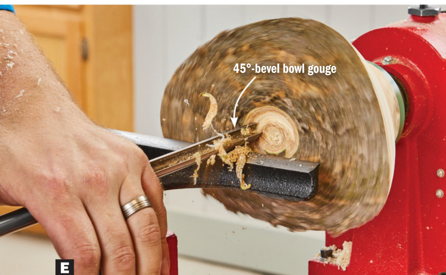
E Start with shallow cuts around the center. Swing the handle to create a dished cut. Expand the diameter and depth of the hollowed area with successive cuts.
