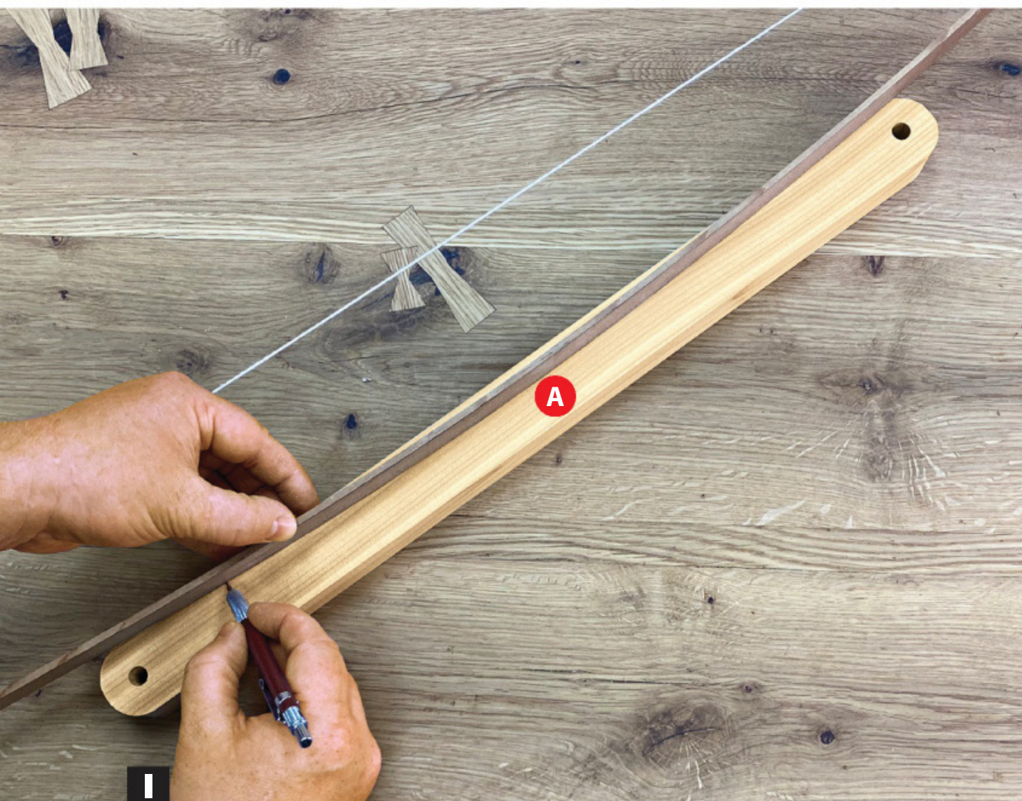
I Lay out a smooth curve along one edge of a center (A). Bandsaw the curve and sand the edge smooth to the layout line.
