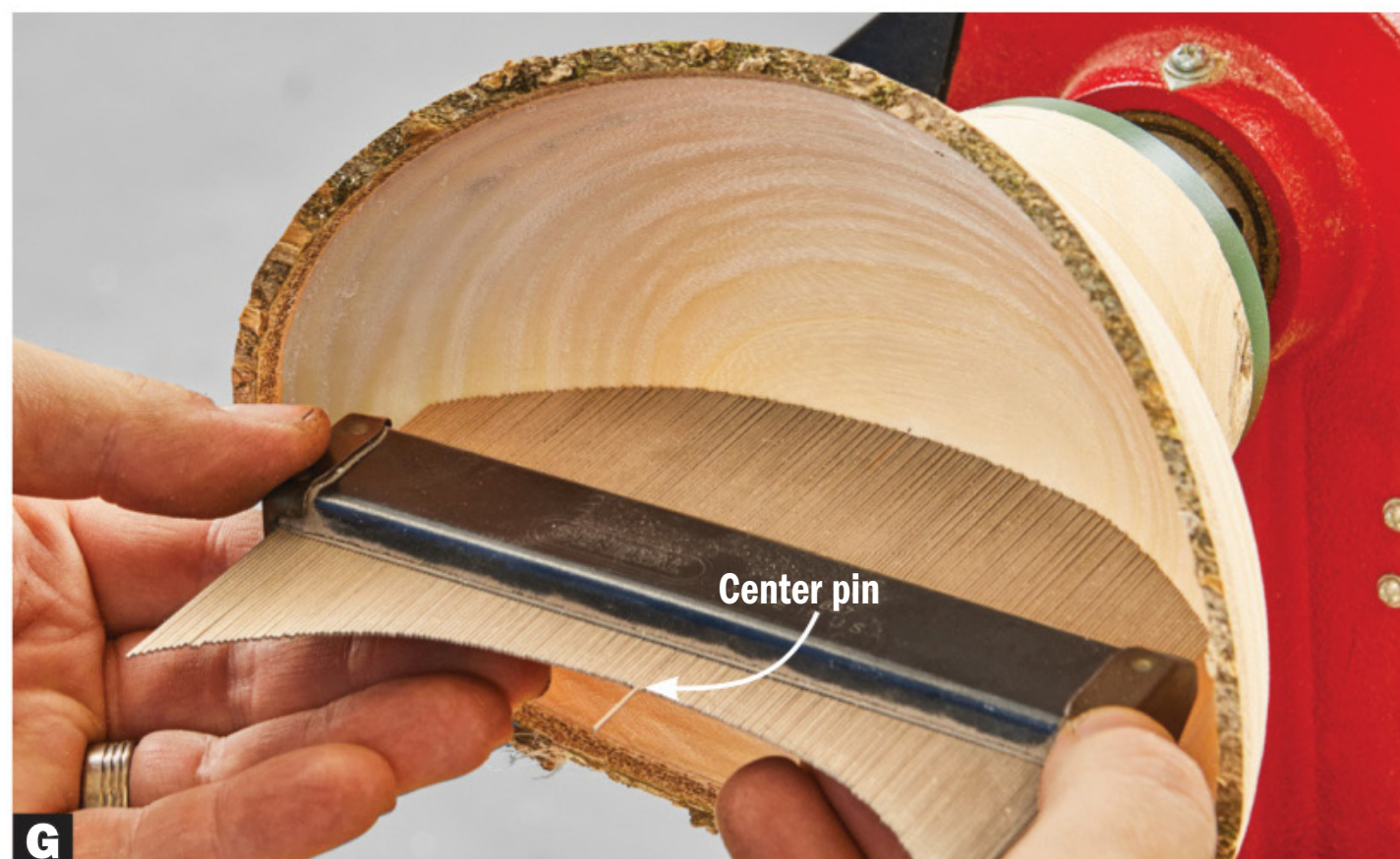
G Press the gauge pins against the bowl's interior. Carefully slide back the center pin (the one aligned with the dot) about \frac{1}{4} ". Trace the profile, including the retracted pin location, to a piece of paper.
