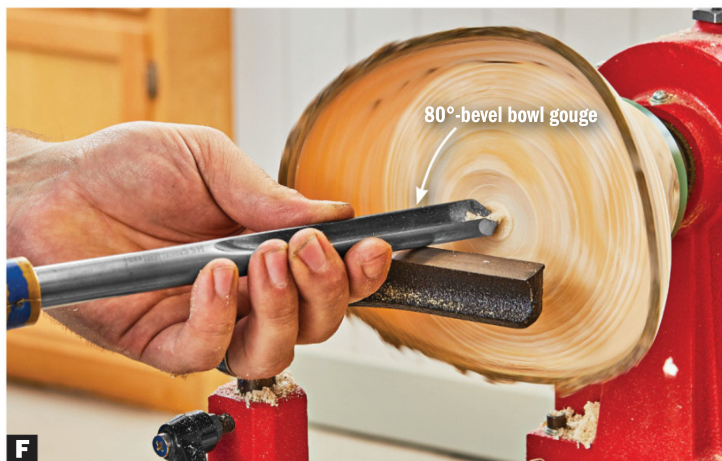
F As the bowl deepens, the 80° bevel allows positioning the tool closer to parallel to the lathe bed while still rubbing the bevel on the surface.
