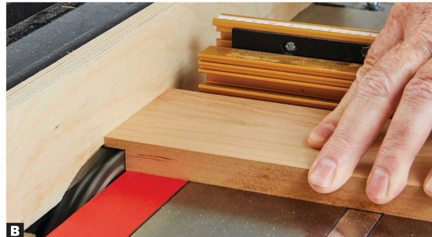
B Rabbet both ends of the front and back, holding the workpiece against the auxiliary fence and a miter gauge to ensure a 90° cut.
