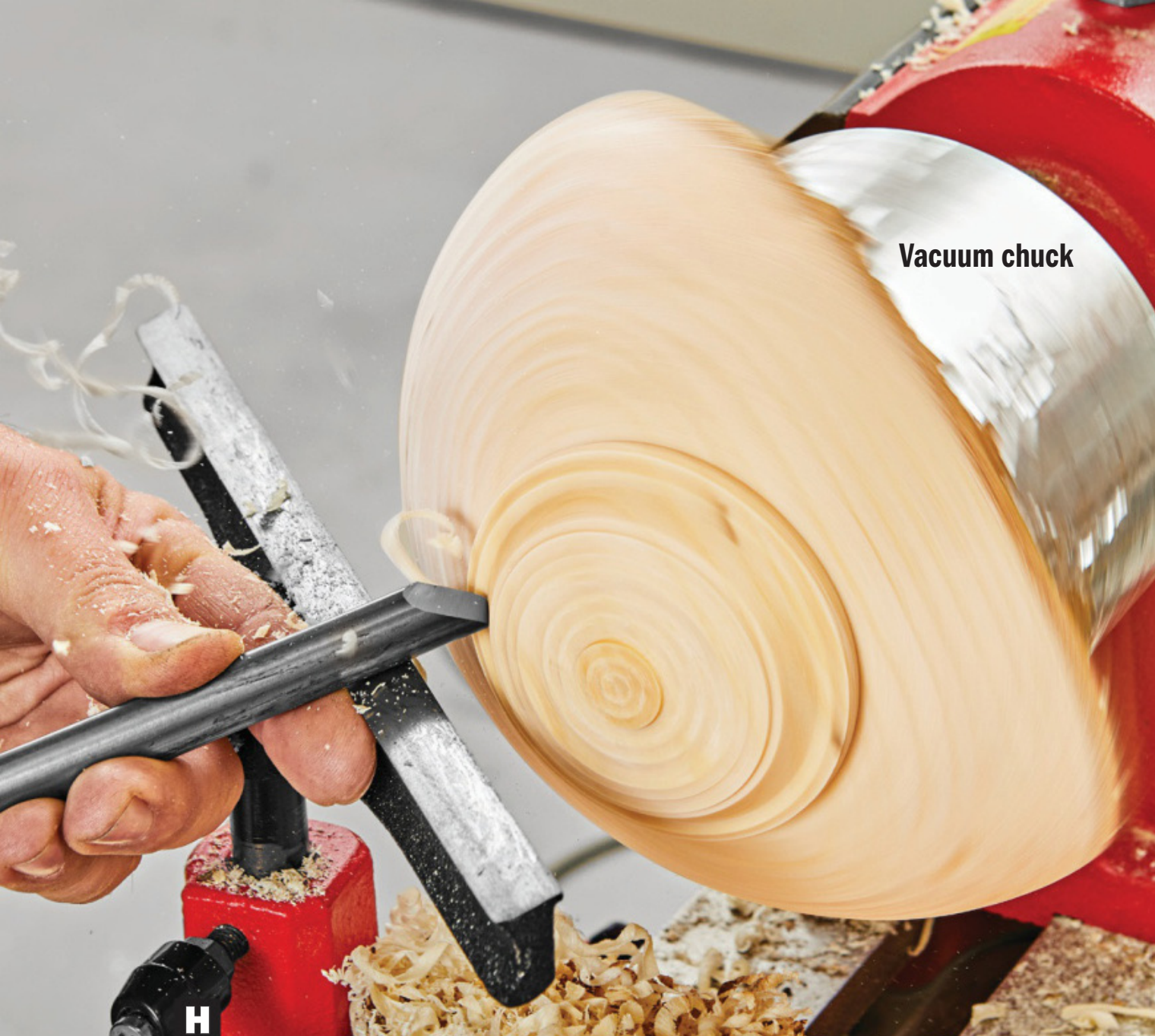
H Turn away the waste to leave a 2"-diameter tenon about \frac{1}{4} " long.
