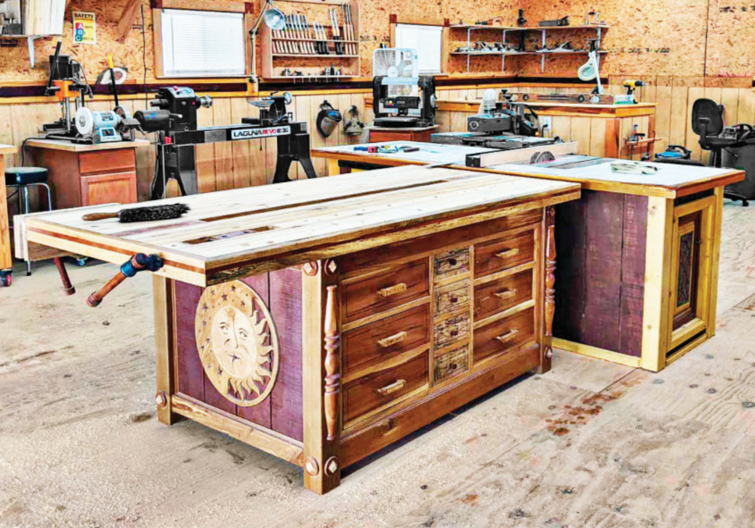
Custom cabinets surrounding Rob's tablesaw offer stock support and accessory storage. Rob's custom-built workbench makes an ideal outfeed support.
