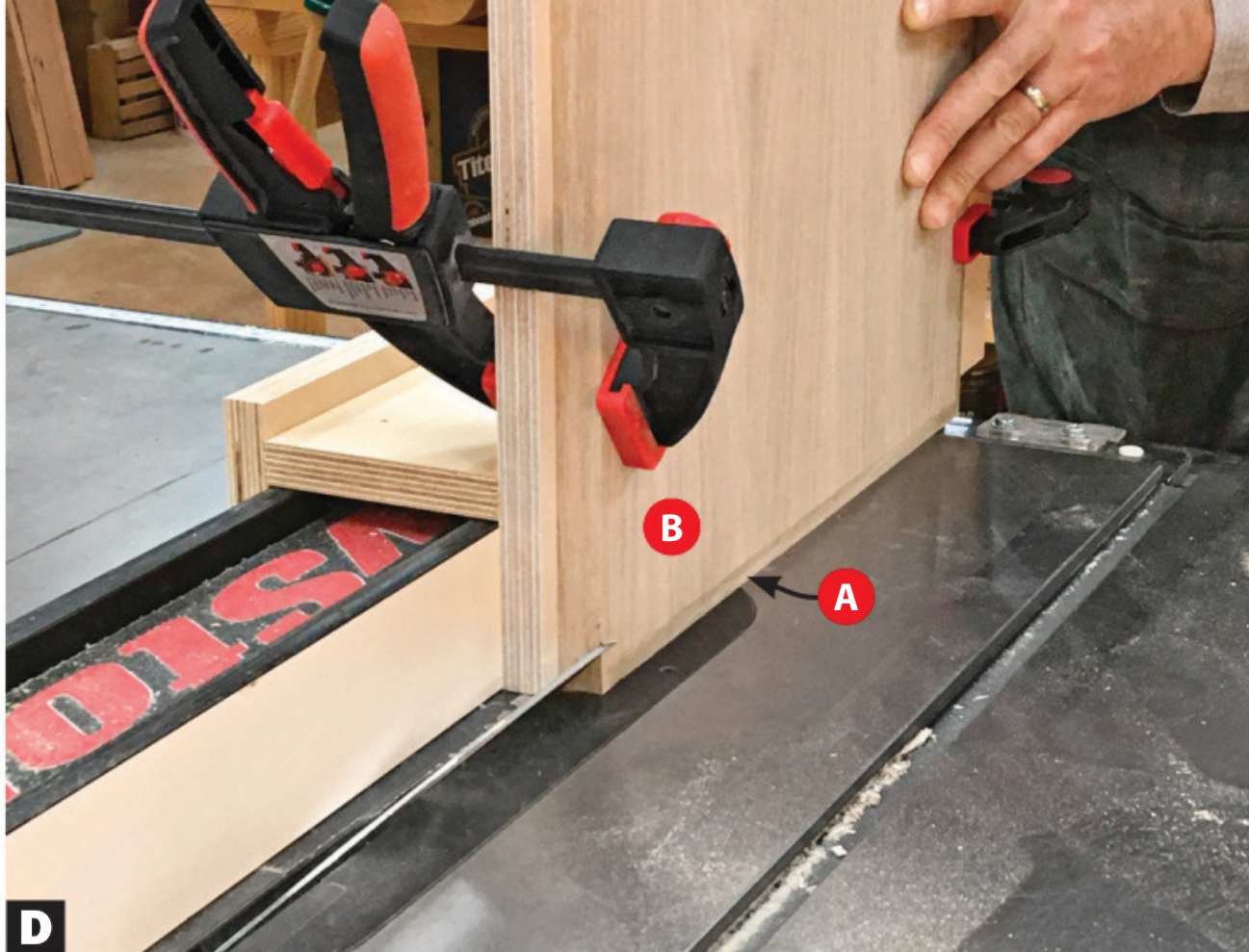
D Bevel-cut one end of a panel, then rotate it end for end and clamp the same face against the jig and bevel-cut the opposite end.
