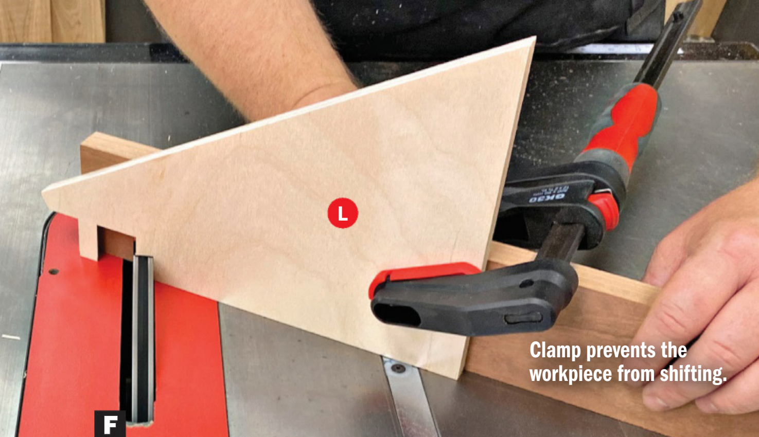
F Adjust the miter gauge to 30° and set the blade for a 1 1/8"-deep cut. A miter-gauge extension minimizes tear-out as you complete the cut.
