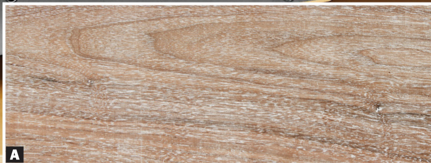
A White chalk reveals minimal milling marks from the DeWalt DW735X when planing at its slowest feed speed.
