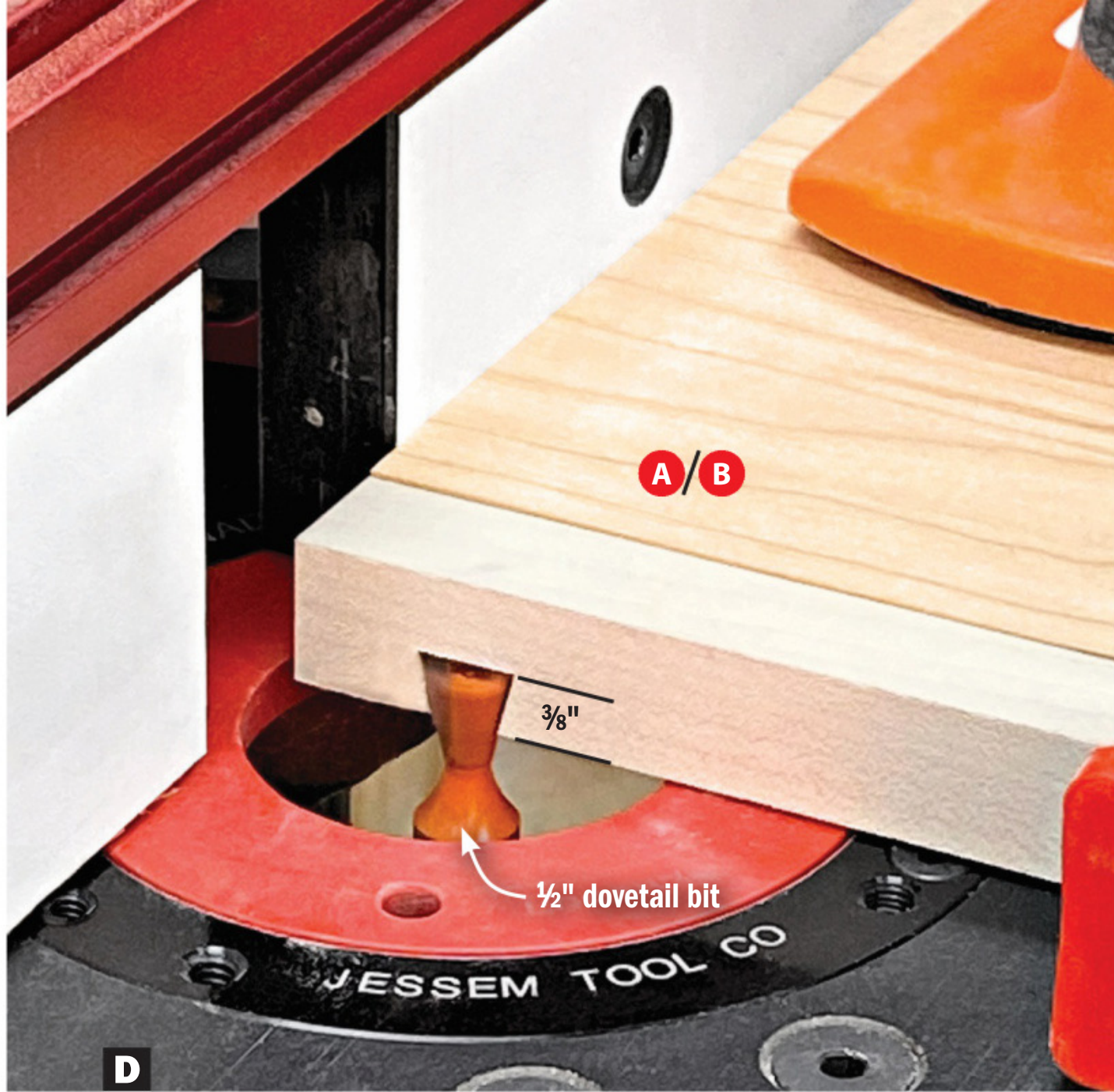
D Swap out the straight bit for a dovetail bit, recenter the bit on the dados, and complete the slots.
