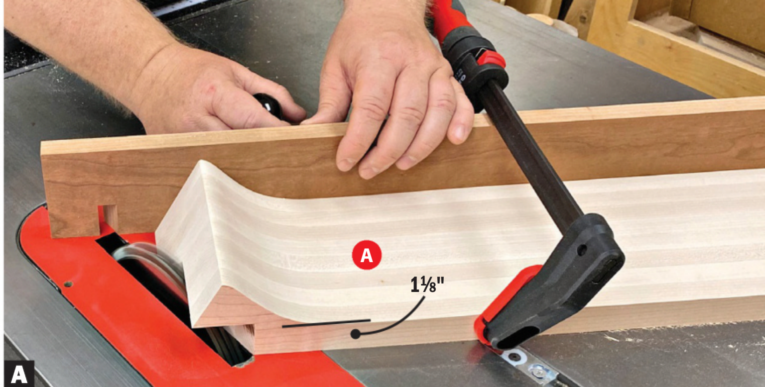
A A deep relief cut on the lane bottom directs balls falling into the lowest hole of the game to the proper ball return.
