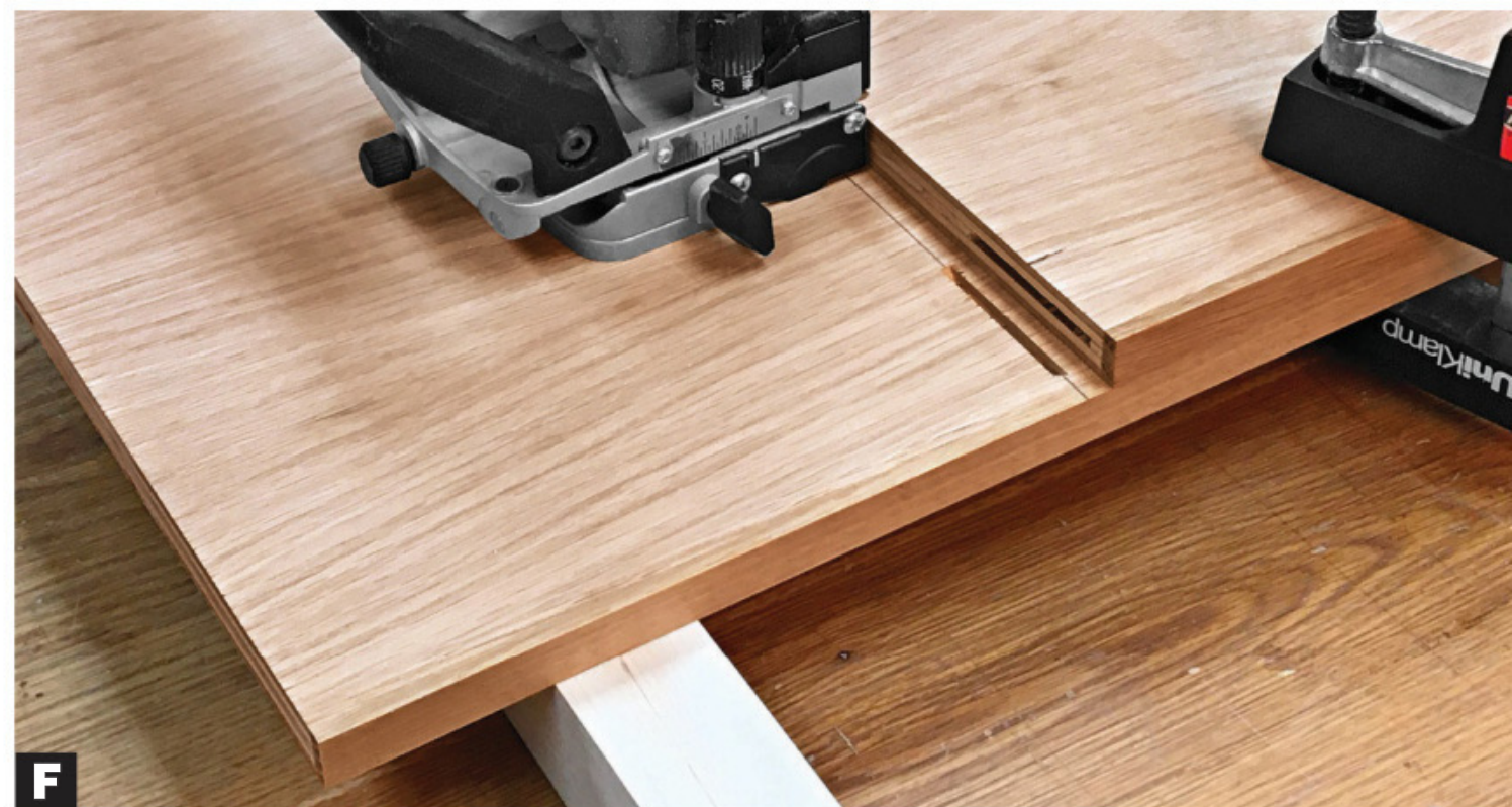
F Align the biscuit-joiner centerline with the marked centerline, using the mating part as a fence to position the tool.
