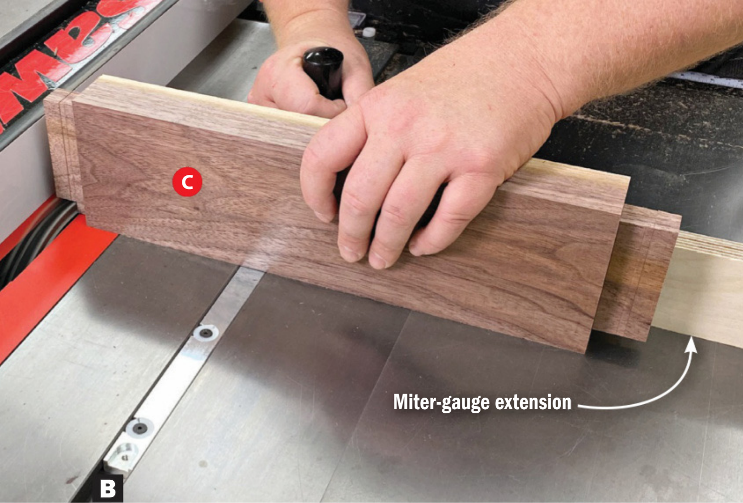
Use the rip fence as a stop when cutting the tenons on the side rails (B, C).
