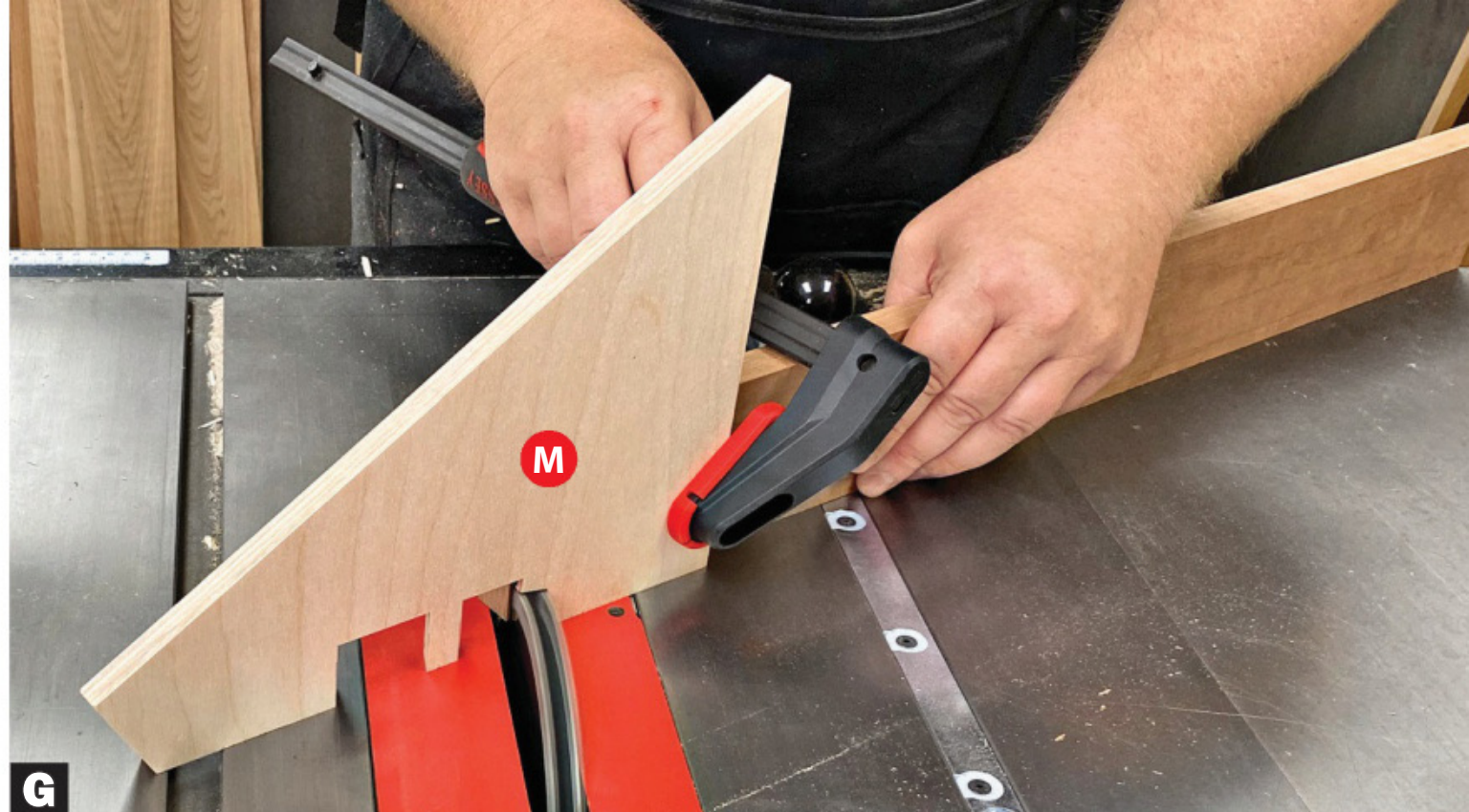
G Rotate the miter gauge to the opposite 30° setting to cut the notches for the right ball-drop side.
