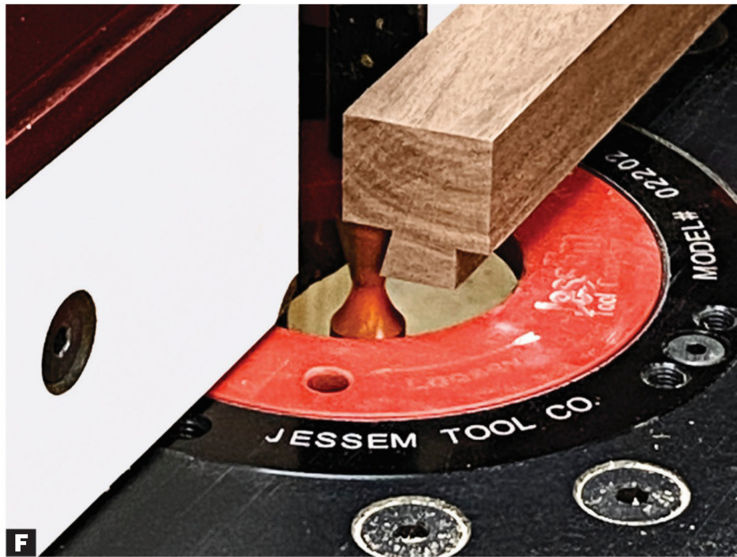
F Rout both sides of the dovetail, checking the fit in the slots in the board.
