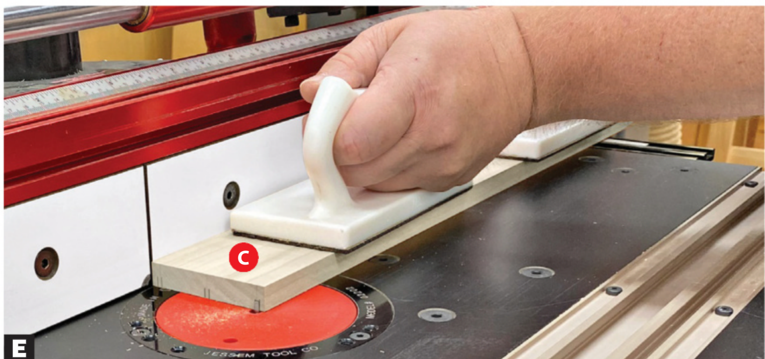
D Rout the grooves in the base (B) and return tops (C), alternating between the base and corresponding return-top groove to ensure perfect alignment. After routing the grooves in the return tops (C), mark them as left and right along with the outside edges to make it easy to match them up with the base during assembly.
