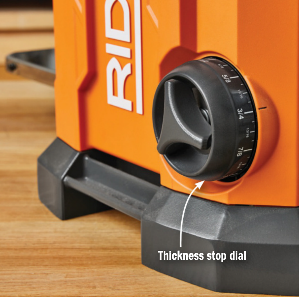
Ridgid provides 10 preset thickness stops from 1/8" to 1 1/4", with markings in 1/32" increments, and a manual lock for ultrafine thickness control.
