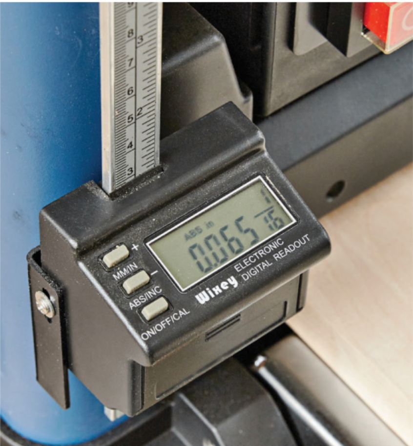
The digital gauge on the Oliver planer accurately displays the thickness setting, readable in fractions and decimals. It runs on two AAA alkaline batteries.
