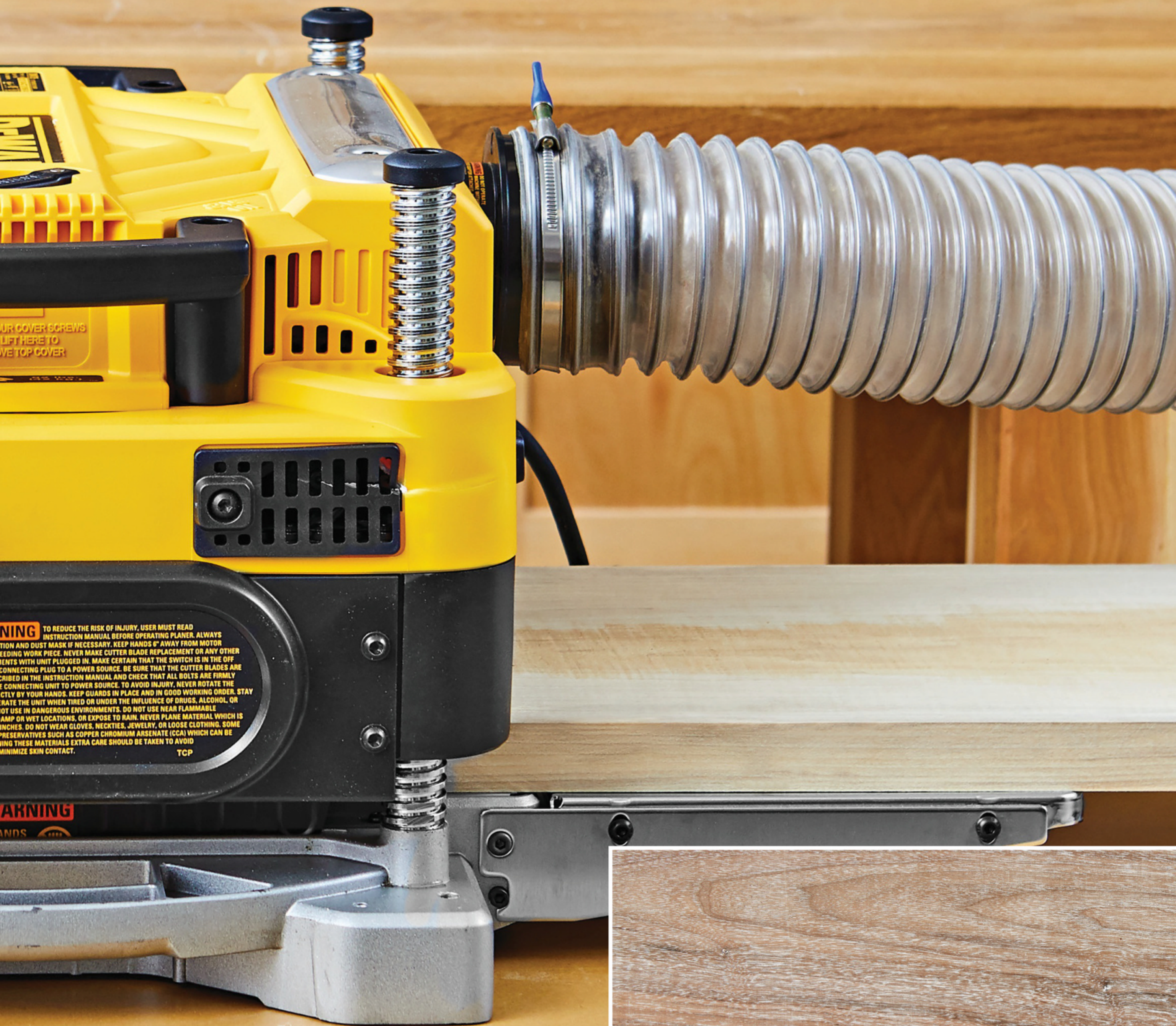
A White chalk reveals minimal milling marks from the DeWalt DW735X when planing at its slowest feed speed.
