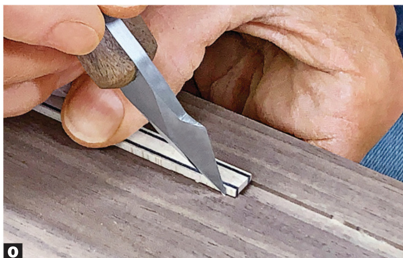
O Press one edge of the banding against the outside wall of the routed channel. With a marking knife, mark along the other edge of the banding.
