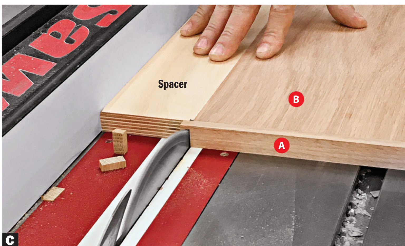
C Butt a part B against the spacer and slide both into the saw blade, cutting the end of the corner trim (A) flush.
