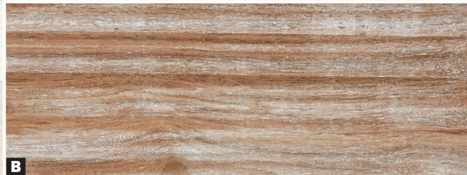
B Though more obvious on this board planed by the Oliver machine, insert cutterheads typically create ridges and grooves along the length of the planed board.
