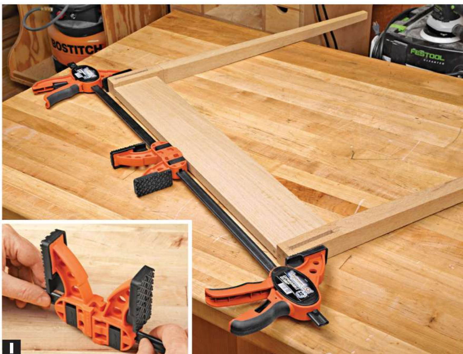
I The fixed jaws of these clamps interlock, combining two clamps into one. Positioning the linked jaws below the bar provides clearance above.
