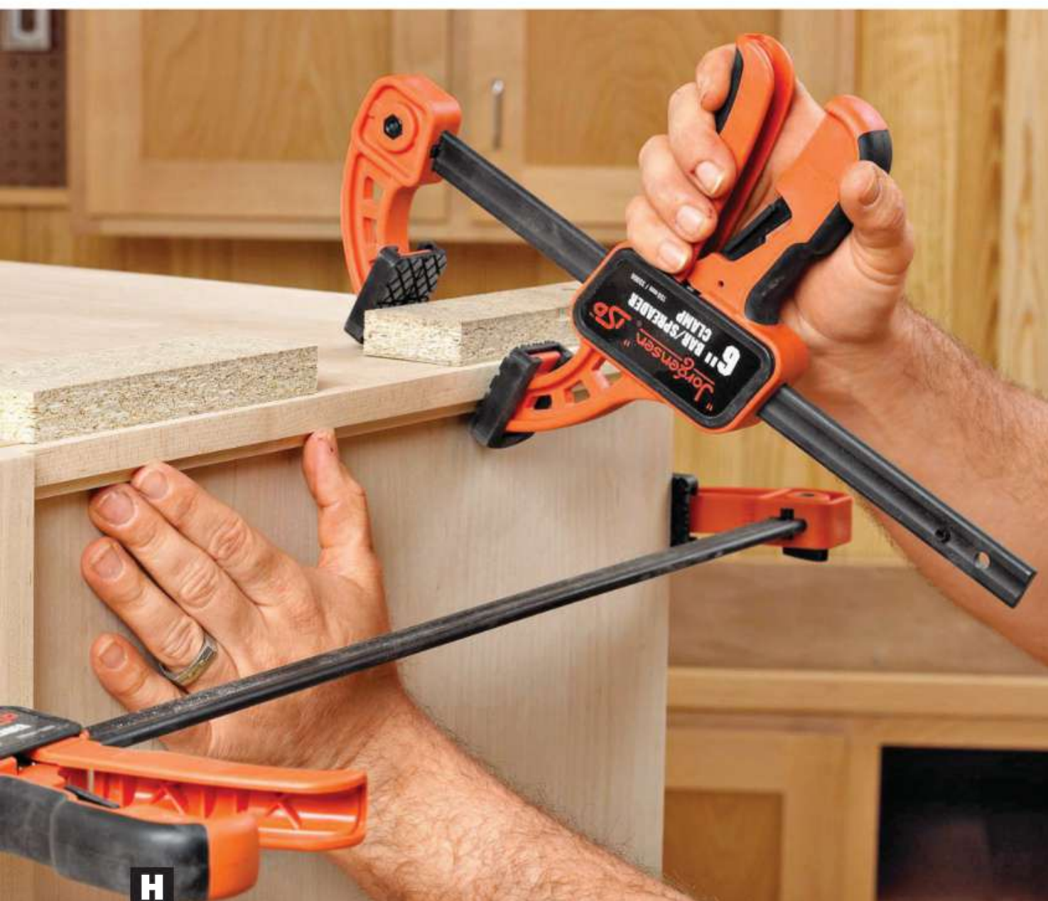
H One-hand clamps free your other hand to align parts as you clamp. If the job requires more pressure, add an F-clamp or pipe clamp after getting parts aligned.
