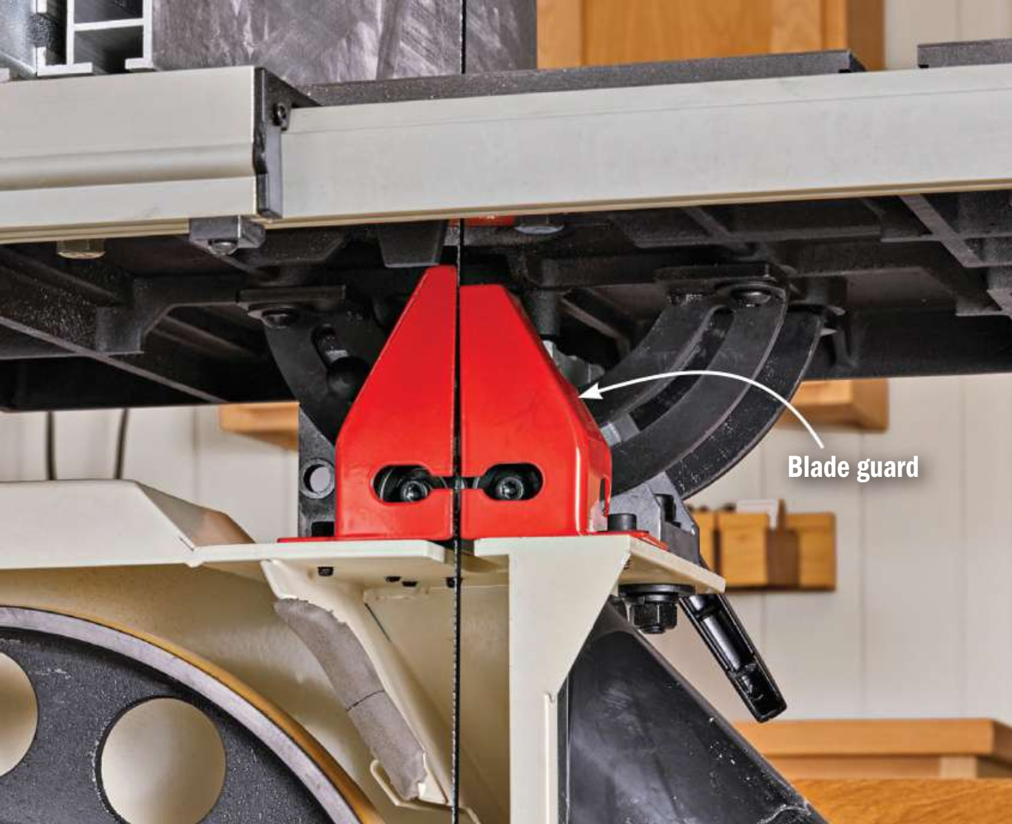
Blade guards below the table hide or impede access to the lower blade guides. These (on the Jet SFX) have hex-wrench access holes.
