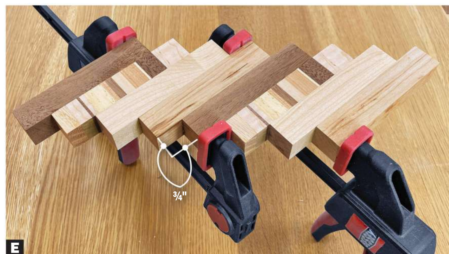
E Once the glue dries, glue and clamp the assemblies together, offsetting the ends, until you have combined them all.
