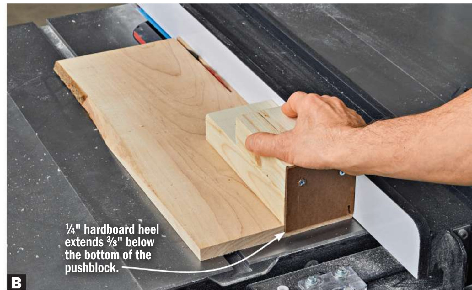
B A pushblock glued up from 2-by lumber provides ample thickness to allow the blade to cut into the pushblock without weakening it. Screw a replaceable heel to the rear to push the strip and blank past the blade.
