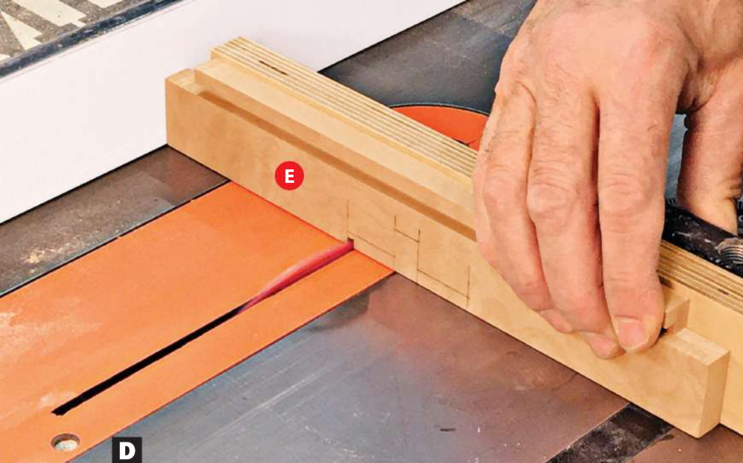
D Using the rip fence as a stop, cut one side of the shallow notch. Flip the board and repeat for the other side of the notch. Move the fence aside and nibble away the remaining material between the kerfs.
