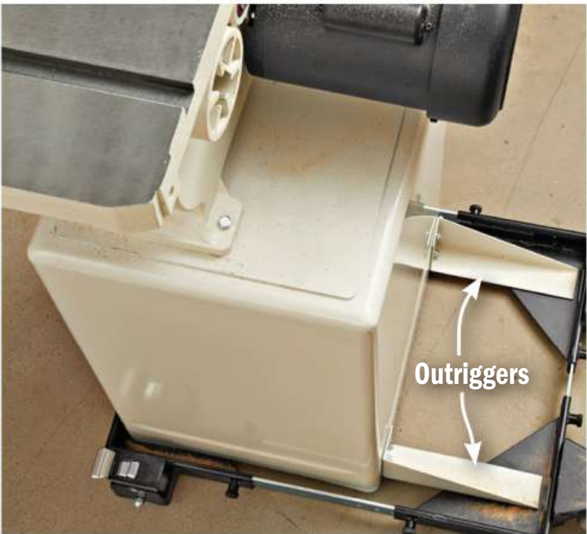
Lean on me. Outriggers on the Jet DXPRO base cabinet add stability, but also increase its overall footprint.
