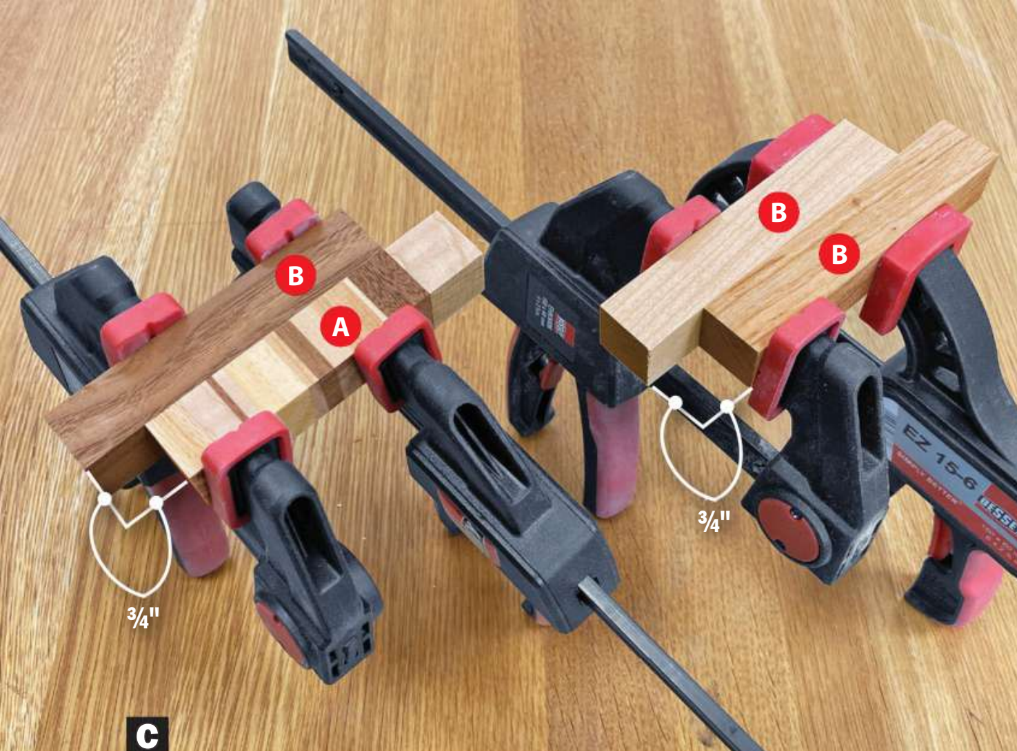
C Glue a walnut strip (B) to a laminated strip (A) and a maple to a cherry, offsetting the ends by \frac{3}{4} ". Repeat with the remaining laminated strips and solid-wood strips.
