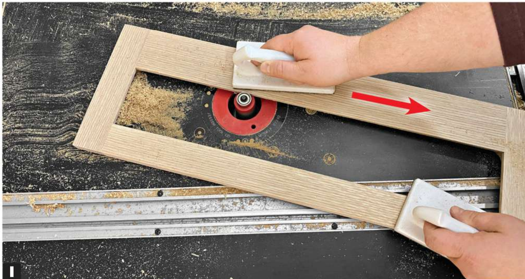
I Install a \frac{1}{4} " rabbeting bit in your router table and rabbet the rear face of the frame. Use several progressively deeper passes to rout to a final depth of \frac{3}{16} ".
