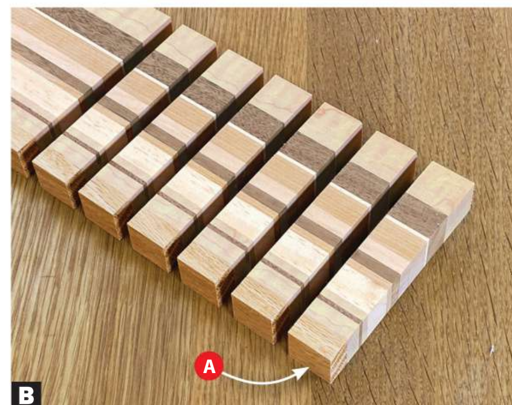
B Install an 80-tooth blade in your tablesaw and crosscut the block into 3/4"-wide laminated strips (A).
