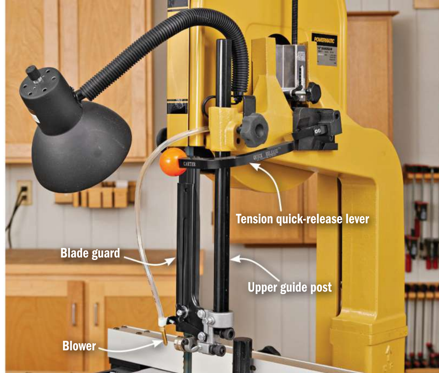
Powermatic's tension-release lever often hangs up on the upper guide post, blade guard, or task light. We had to reposition these at times to release blade tension.
