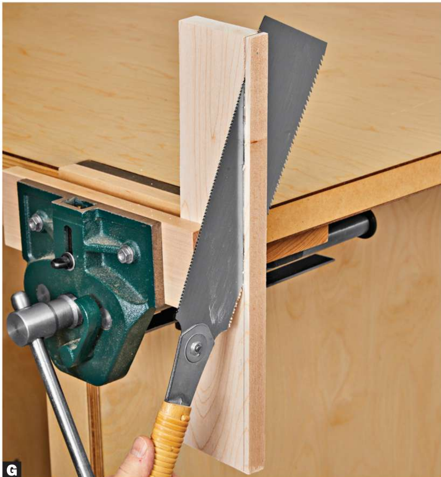
G Cut at a shallow angle to the board—more blade in the cut reduces chatter and wandering. Do not apply heavy pressure, but rather let the weight of the saw do the work as you draw the tool down.
