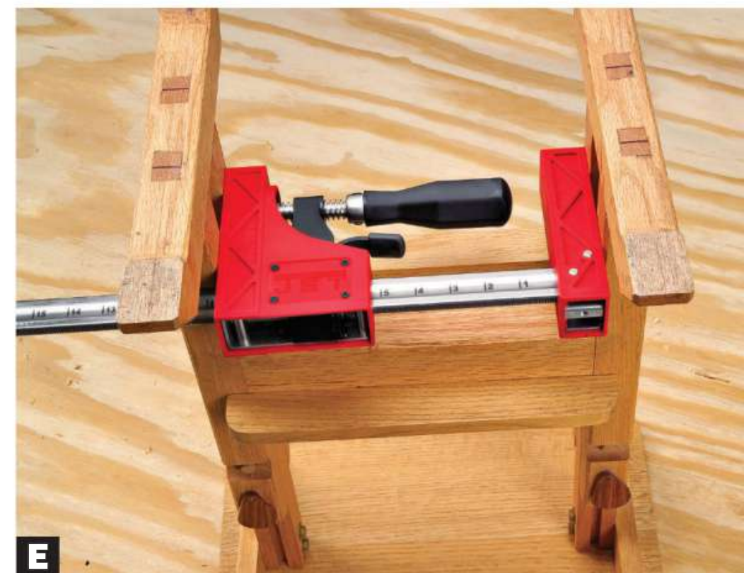
E Reversing the movable jaw of a parallel-jaw clamp creates a spreader, useful for disassembly.
