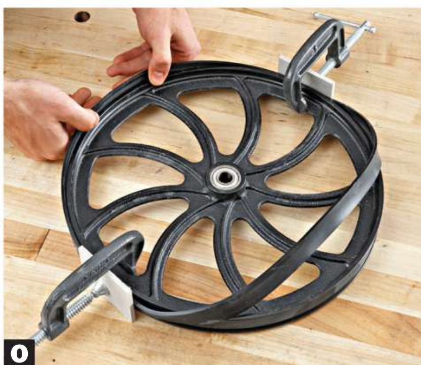
C-clamps provide plenty of pressure for keeping a bandsaw tire in place while stretching it onto the wheel.
