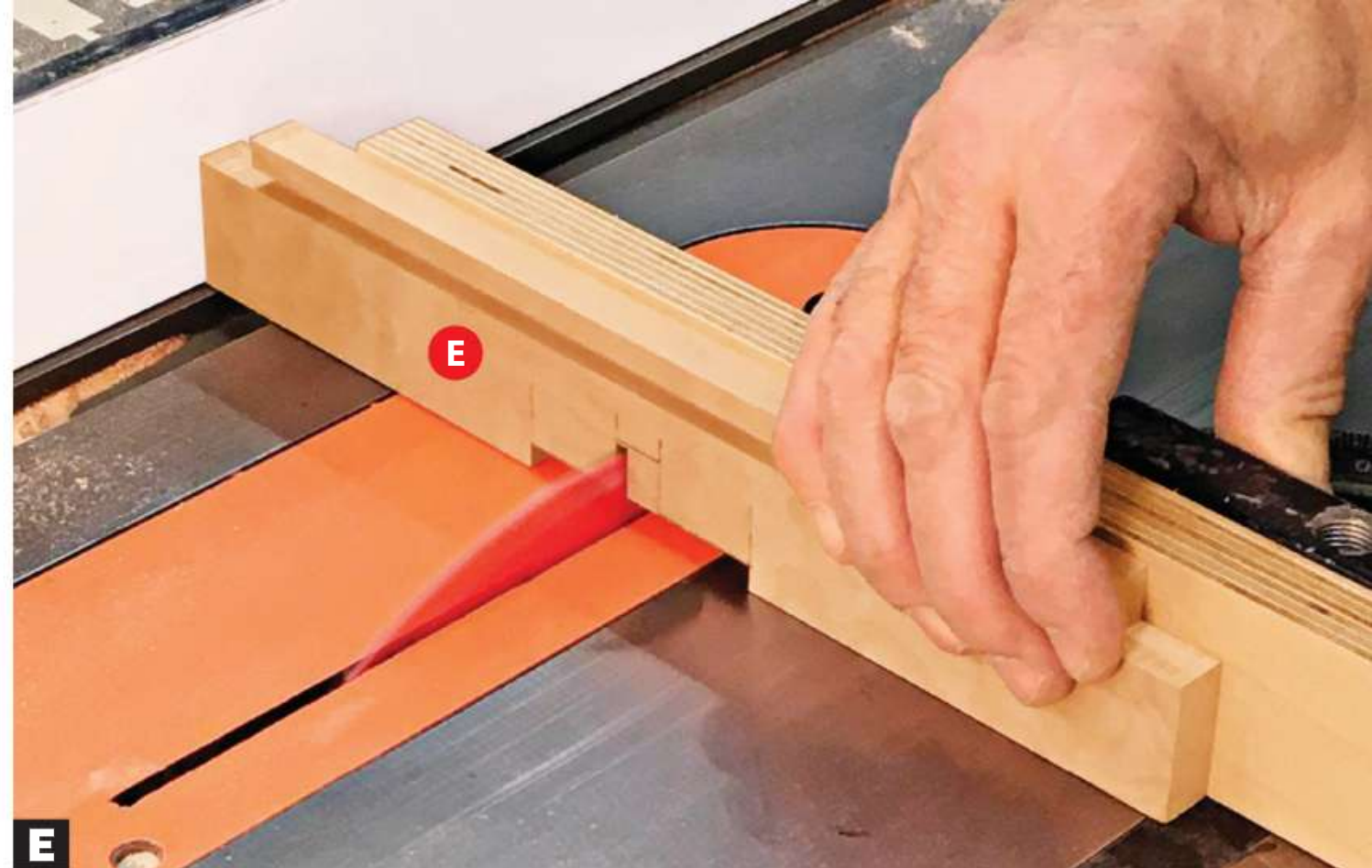
E Reposition the fence, and as you did for the shallow notch, cut the sides of the upper notch, and then nibble away the waste.
