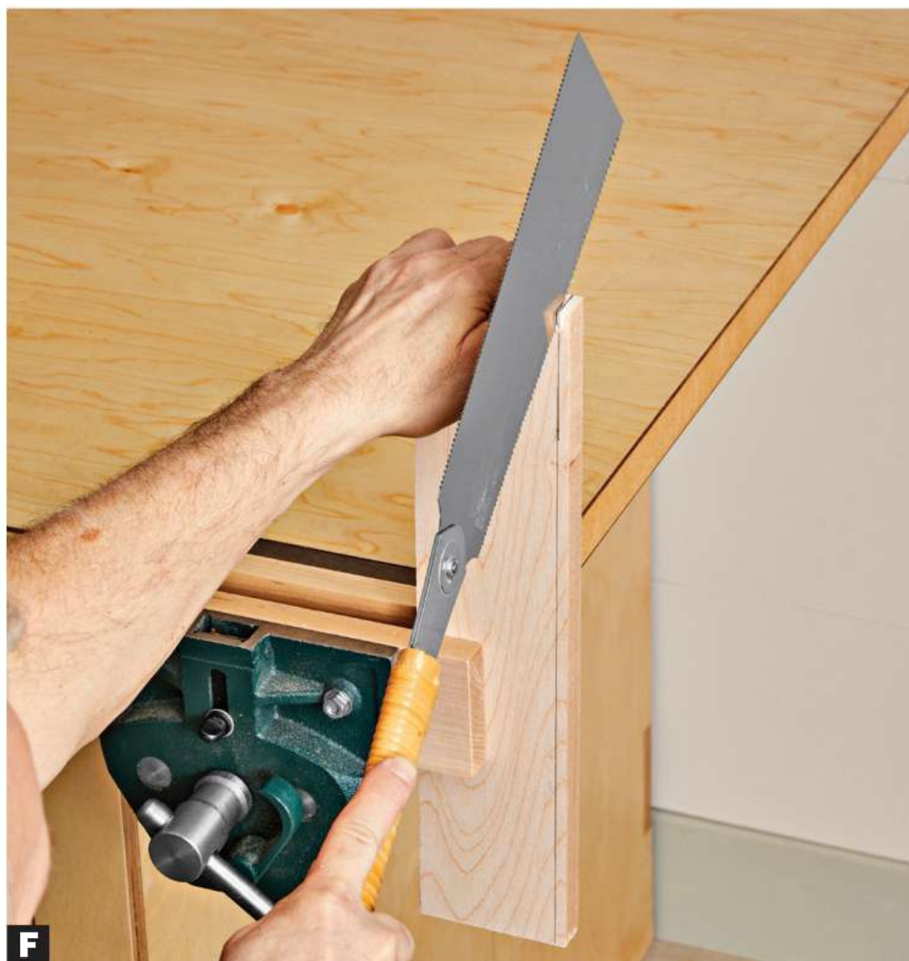
F Sight along the blade and the marks on the face and end. Take light initial strokes, guiding the blade with your thumb knuckle.
