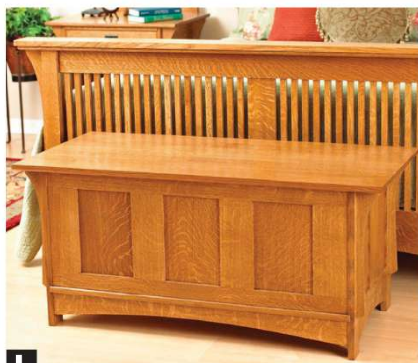
L One 29"-wide panel of quartersawn white oak for the front of this chest might change \frac{3}{8} " in width. Three narrower panels move less than \frac{1}{10} " each.
