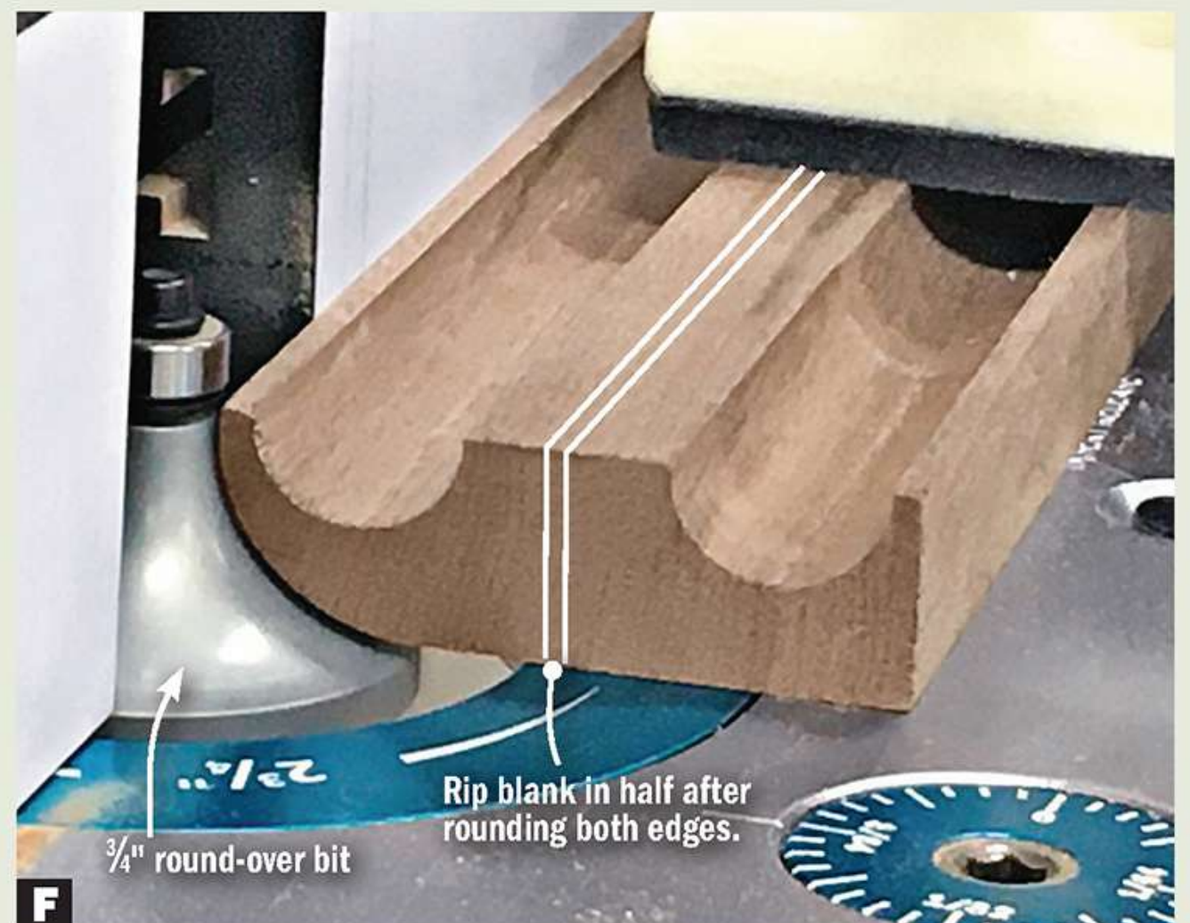
F Position the fence flush with the bearing and round over both edges.
