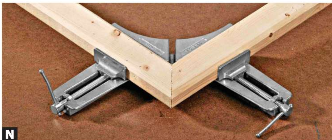
Use a corner clamp to hold mitered pieces in position while the glue dries. These clamps hold the corner of a drawer or carcass as well.
