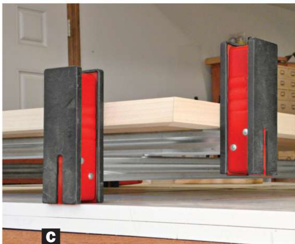
C Long jaws reach far enough to apply pressure even with one set of clamps resting on top of the others.
