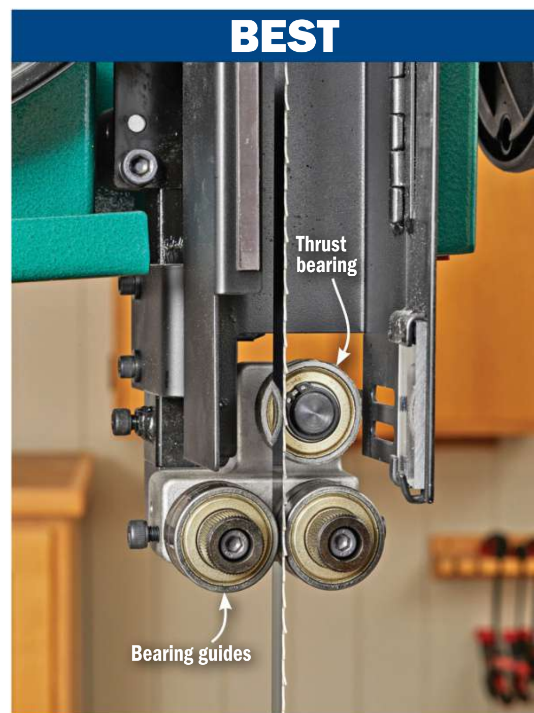
Large stacked-bearing side guides (on the Grizzly G0817), about one-third larger than those on other saws, provide better surface contact with the blade. The perpendicular-mounted thrust bearing works well.
