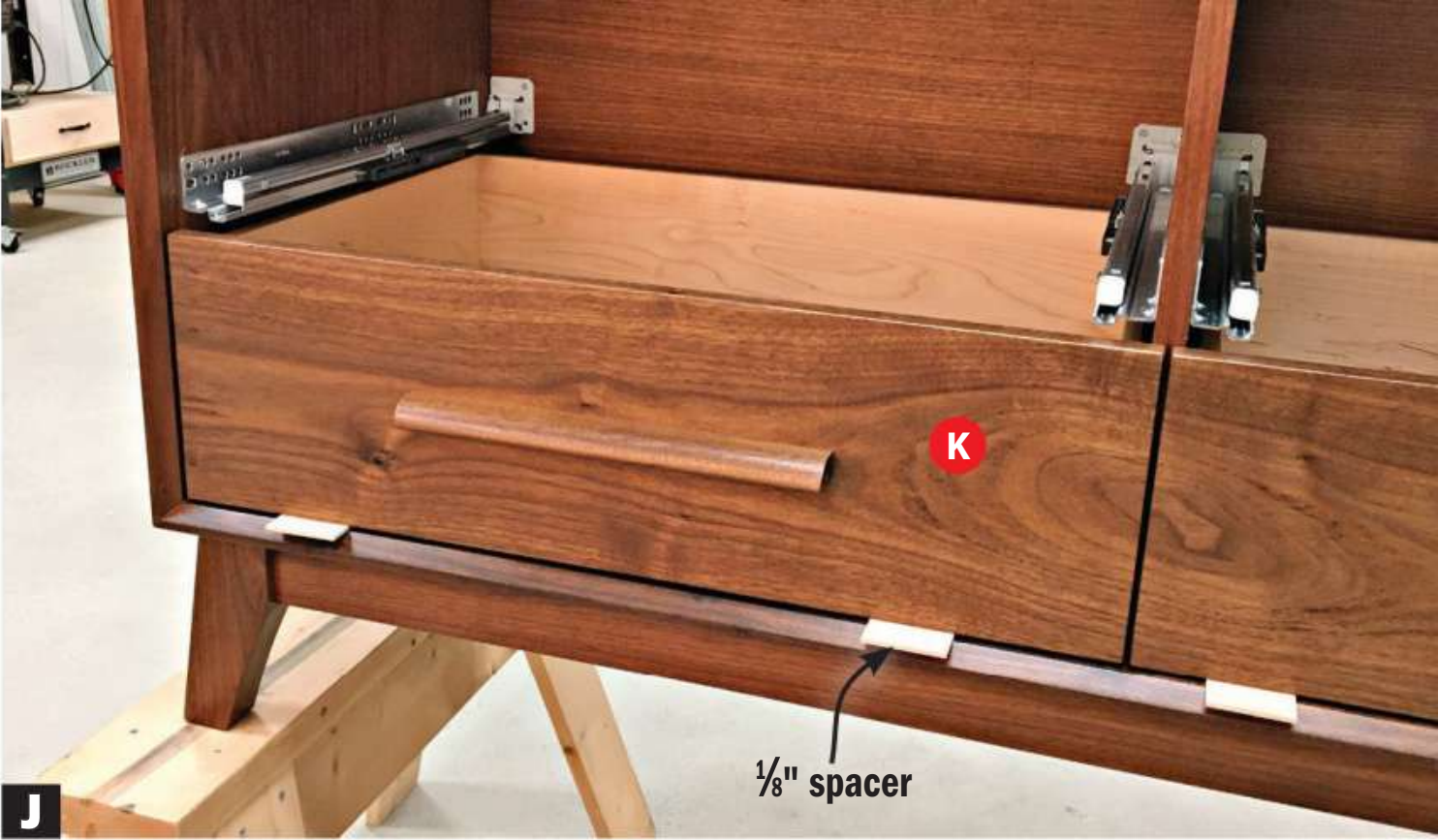
J Apply double-faced tape to the back face of the false front (K). Rest the false front on spacers and press it against the drawer box.
