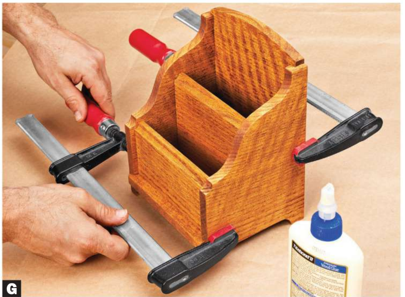
G Hold together glue-ups too small for bar clamps with a few F-clamps.
