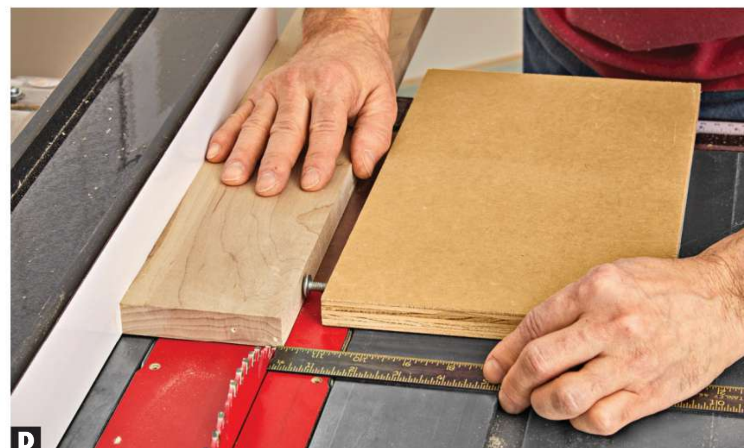
D Anchor the jig in the miter slot, then place your strip blank against the rip fence and the blade, with the desired strip thickness to the outside of the blade. Adjust the screw to just kiss the blank.
