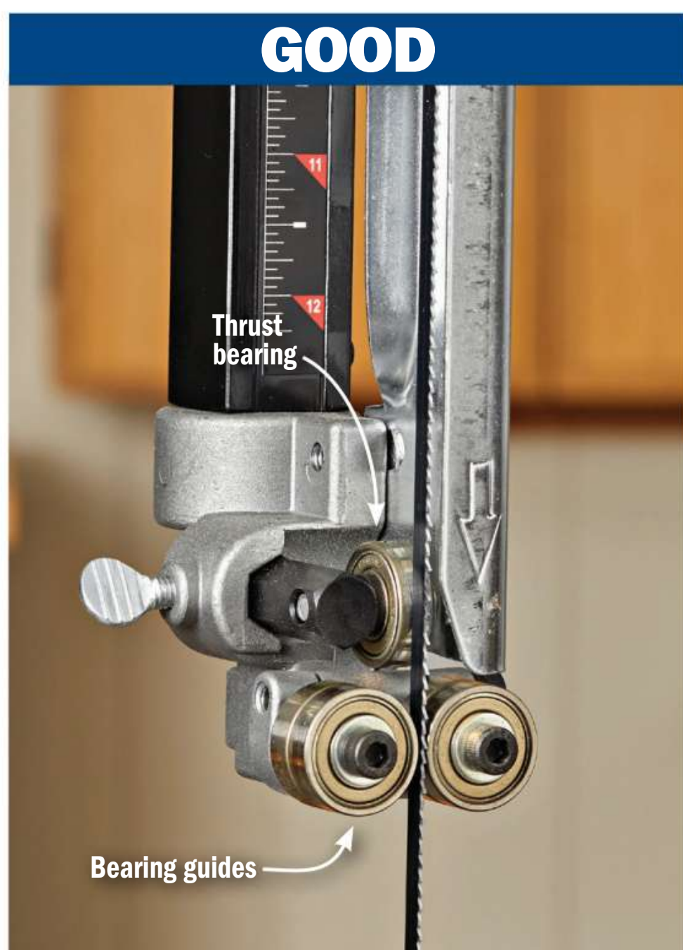
Stacked-bearing side guides (shown on the Grizzly G0555XH) provide single-bearing support for narrow blades, while both support wide blades. The in-line thrust bearing prevents the blade from moving backward during cuts.
