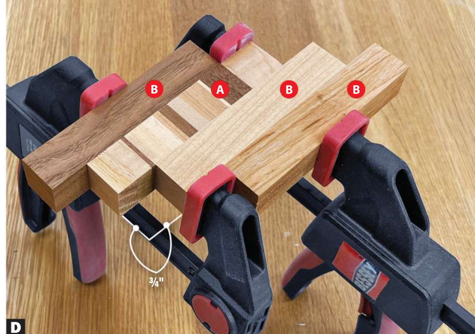
D Glue and clamp the walnut/laminated pairs to the maple/cherry pairs, offsetting the ends. When completed, you should have six of these assemblies.
