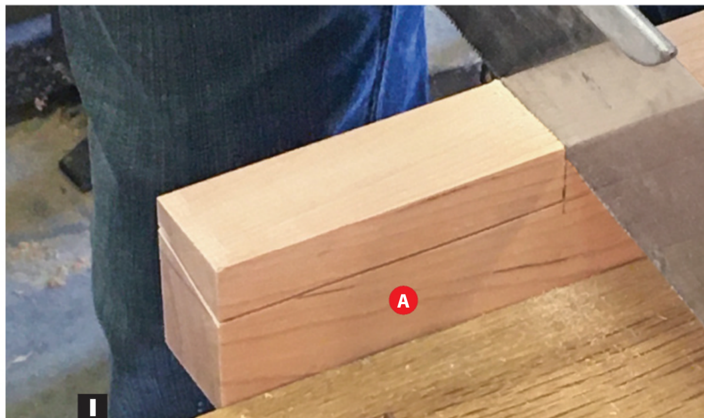
I A handsaw makes quick work of removing the waste and completing the crest-rail notch.
