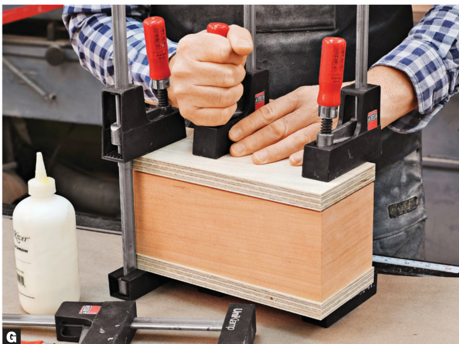
G Spread glue in the rabbet and press in the bottom. Use a caul on top and bottom and apply clamps. Too much pressure can break apart the joints, so go easy.
