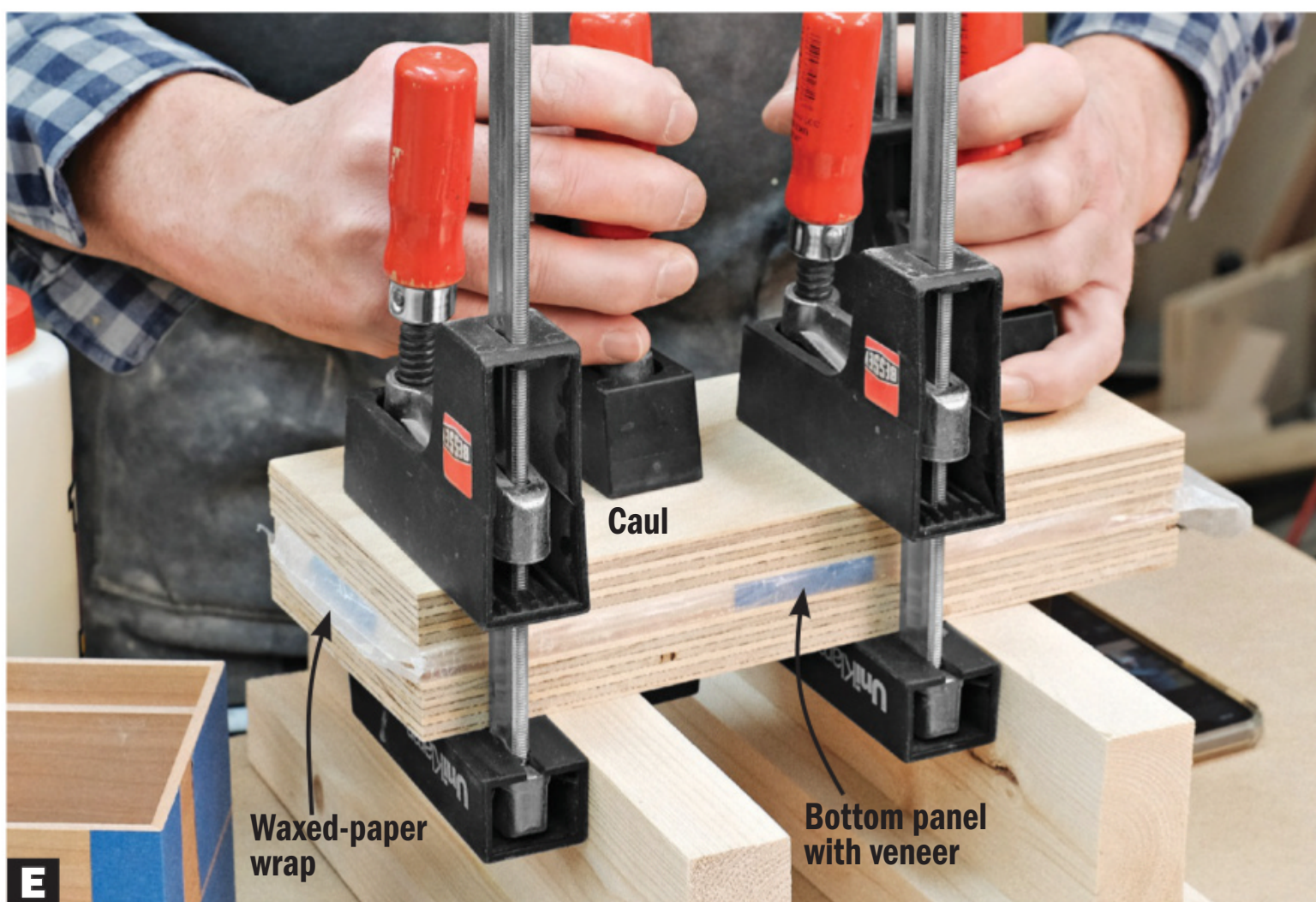
E Spread glue on the bottom panel, making sure it reaches the edges. Apply the veneer, wrap waxed paper around the assembly, then clamp between thick cauls.
