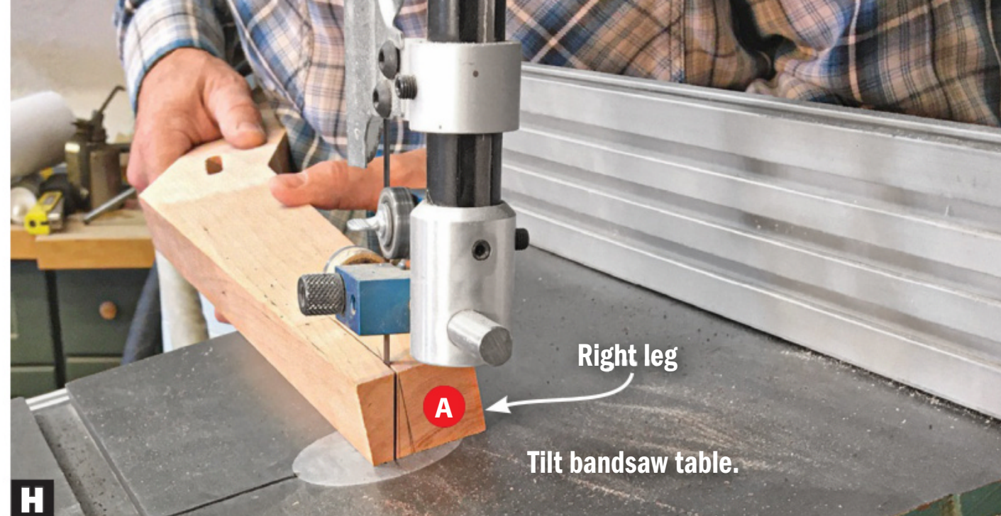
H Tilt your bandsaw table to match the scribe mark on top of the leg, then cut the notch.
