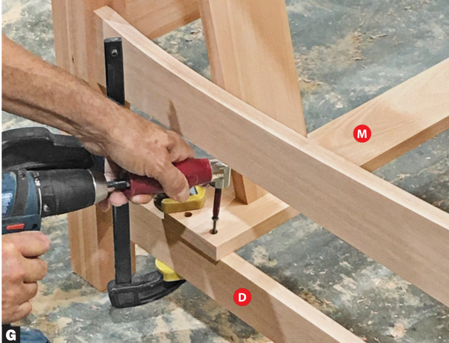
Screw the backrest support (M) to the side bottom rails (D) using a right-angle attachment in your drill.
