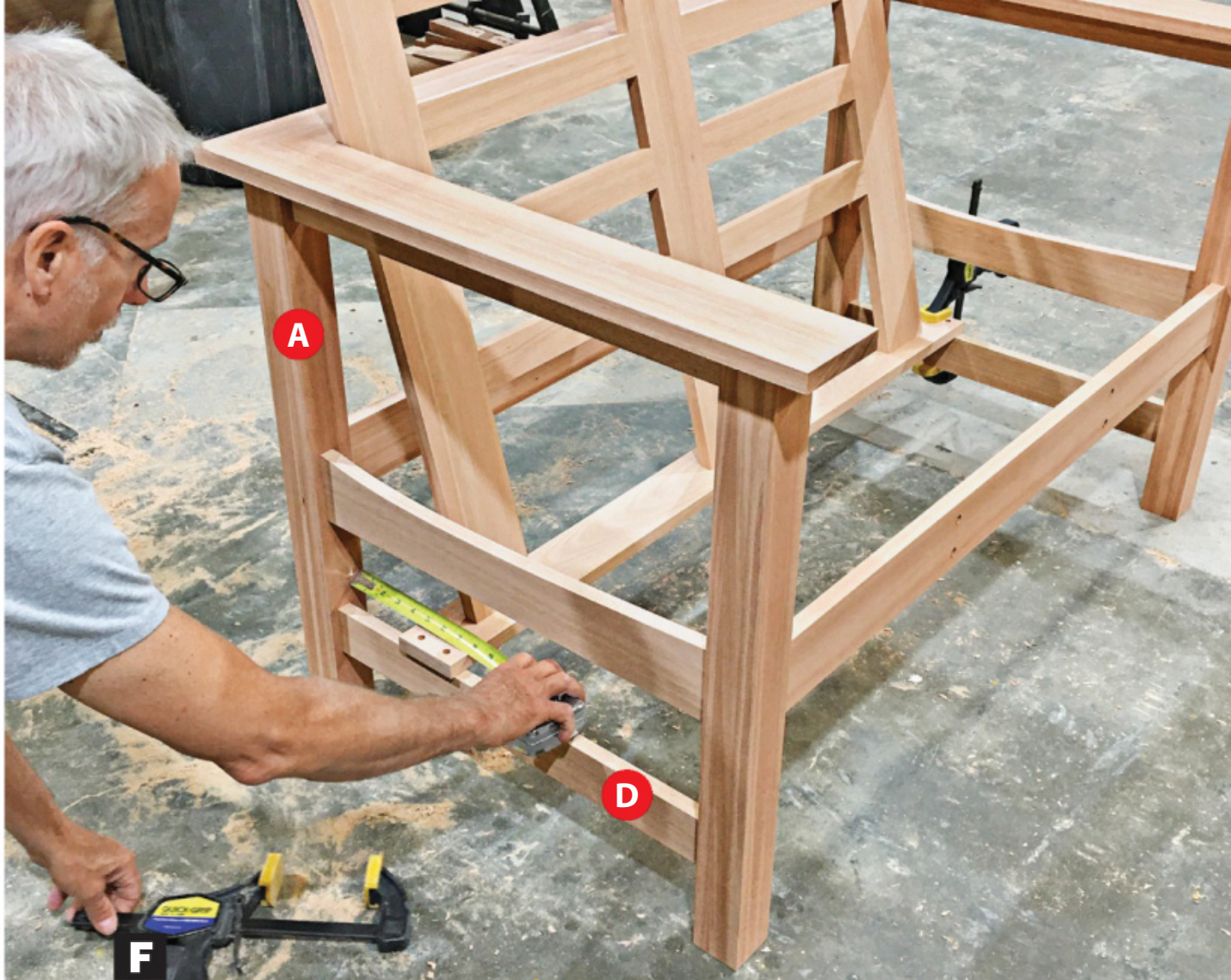
Position the backrest assembly on the side bottom rails (D), 4½" from the back legs (A). Clamp it in place.
