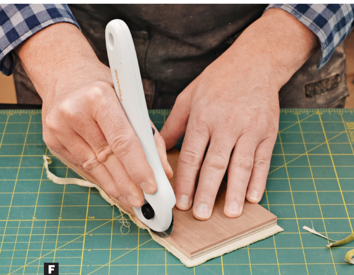
F Start with an oversize piece of fabric and glue it to the plywood with spray adhesive. Cut it flush to the plywood with a rotary cutter or crafts knife.
