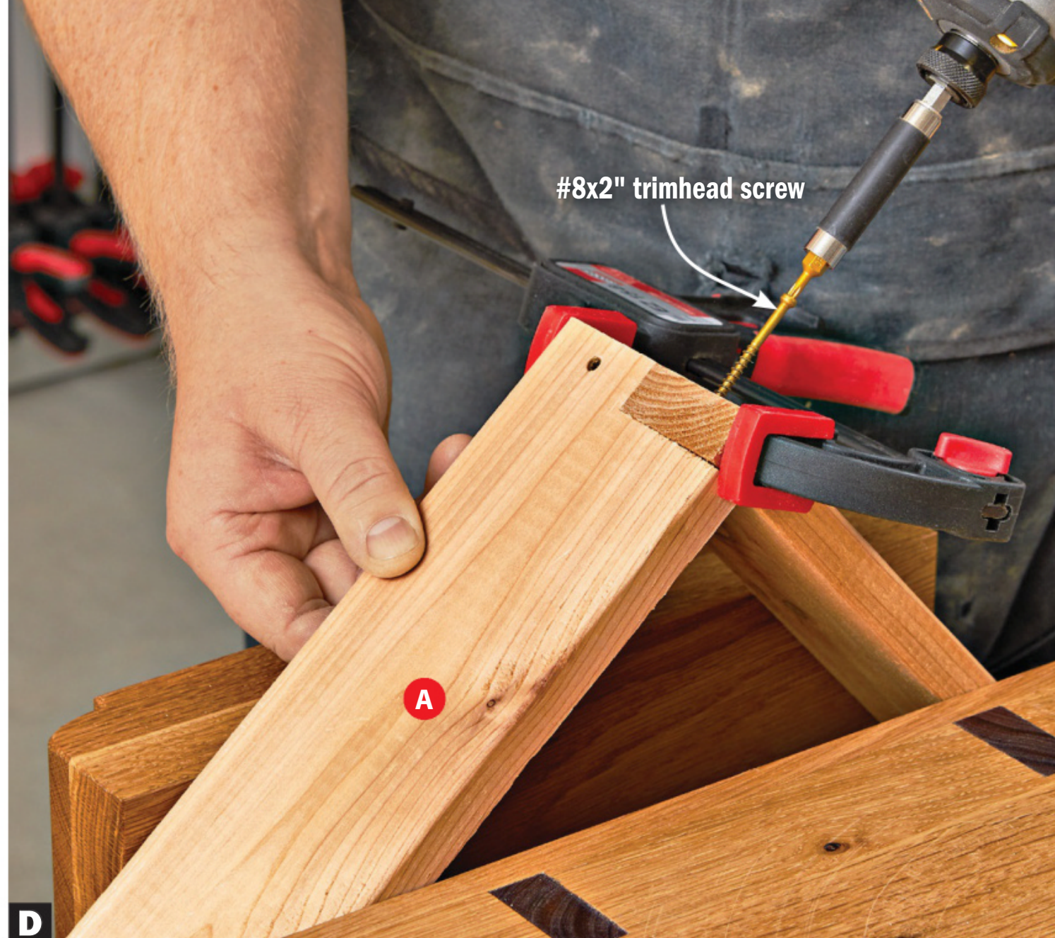
D Clamp the box sides in a vise while driving the screws.
