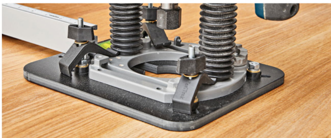
For quick mounting, the Woodhaven jig clamps to almost any router. Although it's not necessary, we removed the subbase to maximize plunge depth.
