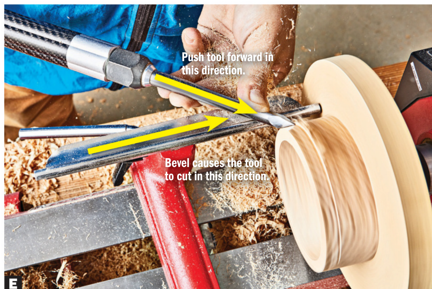
E With the flute mostly closed, position the bevel parallel to the outside face. Push the gouge forward with your rear hand and the tool will cut, from right to left, parallel to the bevel.
