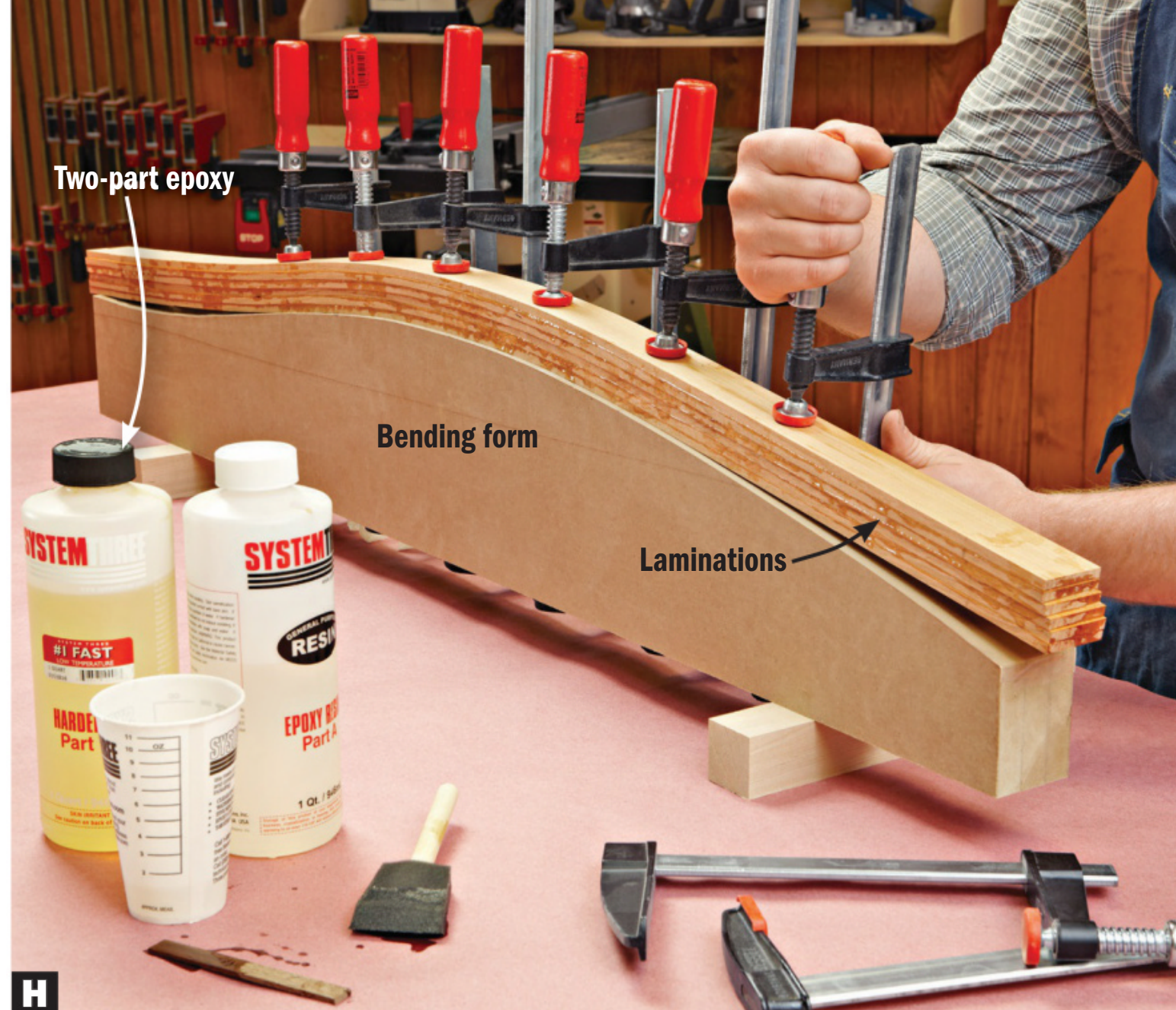
H Bent laminations require plenty of clamps. Space clamps approximately 6" apart for maximum pressure and to eliminate gaps.
