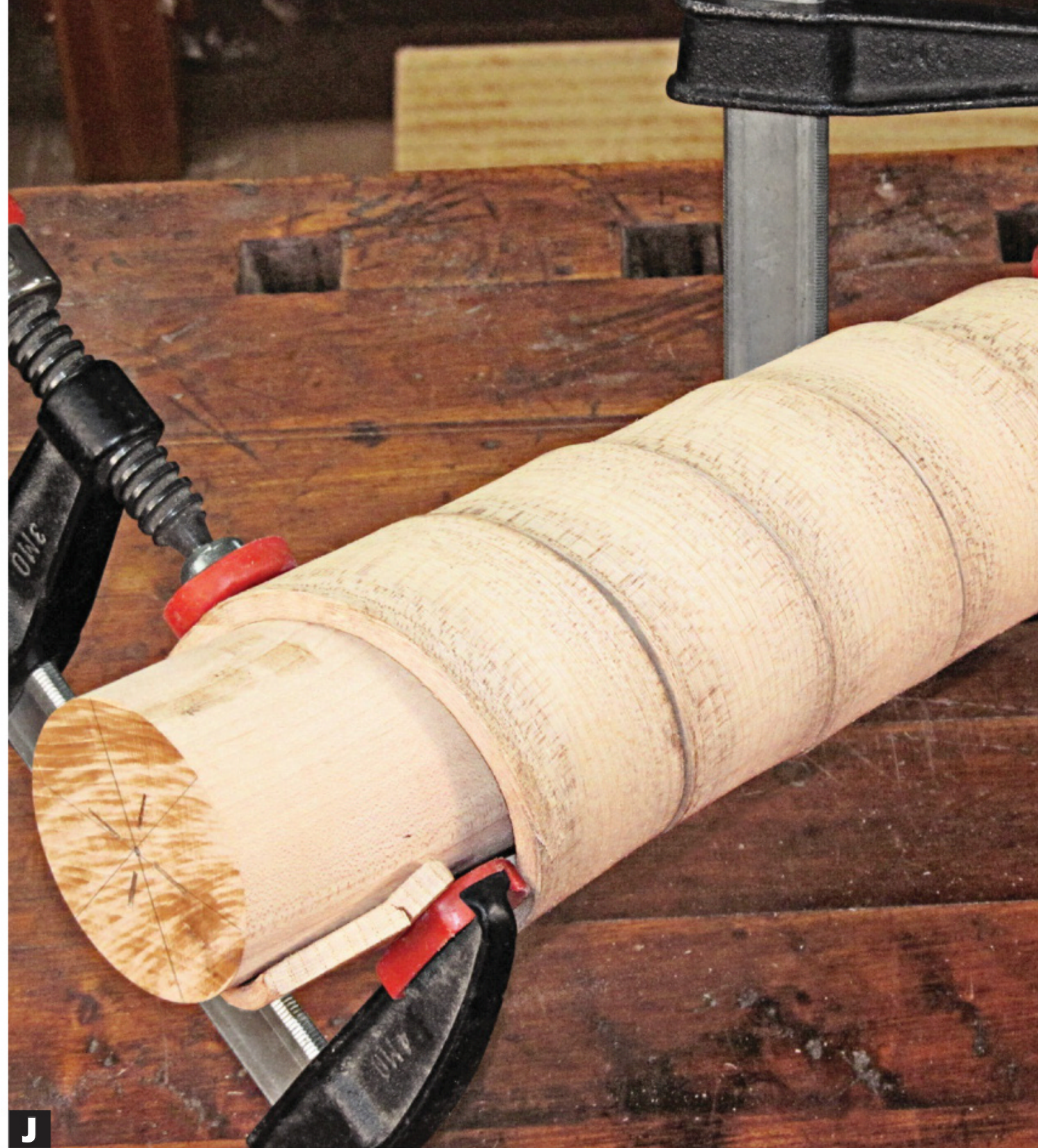
J Bend the wood around a form by hand, using clamps to hold it in position while drying. We let this coil dry around a 3"-diameter dowel for 12 hours.
