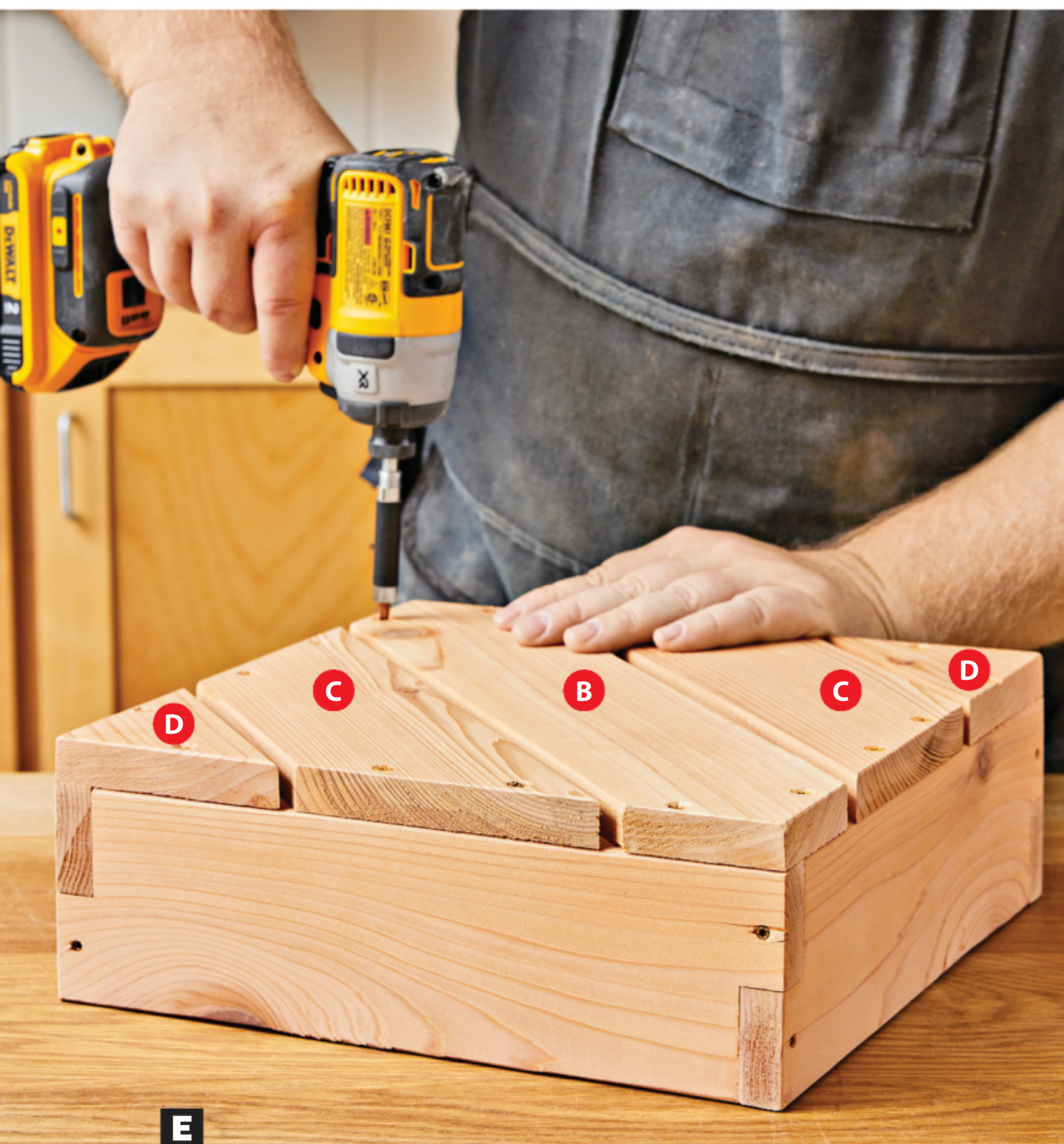
E To prevent splitting the ends, drill countersunk screw holes in the box bottoms before driving the screws.
