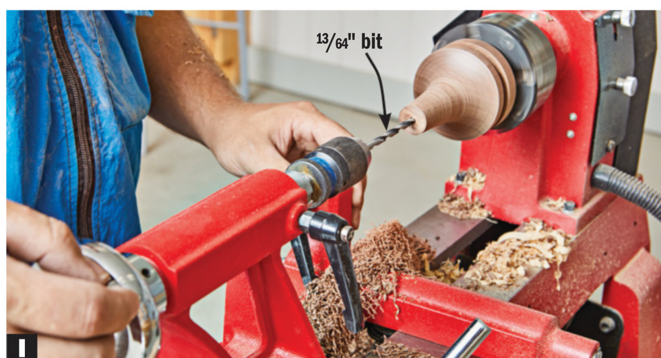
I Drill past the parting cut. Sand the base, then complete the parting cut, creating a slight undercut on the bottom of the base.
