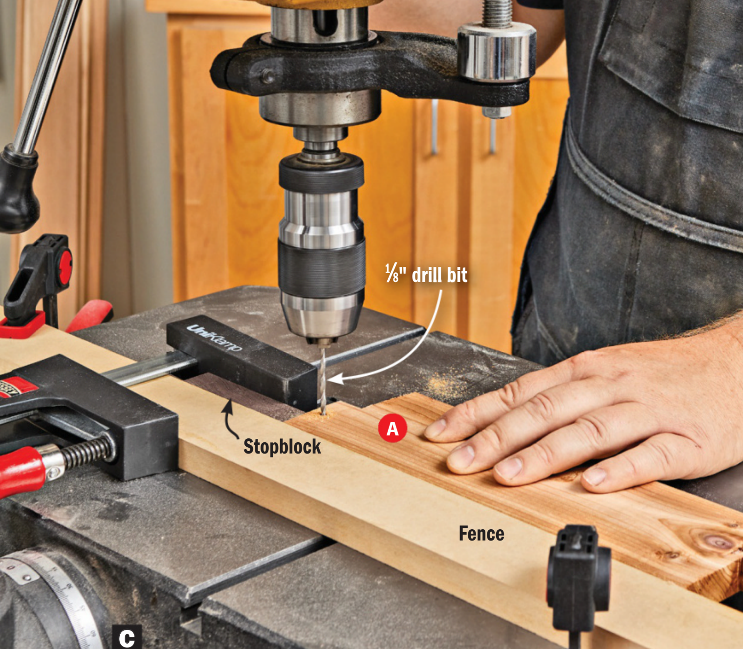
C Use a fence and stopblock to position each box side when drilling the 1/8"-dia. pilot holes.
