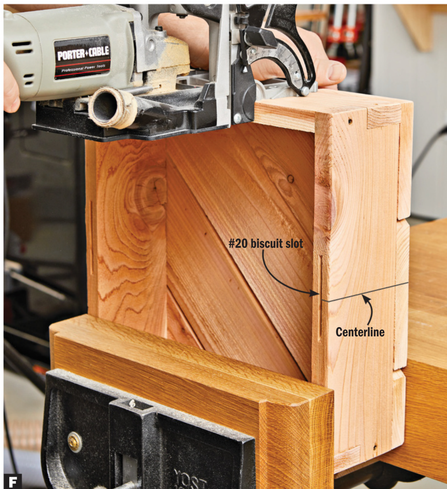
F Cut centered #20 biscuit slots on all the mating edges of the box frames.
