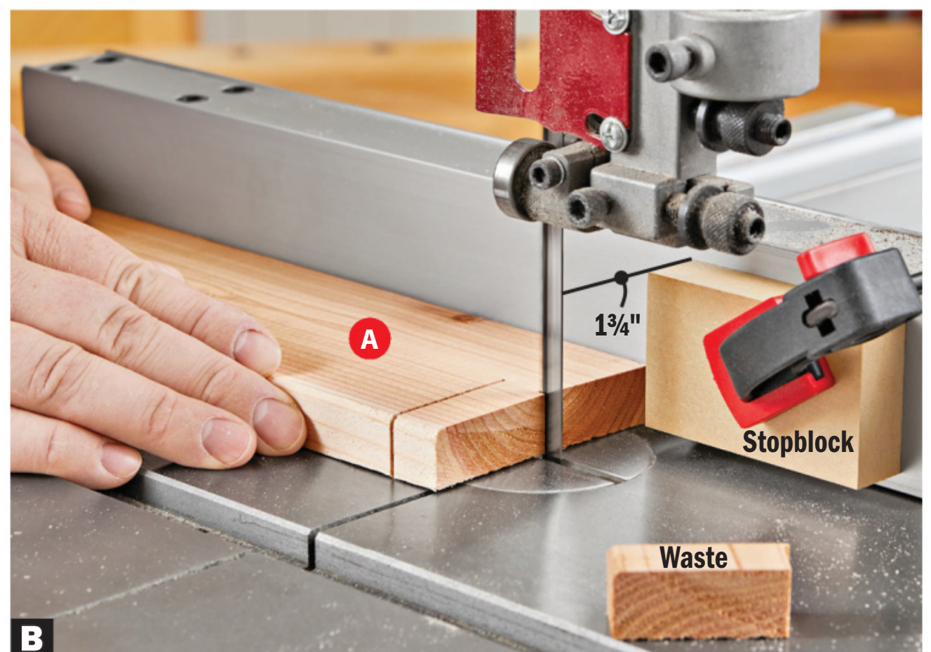
B Reposition the fence and stopblock to complete the notches. The waste piece falls safely to the side.
