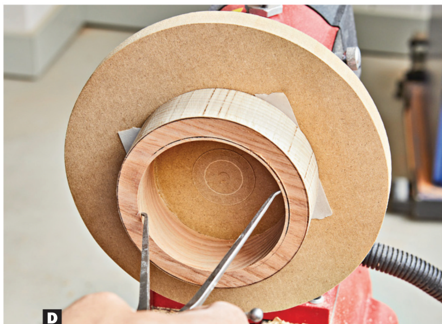
D Set calipers to match the diameter at the bottom of the ring. There should be no binding or gaps as you pull them outward.
