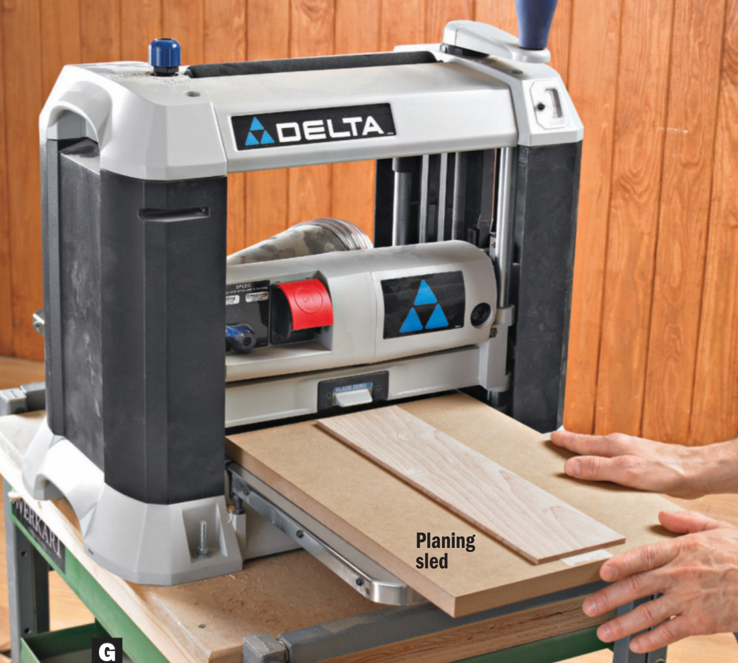
G A planing sled prevents damaging the thin pieces as they pass through the planer. Secure the strips with short lengths of double-faced tape.
