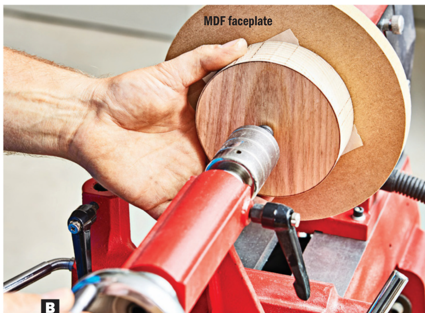
B Using the tailstock to help align the blank and press it in place, center the blank on the MDF faceplate.
