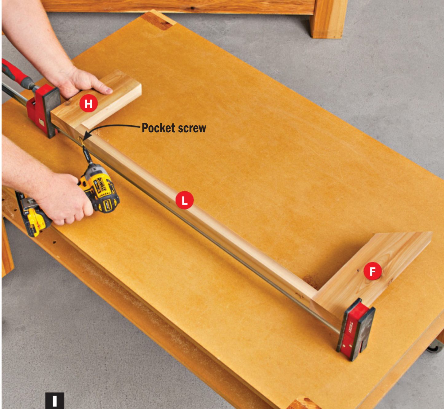
I Lightly clamp the filler (L) between the half rails (F, H) to prevent bowing the assembly. Drive a pocket screw at each end.
