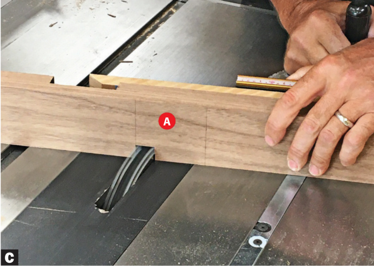
C Set your miter gauge to 15° and dado one edge. Check the fit of the legs (D) in the dado as you near your layout line. Then, simply reverse the miter gauge to cut the other edge.
