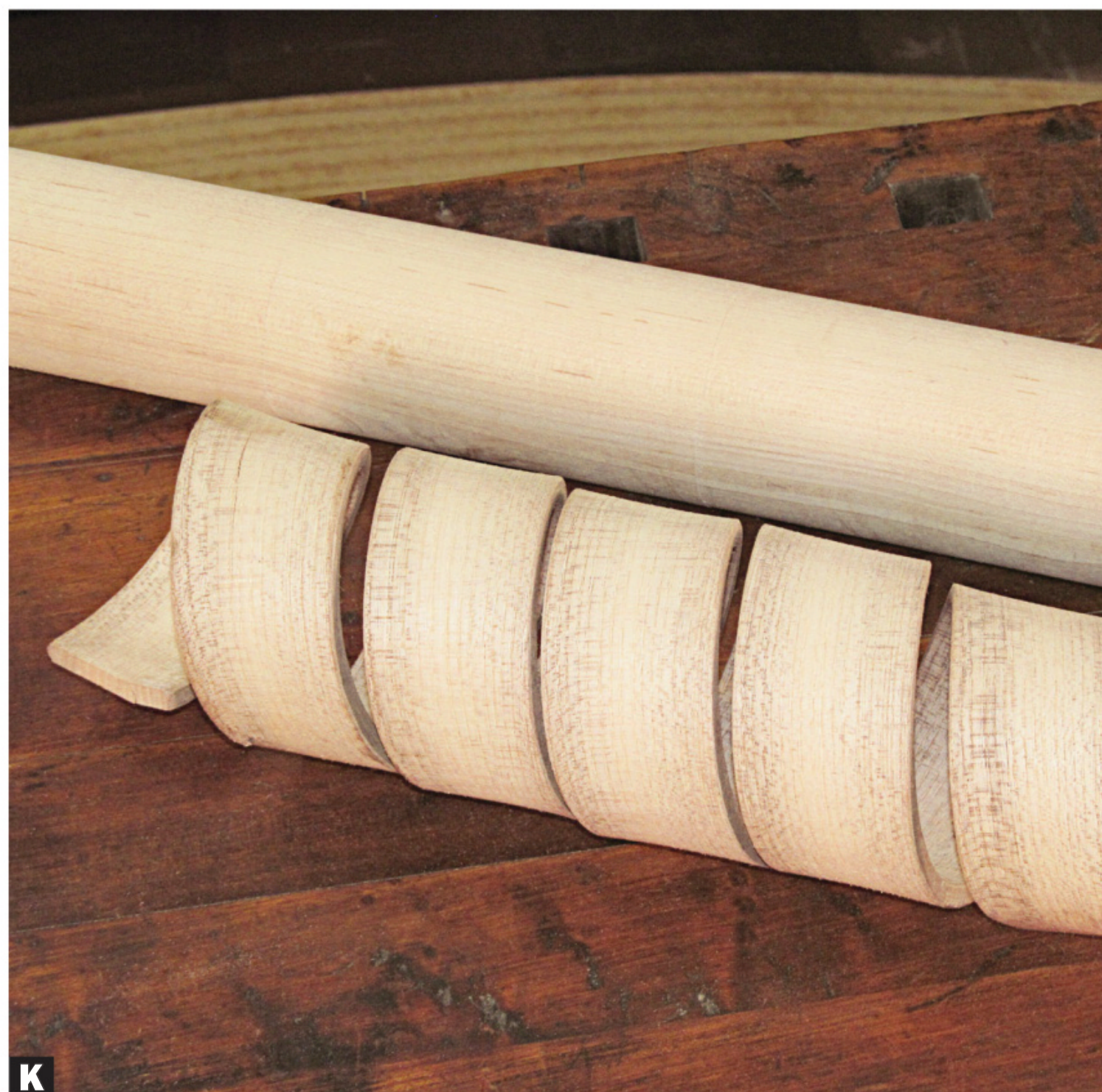
J Bend the wood around a form by hand, using clamps to hold it in position while drying. We let this coil dry around a 3"-diameter dowel for 12 hours.
