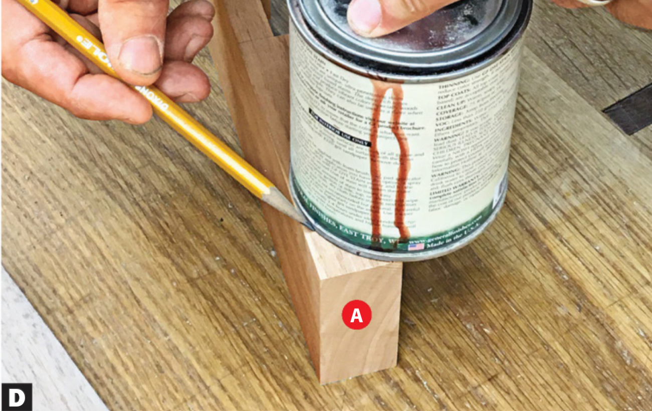
D Use a pint can of finish to lay out the radius. Bandsaw away the bulk of the waste and then sand to the line.
