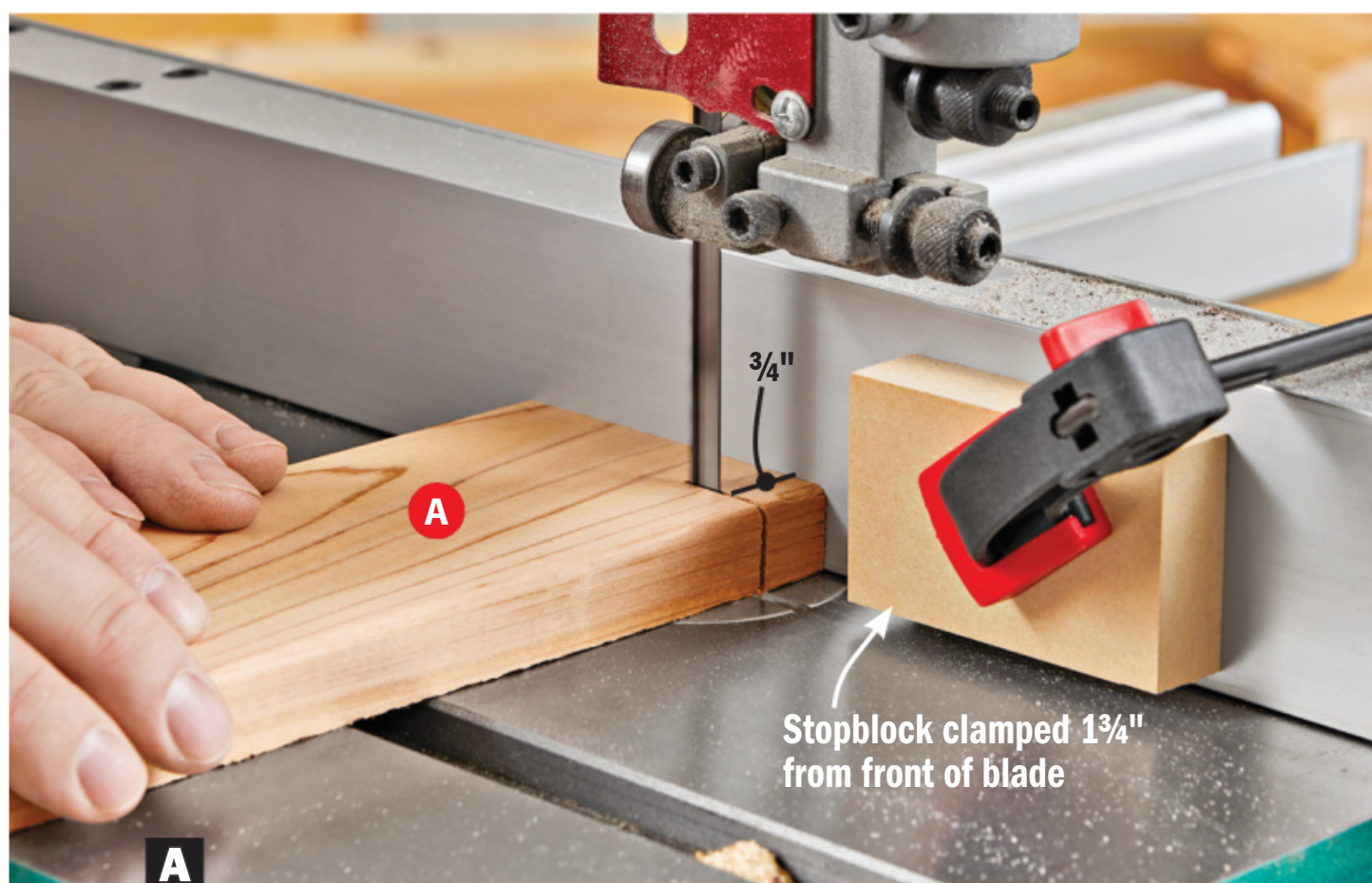
A Use a bandsaw fence and stopblock to make a crosscut at each end of the sides (A), stopping at the centerline of the part.
