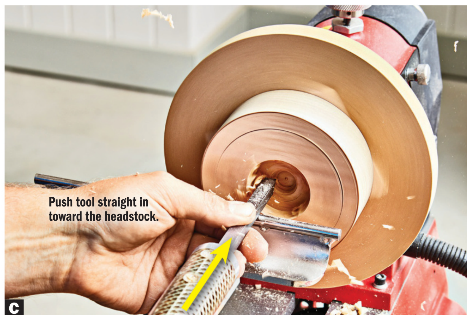
C Keep the tool parallel to the lathe bed both up and down and side-to-side. Make the first cuts near the center and on the horizontal centerline. Then, raise the tool rest to cut just above the centerline.
