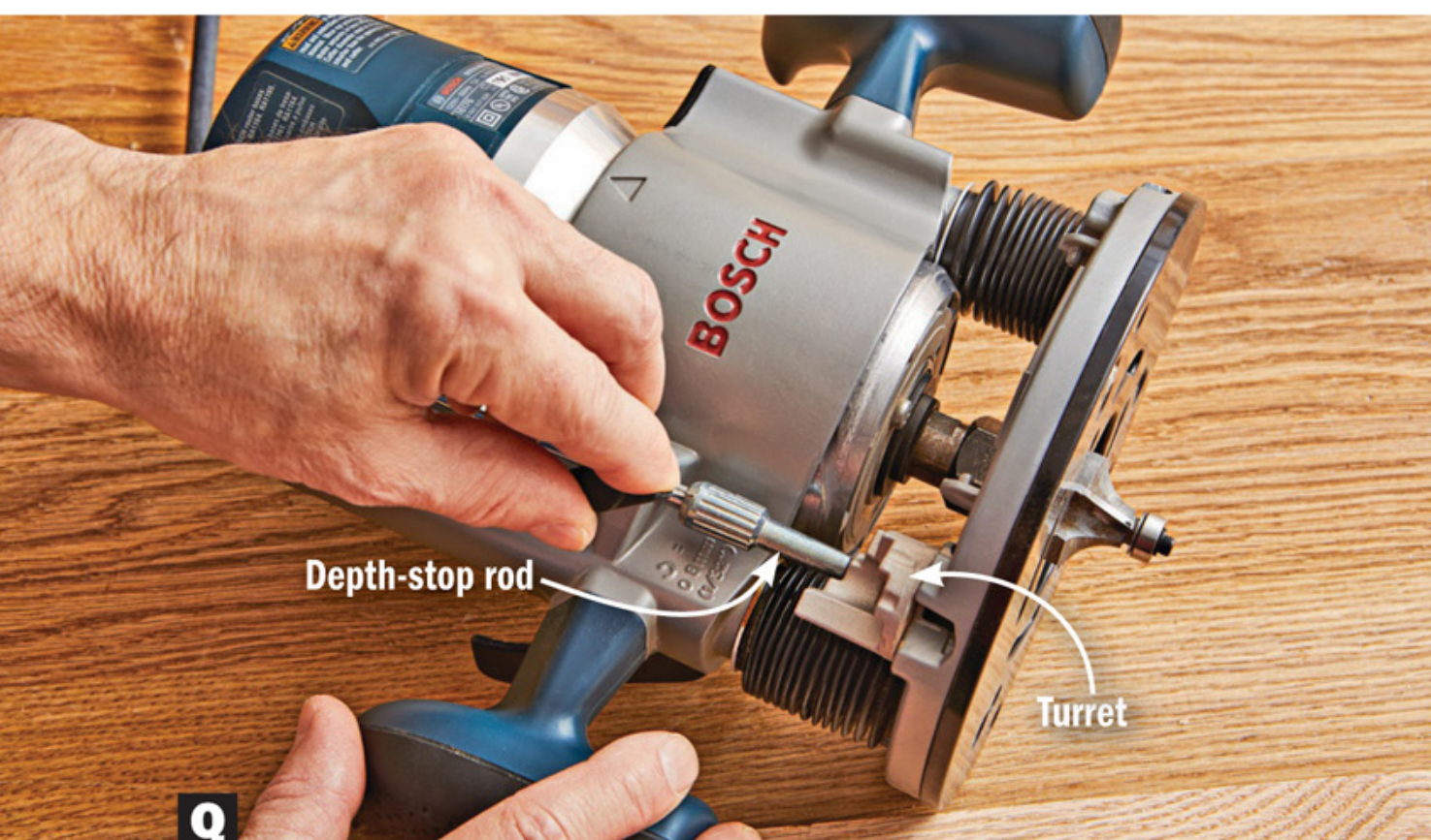
Q For a three-step cut, first plunge the bit to the final depth. Rotate the turret to one of its lower steps and adjust the depth-stop rod to contact it.
