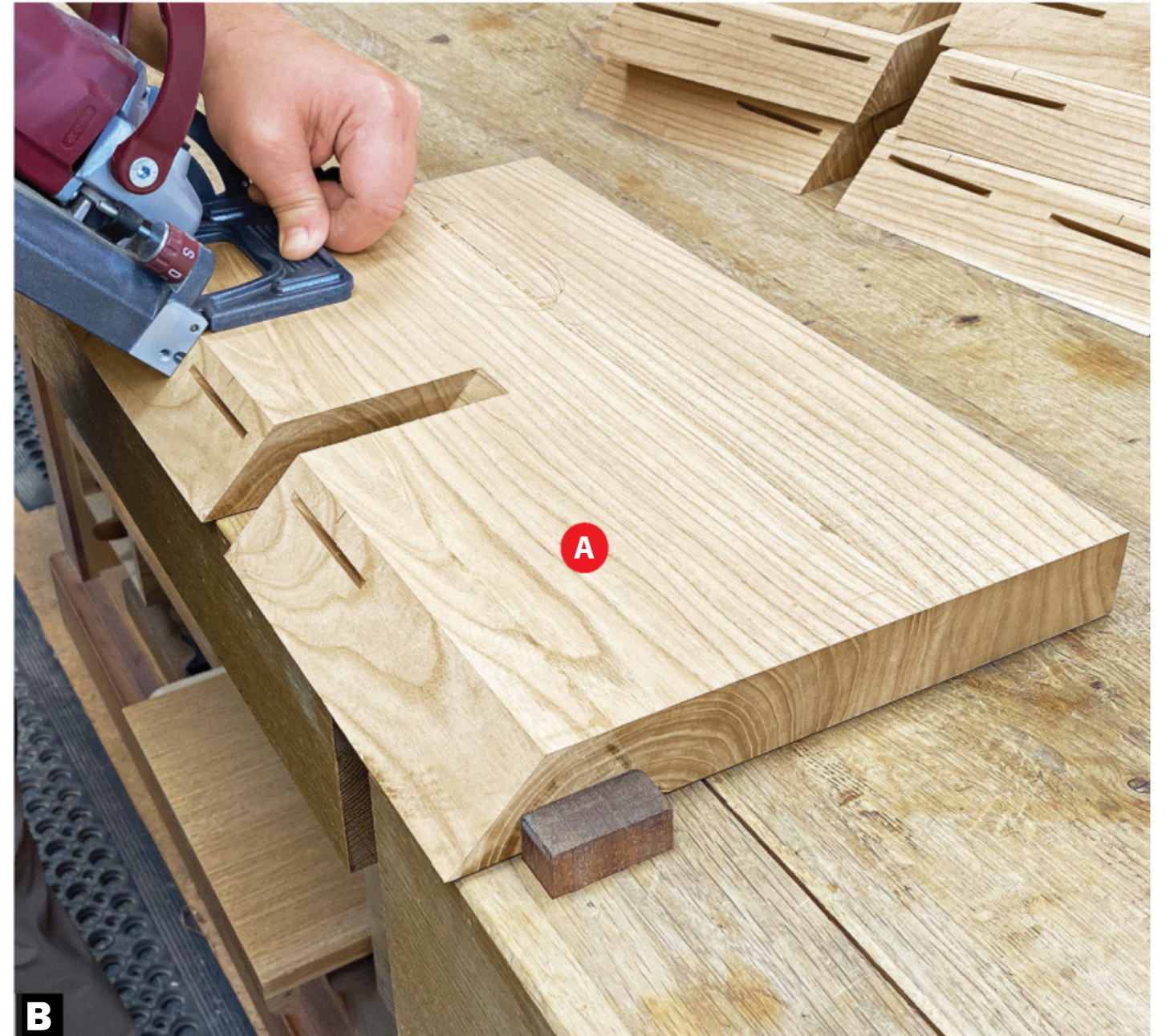
B Cut two slots above the notch and one below making sure you stay clear of the arch that will be cut in each leg.
