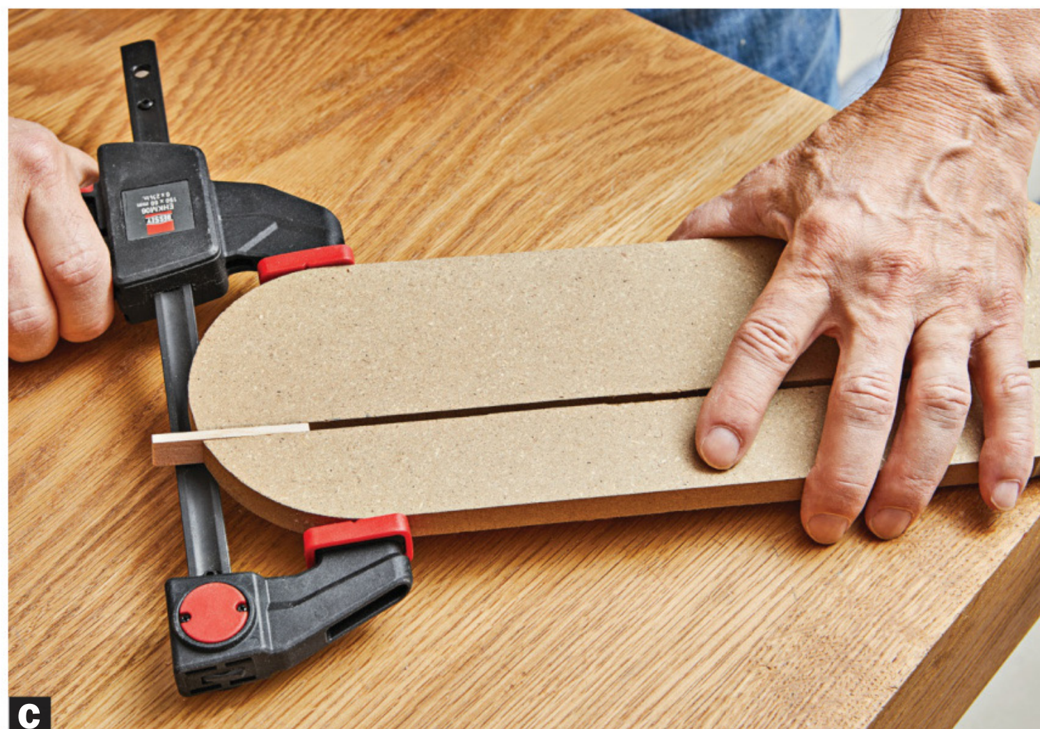
C After gluing in an oversize spacer, use a chisel and sandpaper to bring it flush with the edge and surface of the insert.
