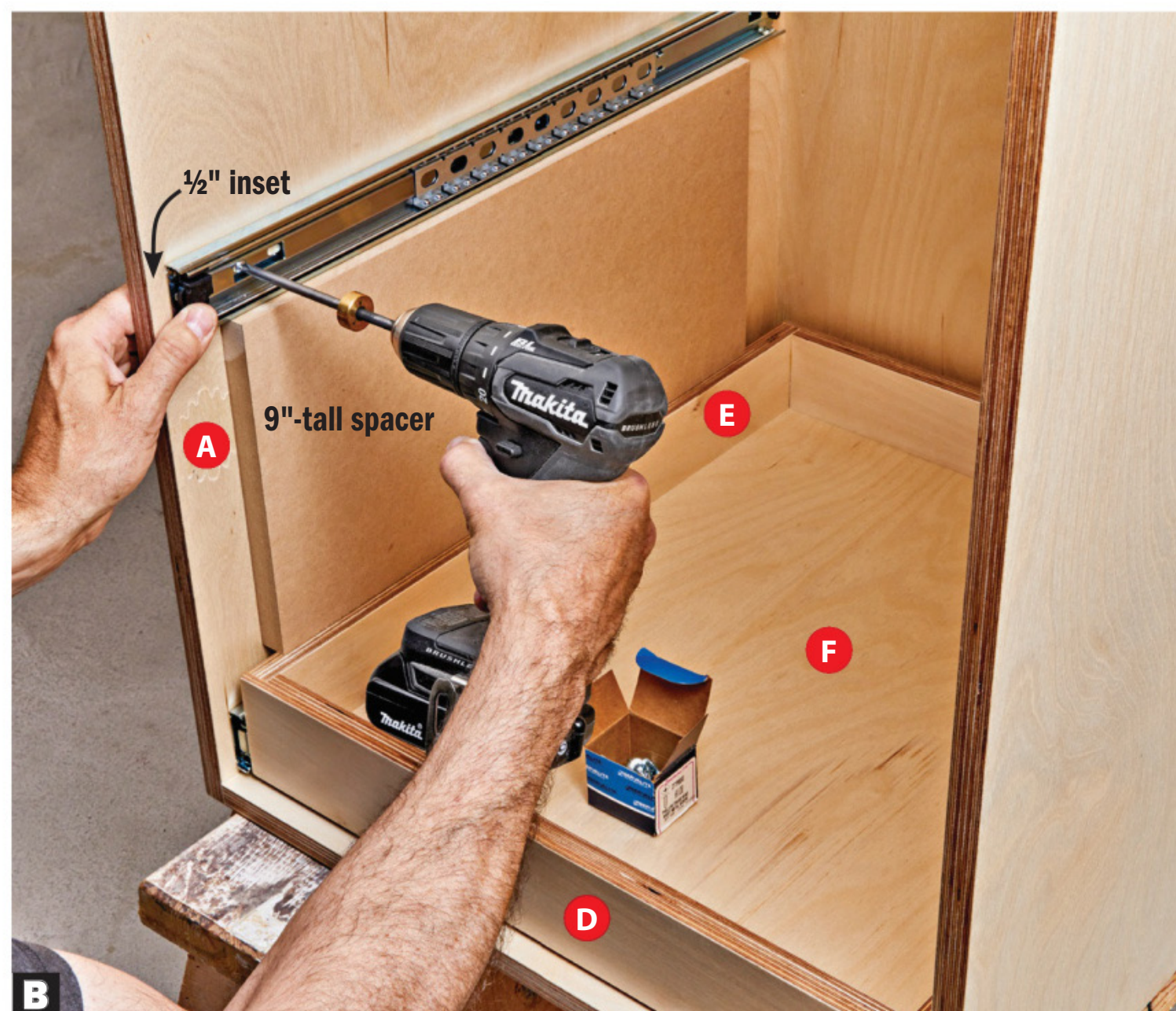
B Rest the drawer spacer and drawer slide on the bottom drawer side (E) while you screw the inset slides to both sides (A).
