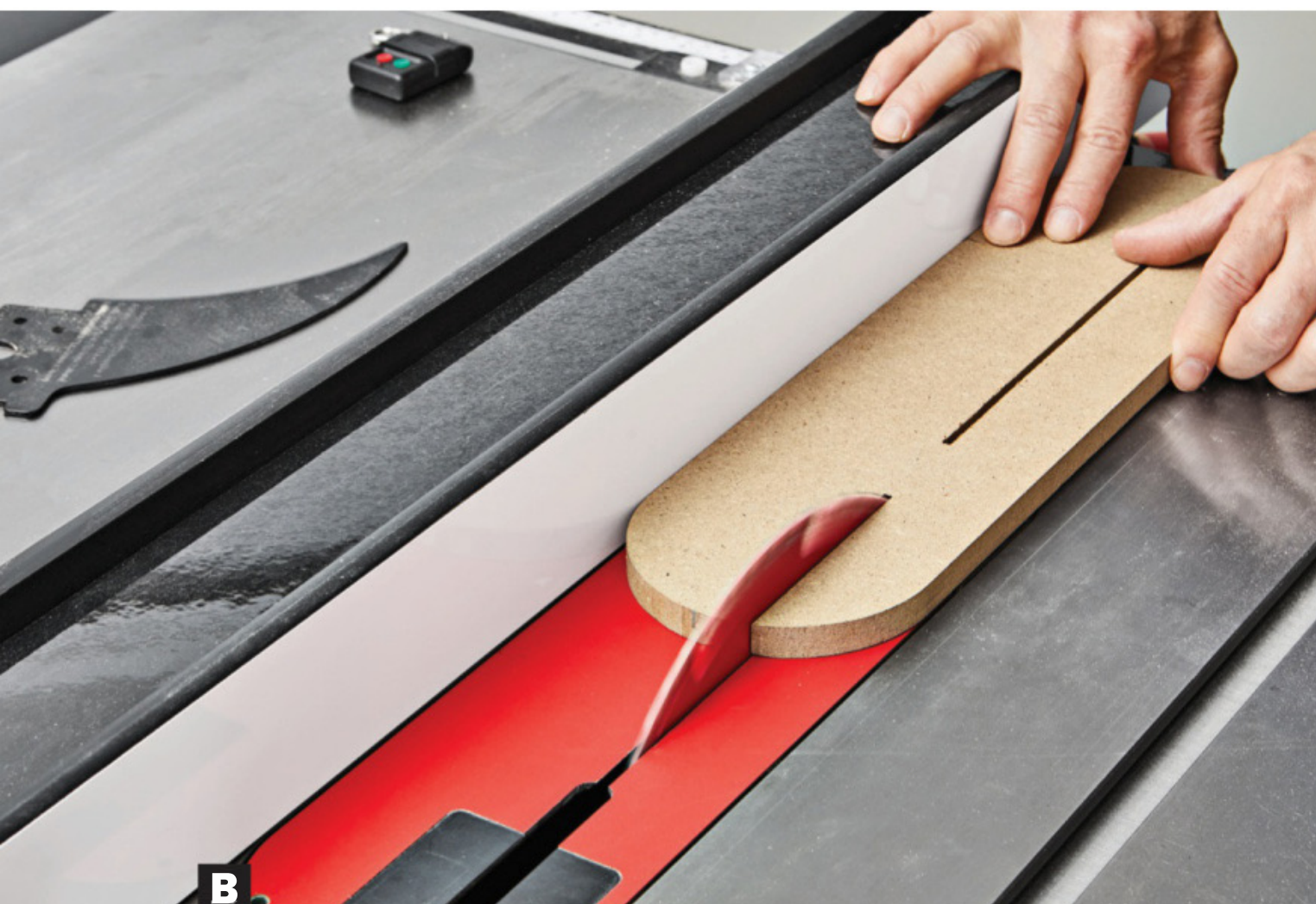
B Guide the insert along the rip fence until you reach the previously cut opening. Turn the saw off and let the blade come to a stop before backing out of the cut.
