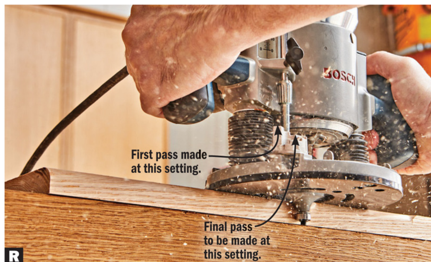
R Rotate the turret two steps to a higher step, and make the first cut. Then, rotate the turret and make a deeper pass. One more pass at the original turret step will complete the profile.
