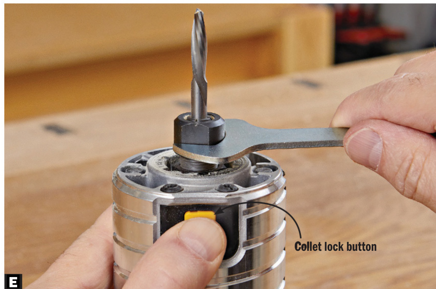
E A collet lock prevents the spindle from turning so you can tighten the collet using only one wrench.
