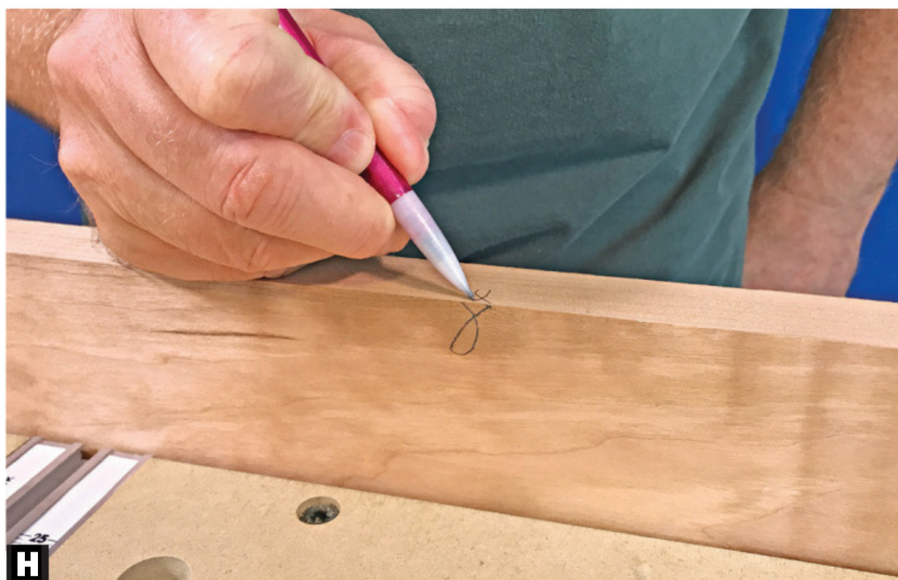
H Mark the squared edge adjacent to the face mark. This face and edge serve as references when trimming to final width and thickness.
