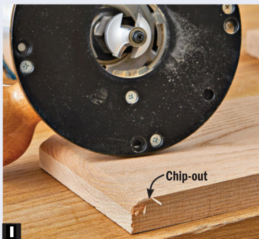
I As the bit rotates out of the workpiece, it tears unsupported wood fibers along the adjacent edge. Stringy woods, such as oak, prove especially prone to chip-out.
