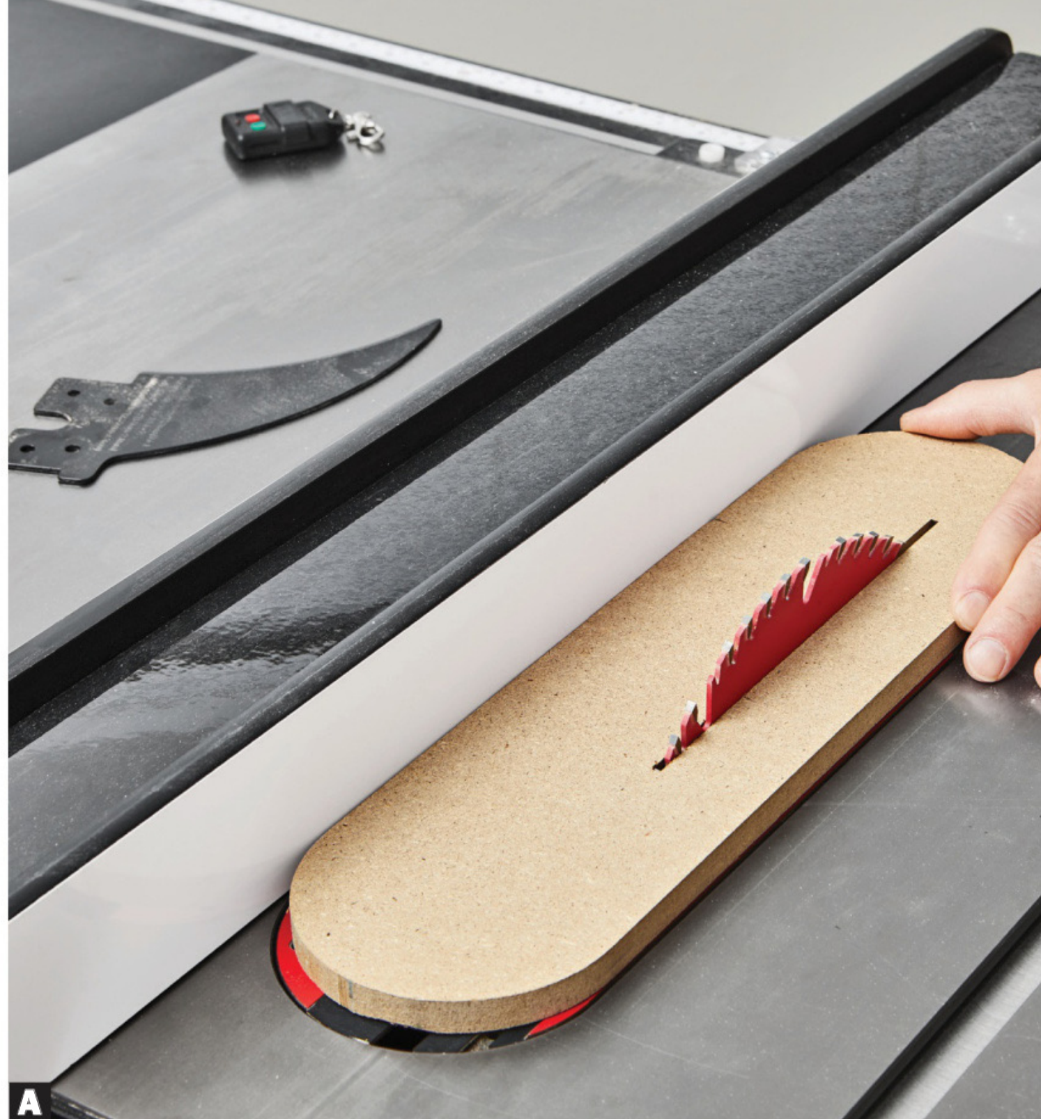
A Use the blade to position the zero-clearance insert, then bring up the rip fence until it just kisses the edge of the insert.
