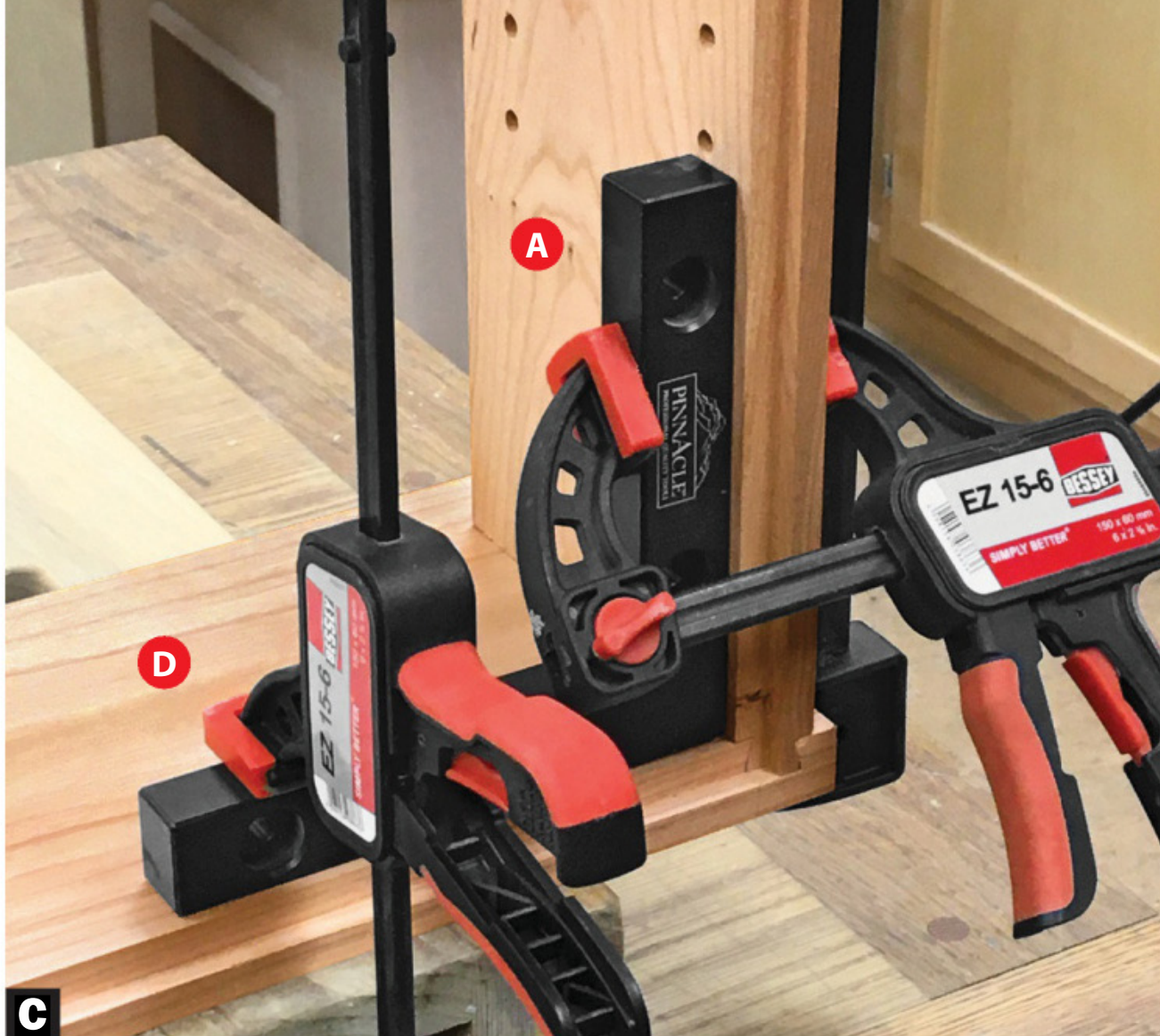
C Use clamping squares to hold the sides (A) and dividers (B) square to the bottom (D) until the glue dries.
