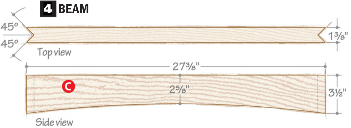
H Tilt the blade to 45° and make successive cuts, raising the blade slightly each time until the low side of the kerf hits the centerline of the beam. Attach a stopblock to the auxiliary fence and make the remaining cuts.
