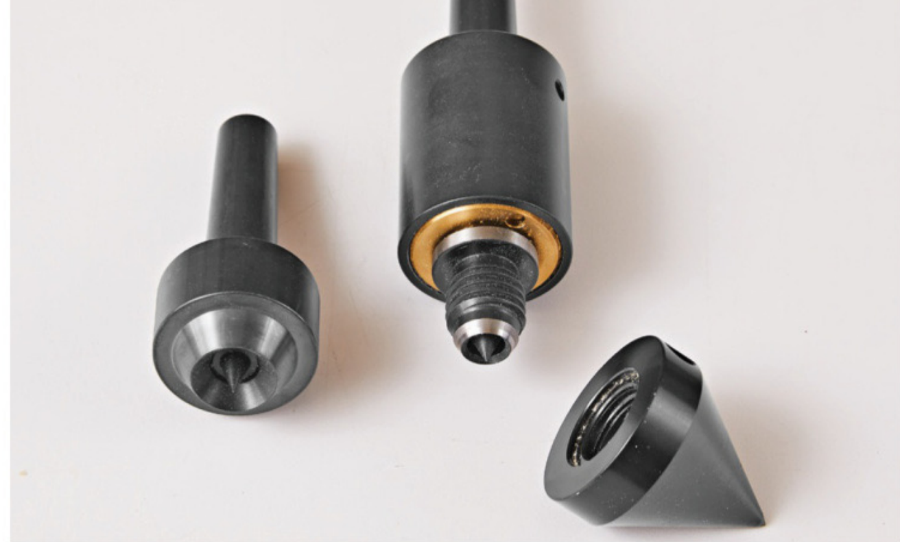
Grizzly and Nova supply a standard live center (left), but Jet, Laguna, Oneway, and Powermatic up the ante with a heavy-duty live center (right) that features more bearings for smoother operation.
