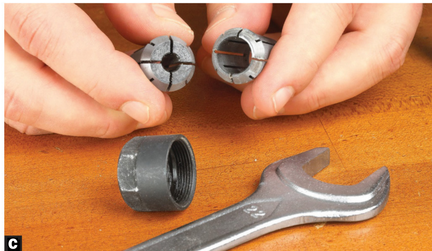
C Collets match bit-shank diameters, the most common being ¼" and ½". Not all routers accept ½" bits, and some use a reducer to fit ¼" bits in a ½" collet.
