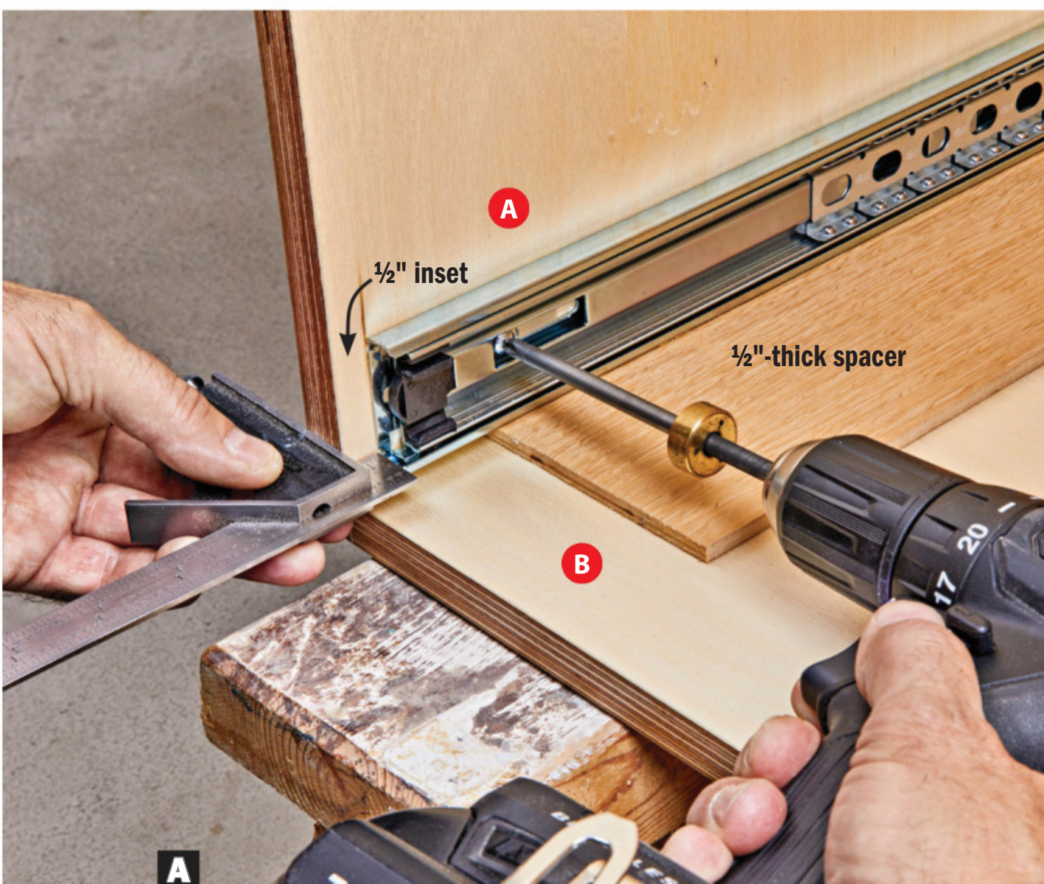
A Rest the drawer slide on a 1/2" spacer with the front end 1/2" from the front edge of the side (A). Then screw the slide in place.
