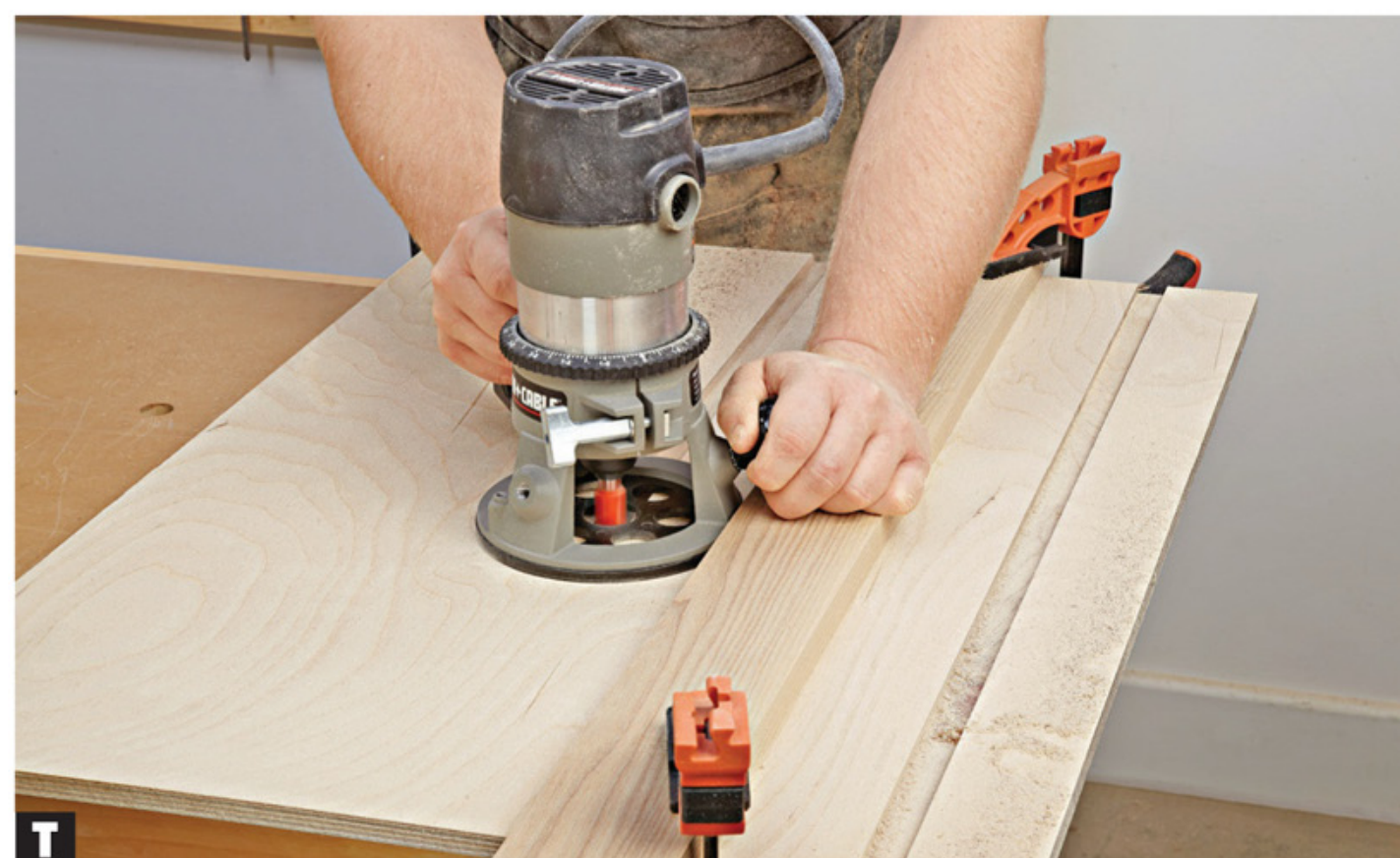
T Ride the router base against a straightedge to cut a dado or groove in a workpiece.
