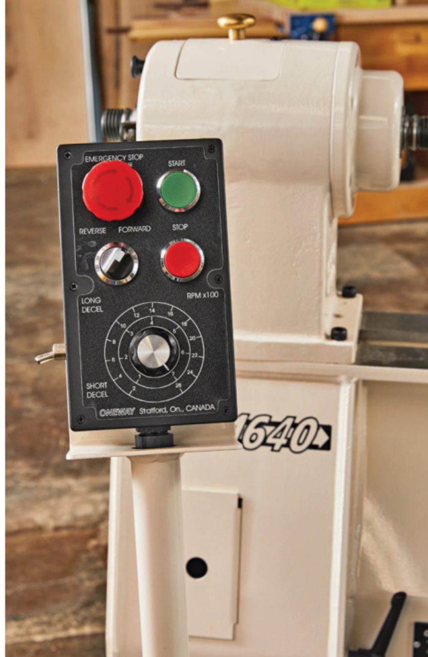
Oneway's pedestal-mounted controls swing easily from the headstock to the tailstock ends of the machine, or anywhere between.
