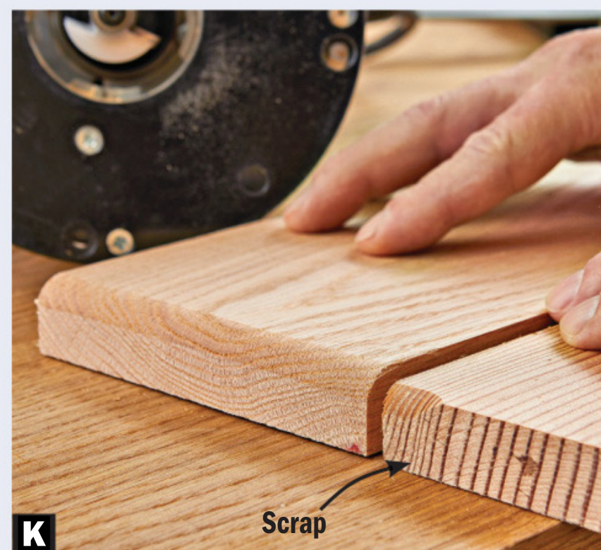
K Clamp a scrap the same thickness as the workpiece flush with the end of the board. This supports the fibers along the edge, resulting in a clean corner.
