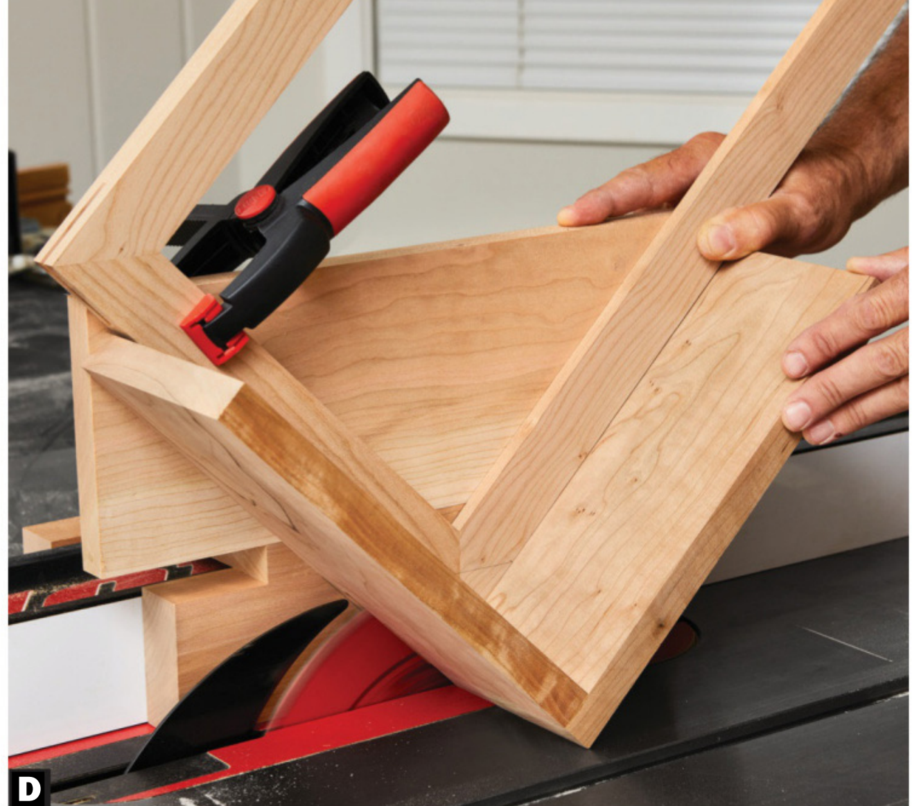
D Use a rip blade when cutting the spline slots. The flat teeth leave a crisp, flat bottom. Adjust the blade height so that you cut about halfway through the miter.
