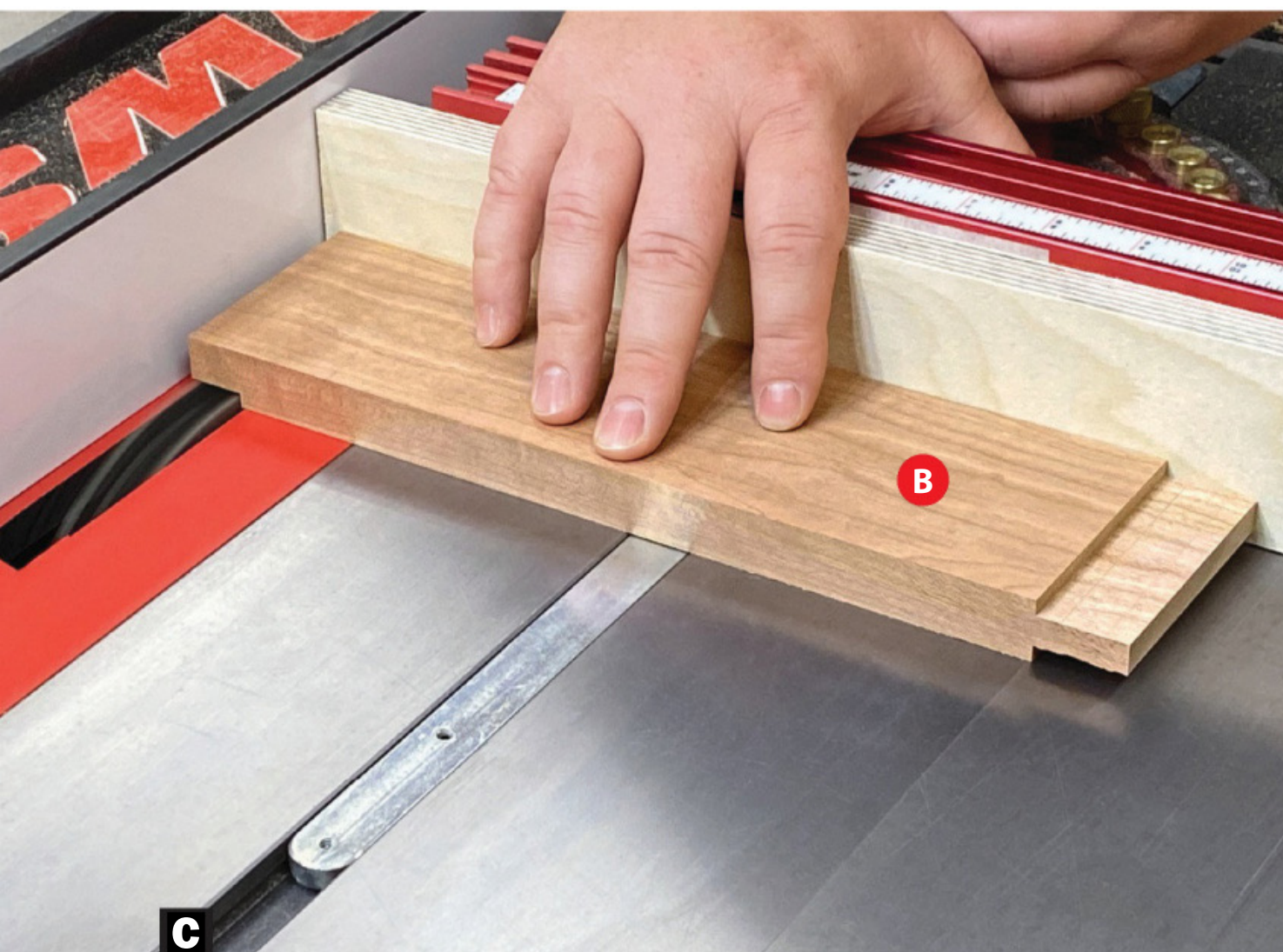
C Set the rip fence 1" from the outside of the blade, and make a pass on each face. Sneak up on the blade height, testing the tenon's fit in the mortise until the tenon slips in.
