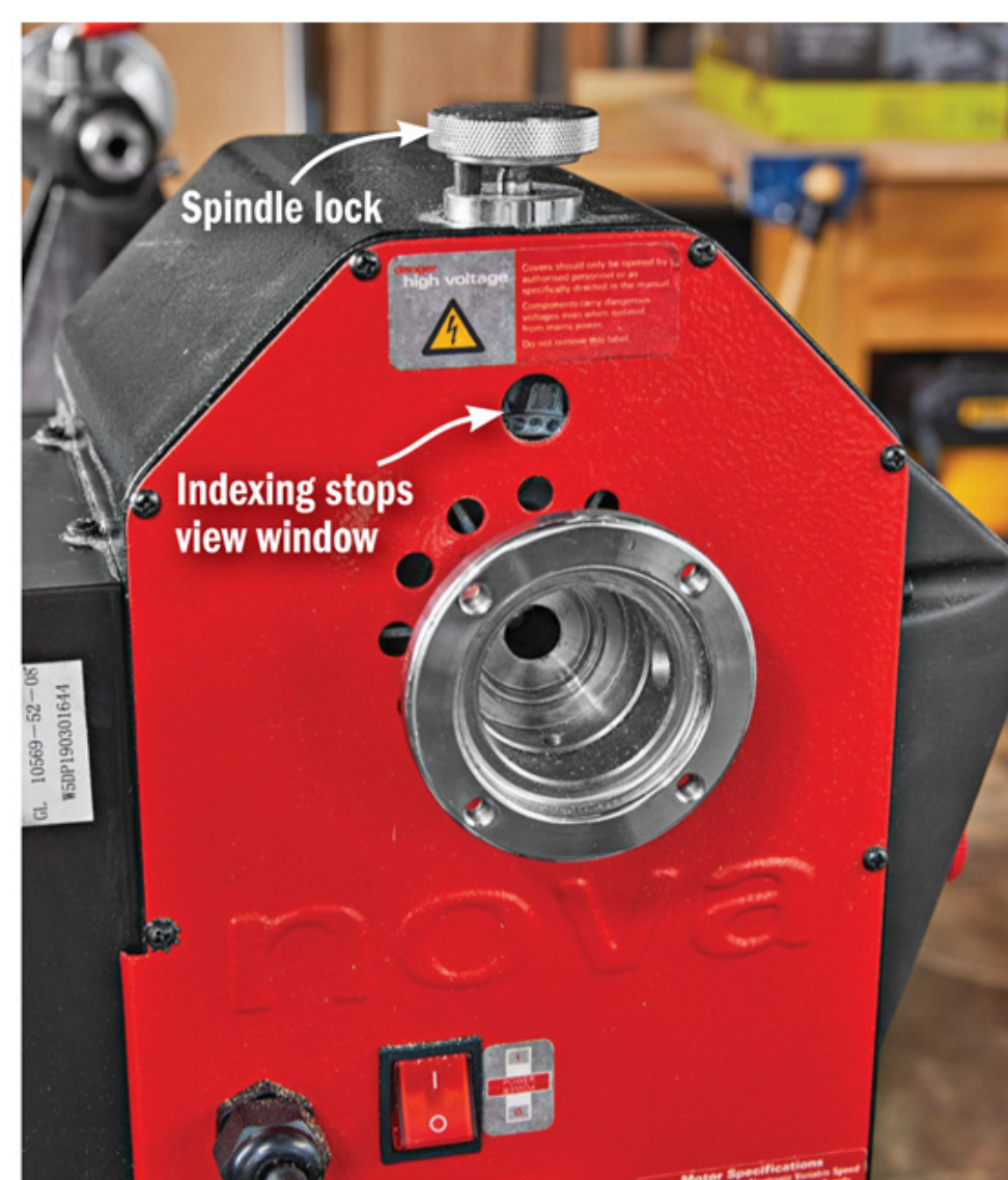
A small view window inhibits spotting the Nova's indexing stops. Once engaged, the stops tested accurate.
