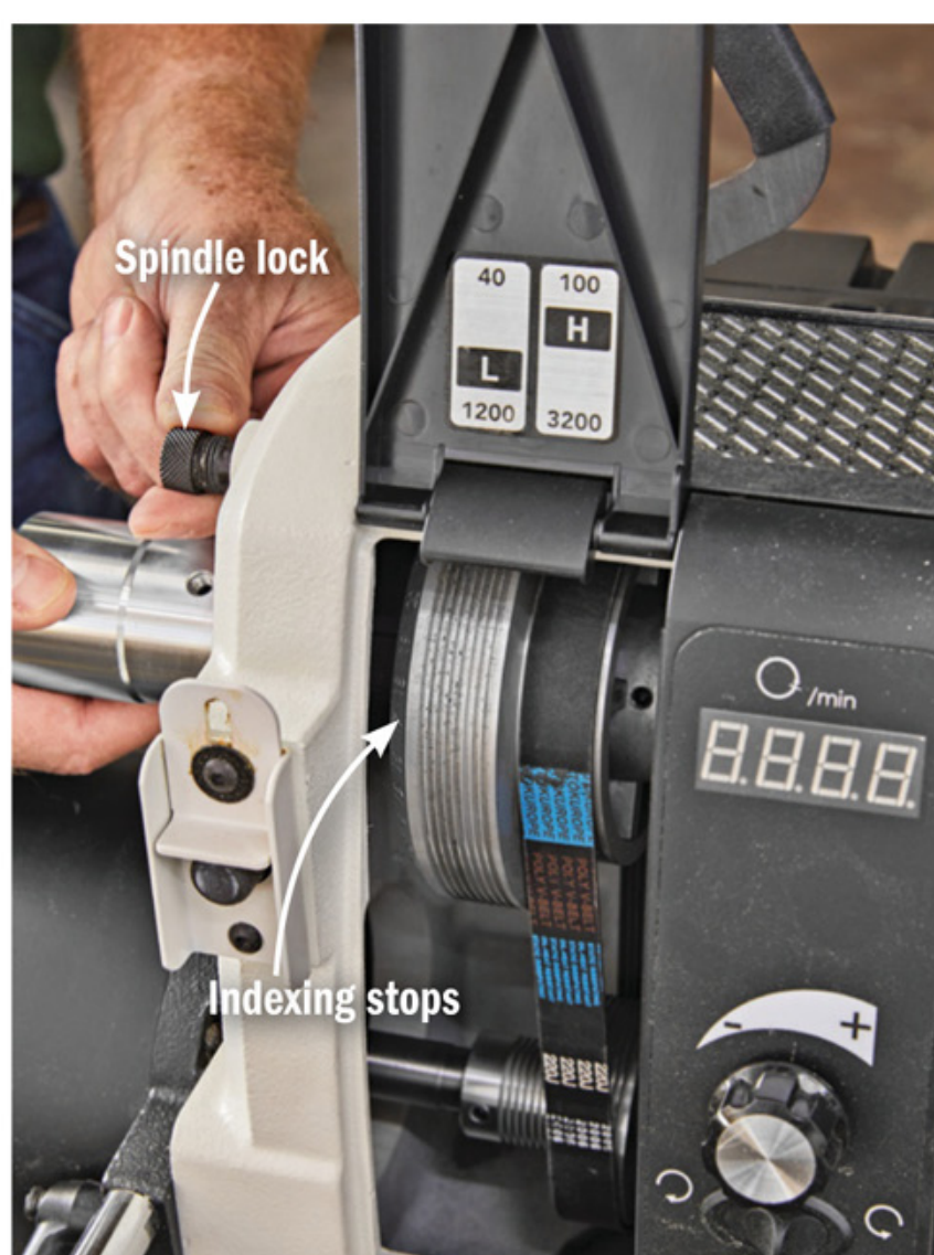
We found Jet's indexing positions difficult to see on the drive pulley. Turn the spindle until the stop you want aligns with the spindle lock, then engage it.
