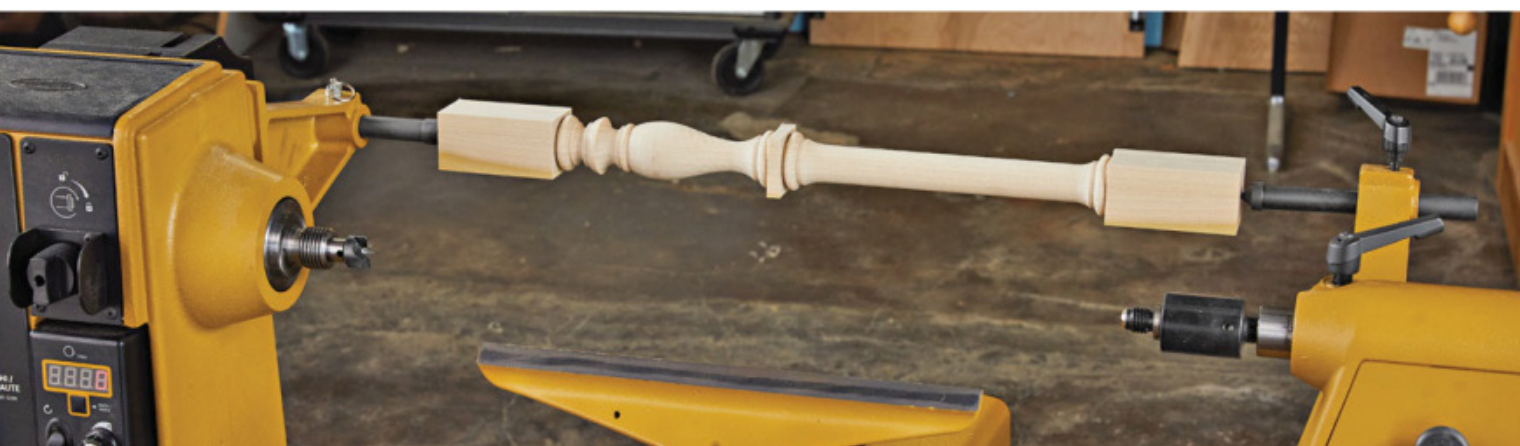
The Powermatic comes with a comparator, a pair of arms with adjustable pointed holders. This allows you to better copy a spindle by having it right in front of you.
