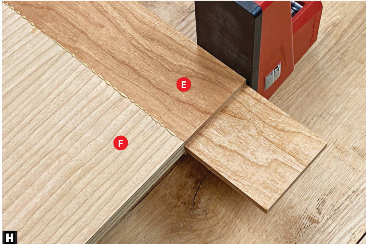
H Align the shoulders of the short trim (E) with the edges of the top (F). Ensure the parts stay aligned as you apply clamping pressure.
