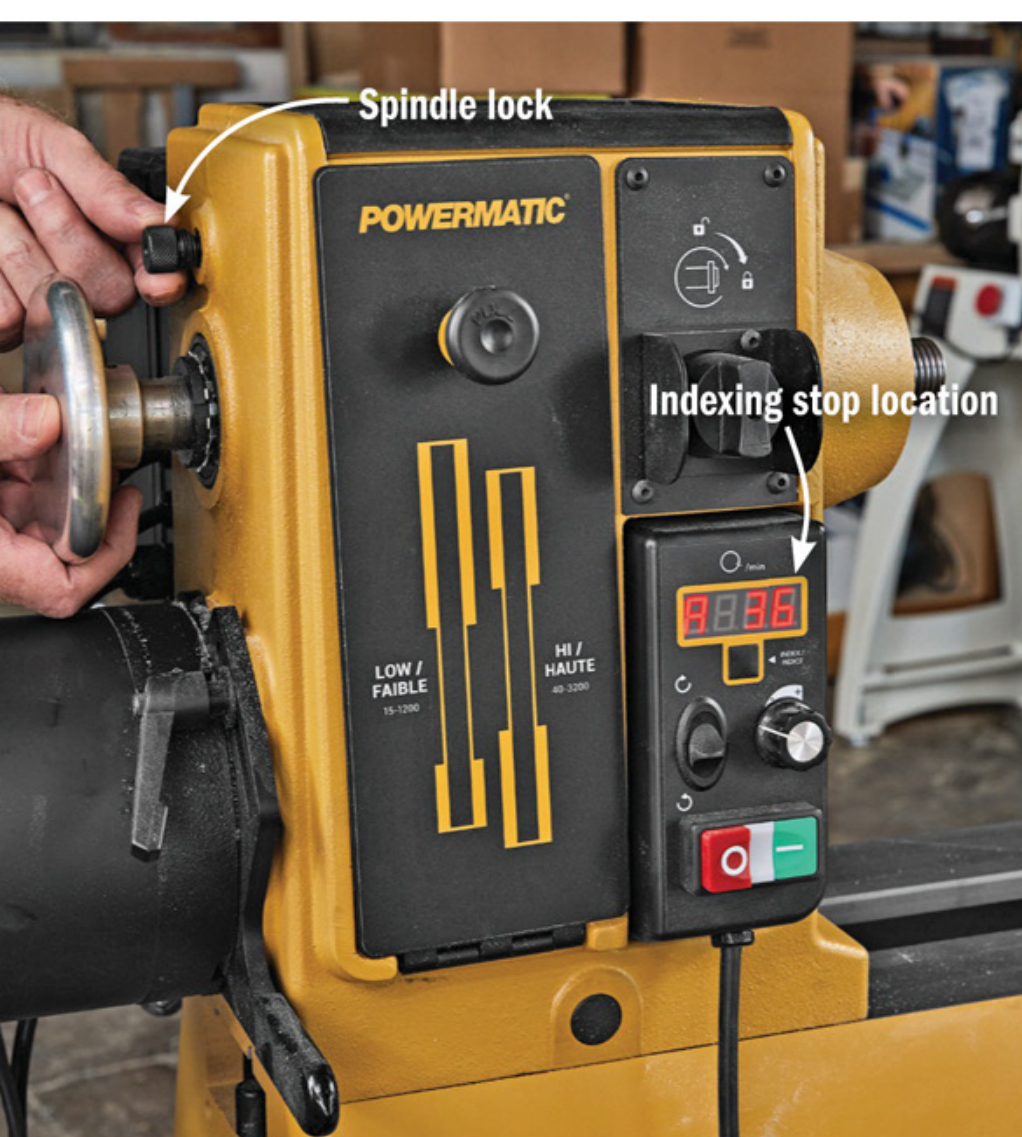
To set Powermatic's indexing stops , turn the handwheel until the stop number appears on the digital readout. Then engage the spindle lock.
