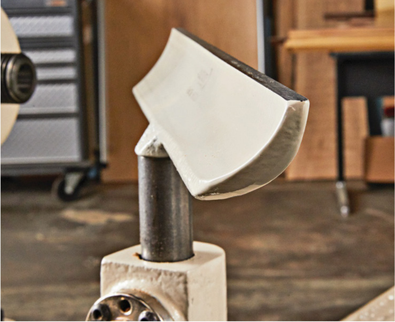
The curved shape of Oneway's tool rest fits nicely into the rounded sides of bowls, giving you better placement and control.
