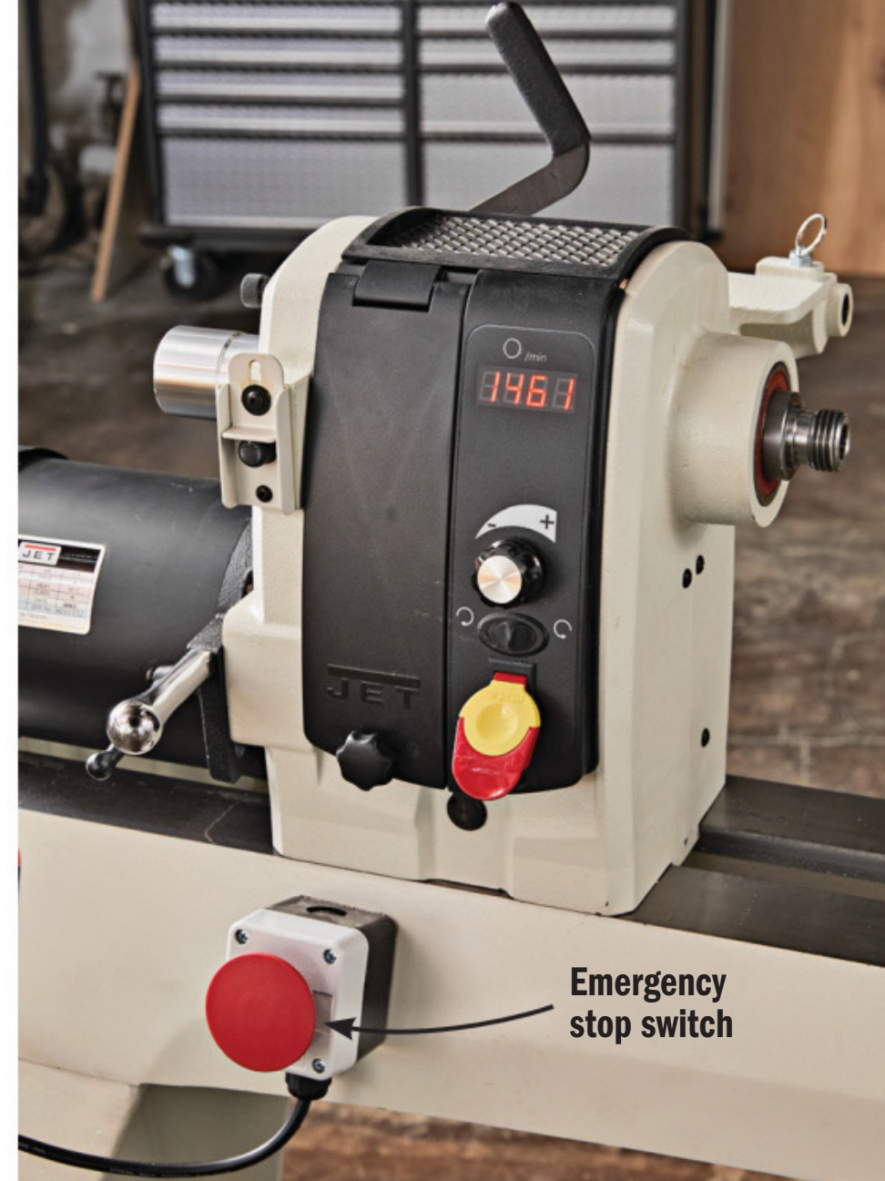
Place Jet's magnet-mounted emergency stop anywhere on the lathe. Restarting after an emergency stop requires using the primary on/off switch.
