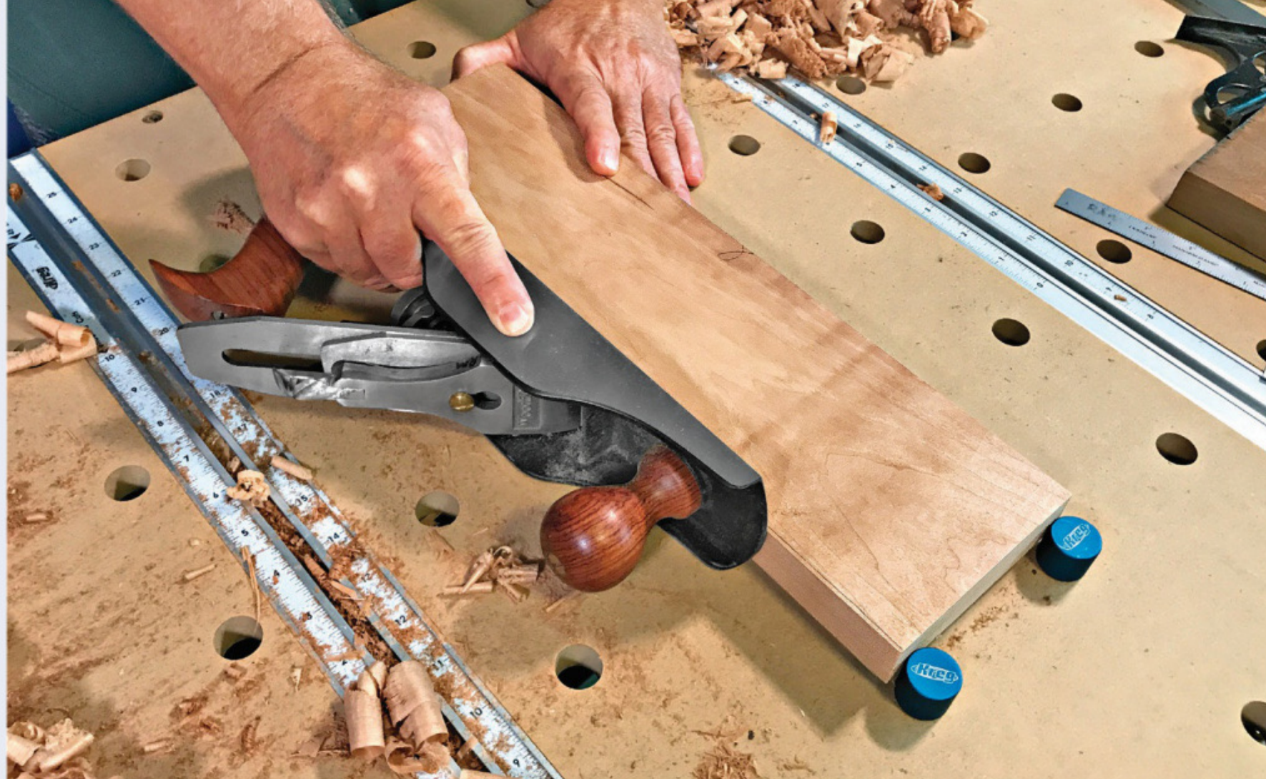
With the workpiece elevated slightly, the full thickness of the workpiece contacts the plane blade.
