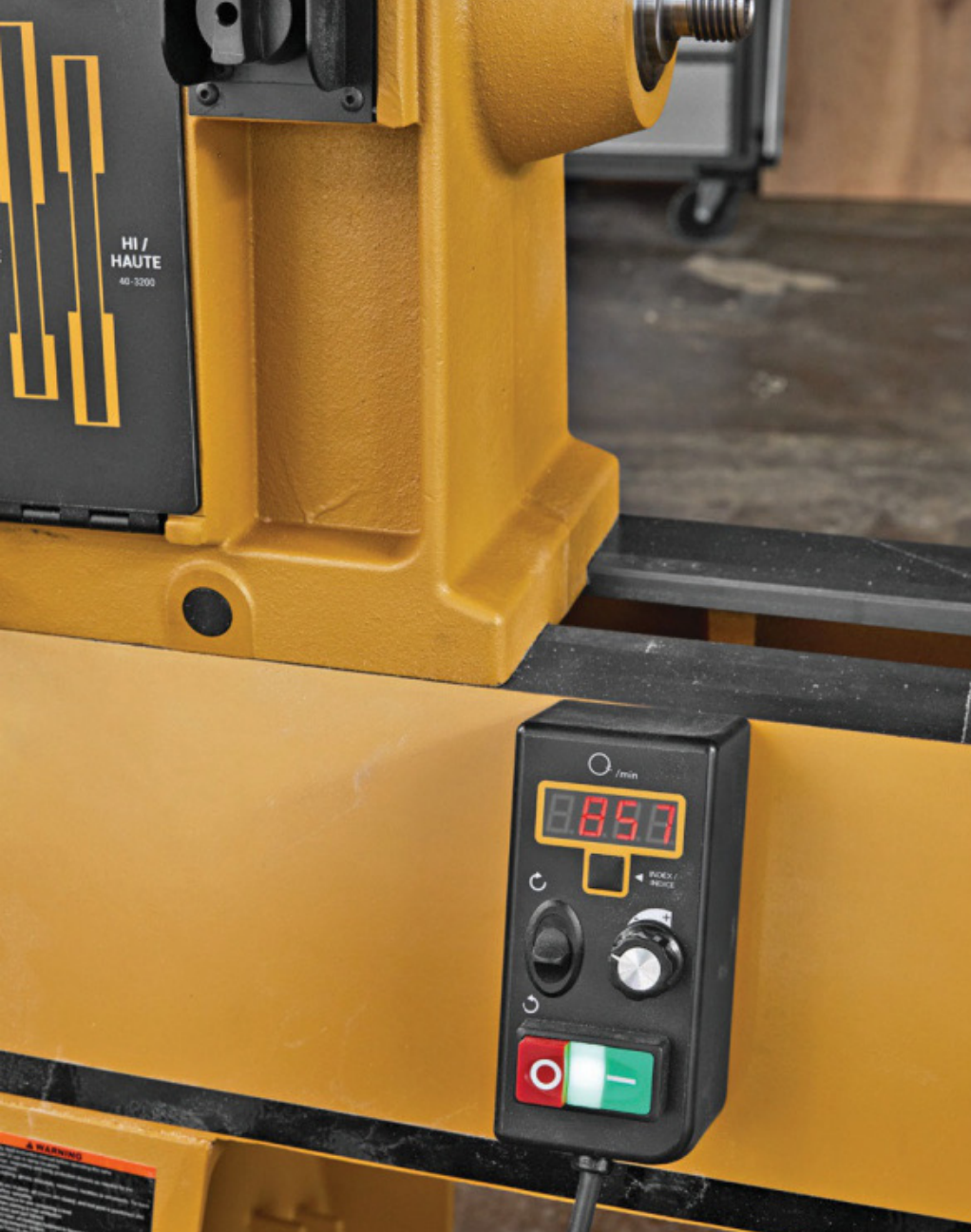
Position Powermatic's magnetic-mounted on/off switch anywhere on the machine you want—helpful if you prefer the switch nearer your dominant hand, and for outboard turning.
