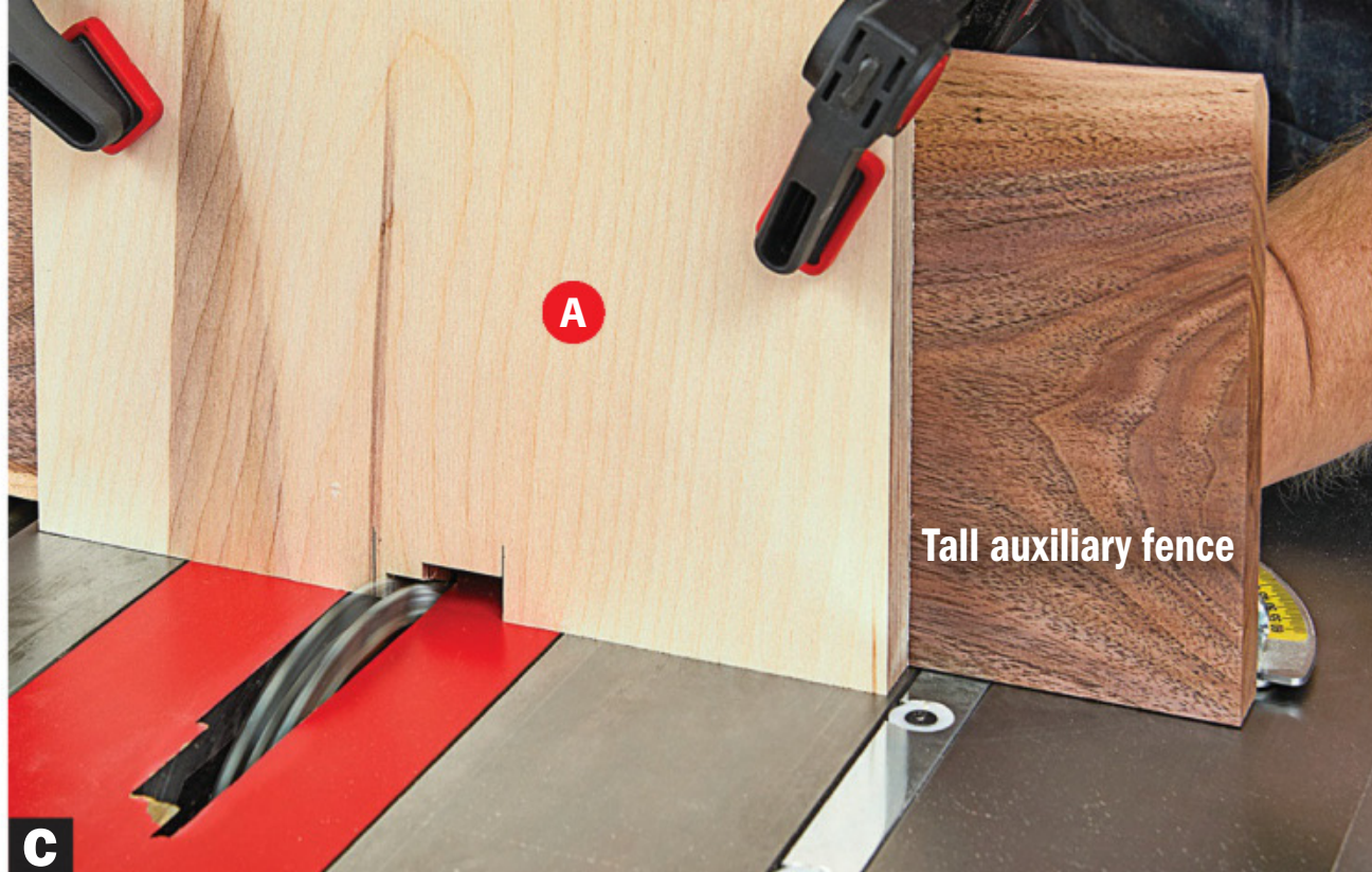
C Make overlapping cuts with a dado blade to cut a centered notch on each end of the riser top (A).
