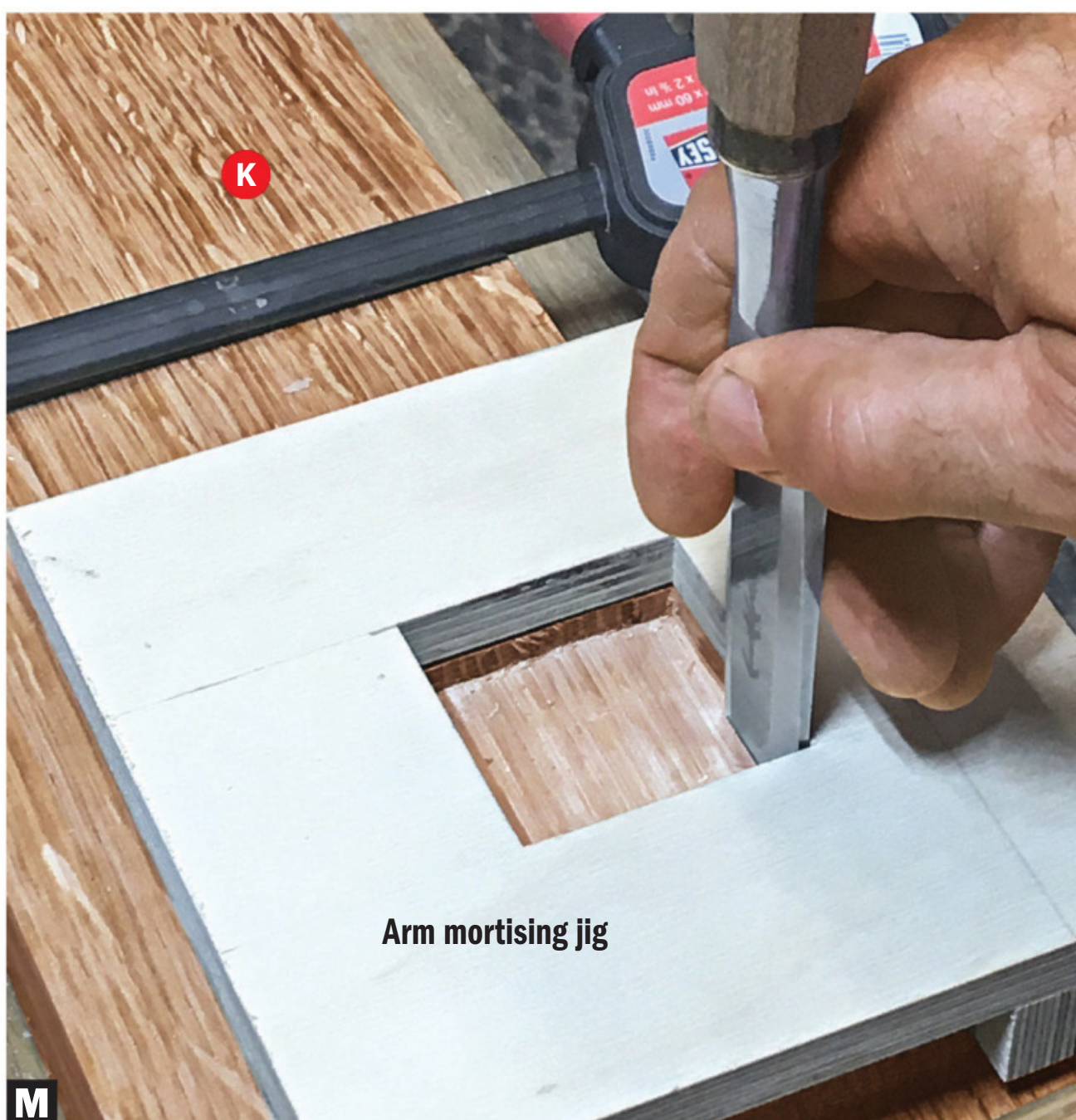
M After routing, leave the jig in place as a chisel guide to square the corners.
