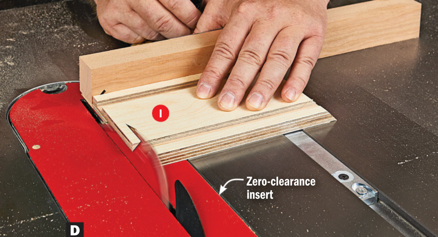
D Tilt your saw blade 45° and miter-cut the drawer and router-stand parts to length.
