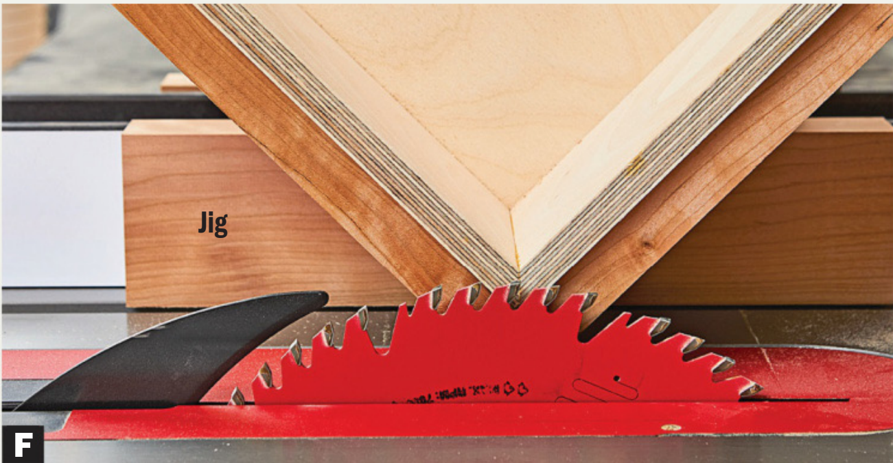
F With the drawer resting in the jig, set the height of the blade to cut halfway through the corner joint.
