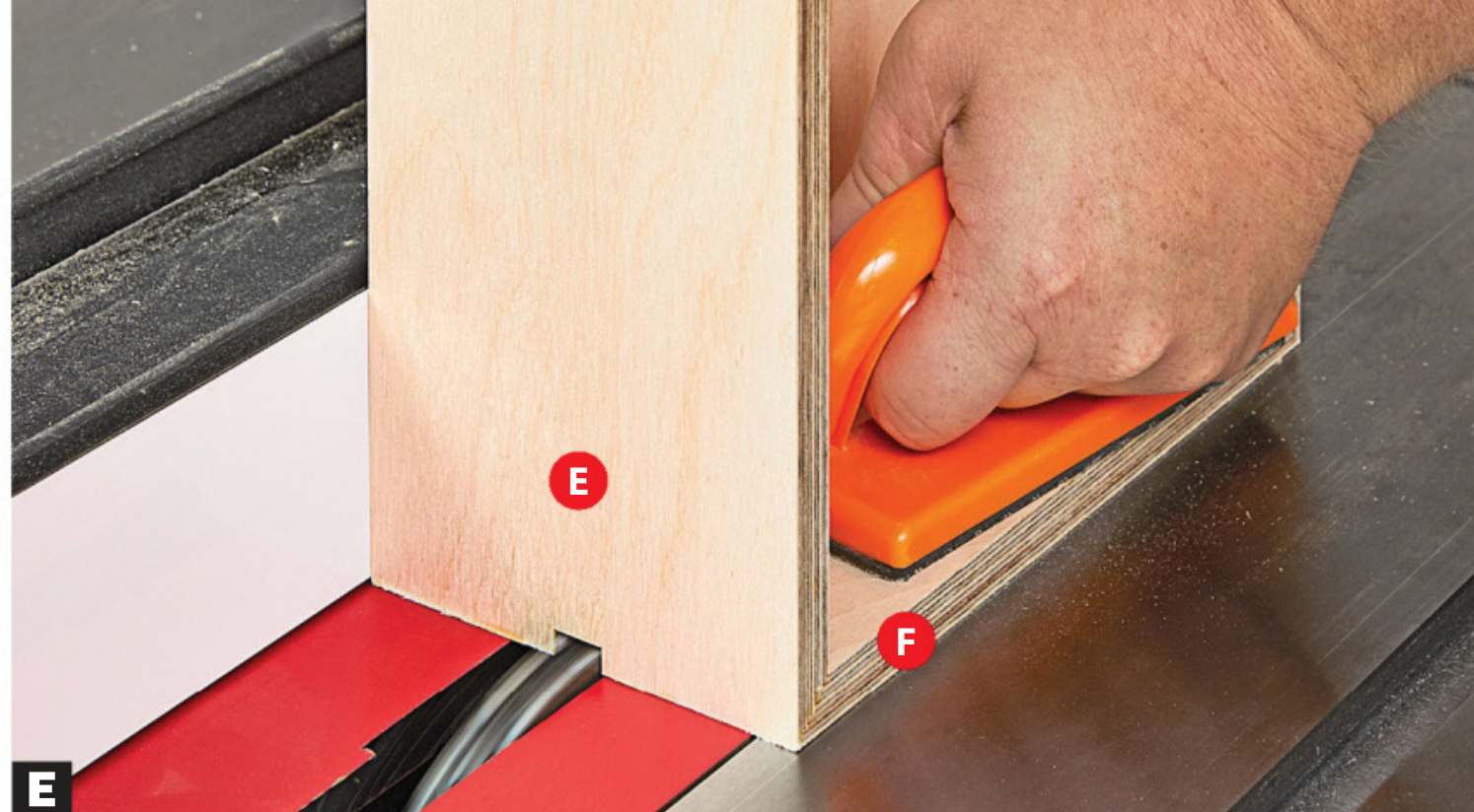
E Using a dado blade, position the rip fence to cut a centered, 1/2"-wide groove on the front of the drawer and router stand for a handle.
