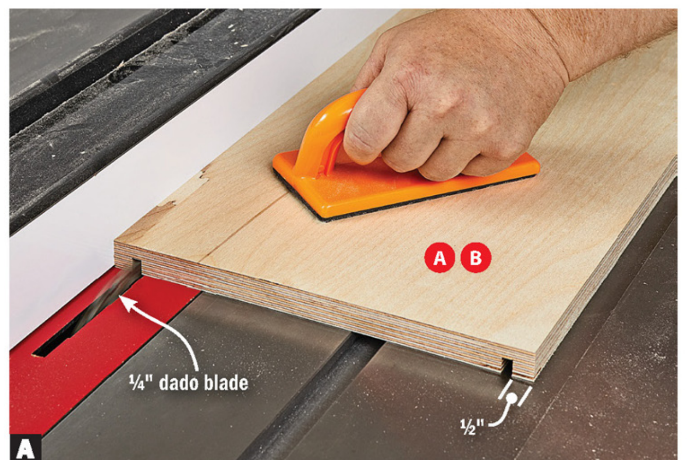
A With a dado blade in the saw, position the rip fence to cut 1/4"-wide grooves 1/2" from the edges of the riser top (A) and bottom (B).
