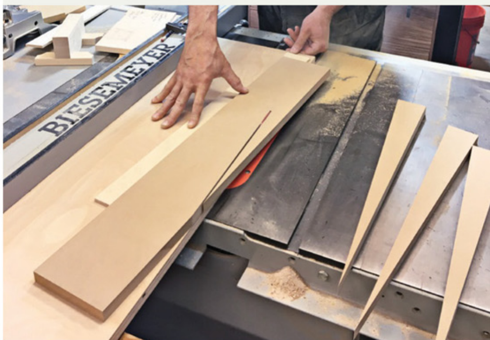
A sled with two cleats positions the blanks for precise tapering. Learn about making and using a tapering jig at woodmagazine.com/taper .
