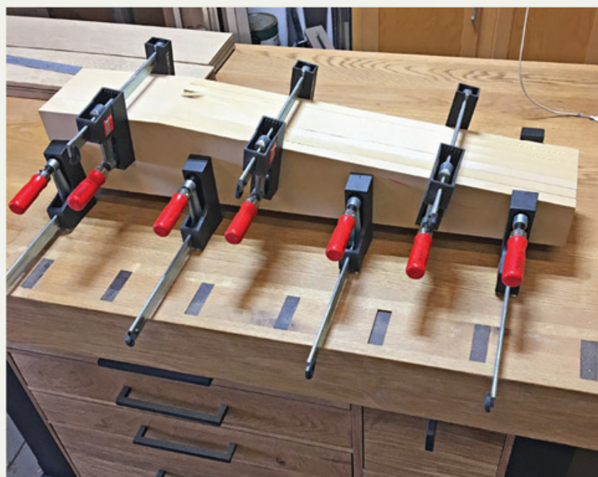
Keep the angled top edges flush as you glue and clamp the form. Brad the layers together as you build up the form to prevent slipping when clamped.
