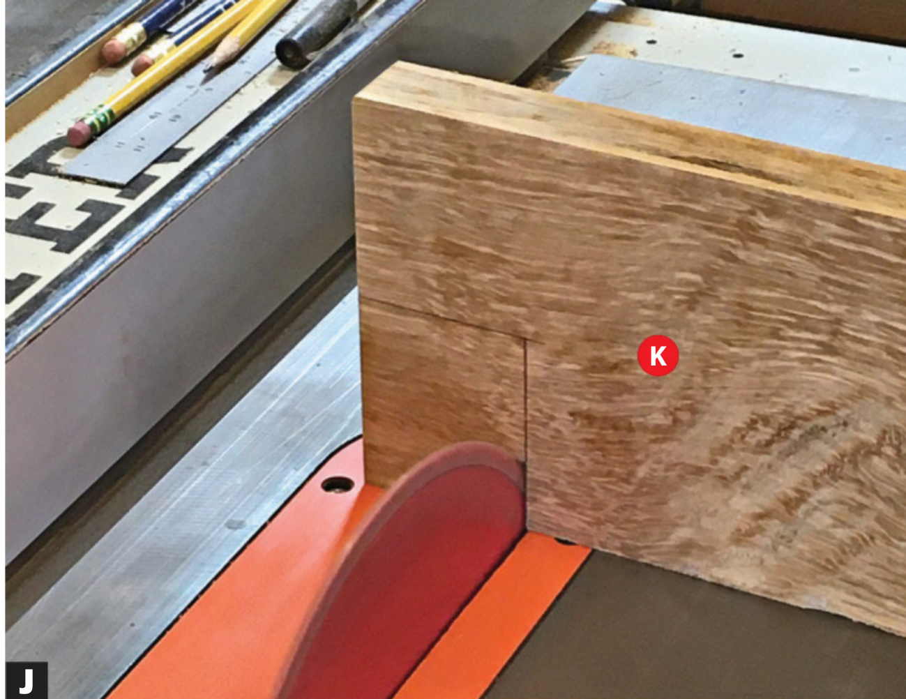
J Raise the tablesaw blade to 2 1/4" and cut the front of the arm notch with the miter gauge adjusted to the correct angle for each arm.
