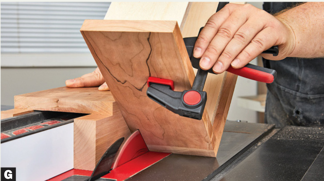
G Clamp the workpiece to the jig before pushing both through the blade to cut the kerfs for the splines.
