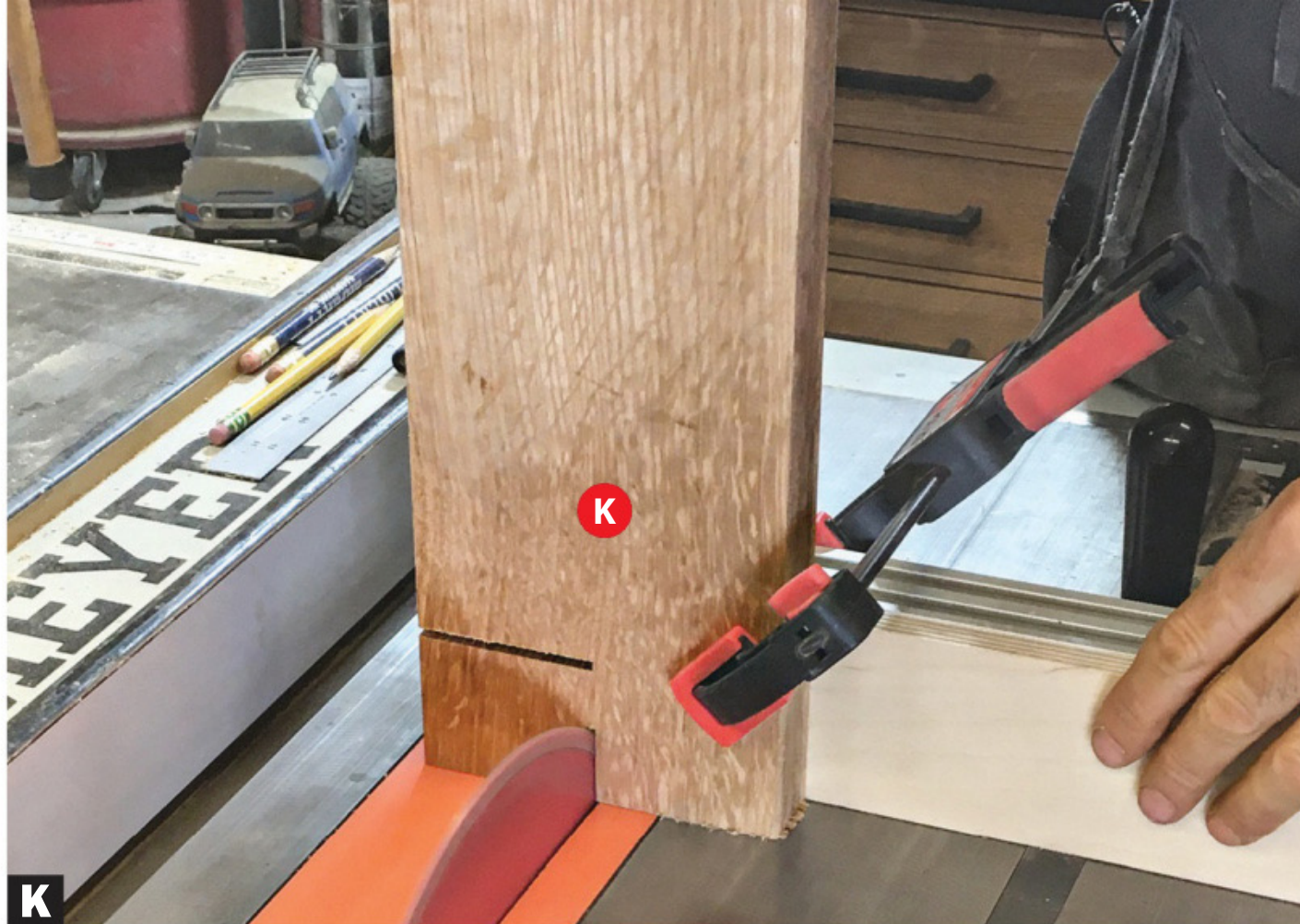
K Set the blade height to the lowest edge of the angle cut and saw the notch. Clamp the arm to the miter-gauge fence for stability. Finish with a handsaw.
