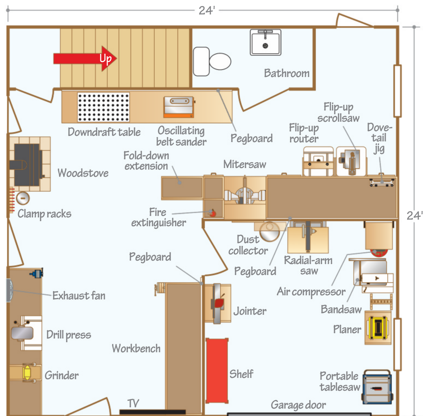
Eric walled off the machines that generate the most noise and dust in a separate area. The garage door eases unloading of lumber and materials.
