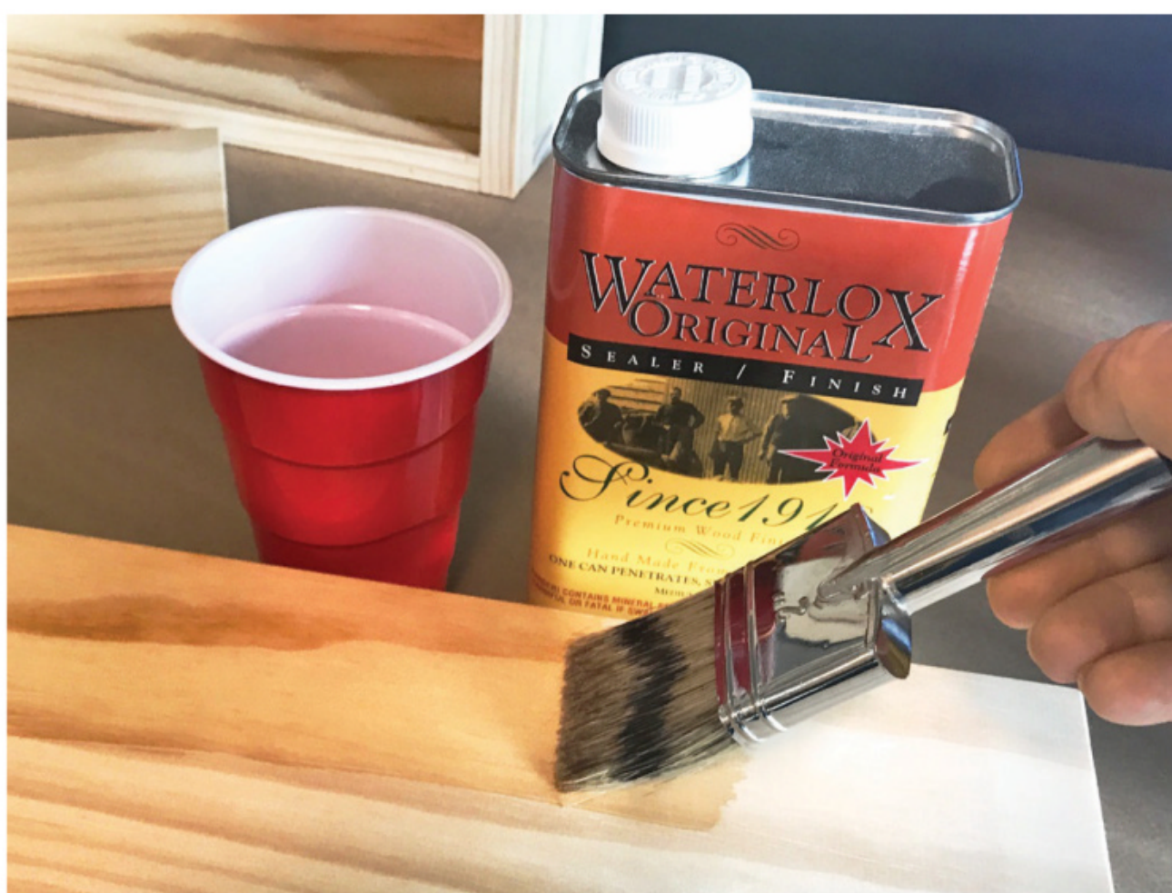
This water-thin coating soaks into the wood while leaving a protective film on the surface. Use a natural bristle brush to lay down a smooth finish.
