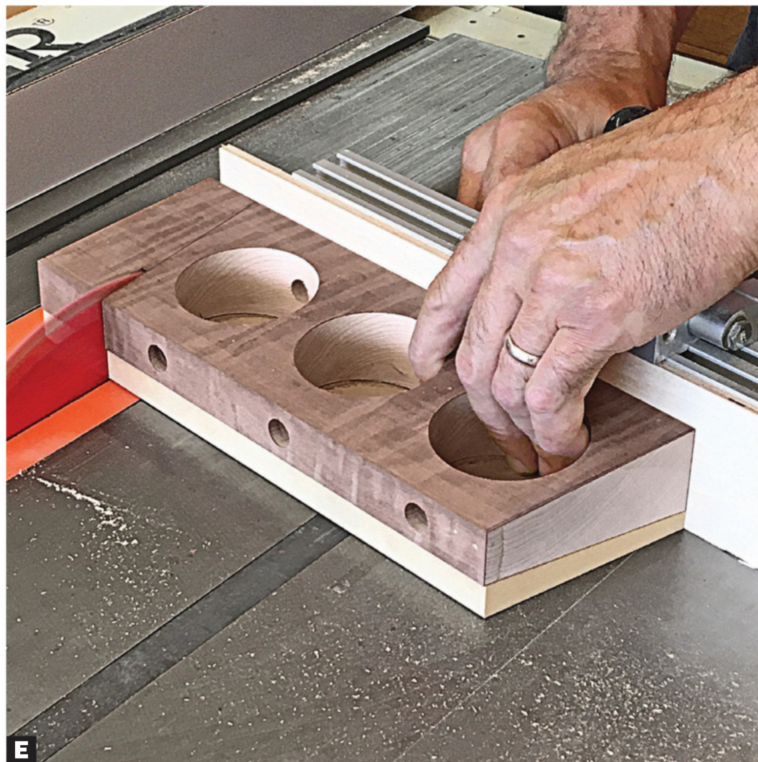
E With the caul resting on the table, cut an end of the base. Reset the miter gauge for the opposite 8^\circ setting and miter-cut the other end.
