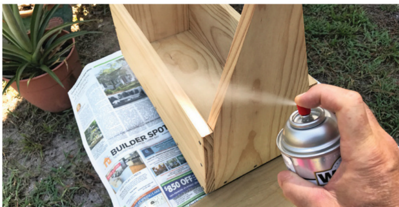
A quick-drying, spray-applied lacquer allows you to build multiple coats quickly.
