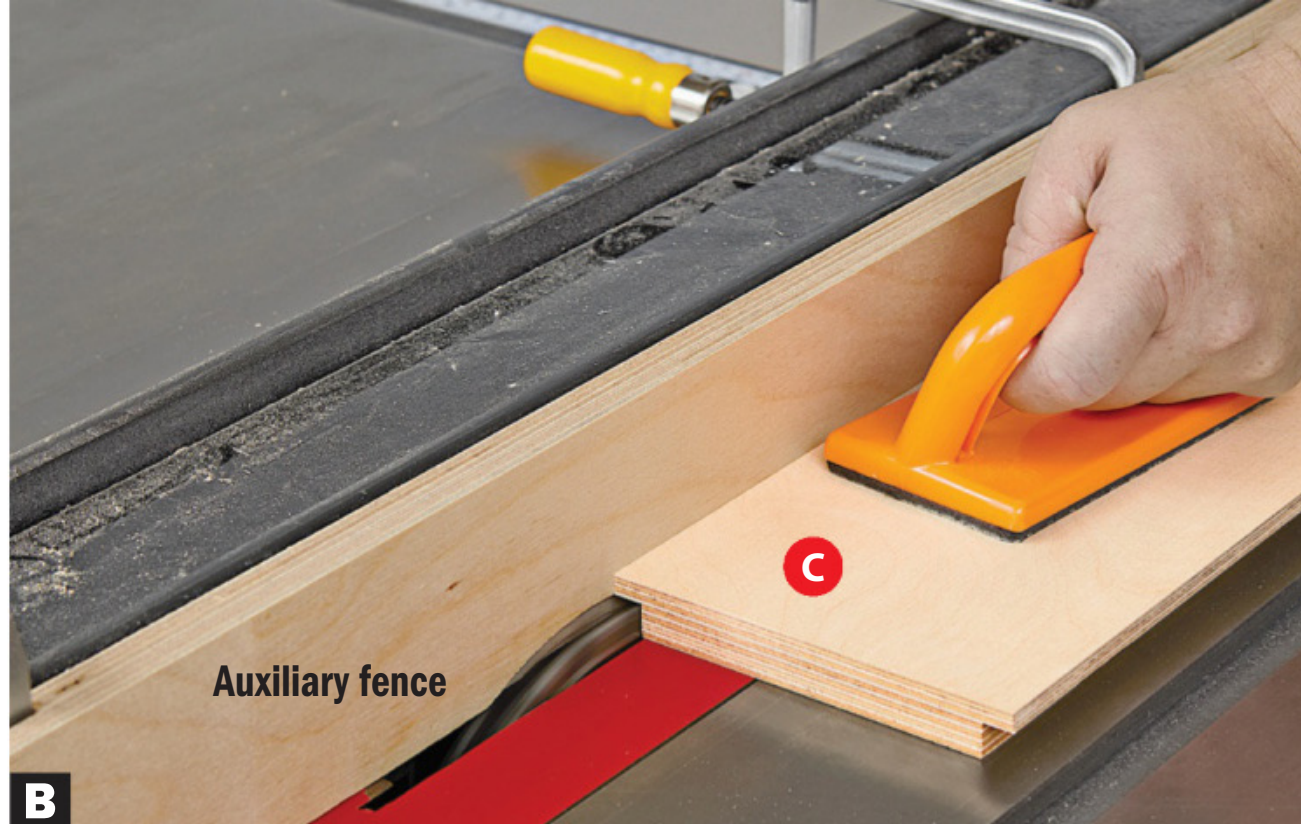
B Cut rabbets along the edges of the riser sides (C) to create tongues that fit the grooves in the riser top and bottom (A, B).
