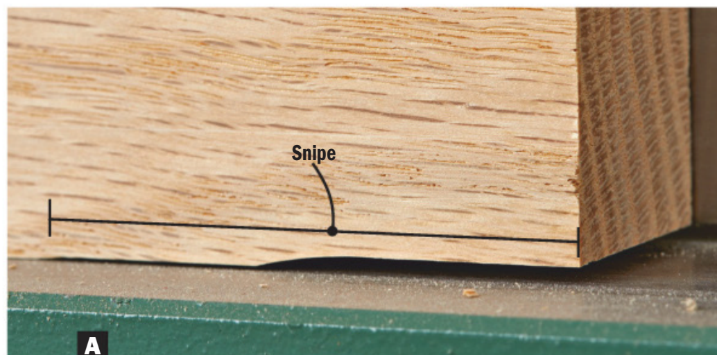
A Snipe happens when the board drops off the infeed table onto a too-low outfeed table at the end of a pass. Raising the outfeed table eliminates this problem.
