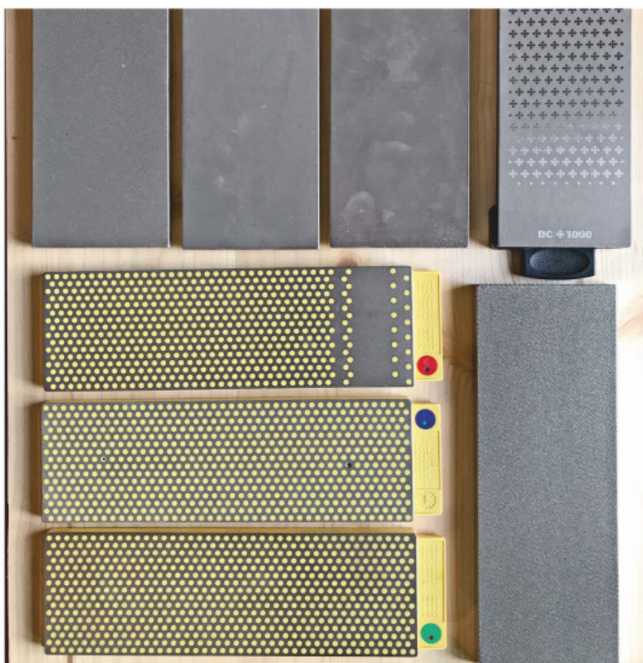
Diamond sharpening stones are available in a variety of styles. Holes or patterns in the surface hold swarf away from the abrasive for faster sharpening.
