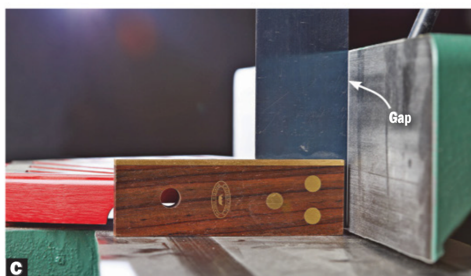
C Light showing between the square blade and the fence indicates the fence doesn't rest exactly 90° to the table.
