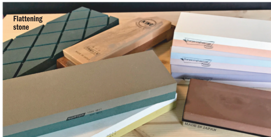
Waterstones come in single- and dual-grit types. Use a flattening stone (top left) between sharpenings to ensure that the surface of the waterstone remains flat.
