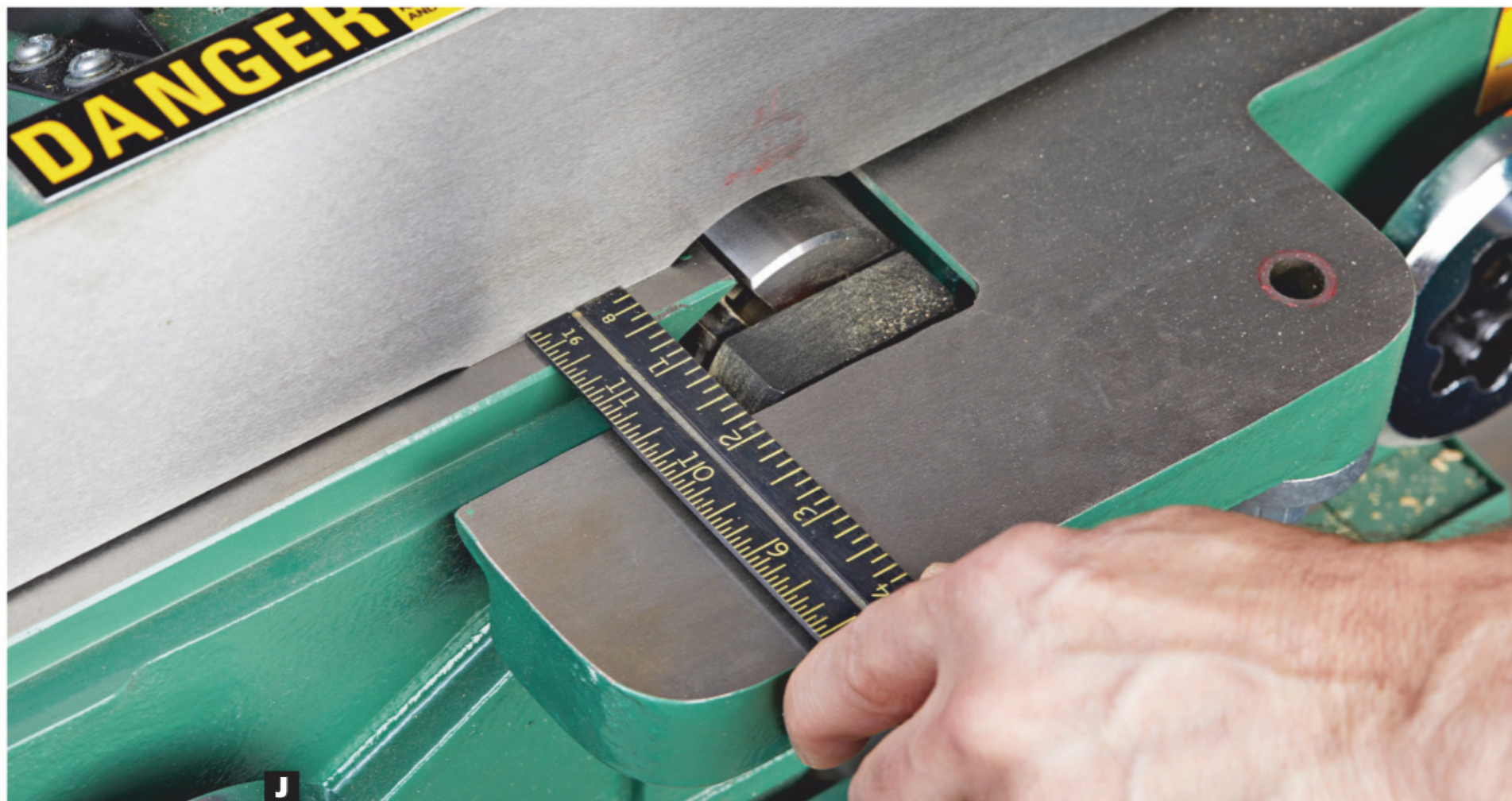
H Tilting the fence toward the tables captures the workpiece, providing better cuts. The jointer helps you create a chamfer cleaner than any made with a tablesaw.
