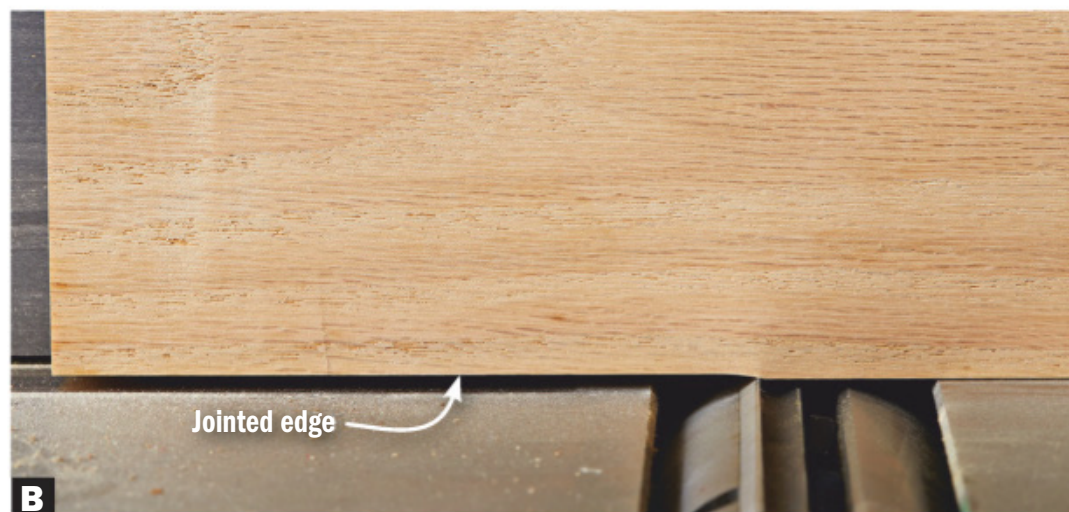
B When raising the outfeed table , be careful not to lift the test piece from the infeed table. You may have to repeat this adjustment to set the table perfectly.
