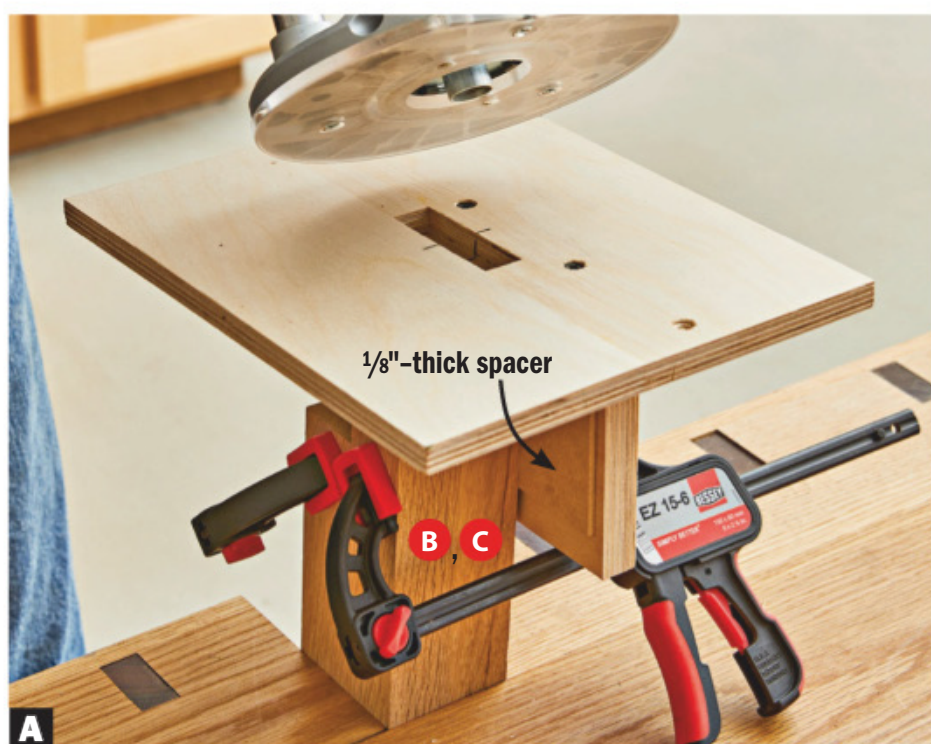
A When routing mortises in the rails (B, C), place a \frac{1}{8} "-thick spacer between the jig fence and rail. Rout mortises in the legs without the spacer.
