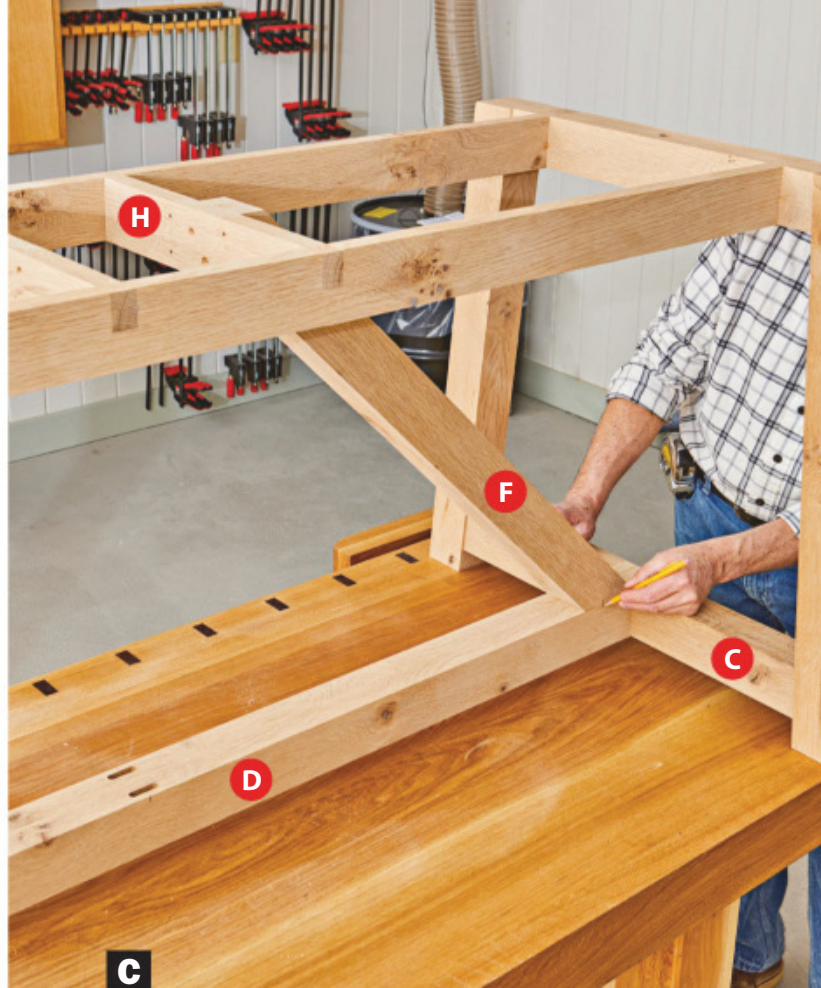
C Place a brace (F) on the lower stretcher (D) and against the brace rail (H). Align the end of the brace with the inside edge of the lower end rail (C). Mark the mortise location on the brace.
