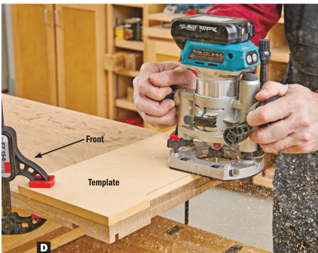
D Take several shallow passes to pattern-route the side bottom profile. Lighter cuts ensure a cleaner edge and minimize the risk of burning.
