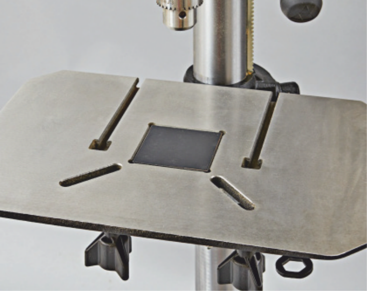
Delta's table ranks best among the test machines, with slots for attaching accessories, easy clamping along its perimeter, and a replaceable insert.
