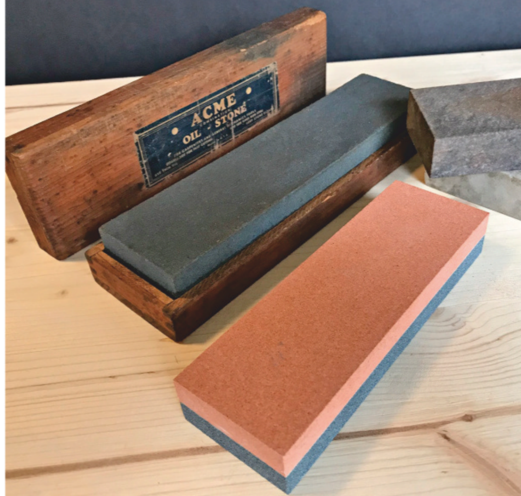
Natural oilstones (top) are traditional sharpening media while synthetic versions offer a wider variety of grits, including the dual-sided, dual-grit stone (bottom).
