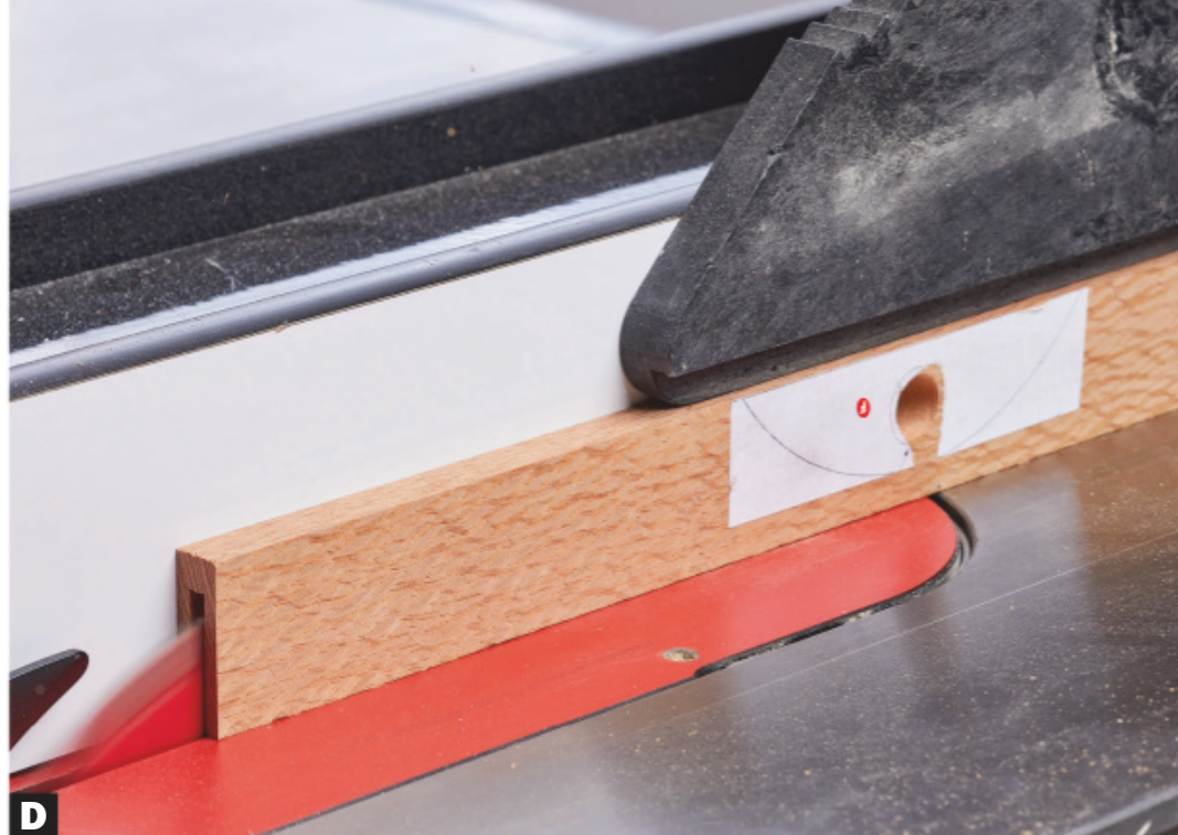
D Make test cuts on scrap to center the blade on the handle blank. Set the blade height so the groove depth extends just above the hole in the blank.
