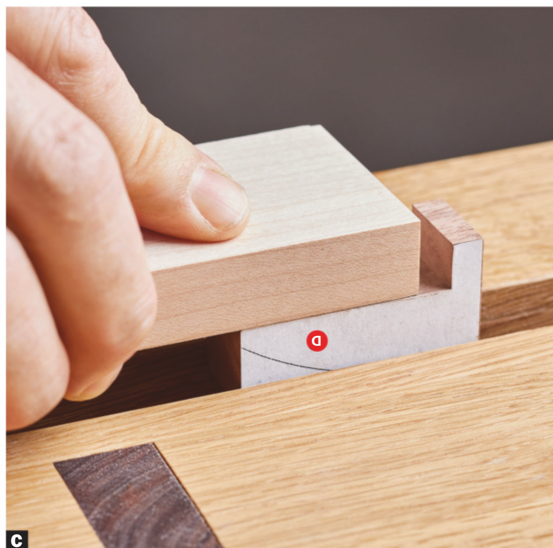
B Cut a birdsmouth notch in a scrap to create a pushstick that moves the foot (D) forward while pressing it against the bandsaw fence.
