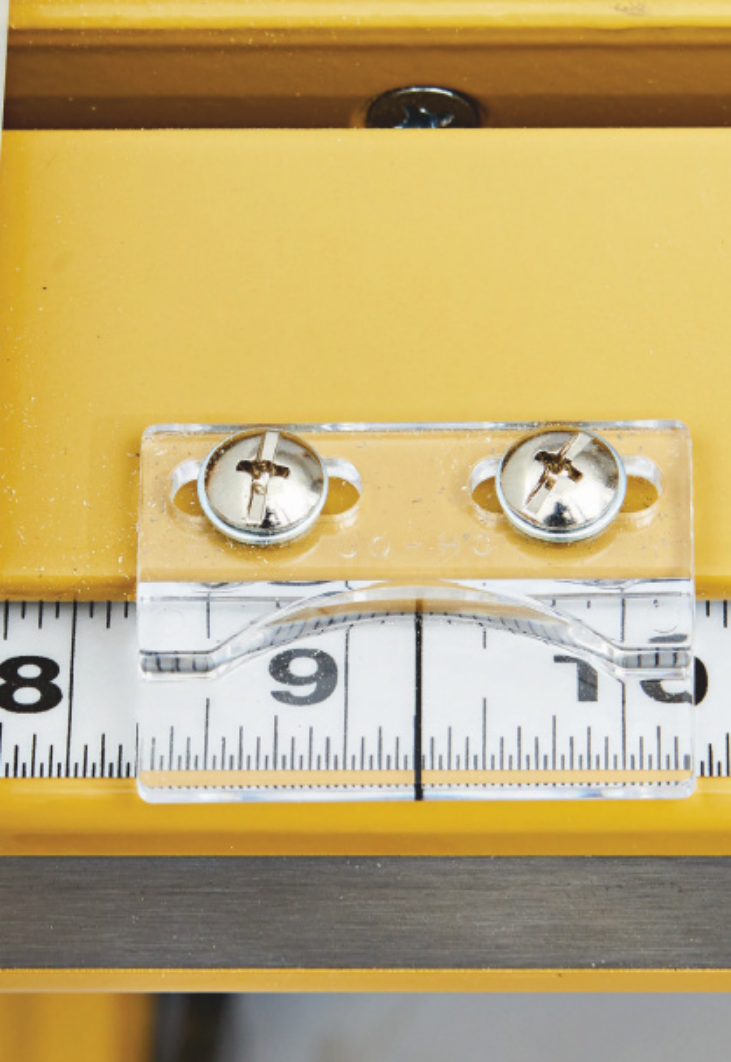
The Powermatic's intuitive increments and wide, clear bezel with hairline cursor make it easy to quickly and accurately set a precise rip width.
