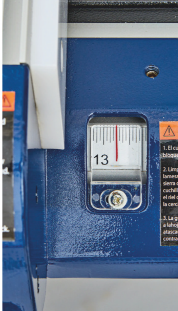
Rikon's rip-fence scale increments are similar in length, making them difficult to distinguish, especially with the narrow view window and thick cursor.
