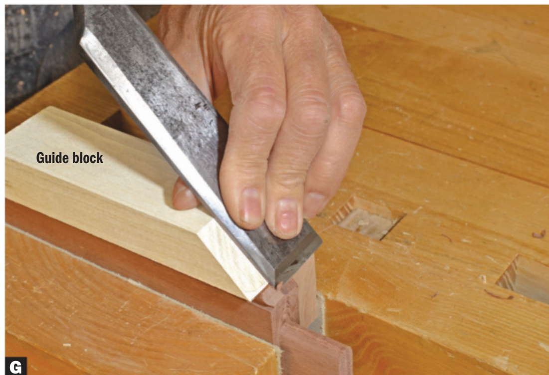
F A vise will suffice for paring work. When necessary, clamp a guide block to the workpiece to ensure accurate chisel placement. Hold the chisel tight to the block.
