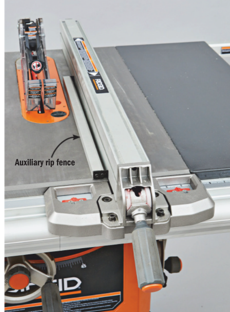
Ridgid's auxiliary rip fence can be positioned on either side, allowing you to get better support under the blade guard on narrow and thin rips.
