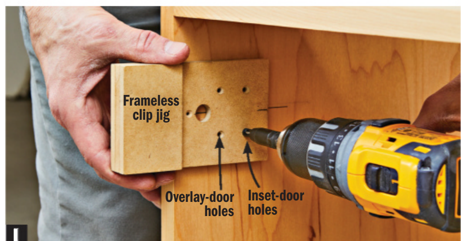
I For frameless cabinets, use the far set of holes for an inset door, the near set for overlay doors.
