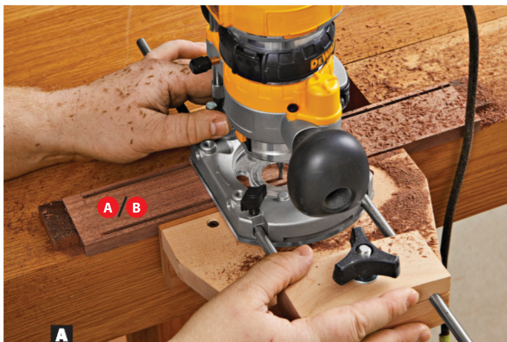
A Secure the blank between bench dogs. Mount an edge guide to your router and cut the grooves.
