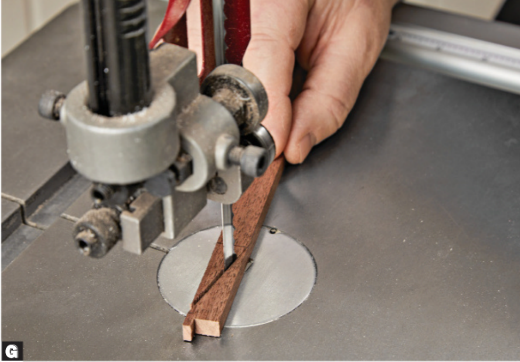
Notch the end of a 6"-long blank to make a tongue that fits the grooves in the box front (C). Then bandsaw the angle.
