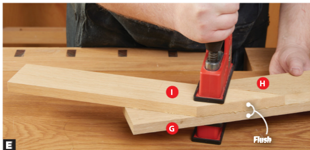
E The square end of the outer side (G) extends past the inner side (H) and the inner headrest (I). Make the end of I flush with the edge of G.
