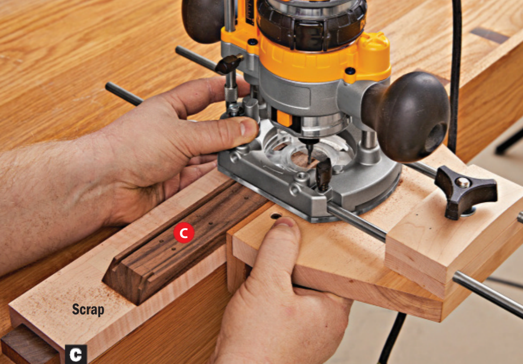
C Secure the box front (C) to a scrap with double-faced tape and clamp the scrap to your bench. Rout the latch grooves.
