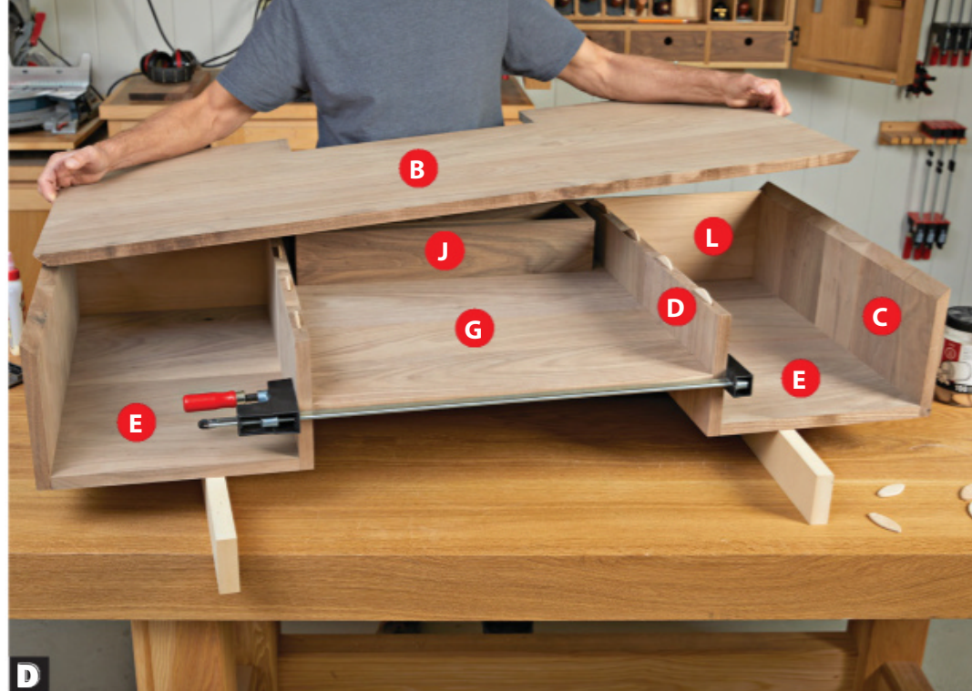
D Insert biscuits without glue for the dry assembly. Capture the case backs in the grooves and make sure the front surfaces are flush and the miters are tight.
