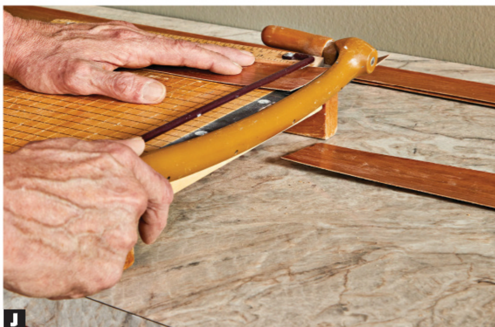
J From the 96"-long strips, crosscut lengths for each stile.
