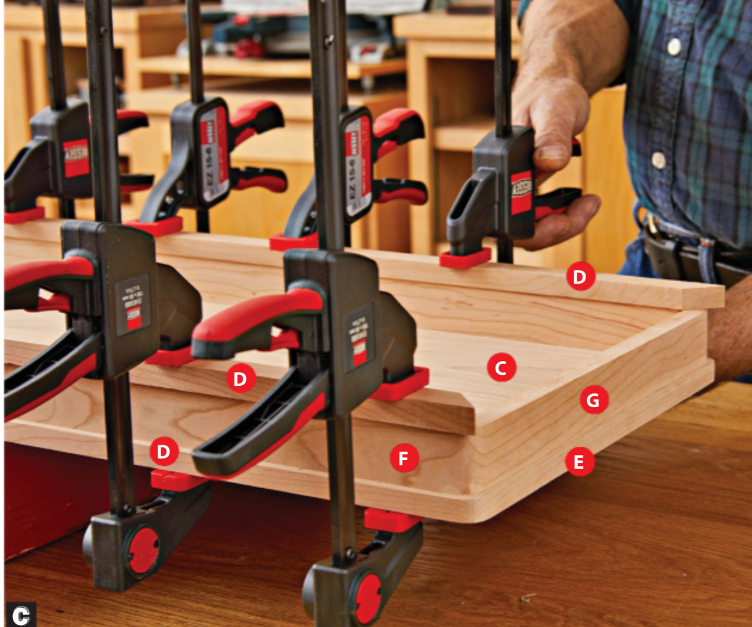
Overhang the side trim (D) on the gutter (F), \frac{1}{16} " on the inside. Line up the miters of the trim and gutter.
