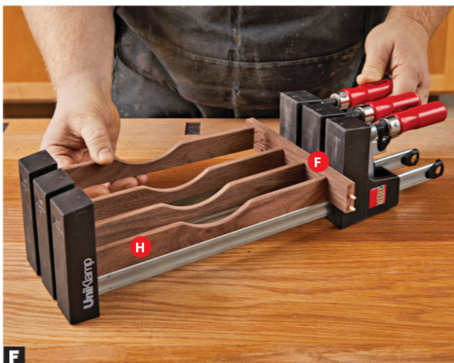
F Glue each chisel divider (H) to the mid divider (F). This assembly floats above the box panel (G), providing additional strength to the box.
