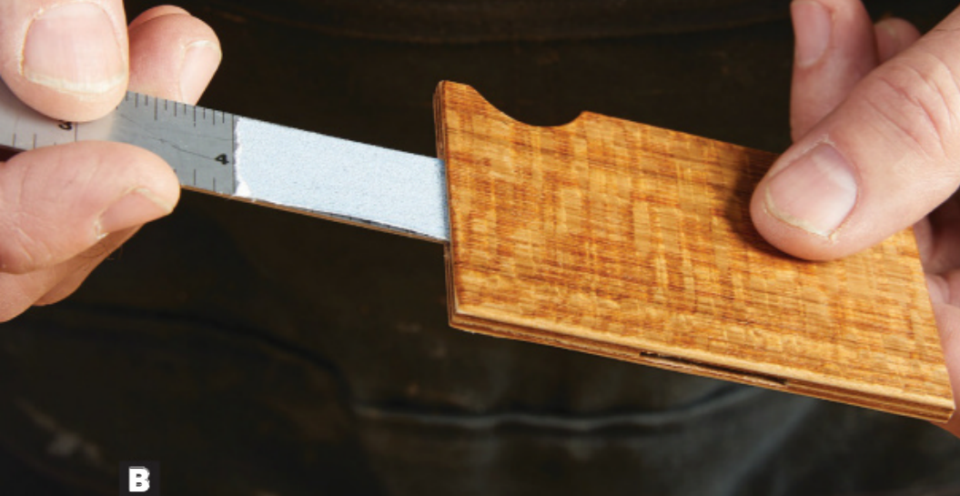
Sandpaper taped to a metal ruler lets you enlarge slots in the laminations until the elastic band easily slides into place.
