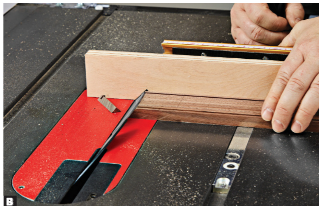
B Attach an auxiliary fence to your miter gauge, and tilt your tablesaw blade to 45°. Make a pass through the fence to help you align the workpieces.
