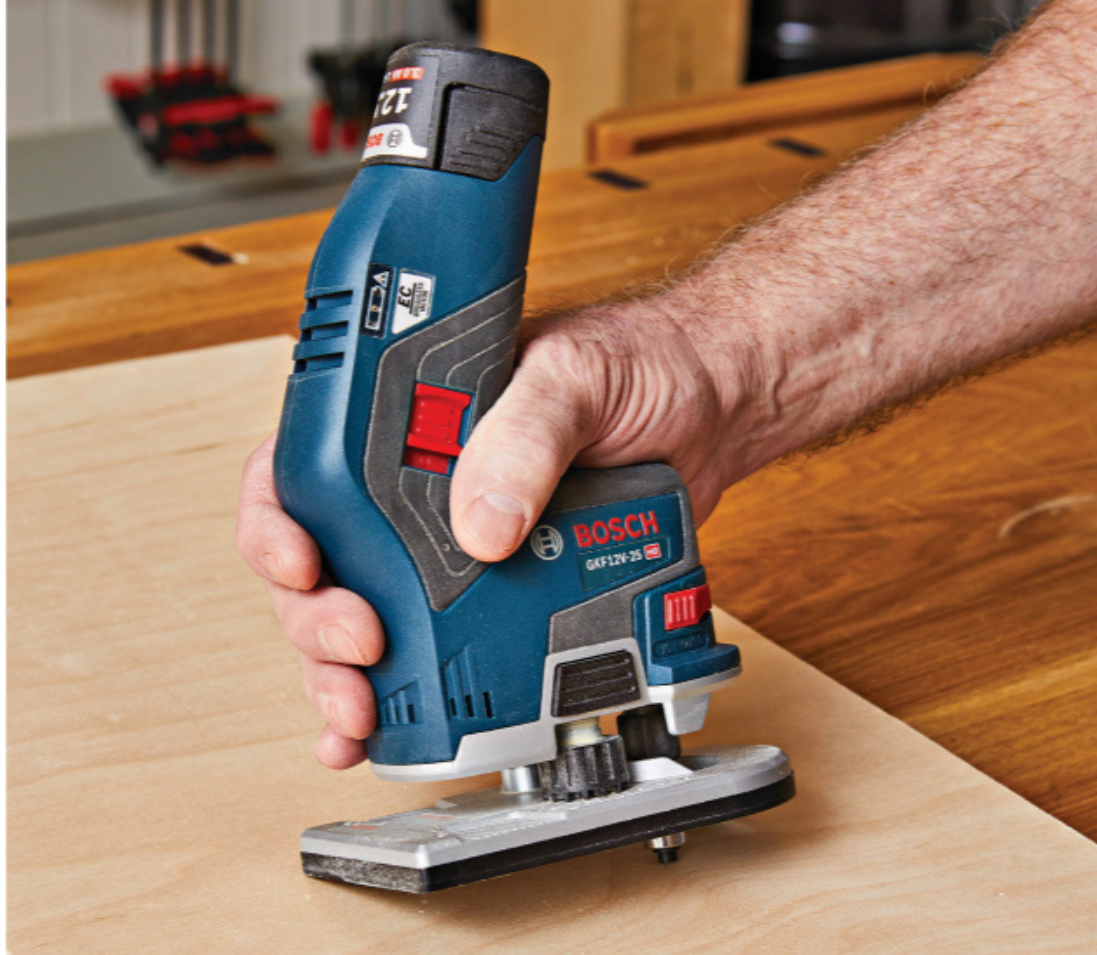
The Bosch 12-volt router has an offset design , with the battery (on top) angling away from the spindle (far right). This unusual shape makes it awkward to grip.
