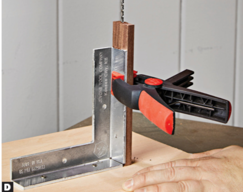
D To steady the divider as you drill, clamp it to a square screwed or clamped to your drill-press table.
