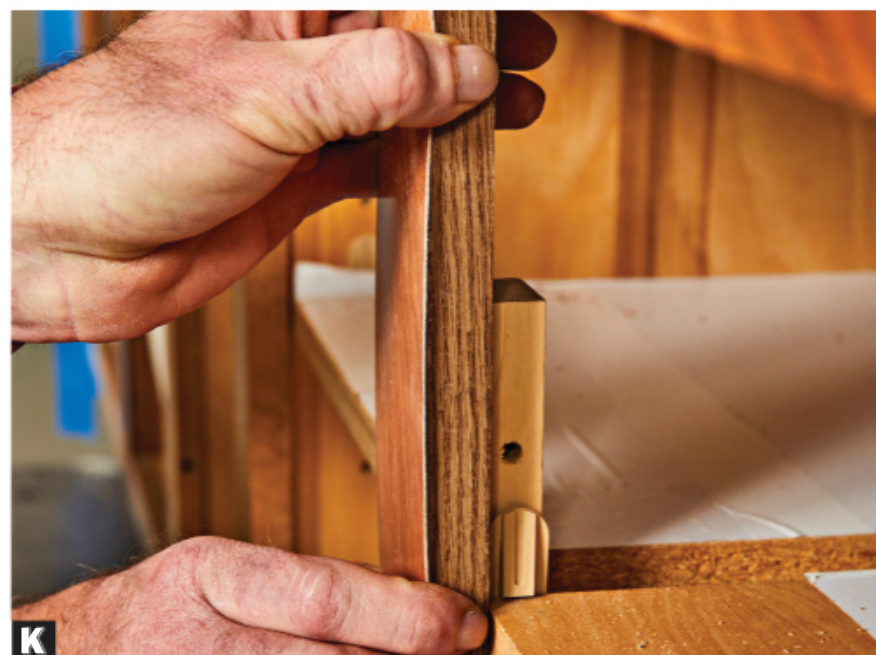
K Use your fingertips to gauge when the veneer is centered on the stile, then lightly press it in place, working from one end to the other.
