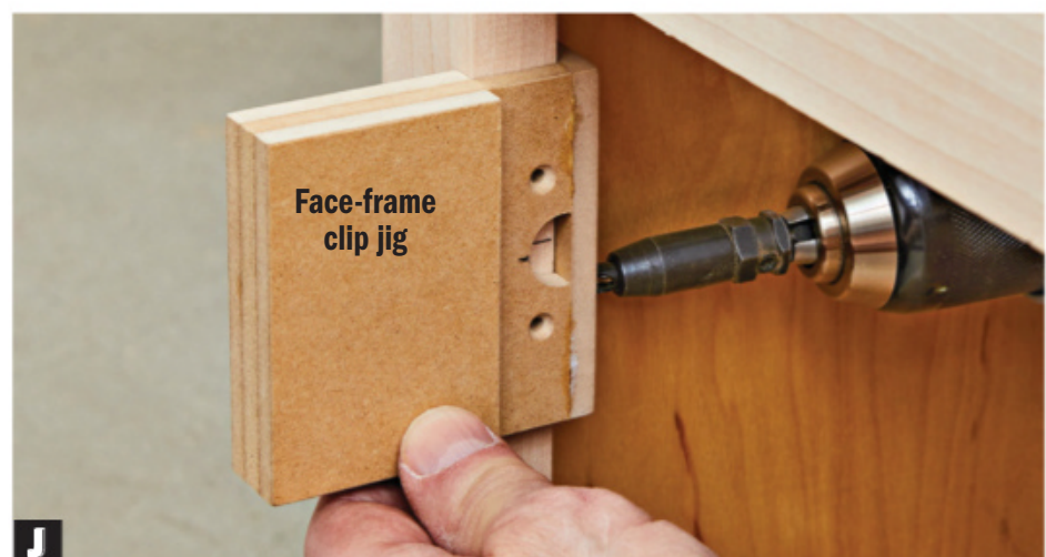
J On face-frame cabinets, drill holes on the edge of the stile for overlay doors, and on the rear face of the stile for inset doors.
