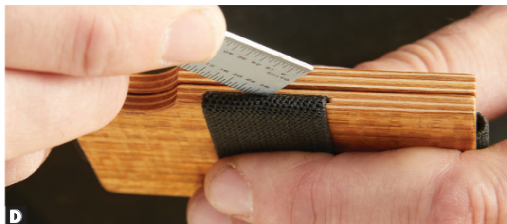
The outside elastic band will be stretched when gluing the final end. Use a metal ruler to push the band into the slot, then hold the band in place while the adhesive dries.
