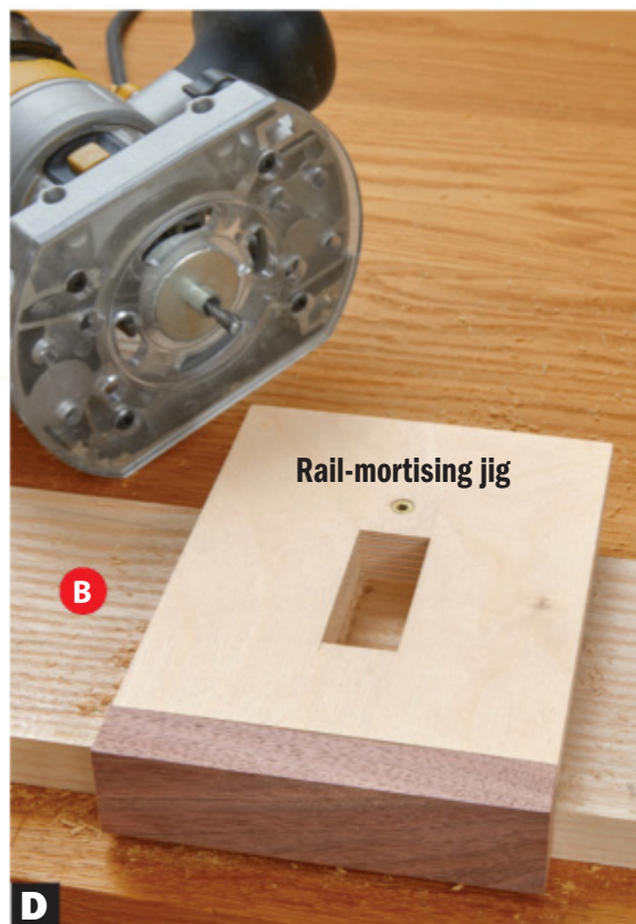
D The rail-mortising jig screws to the rail. Later, you'll cut away the screw holes while forming the curves.
