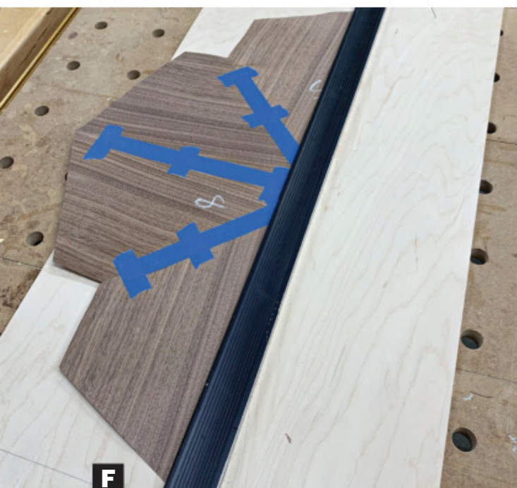
D Attach 120-grit sandpaper to a straight scrap. With the mating edges of two veneer wedges overhanging a scrap of plywood, press the veneer in place with the MDF wedge, and gently sand a straight edge.
