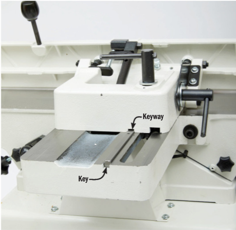
A fence using a keyway slide requires a little more effort to move, but also less space behind the machine.
