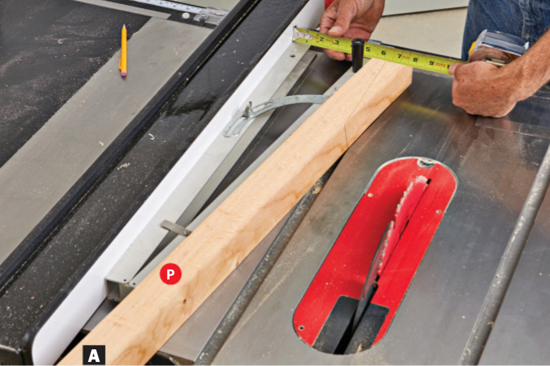
A Adjust the angle of a taper jig to align the taper line drawn on the leg parallel to the rip fence.
