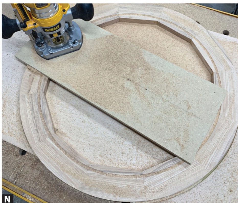
N Rout through the border in consecutively deeper passes, just as you did with the field.
