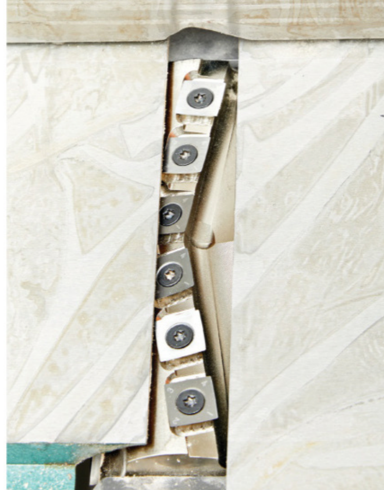
The carbide-insert cutterhead on Grizzly's G0814X uses a V-shaped pattern for the inserts (the only one in our test). It did not cut as cleanly as most others.
