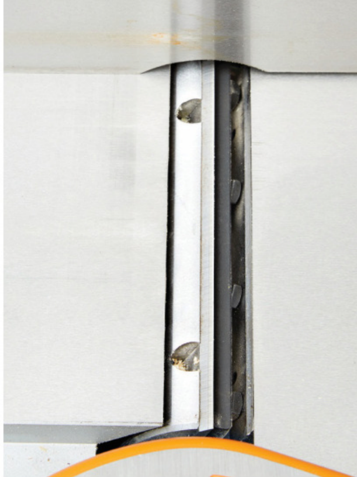
Ridgid's straight-knife cutterhead cuts very well when sharp. As the knives dull, you must remove and sharpen (or replace) them.
