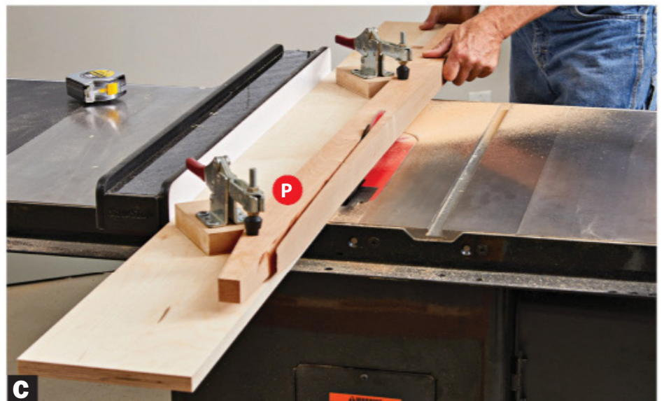
C Cut the long taper with the leg against the lower and middle blocks, and the upper end in the end-stop notch. Secure the leg with toggle clamps.
