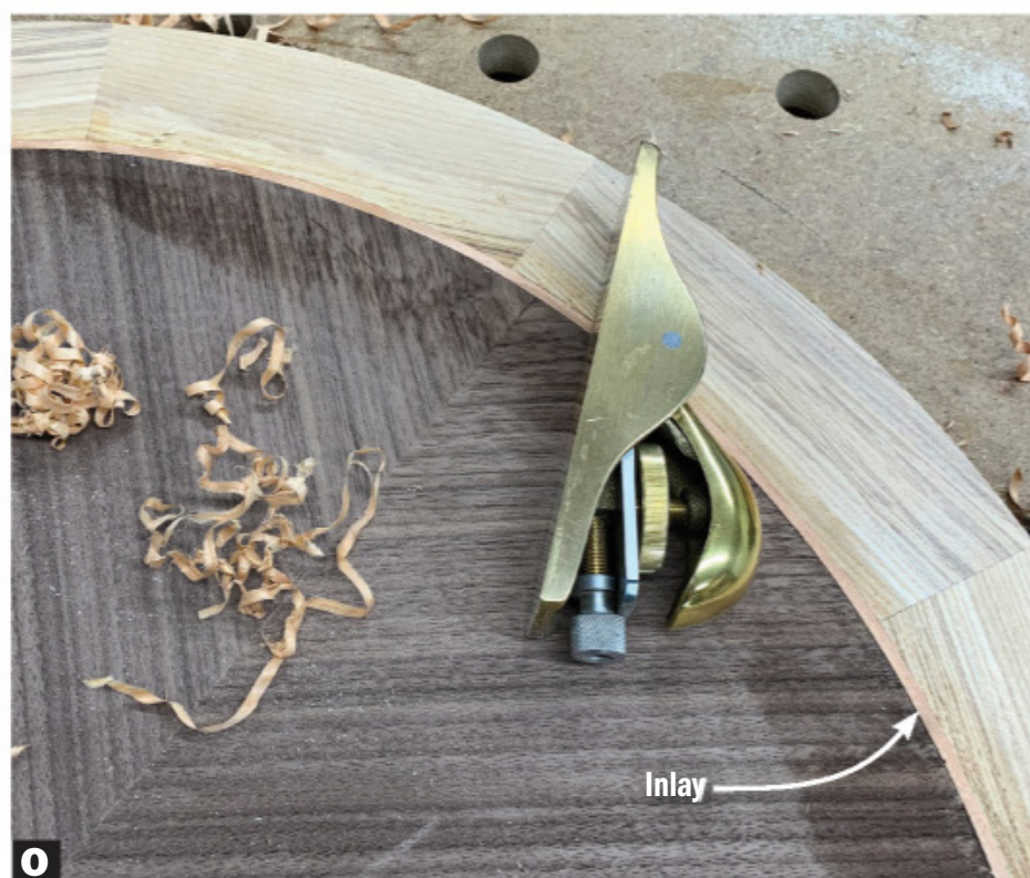
O Plane away most of the inlay, then finish up with a card scraper and sandpaper, being careful to not sand through the veneer.
