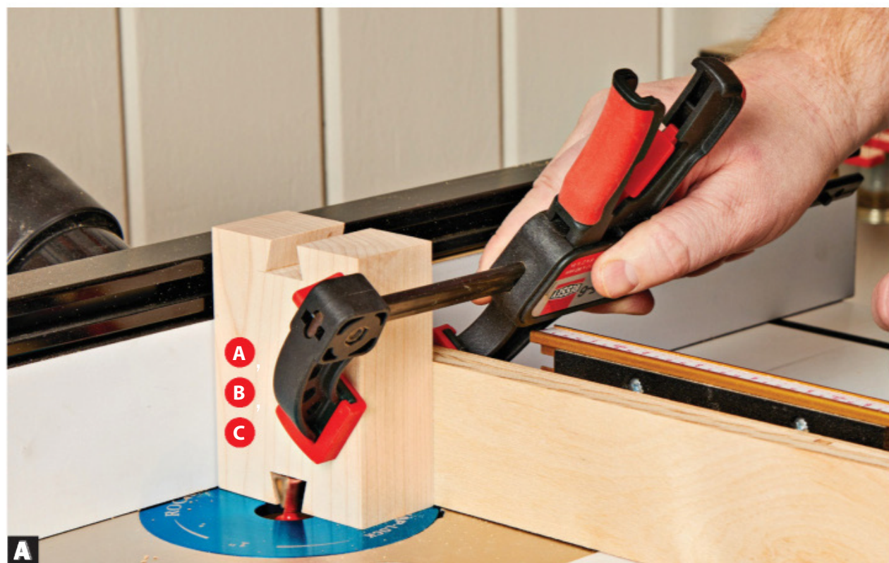
Rout the dovetail grooves using a backing block to prevent tear-out. Make one pass, rotate the workpiece 180°, and make a second pass for a centered cut.
