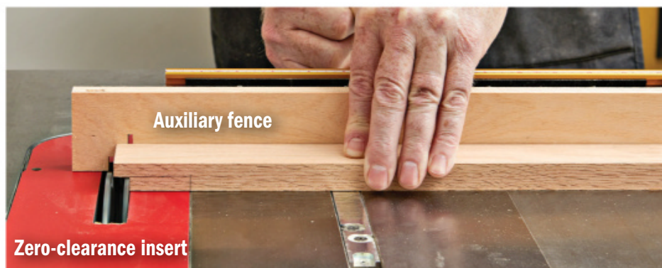
Raise the dado blade to about half the workpiece thickness, and then cut away a short section on one face of each of the mating workpieces.
