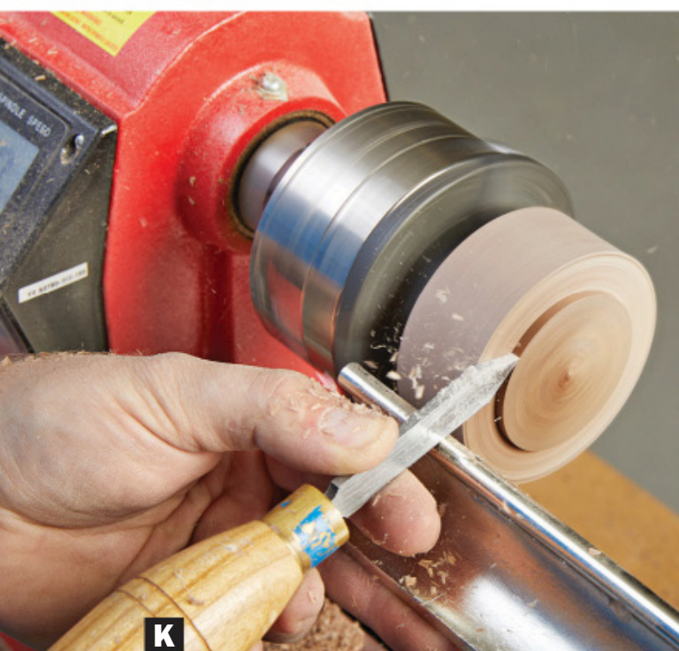
I Use a squarenose scraper to make a 2"-diameter mortise \frac{3}{16} " deep.
