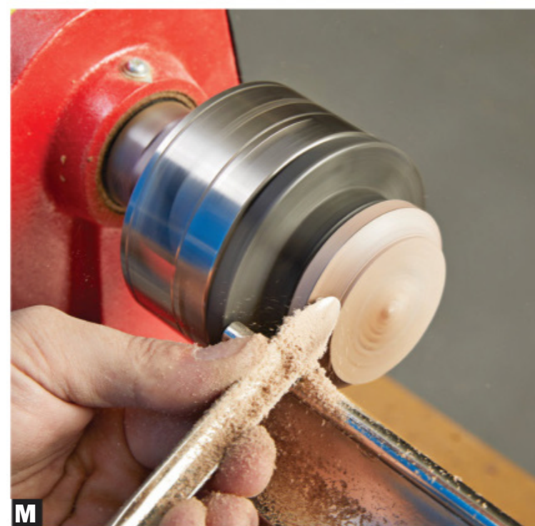
J Press a cone center against the urn to help stabilize the workpiece. Continue shaping the remainder of the sphere.
