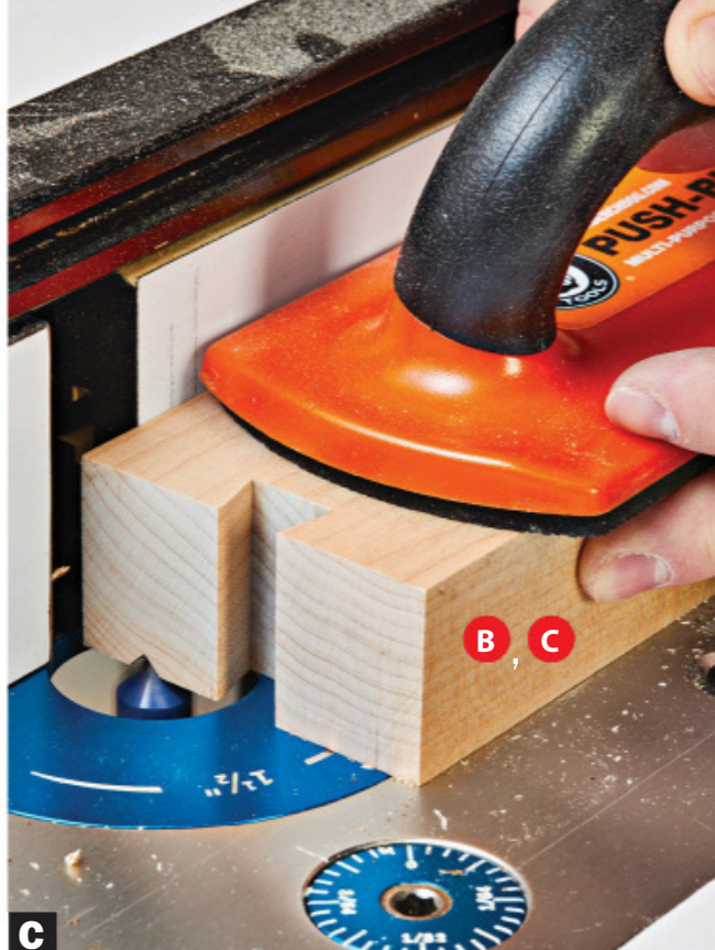
C Rout the horizontal grooves (shown) and vertical grooves in the jaws using a 45° V-grooving bit. Back the cross-grain cuts to prevent tear-out.
