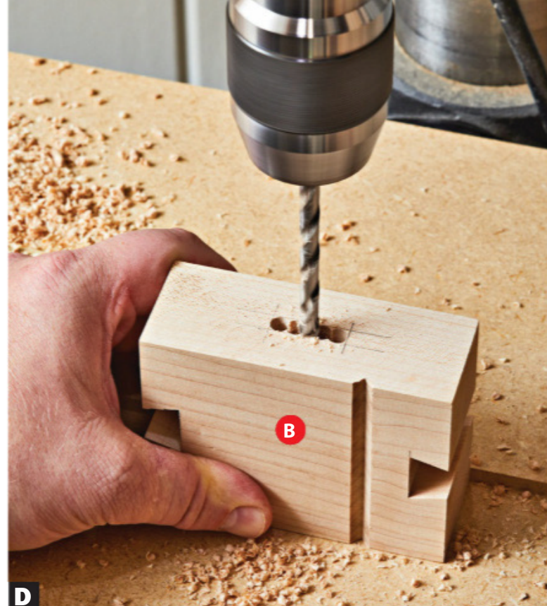
D Use a brad-point drill bit to remove most of the waste for the through mortise in the movable jaw. Drill from both edges to complete the removal.
