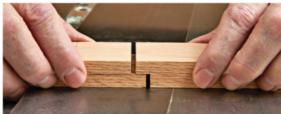
Test the fit , adjust the dado height, if necessary, and repeat until each board is precisely half the thickness (for a perfect fit).
