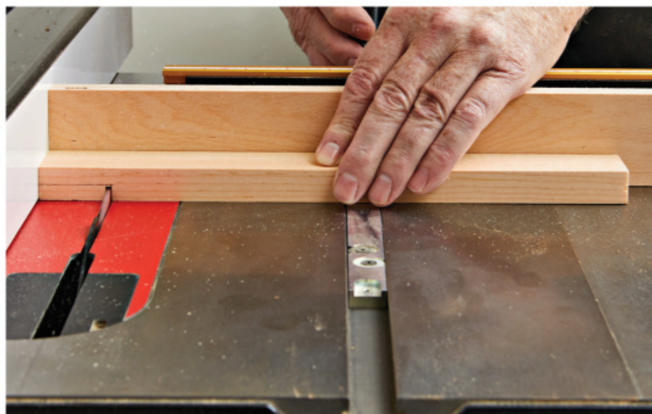
Cut the shoulder first , using the rip fence as a stop.
