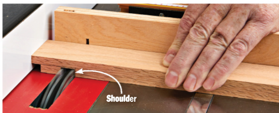
Using the rip fence as a stop , make the shoulder cut. Lift the workpiece, retract the miter gauge, and reposition the workpiece to cut away the remaining material between the two cuts with one or two passes.
