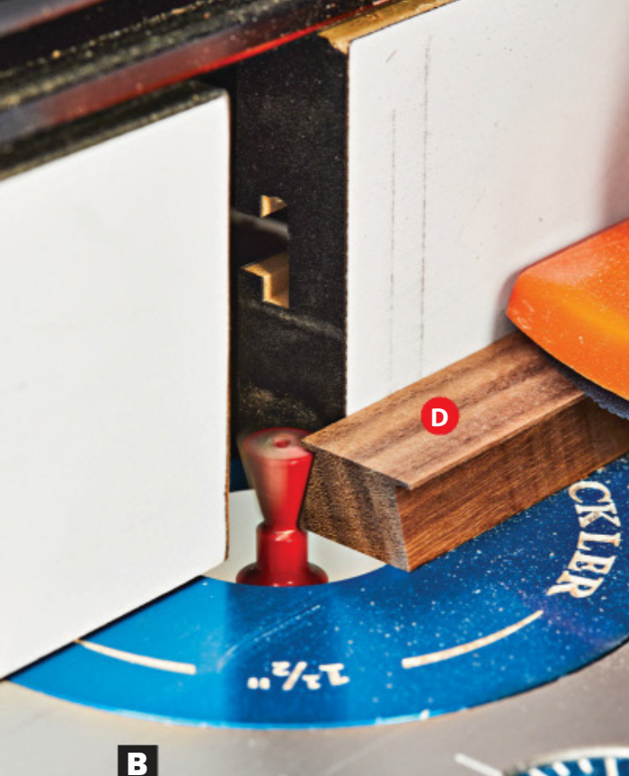
B Rout both edges of the runner blank, leaving a tiny lip that rides along the router-table fence. Sneak up on the final cut to ensure the runners slide snugly in the jaw dovetails.
