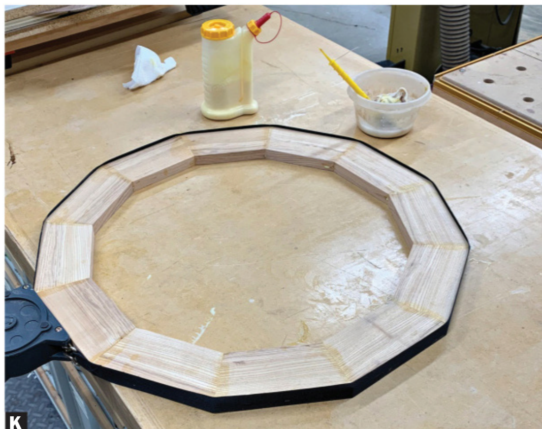
K Dry-fit the segments and check for gaps before gluing up the circle. A band clamp pulls everything together.
