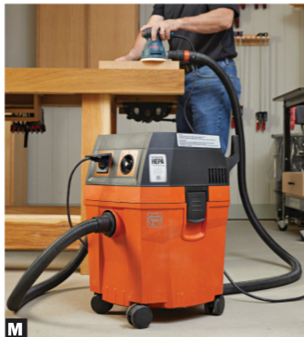
M A dust extractor connected to the port of a random-orbit sander pulls dust through the holes in the sanding pad and traps it.
