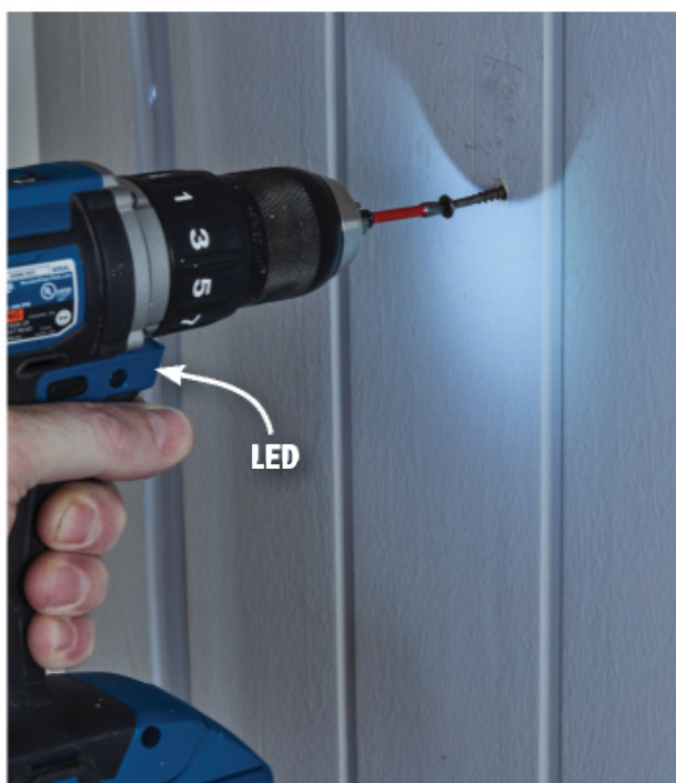
LEDs located beneath the clutch assembly cast a chuck shadow in the work area, sometimes blocking light from exactly where you want it.
