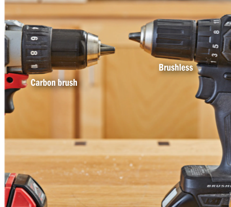
Clutch position determines its ease of use. On models with carbon-brush motors, the clutch ring sits forward of the handle and trigger. But on brushless-motor models, the clutch ring is farther back, where the handle and trigger interfere.
