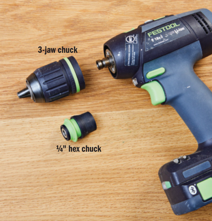
Festool's drill uses a quick-connect system for swapping detachable chucks.
