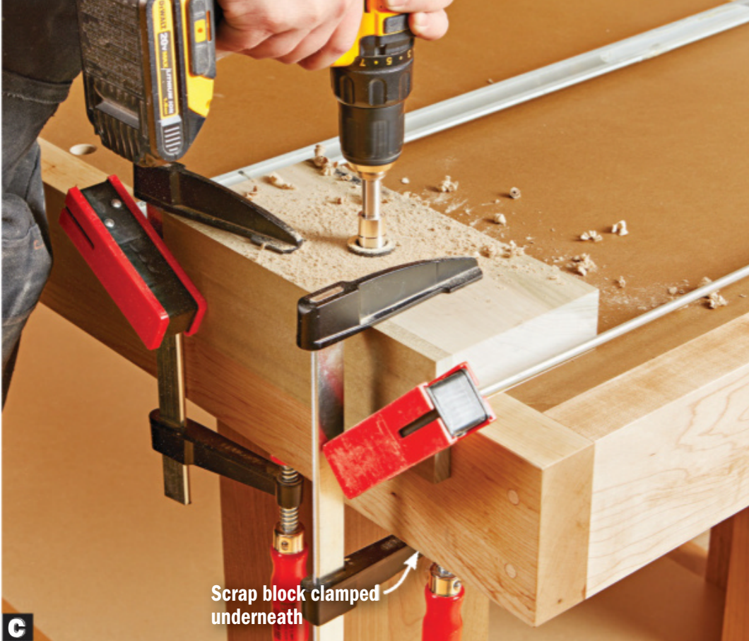
Drill dogholes using the drill guide clamped and aligned with hole centerlines. A scrap block clamped underneath prevents tear-out.
