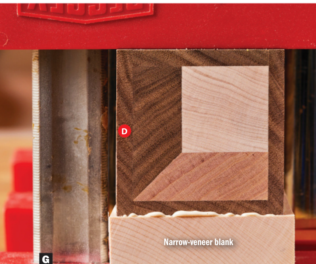
G Glue on the narrow veneer (E) blank with equal overhang on both edges.
