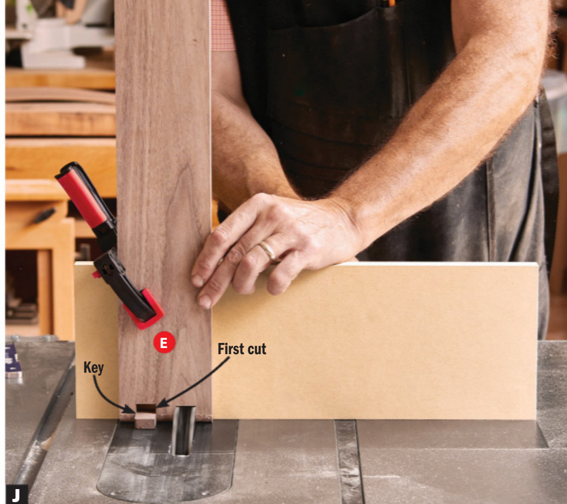
J Fit the notch from the first pass over the index key for the second cut. Saw the other stretcher the same way.
