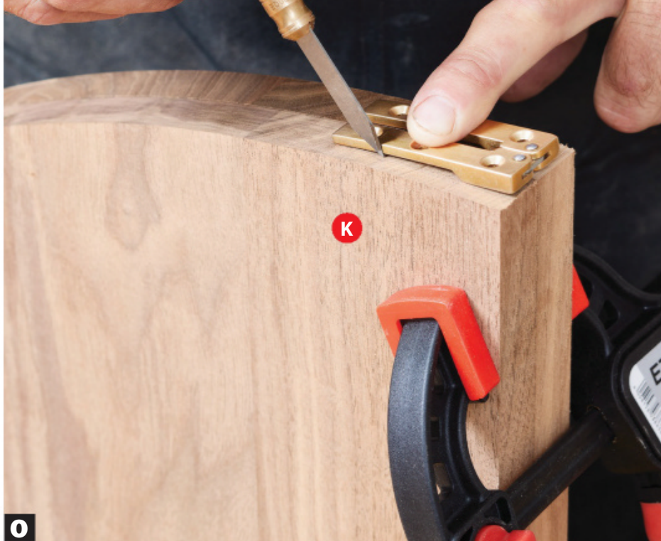
Scribe the hinge locations centered on the edges with a knife or pencil. Rough out the recesses with a trim router and 1/8" bit; fine-tune them with a chisel.
