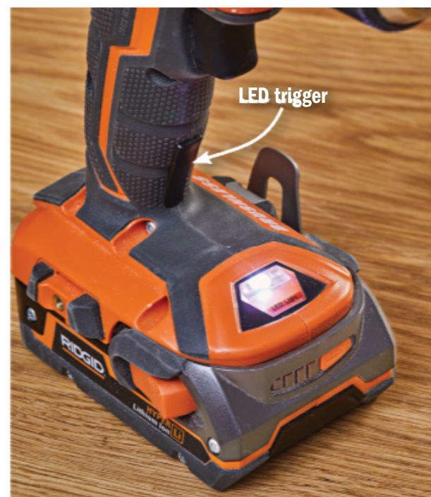
Ridgid's drill has a trigger for the LED that activates when you grip the tool. The LED stays on for 10 seconds after you release the trigger.
