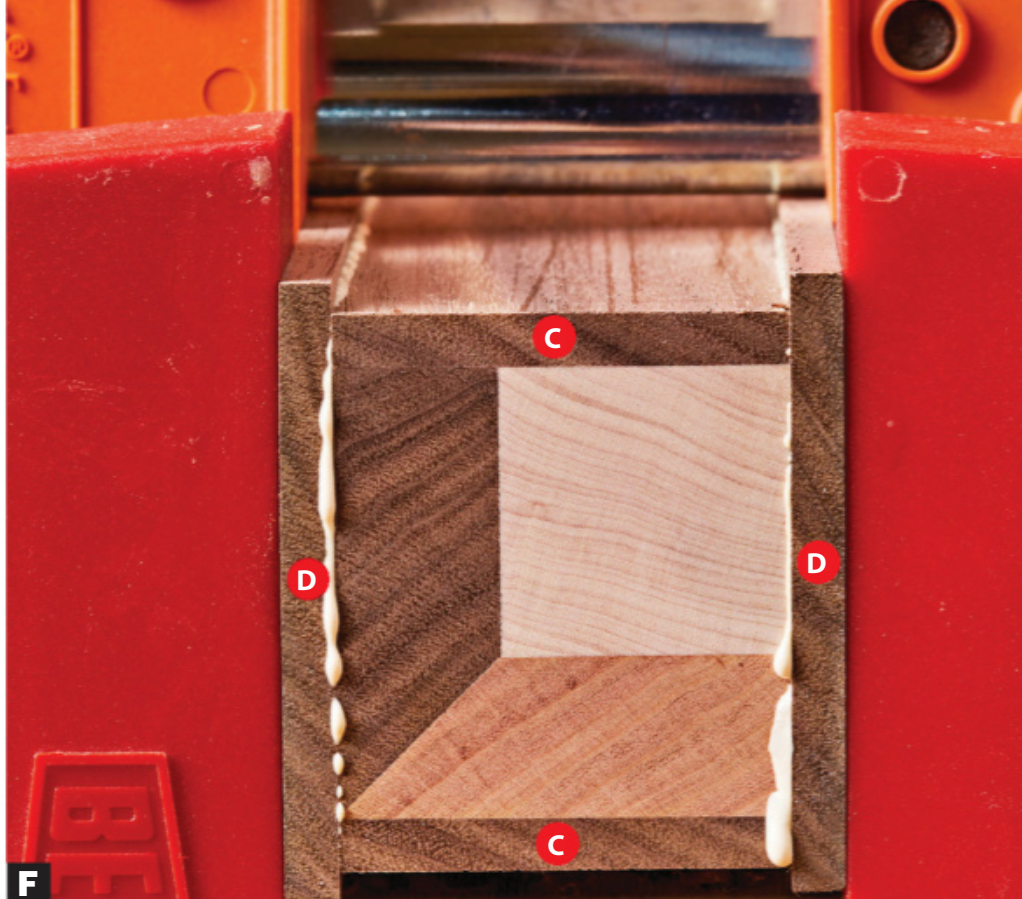
F Glue on the wide edging (D) just as you did the narrow edging (C).
