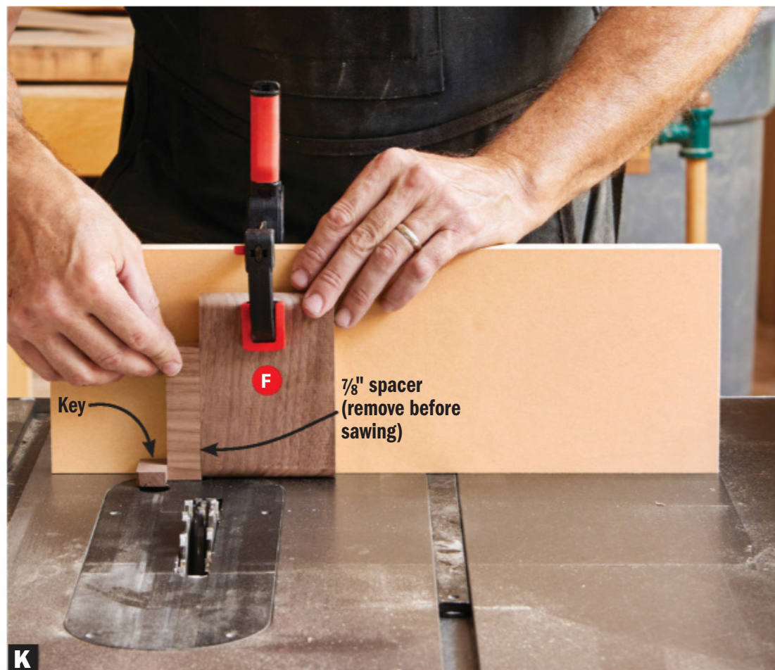
K Space the pivot block (F) \frac{7}{8} " from the key for the first cut. For subsequent cuts on each end, put the notch from the previous pass over the key.
