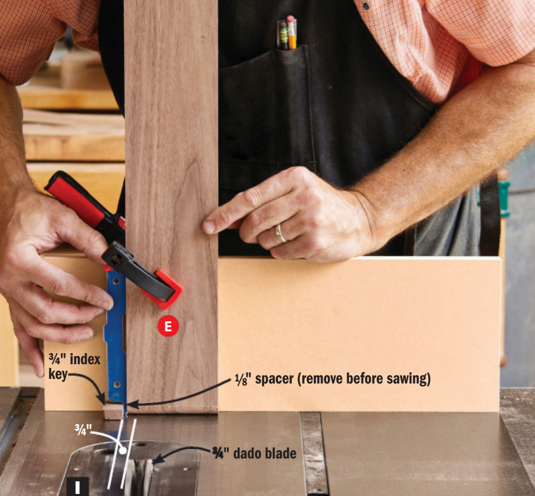
I Insert a \frac{1}{8} " spacer between the stretcher and the index key to make the first pass. Clamp the part to the jig fence for greatest accuracy.
