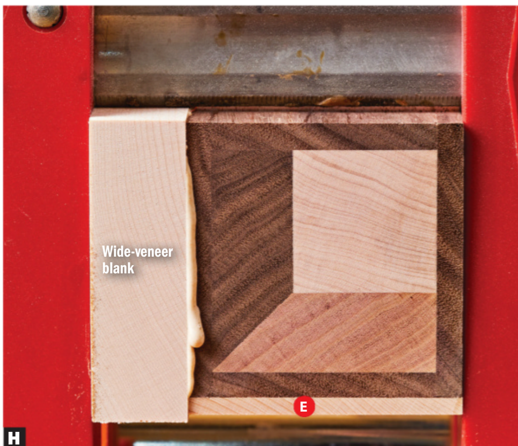
H Glue on the wide veneer (F) blank just as you did the narrow veneer (E) blank, with slight overhang on both edges.
