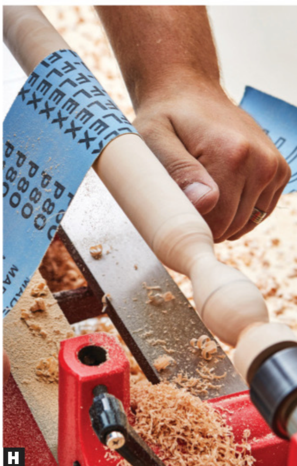
H Sand with cloth-backed abrasive in progressively finer grits from 80 to 220. Run the lathe at a slower speed (750 rpm or so) with coarse abrasive.
