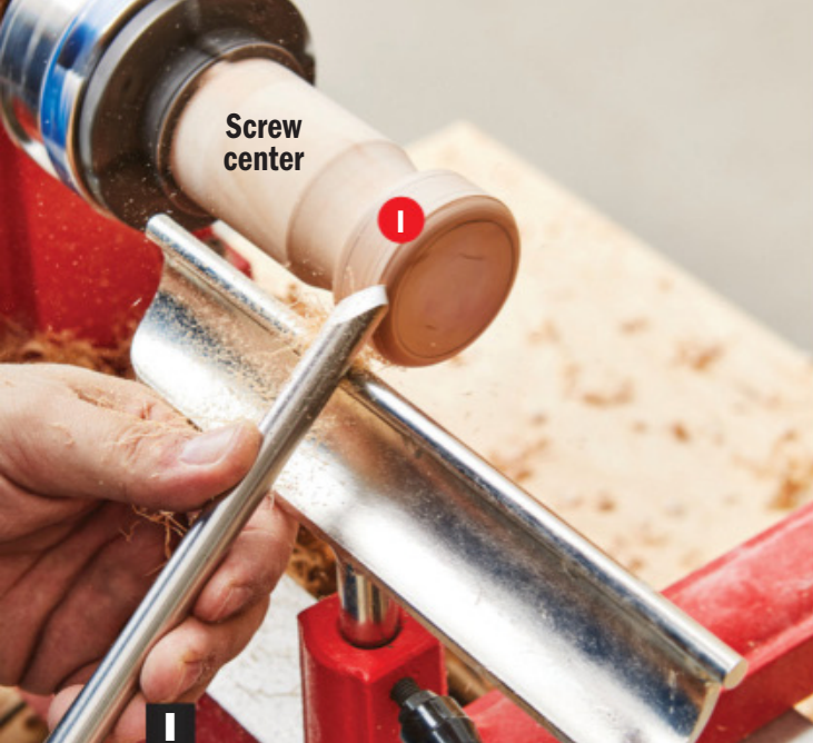
I Turn the arm cap to final diameter and round over the edge. Finish-sand the cap, remove it from the screw center, and drill the center hole to \frac{3}{8} " deep.
