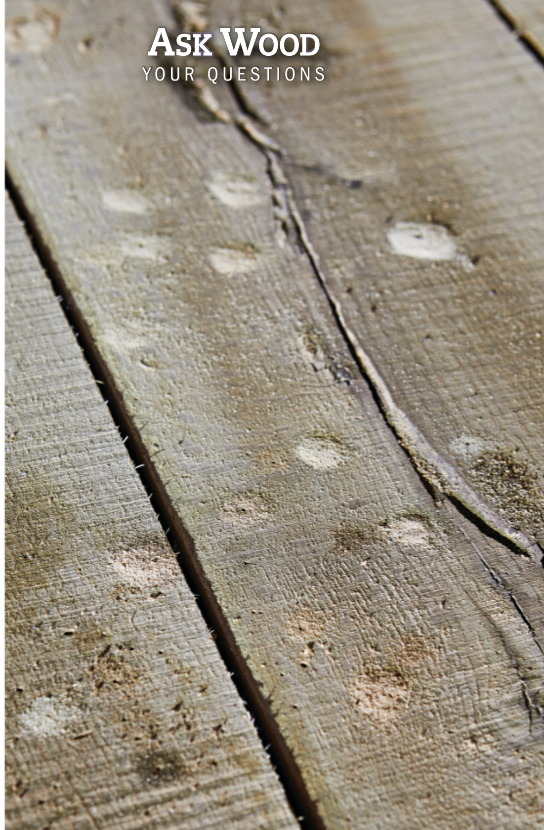
Tiny holes and dust piles indicate the presence of wood-boring insects such as powder-post beetles. Saturating the wood with a borate treatment, such as Tim-bor or Bora-Care, should kill the bugs.
