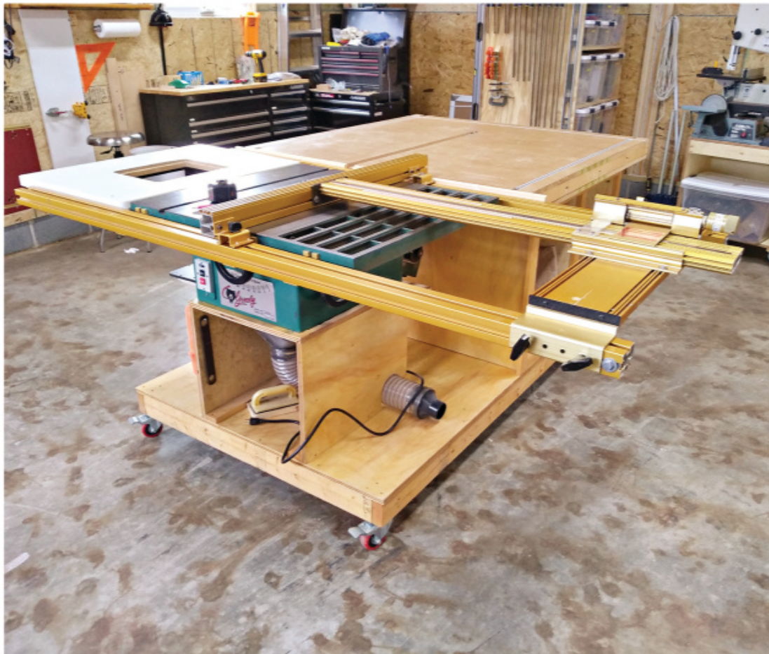
The centerpiece of the shop is this mobile tablesaw and router-table workstation. John designed it for plenty of support for large workpieces and lots of storage. The outfeed table is a torsion box assembly.
