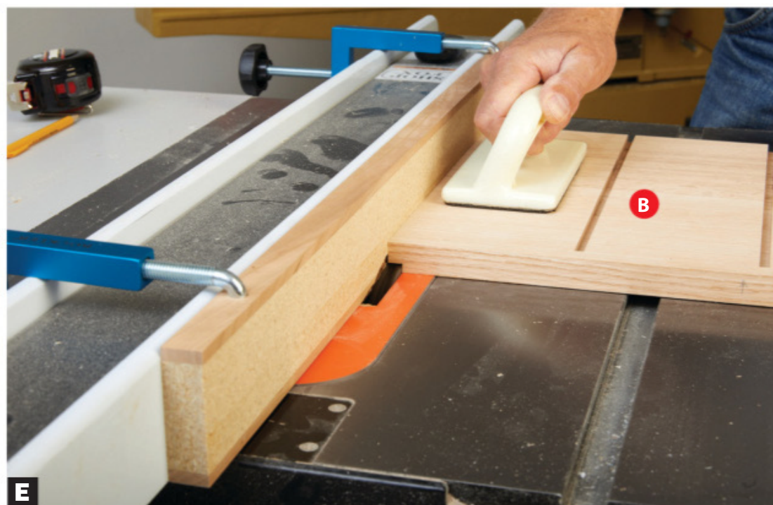
E To rabbet the top face of the shelf and the bottom, work with the dadoed side of the shelf (B) and the plain face of the bottom (C) facing up.
