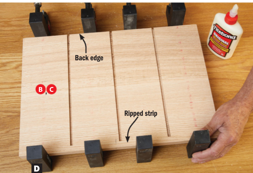
D Form stopped dadoes by gluing the ripped strips back onto the shelf and bottom. Keep the faces and ends flush as you clamp them.
