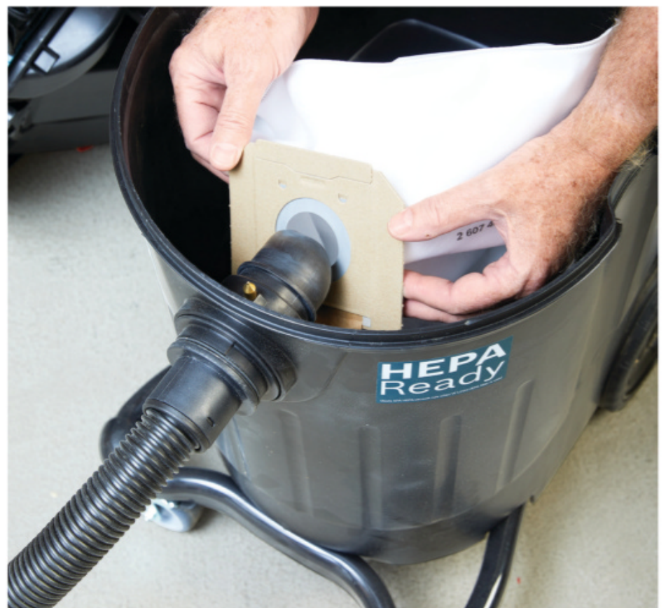
A fleece filter bag captures all debris and does the best job of filtering dust before it can reach the HEPA filter.
