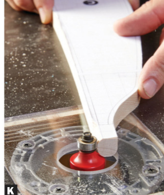
K Shape the arm tenon with a \frac{1}{4} " round-over bit. Set the bit slightly low in the table to leave a flat surface for the bearing to ride on. Sand the tenon to shape.
