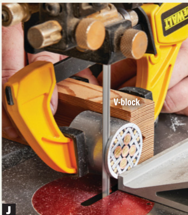
J Clamp the cylinder to a V-block for stability when bandsawing the medallions. A fine-toothed woodcutting blade easily slices the soft metals and epoxy.
