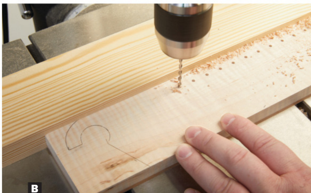
B Clamp a straight scrap to your drill-press table to align rows of holes.
