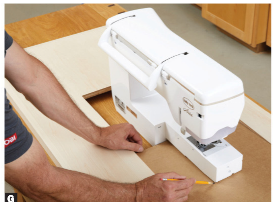
G Reposition the cardboard and mark the side-to-side extents of the machine. Extend both sets of lines to derive the outline of the filler opening.
