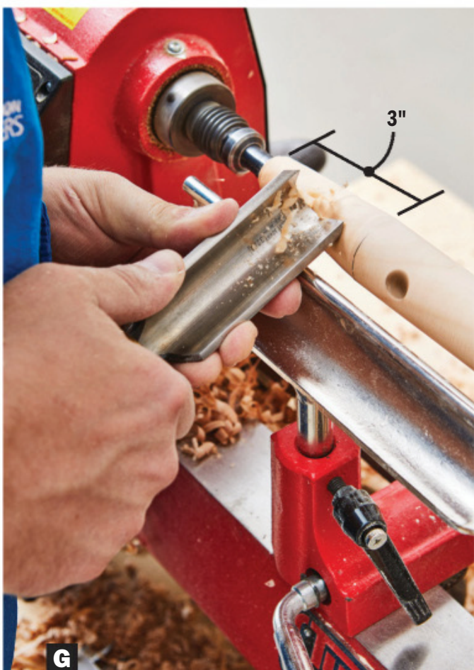
G Form a straight taper for the foot. Establish the foot's bottom diameter with a parting cut, then work down from the guideline with the roughing gouge.
