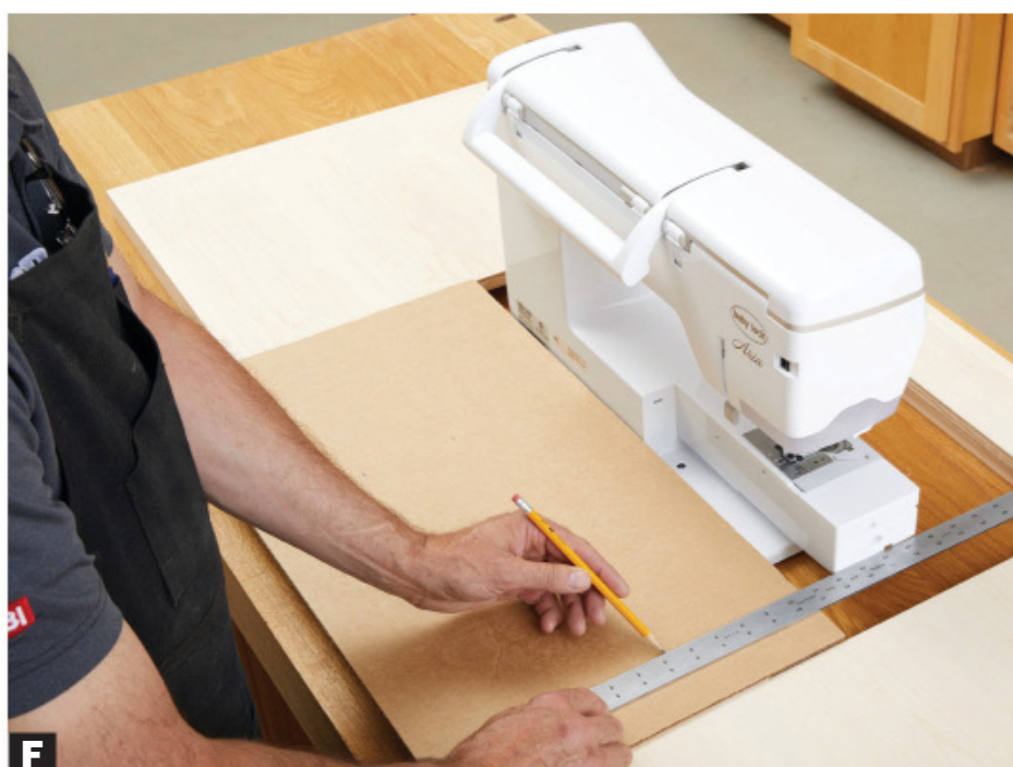
F Mark the front-to-back extents of the machine bed on the piece of cardboard aligned with the tabletop opening.
