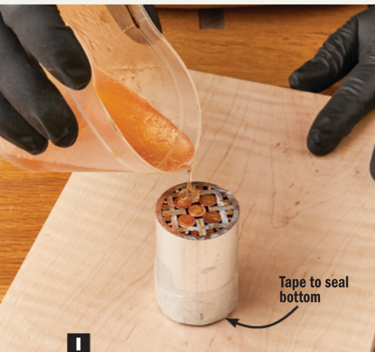
I Pour the epoxy slowly to let it flow into the spaces. Rap the sides of the cylinder frequently as you pour to release bubbles.
