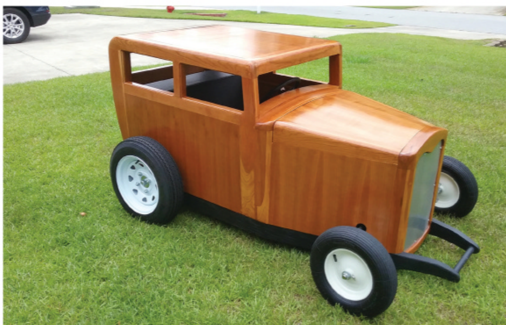
This miniature 1932 Ford, built by Bill Proctor , of Chocowinity, N.C., is powered by a 48-volt electric motor. It sports rack-and-pinion steering and hydraulic disc brakes. And, of course, it's cherry. 🌳
