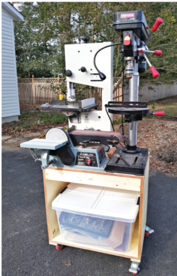
Consolidating tools on a mobile cart saves John a lot of floorspace. Plus, he can move the tools into the driveway when the weather is nice.
