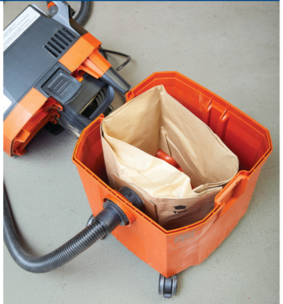
A paper filter bag captures all debris inside with only the finest dust getting through to the HEPA filter.
