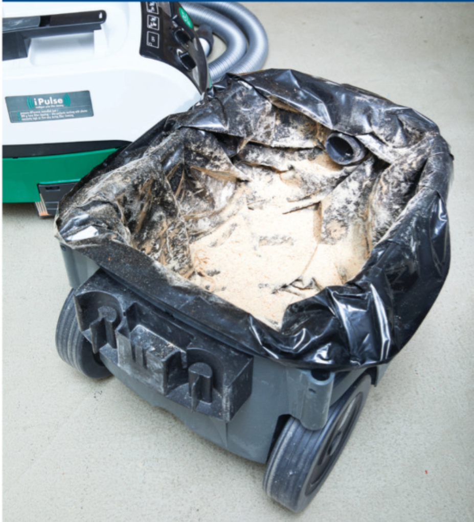
A drop-in bag liner collects debris so it's easier to lift out for disposal, but allows all dust access to the HEPA filters.
