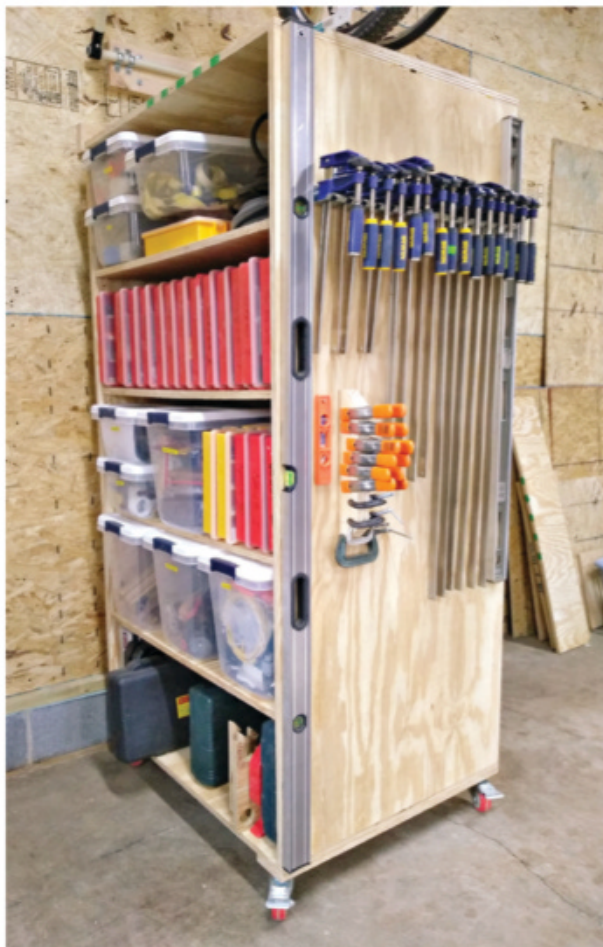
John designed this 6'-tall storage cabinet to fit a collection of plastic tubs and trays. A center divider allows for access to shelves on both sides.
