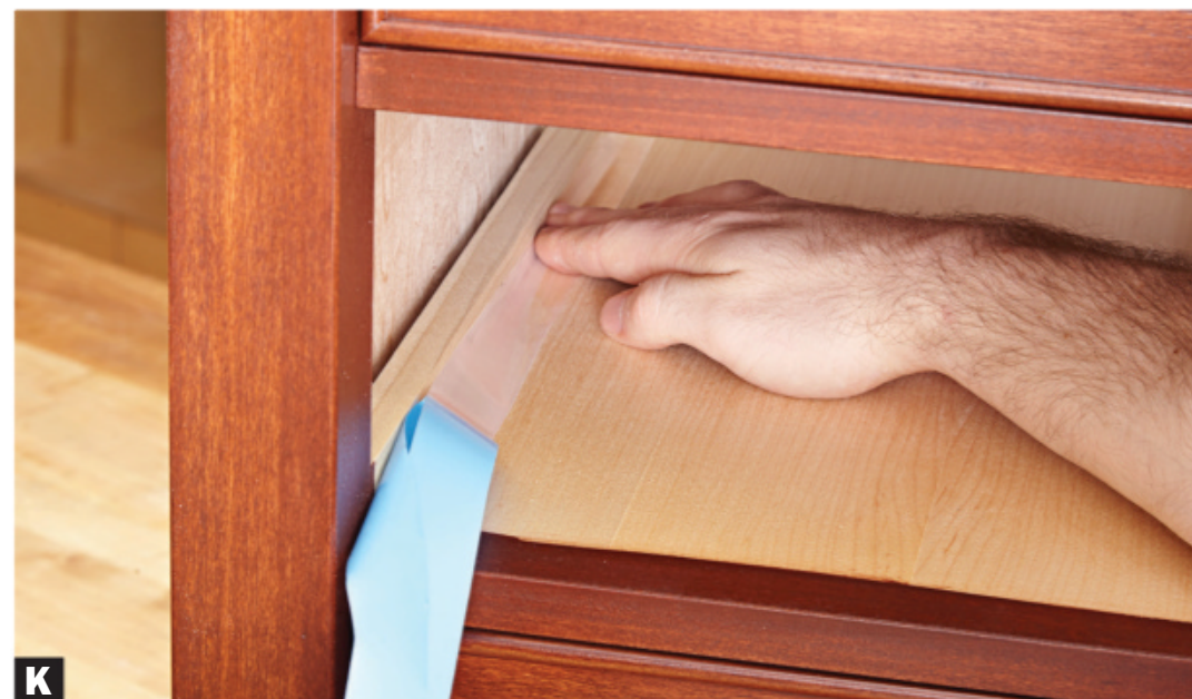
K Apply self-adhesive glide strips to the dust frame inside a cabinet or case so the drawer slides easily on their slippery-smooth surfaces.
