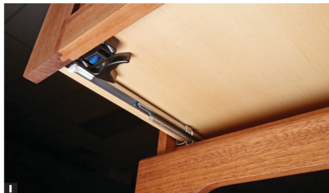
I Soft-close slides close by hand, but the self-closing mechanism engages the last couple of inches to gently close the drawer and keep contents from scooting.
