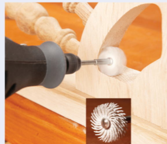
Powered by a rotary tool, these discs (inset) conform to the radius of an inside curve without changing it.
