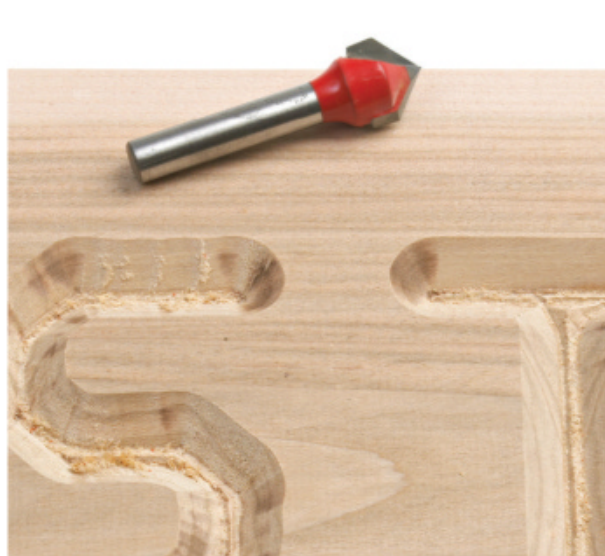
A V-groove bit creates beveled side walls , but slight play between the bushing and templates leaves a thin ridge in the bottoms.
