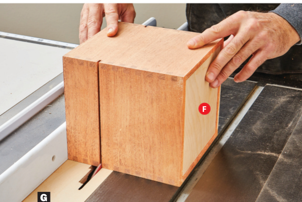
G Position the fence to leave just more than six fingers between the blade and fence. Make a pass on each face, placing shims in the kerfs on the third and fourth cuts to prevent them from pinching shut.
