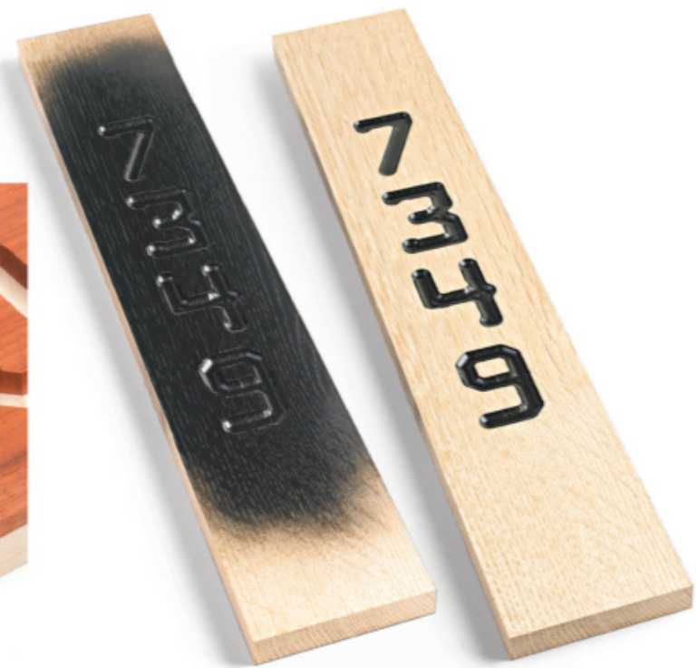
When planing a sign to remove overspray , skim off no more than 1/64" per pass to avoid tearing out the wood around the characters.
