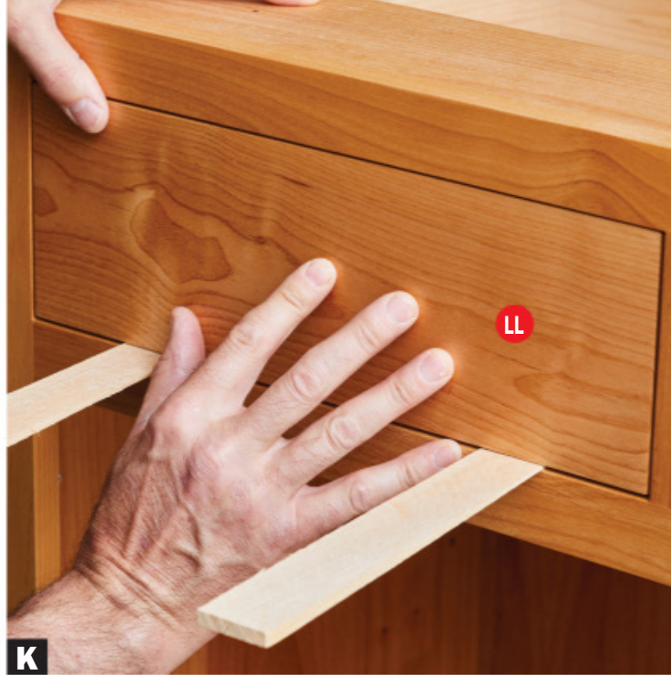
Firmly press the drawer face (LL) onto double-faced tape applied to the front of the drawer box. Shims ensure equal gaps at top and bottom.
