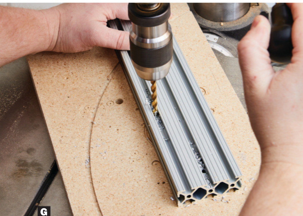
G Center the bit between the rail edges as you drill through the triple-rail web. The holes provide access to tighten socket cap screws in the bottom rail.
