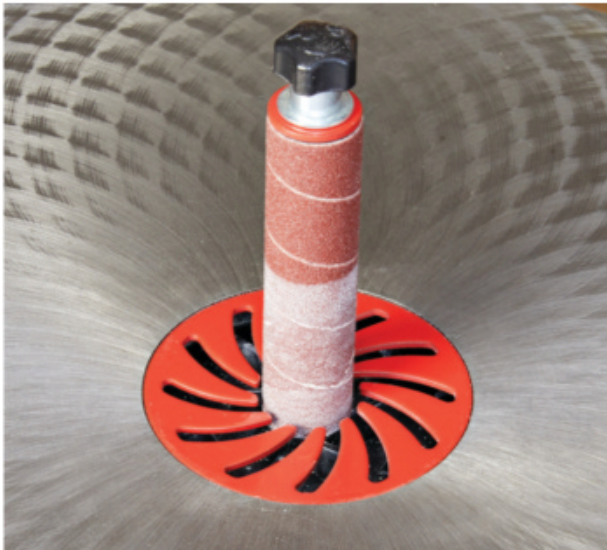
Dust evacuates easily into slotted insert rings, shown on the Grizzly G0723, when a shop vacuum provides adequate suction.
