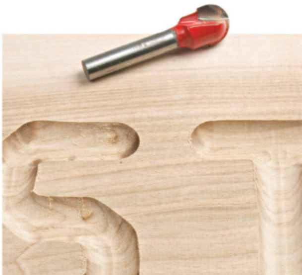
A 1/2" round-nose bit adds greater depth and width to the characters than the 3/8" round-nose bit included with the kit.
