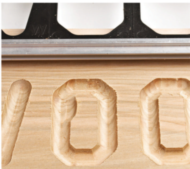
We goofed this "O" because the router strayed from the template edge. Shallow cuts and concentration will help avoid this.
