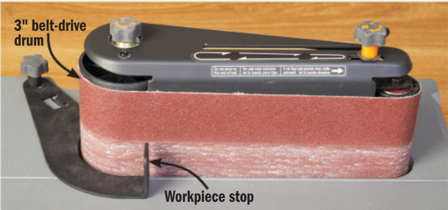
Instead of a dedicated 3" drum, the spindle/belt sanders offer the use of the belt-drive drum (minus the workpiece stop) for curves of that size.
