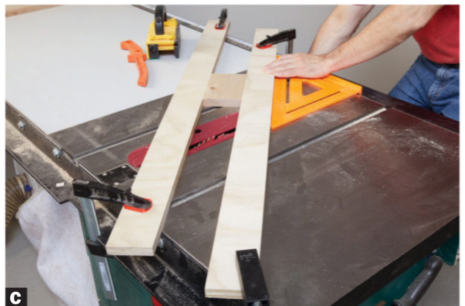
C Use a cutoff from the cove (W, X) blanks to space the guides on the tablesaw.
