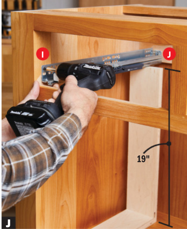
Screw the drawer slides to the slide blocks (I) while resting the rear of the slide on a temporary support. Then screw the rear-mounting brackets to the rail (J).
