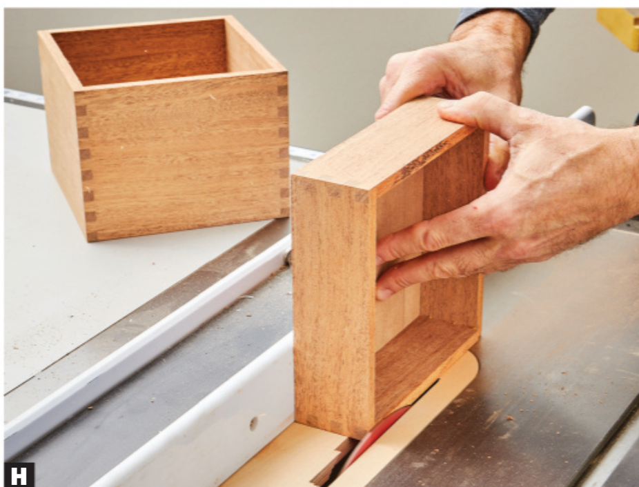
H Trim away the partially cut finger on the lid and the next finger on the box to maintain the joint pattern with the lid in place.
