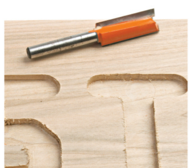
A straight bit tears out the wood slightly more than other bits , but the perpendicular side walls add shadows for more contrast.
