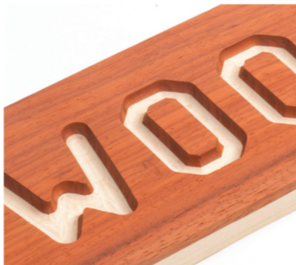
Laminate 1/4"-thick padauk or another dark species onto 1/2" or thicker maple, and then rout at least 3/8" deep to get contrast.
