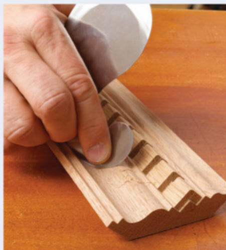
Work a goose-neck scraper at a slight skew angle to remove machine marks from coves prior to finish-sanding.
