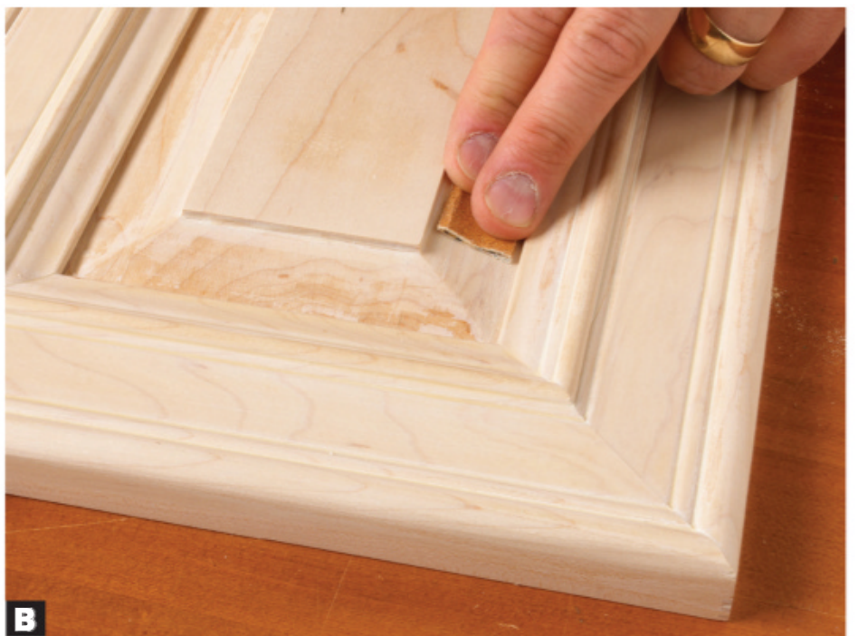
B Overlapping fingertips and a piece of folded sandpaper smooth the bevel on this manufactured door panel.
