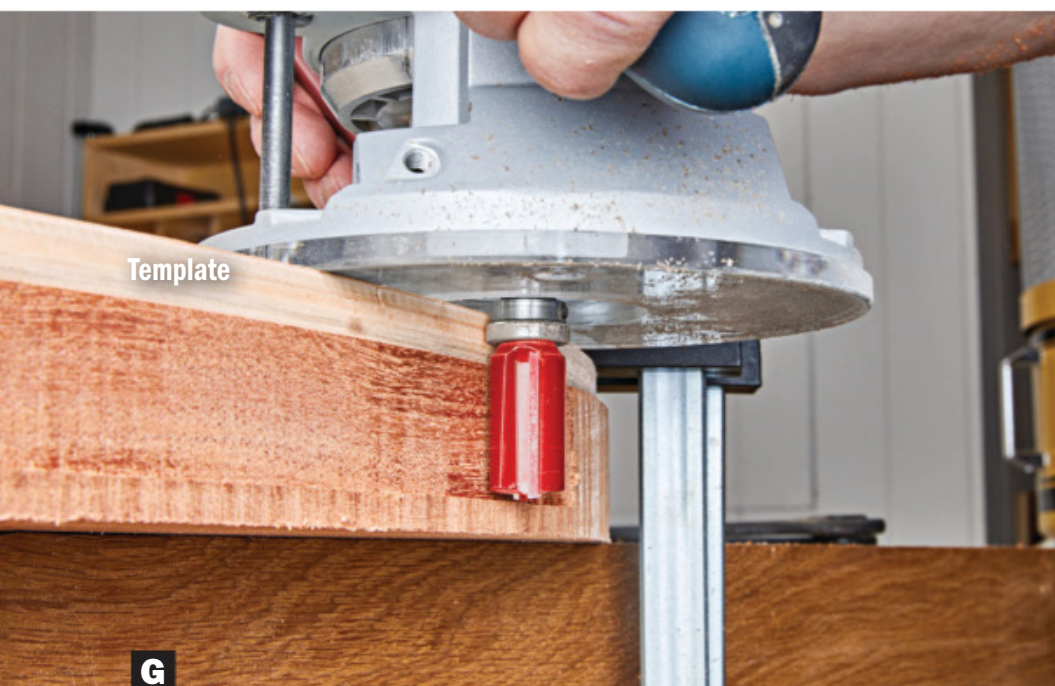
E A pattern bit places the bearing between the cutters and shank. The router rides on the template.
