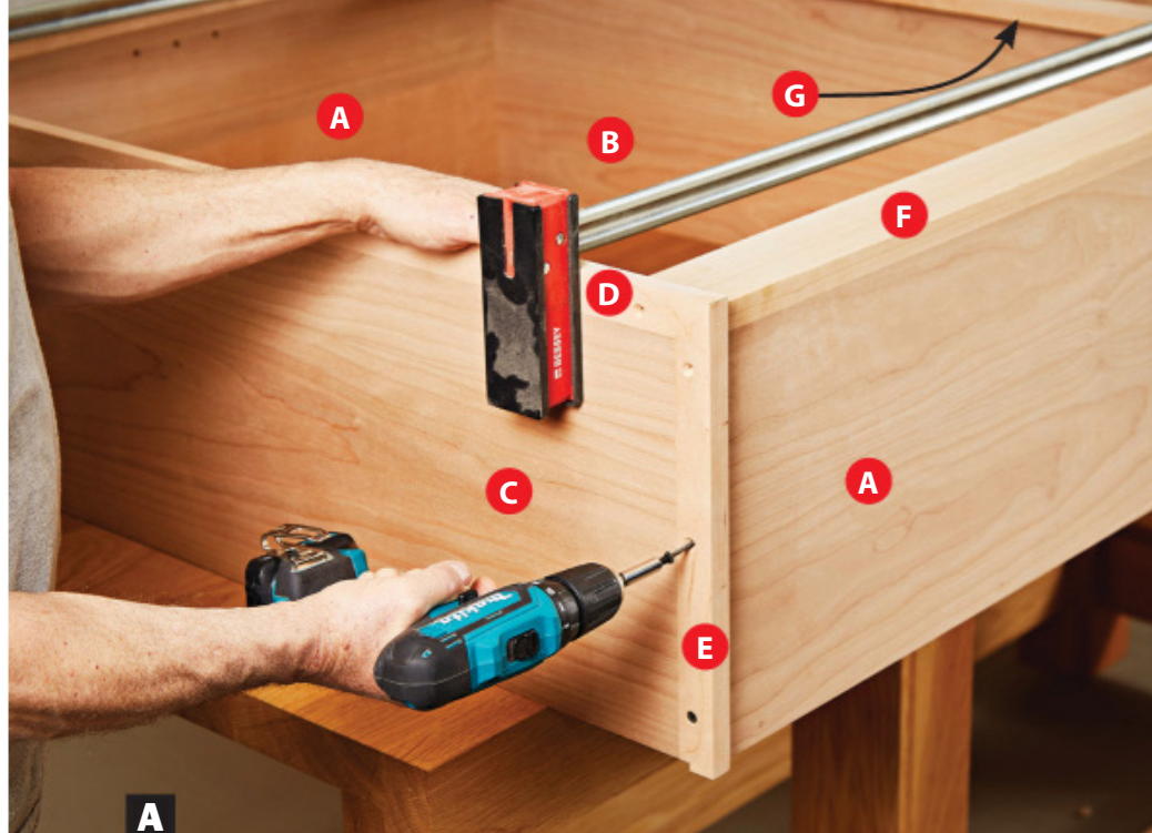
A Center the bottom from side to side and align the back of the bottom panel (C) with the inside edge of the side rabbets.
