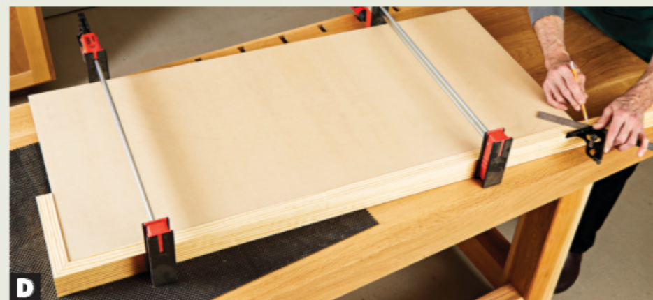
D Clamp the side edging in place and mark the miter at the second corner. Cut the miter and clamp the side edging back in place.
