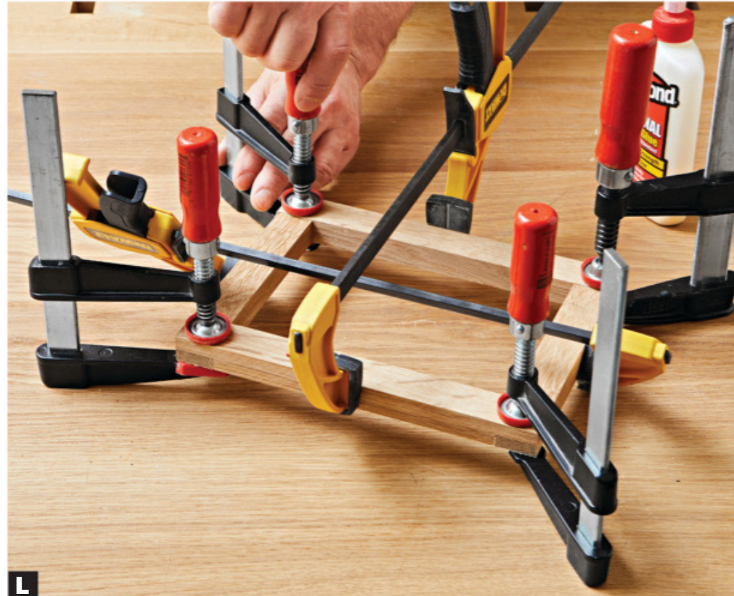
L Glue up the joint with a clamp in each direction pulling the shoulders tight, and others pressing the joint faces together.
