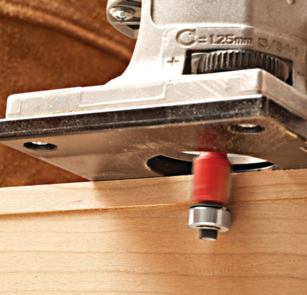
Using a flush-trim bit in a router, shave off the excess edging in a right-to-left direction (called “climb-cutting”) to avoid tear-out.
