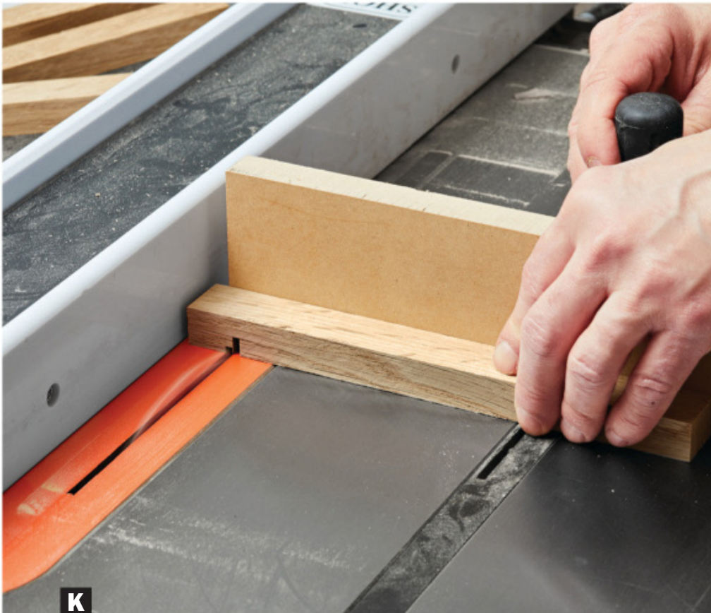
K Rabbet the ends of each frame piece. An auxiliary miter-gauge fence steadies the workpiece and prevents chip-out on the trailing edge of the cut.
