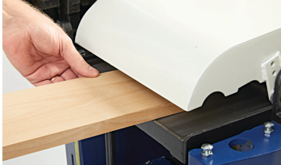
The chip-collection hood limits access to the planer infeed table on several machines (Rikon 25-210H shown here) when planing 2"-or-thinner boards.
