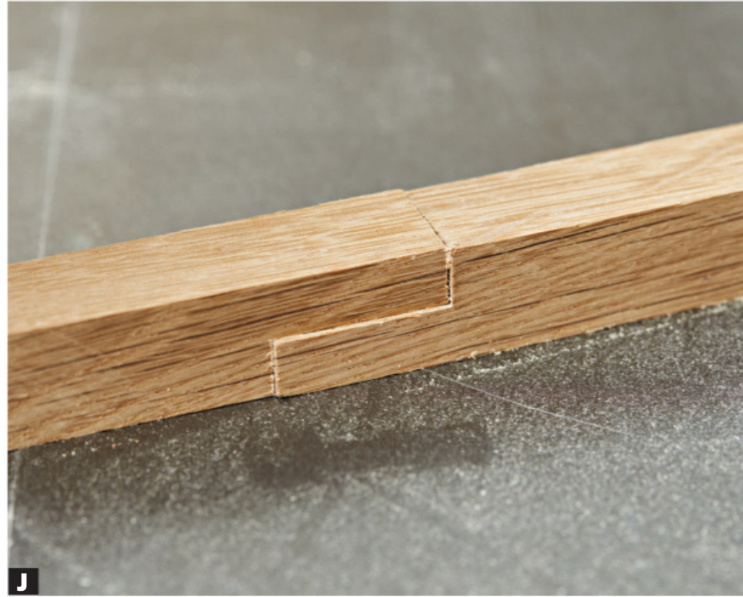
J Rabbet the end of two scraps the same thickness as your frame pieces. Lying on a flat surface, the two rabbets should meet, with their top faces flush.
