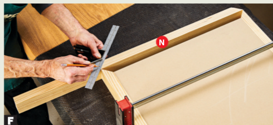
F Align the second end edging (N) miter point to point with the second side edging. Mark and cut the miter.
