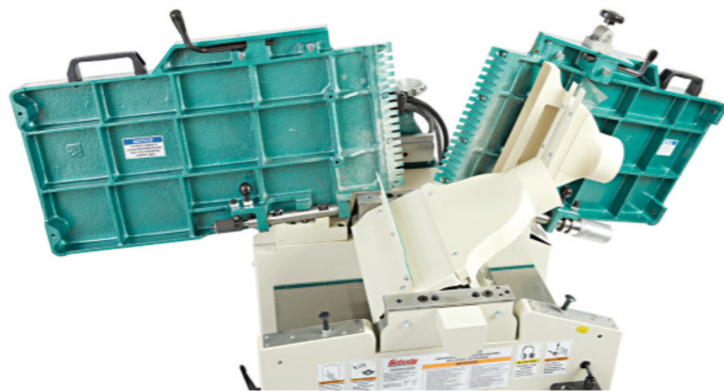
The Grizzly has separate chip-collection hoods and split jointer tables, making its changeover different from the other jointer/planers.
