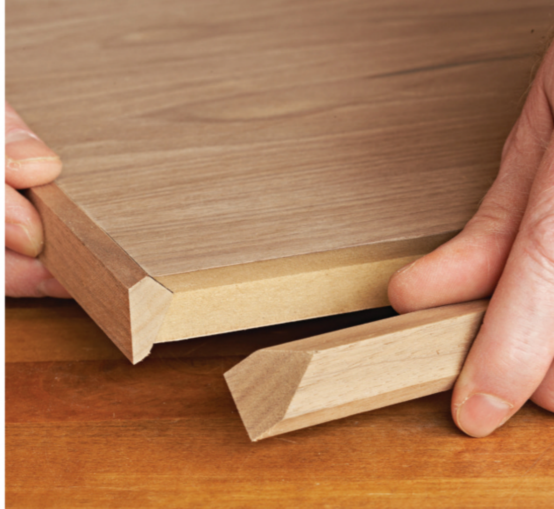
To wrap all the plywood or MDF panel's edges in solid wood, make edging pieces extra-long and then miter-cut to fit. Glue the mitered corner as well as the edges.
