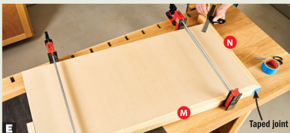
E Position the first end edging (N) and secure the joint at the second corner with tape. Mark and cut the miter. Repeat with the second side edging.
