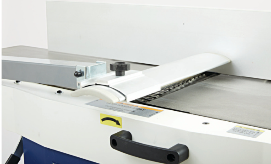
European-style guards cover the full cutterhead, and raise and lower for different board thicknesses.
