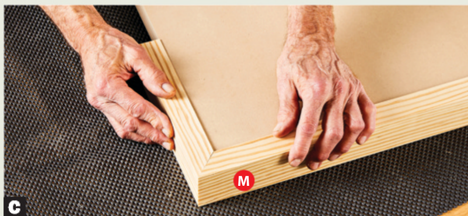
C Align the mitered end of the first side edging (M) at the first corner using the mitered scrap.
