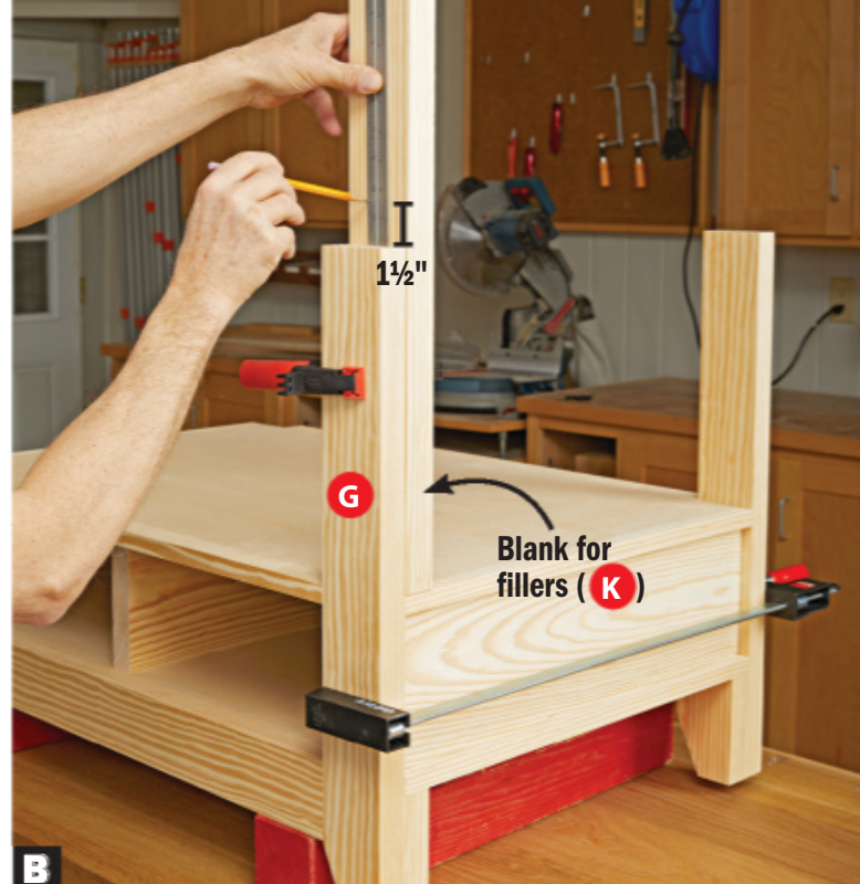
B Mark the length of the fillers (K) on the filler blank to compensate for any slight dimensional variations in the case, leg, and upright assemblies.
