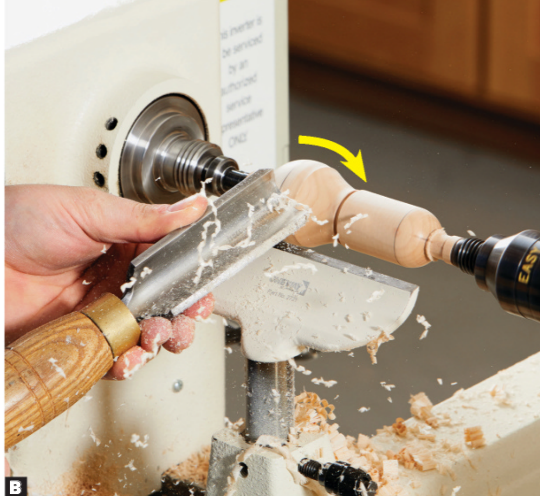
B Start away from the line that marks the equator of the hemisphere and work toward the parting cut. Start closer to the line with each cut.
