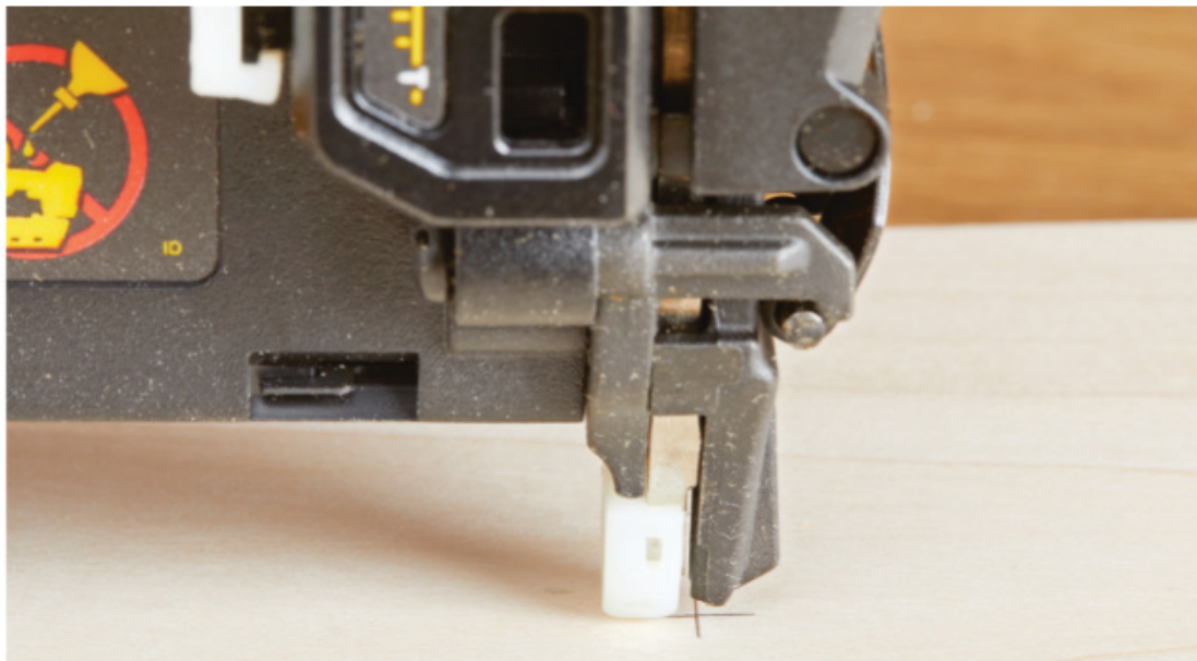
BETTER: DeWalt's nose tip sits behind the nose, providing good visibility of the target.
