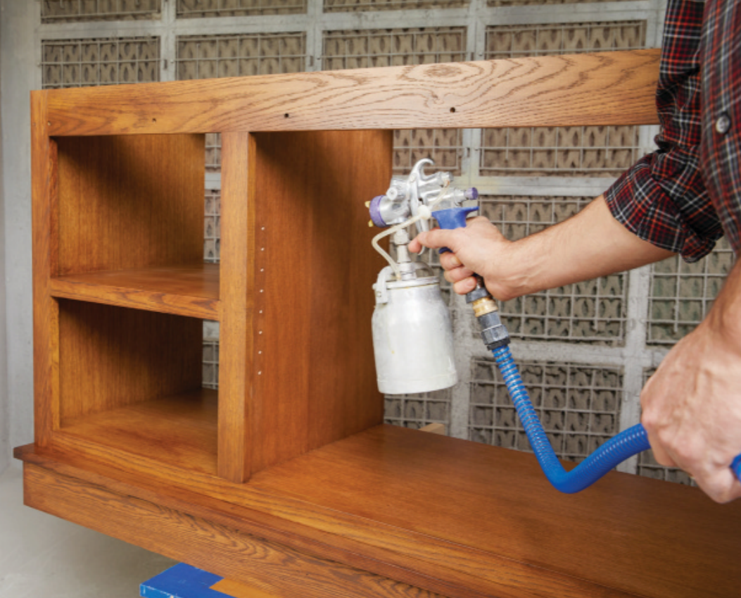
With case-type projects, spray the interior upright elements first.
