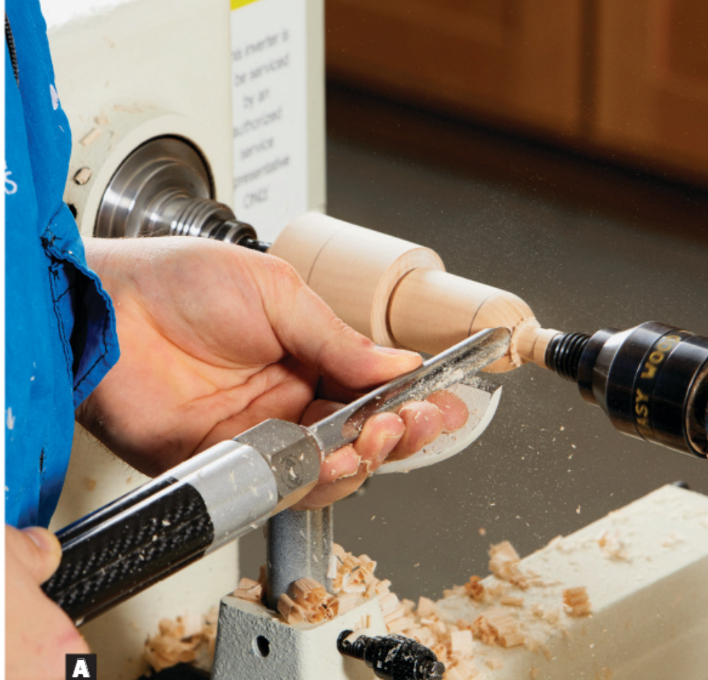
A Work from large diameter to small, lifting the handle and rolling the gouge.
