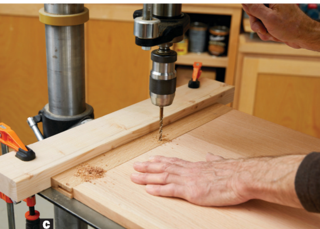
C Drill \frac{1}{4} " holes for dowels, either all the way through to expose the dowels, or from the bottom, stopping \frac{1}{8} " from the top surface, to conceal them.
