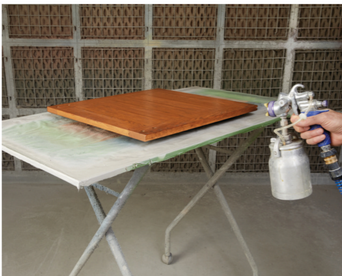
For doors, spray the outer edges first, then spray the rail and stile faces and panel.
