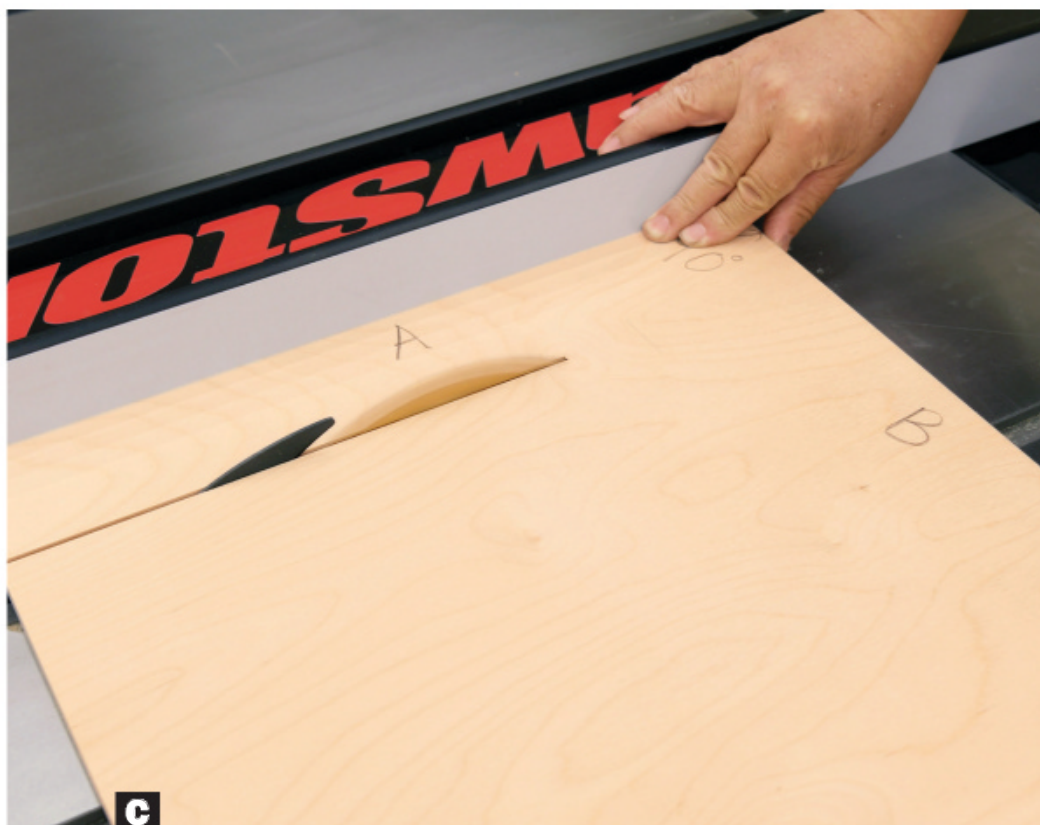
C Cut the “A” leg 3" wide, stopping 3" short of the “B” edge, as measured on the bottom side of the panel.
