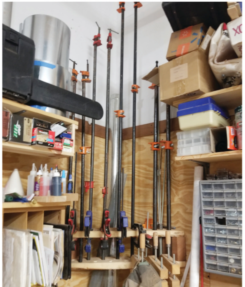
Joe took advantage of unused corner space by installing racks to hold his clamps.
