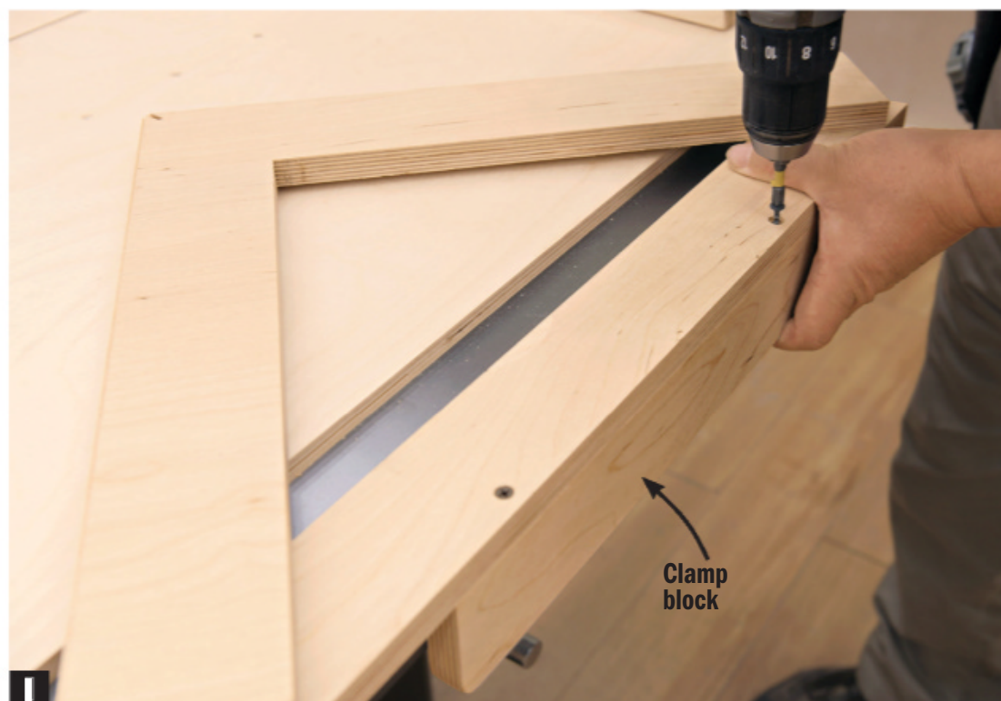
G Space the short leg using a feeler gauge and cut another test triangle, measure the short edges, and, if needed, calculate any error as you did before.
