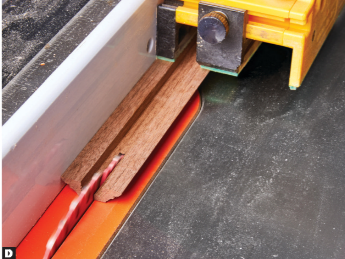
D A pushblock keeps your hands clear of the blade while ripping the blanks.
