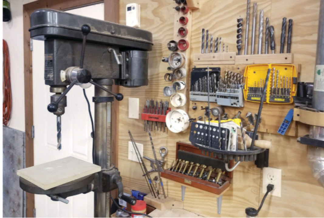
Lining the shop walls with 1/2"-thick plywood allows Joe to cluster custom storage racks, such as these drill-bit organizers, near his drill press.
