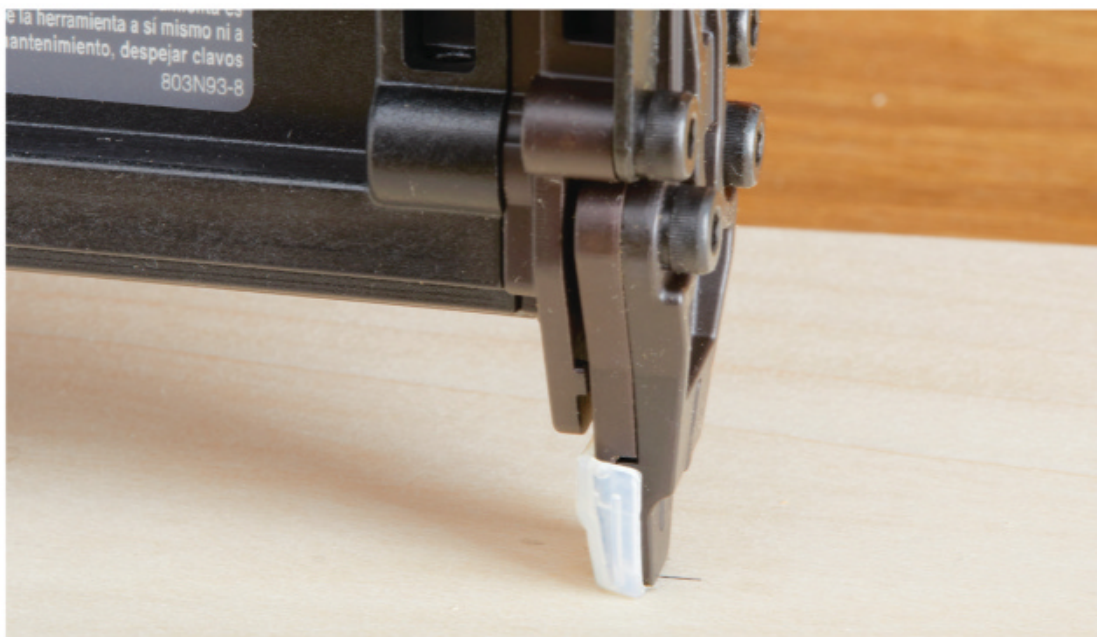
BEST: Makita's tiny translucent nose tip makes for the easiest alignment of any of the test nailers.
