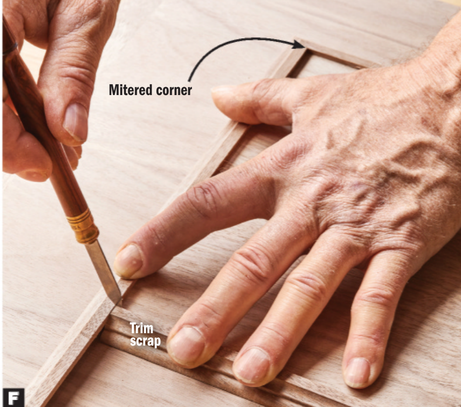
F Precisely fit the panel trim by marking the joint corners with a knife. A piece of scrap trim, or a good piece not yet miter-cut, aids accurate marking.
