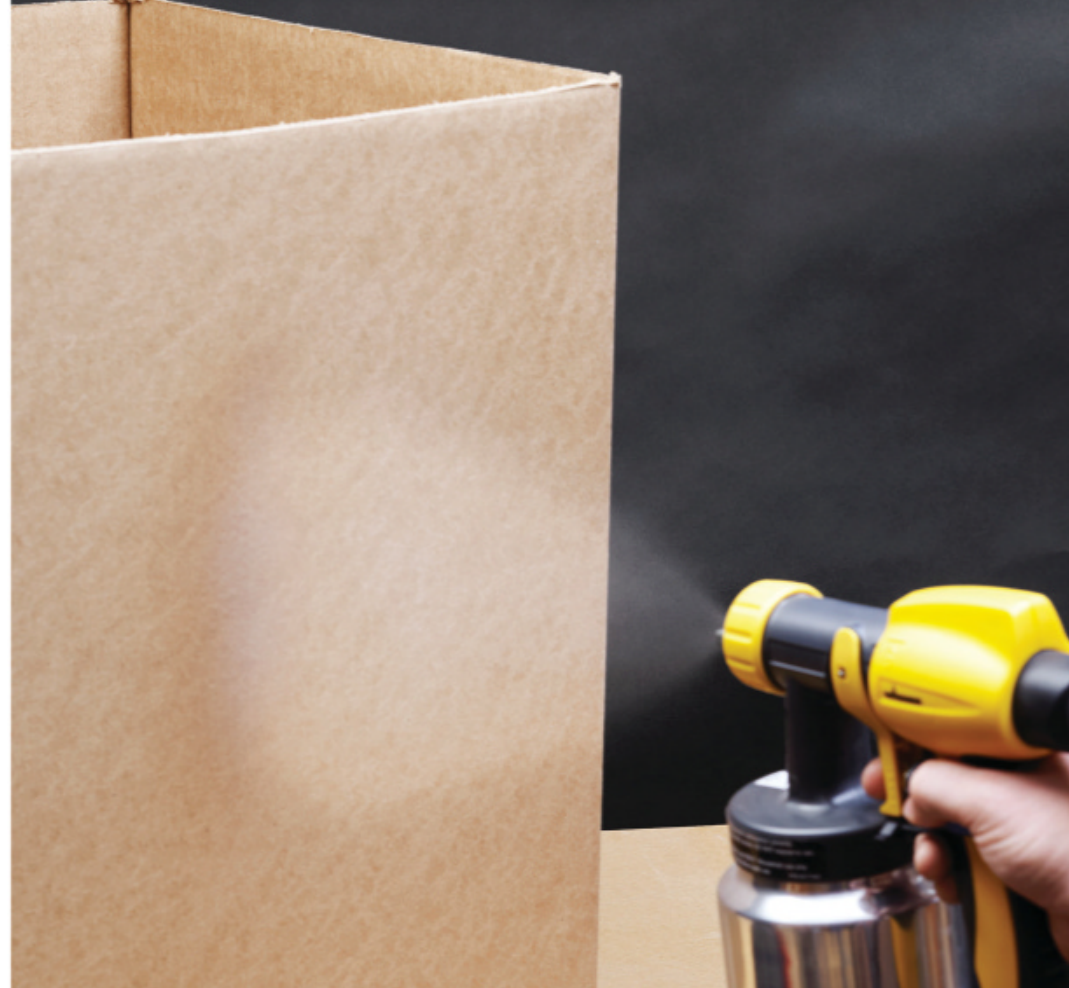
Spraying on cardboard lets you adjust the fan pattern and volume of finish as well as your technique without the worry of wasting wood.
