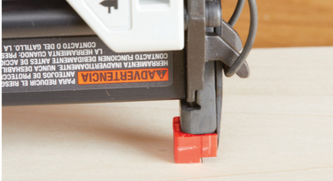
FAIR: Porter-Cable's U-shaped no-mar nose tip makes it difficult to see the driver location and align the nose precisely.
