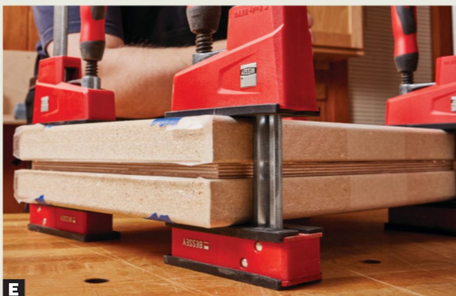
E Thick platens help spread clamping pressure evenly, but for panels exceeding 15" in width and length you may want to add deep-jaw clamps for exerting pressure closer to the sandwich center.
