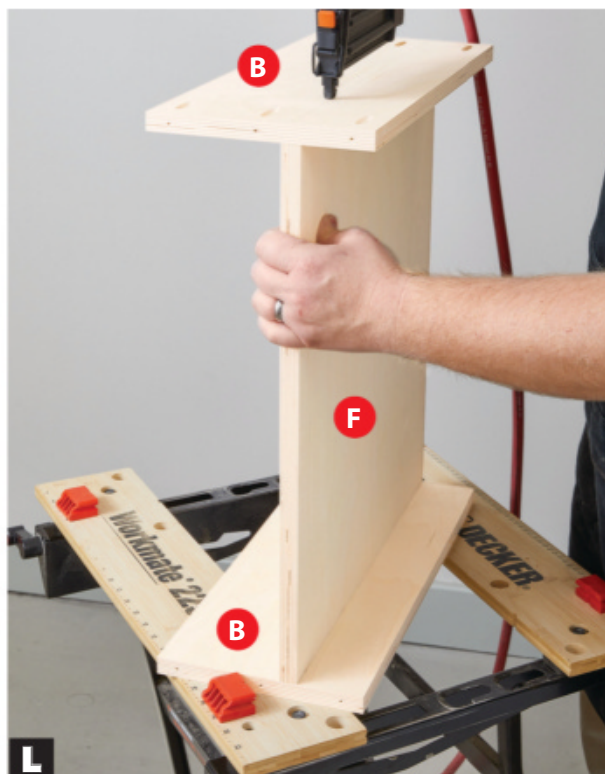
L Nail the divider (F) off center on the carcass top (B) and shelf (B) to leave space to drive pocket-hole screws.
