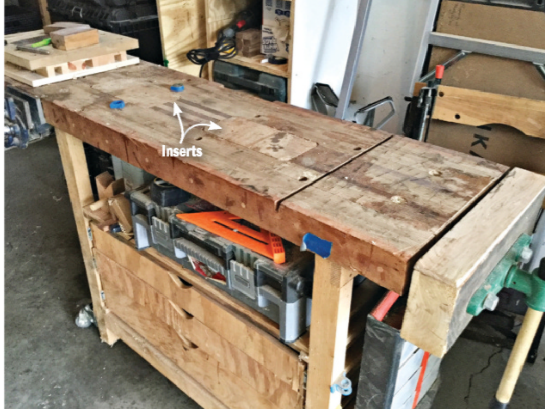
Timothy cut a pair of rabbeted openings in the benchtop and fitted each with an insert. Removing an insert allows him to slip the head of a clamp in place for additional options when assembling a project.
