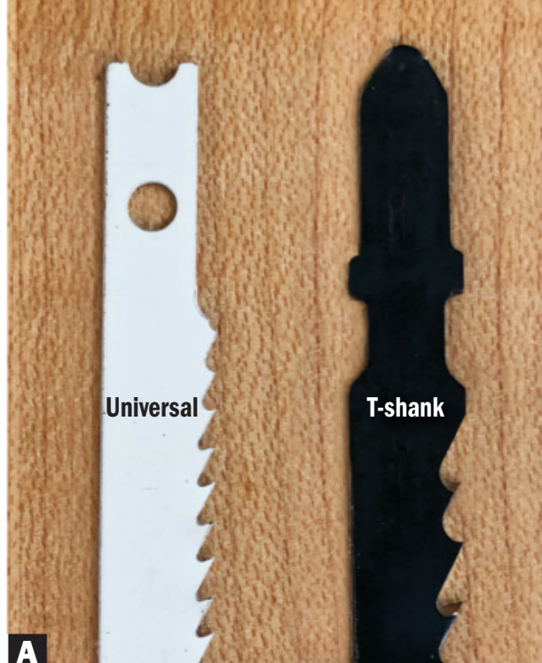
A A setscrew presses against the side of, or extends into a hole in, a universal blade. T-shanks hold securely and provide a much wider selection of blades.
