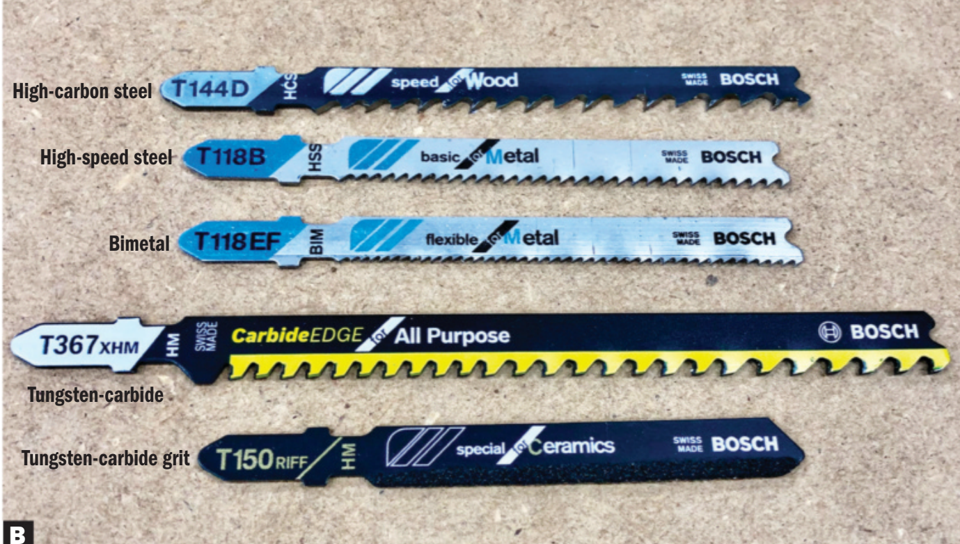
B Some blade types cut more than one type of material, and some materials can be cut by more than one type of blade.
