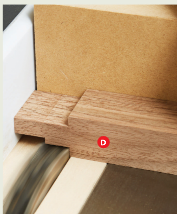
Raise the blade to 3/8" above the table and rabbet the top face of each side rail (D).
