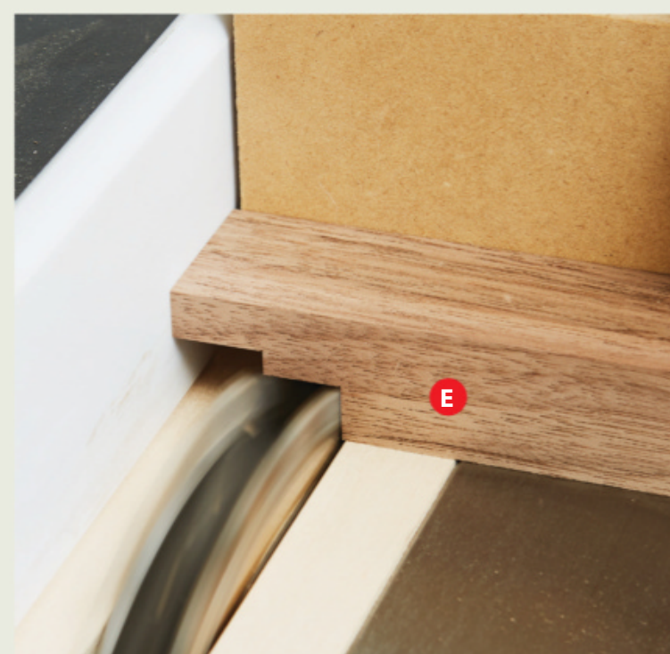
Raise the blade to 5/8" and rabbet the bottom face of the front and back rails (E).
