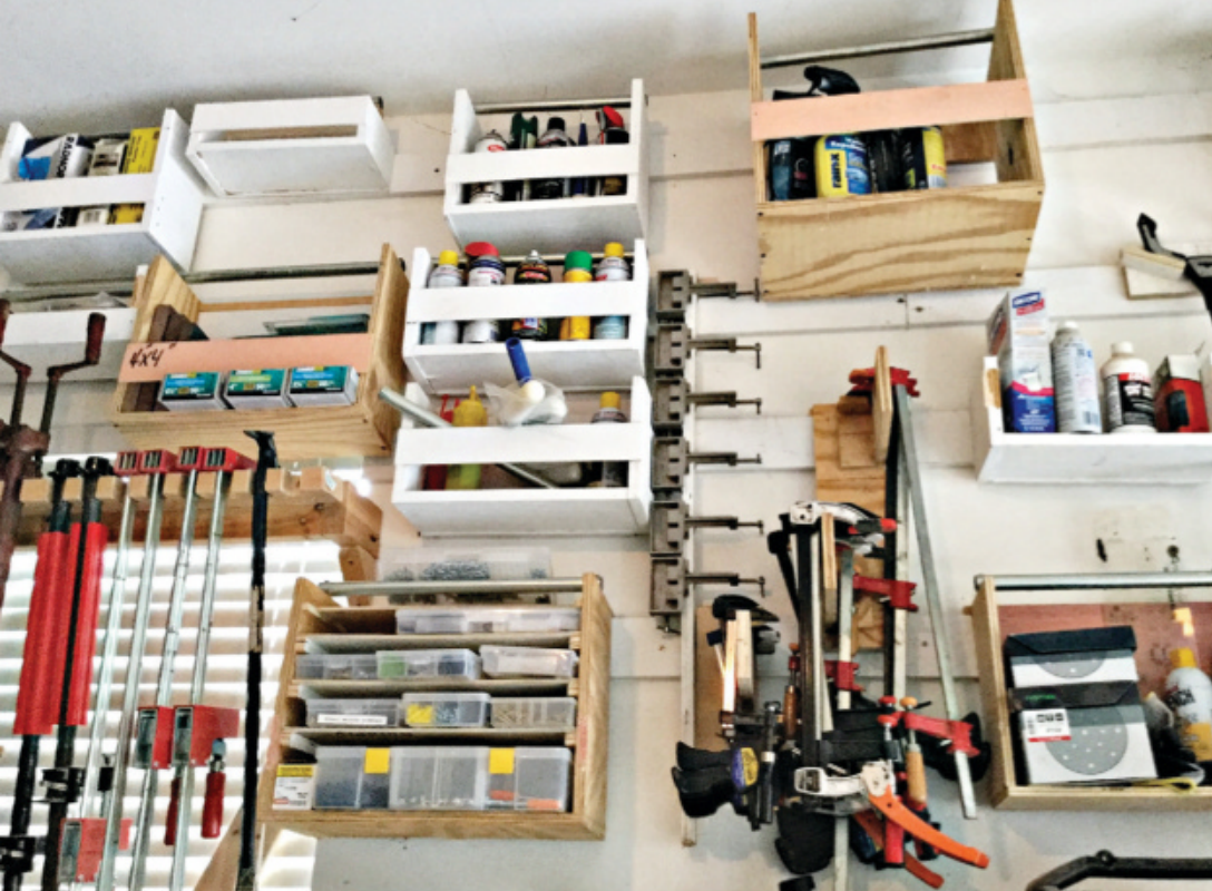
Lining one wall are rows of French cleats upon which hang custom storage racks. Timothy uses a step stool to access the highest bins.
