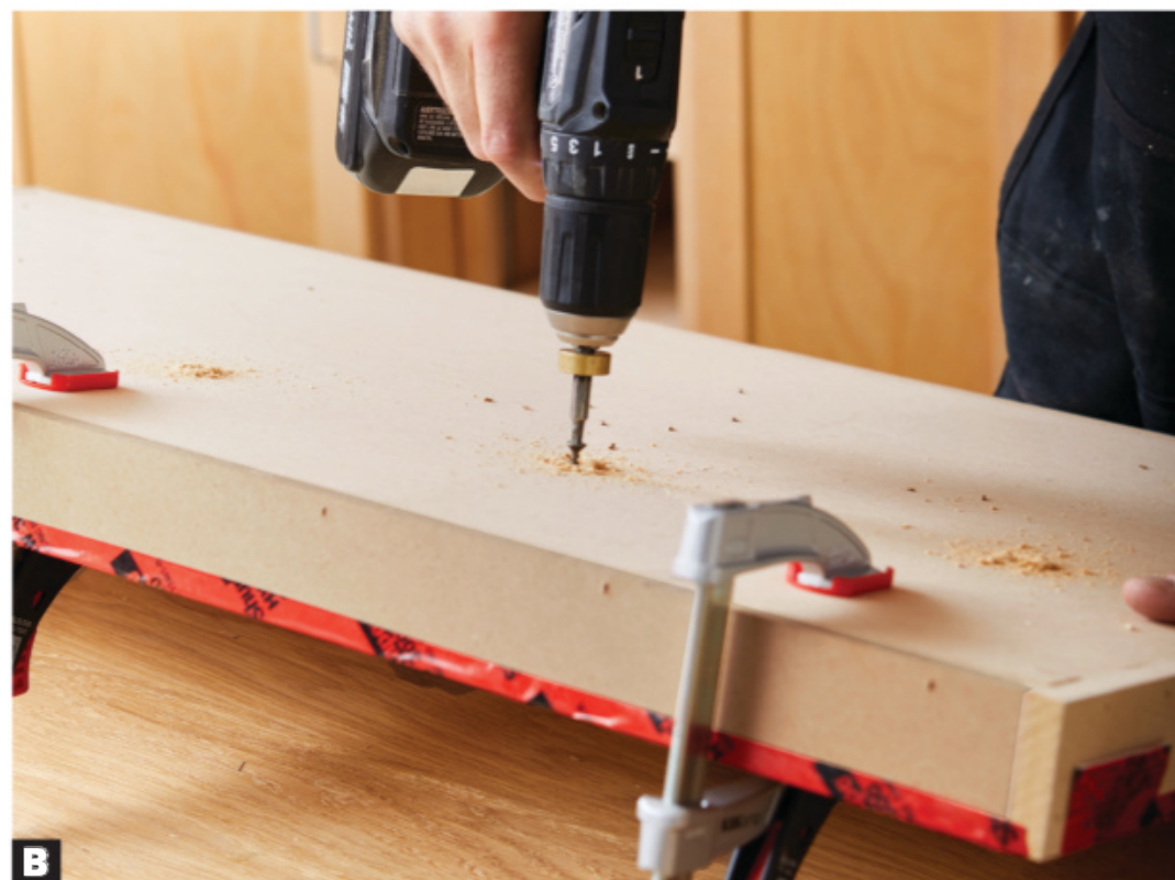
B Flip the tray over and countersink 1¼" screws through the bottom into the slabs, staying inside the outlines drawn earlier.
