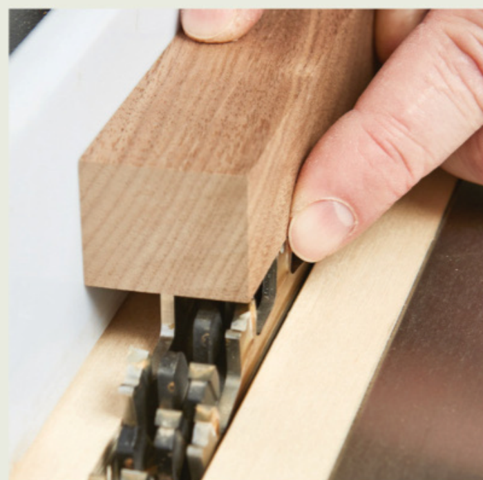
Use one of the test pieces to set your rip fence so the outside edge of the piece is flush with the outside tooth of the blade.
