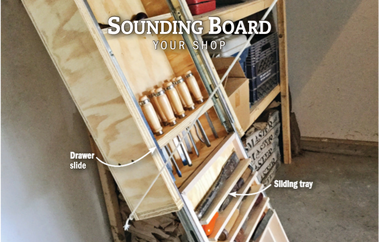
Timothy created double-decker chisel storage in one of the drop-down trays. The upper tray slides out on full-extension drawer slides, exposing the tools underneath.
