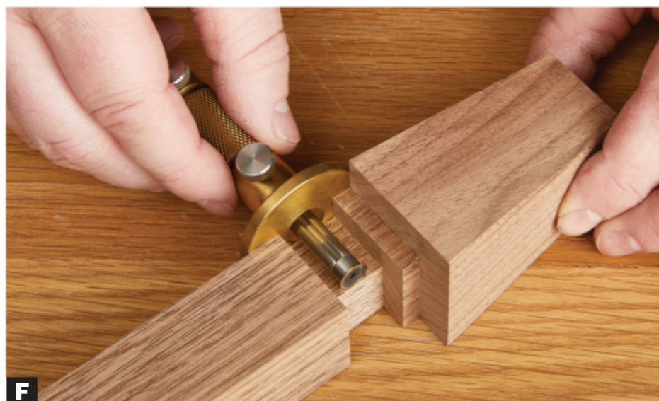
F Set a marking gauge to match the remaining width of the leg.
