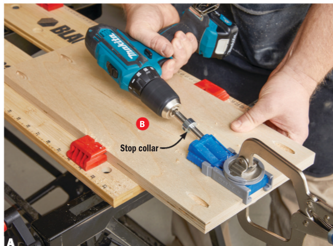
Adjust the pocket-hole-bit stop collar to drill 3/4"-thick material before drilling the outside faces of the carcass top and bottom (B).
