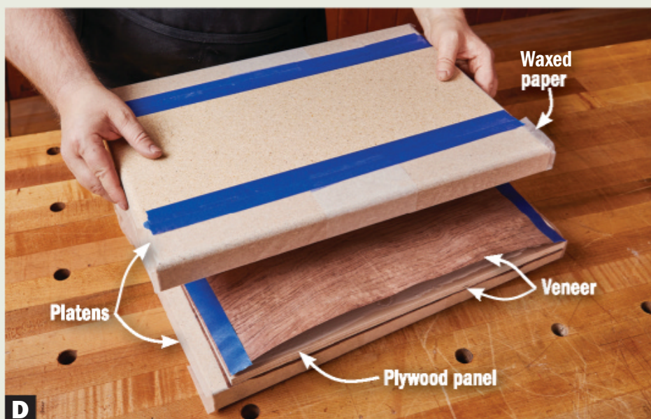
D Make a sandwich with the panel and veneer pieces between the platens. Double-check the layers to ensure they don't slip out of alignment as you work.
