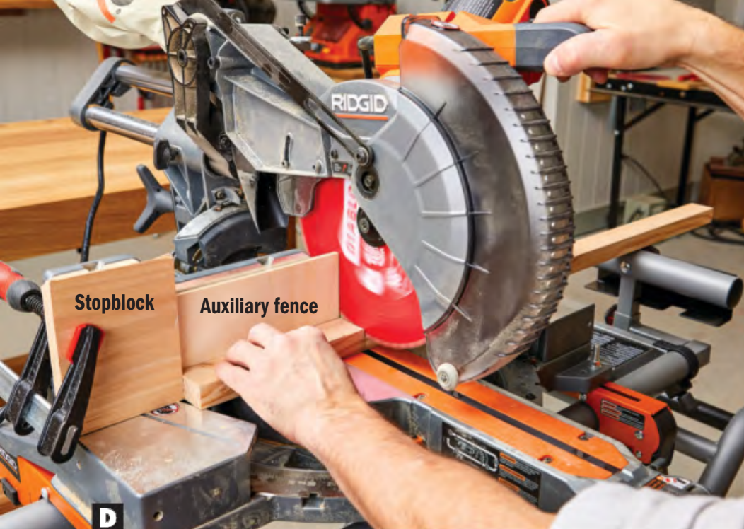
D An auxiliary fence prevents chip-out on the rear edge of the workpiece. Adding a stopblock simplifies cutting identical-length boards.
