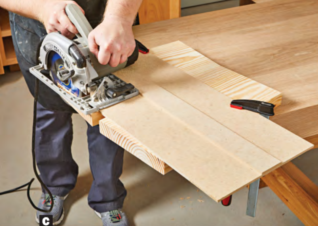
C Clamp the cutoff jig across the bottom of each leg assembly aligned at the outer corners. Cut to provide straight ends that will sit flat on the floor.
