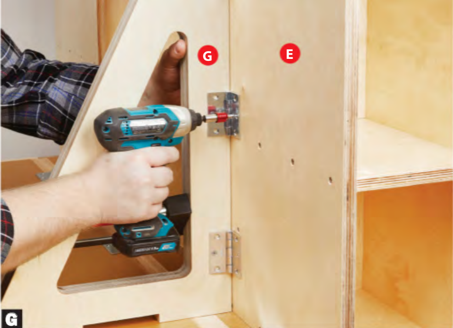
Install only the center-hole hinge screws , then check that the support swings smoothly before driving the remaining screws.
