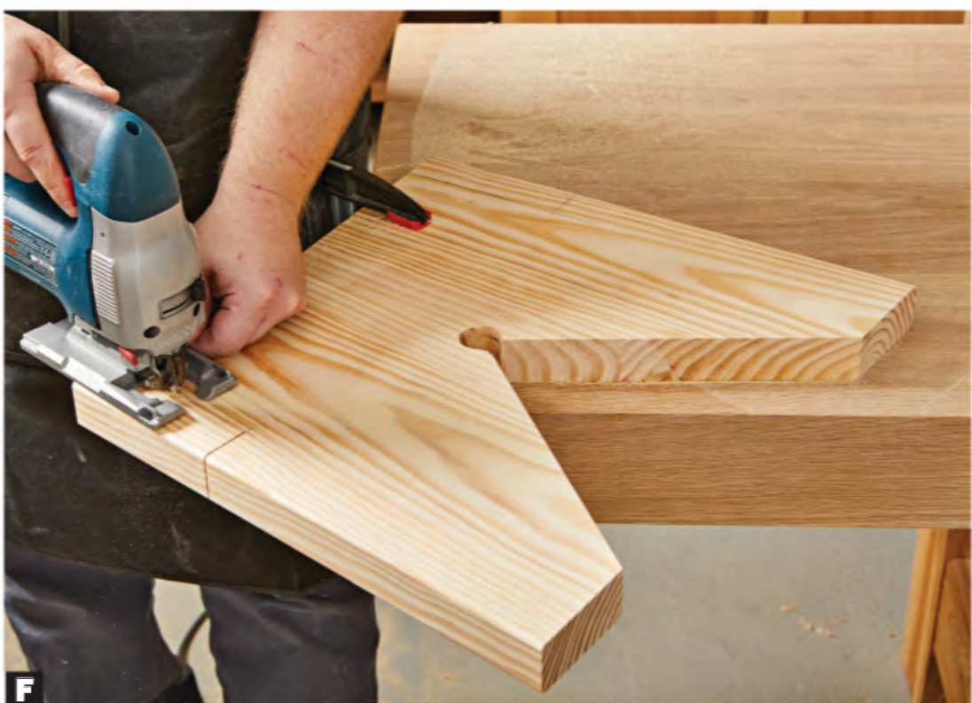
F Use a jigsaw to cut the notches on each leg assembly. Clean up the cuts as needed with chisels and sandpaper.
