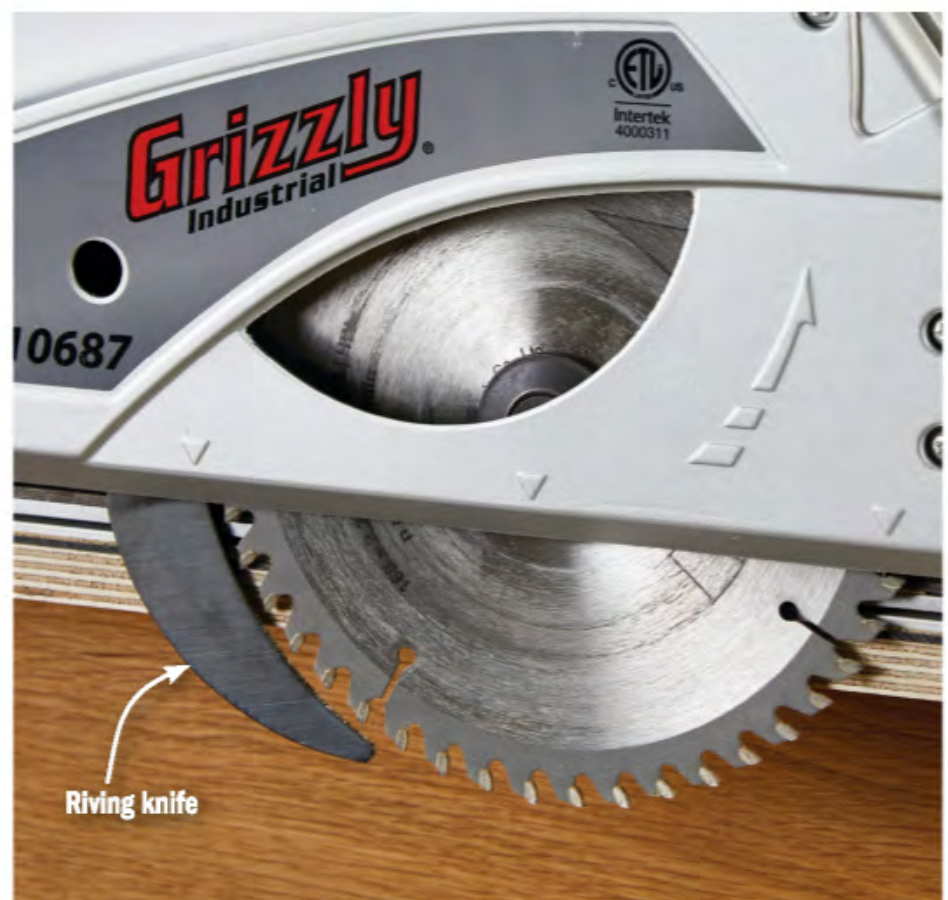
A riving knife follows the blade, and keeps the kerf open to prevent kickback resulting from the workpiece touching the back edge of the blade.
