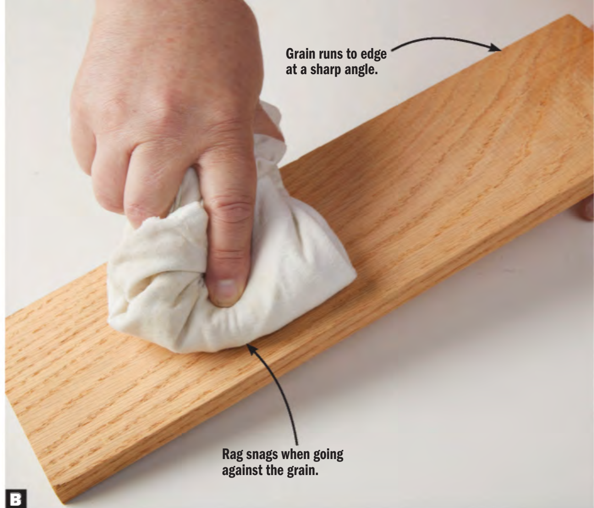
B Going with the grain feels smooth because the ends of the fibers at the surface point in the same direction as the movement of the rag.
