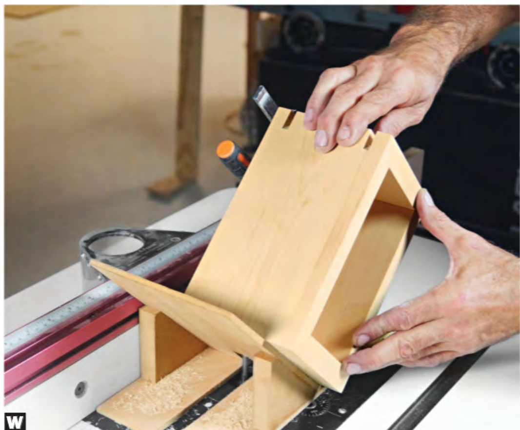
W Register the jig against the router-table fence. A straight bit cuts the spline slots. Move the stop on the jig to reposition the box to rout additional slots at each corner.
