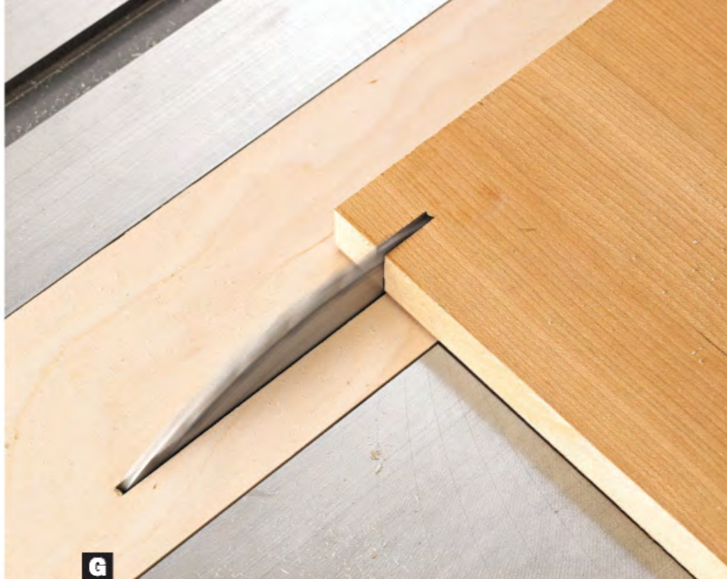
G A zero-clearance tablesaw insert and a high-quality crosscut blade will give you practically splinter-free cuts across the grain.
