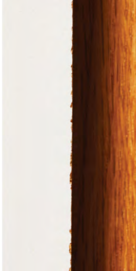
The Grizzly saw created more chip-out in the same material.
