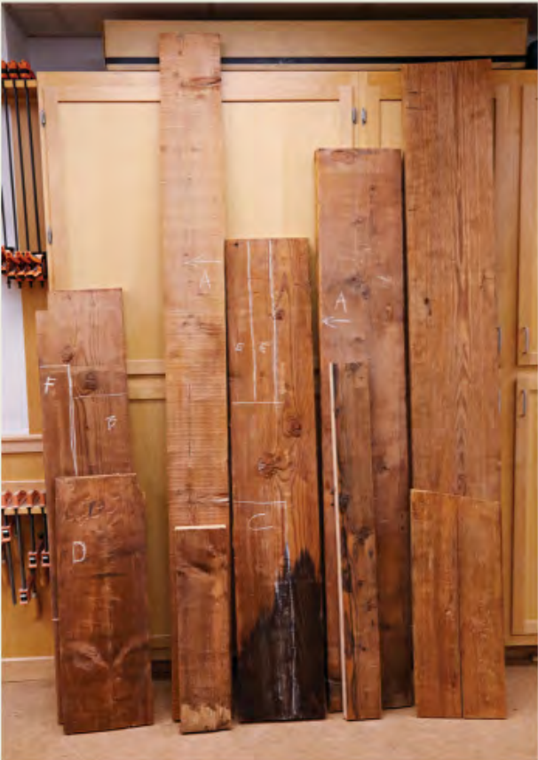
Even careful layout of parts leaves a few imperfections in workpieces cut from reclaimed Douglas fir joists.
