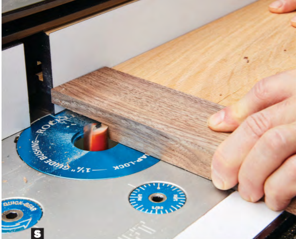
S Set up the same as for cutting a tenon, sneaking up on the bit height until the faces of the dry-fit workpieces rest flush.
