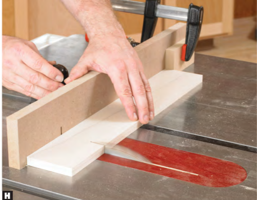
H A miter-gauge extension with a blade kerf supports the board on both sides of the cutline and reduces splintering on the trailing edge.
