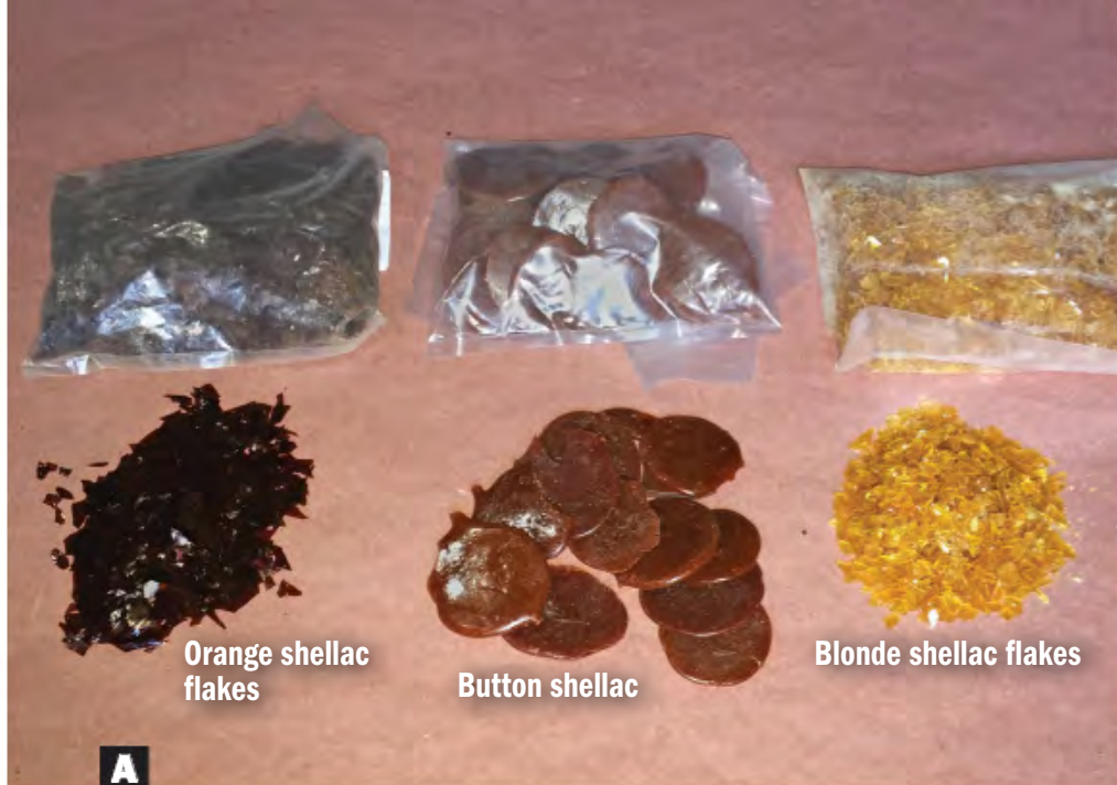
A Find shellac in flake or button form. Button shellac creates a more mar-resistant finish than flakes but comes only in darker hues.
