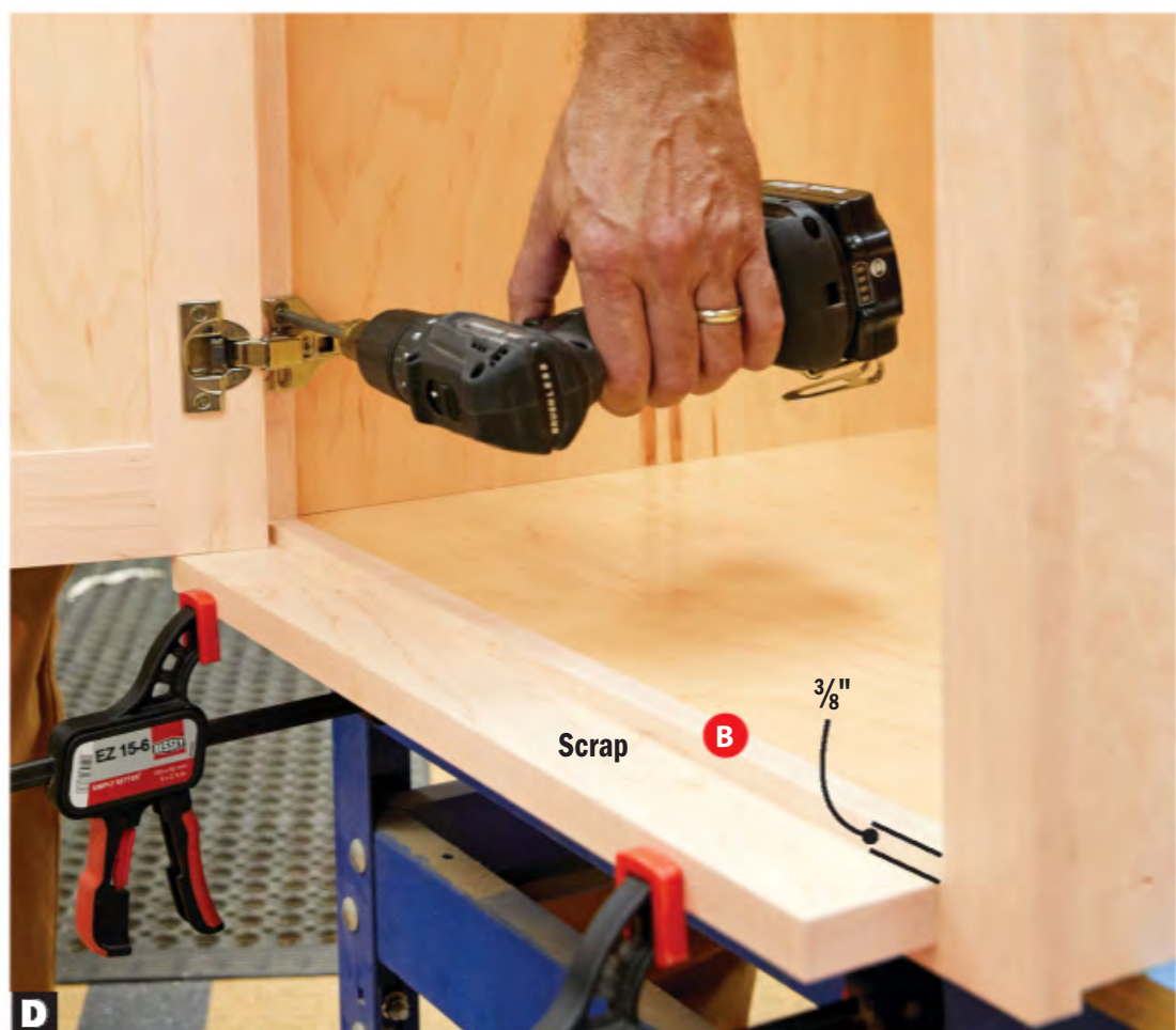
To position the door, clamp a scrap to the face frame, 3/8" below the top edge of the rail (B). Rest the door on the scrap, and screw the hinge plates to the face frame.
