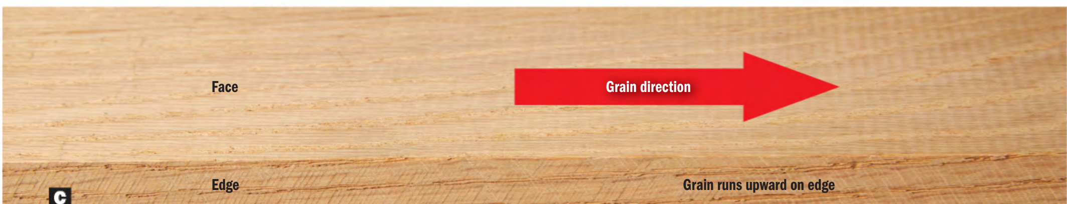
C Upward trending grain lines on the edge point in the direction the grain runs on the adjacent top face of this board. It runs opposite on the other face.
