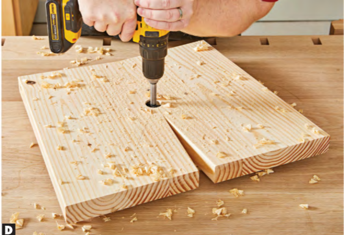
D Use a 1 1/4" Forstner bit to drill the hole. Support the back side with a piece of scrapwood to prevent tear-out.
