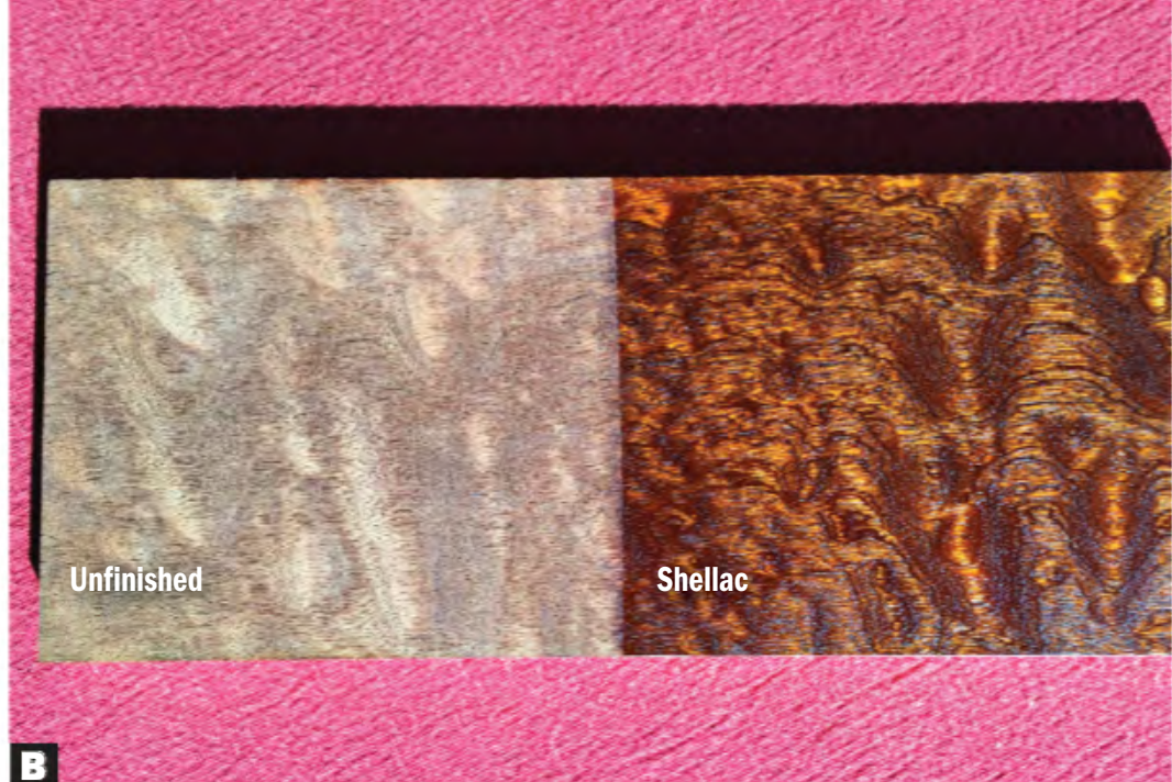
B The finish on this sample of figured bubinga veneer shows how well shellac (orange, in this case) enhances the look of any wood by adding color and depth.
