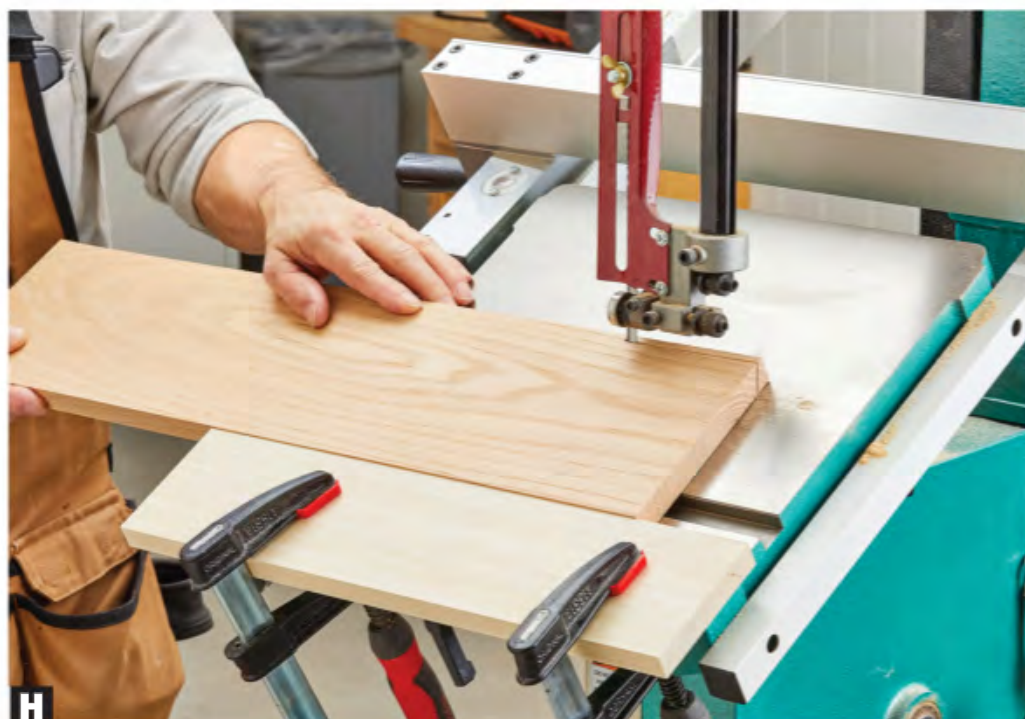
H For best workpiece stability, place the fence below the blade and bevel the edge opposite the fence. This scrapwood fence accommodates a wider workpiece than the factory-supplied fence.
