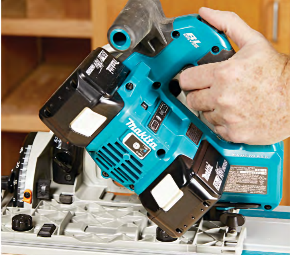
Makita's cordless saw allows plenty of hand room at the handle with the batteries installed. The other cordless saws' batteries get in the way.
