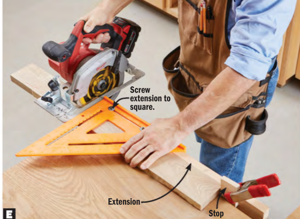
E A rafter square provides an accurate guide for crosscutting with a circular saw. Adding an extension and a stop helps you cut pieces to identical length.
