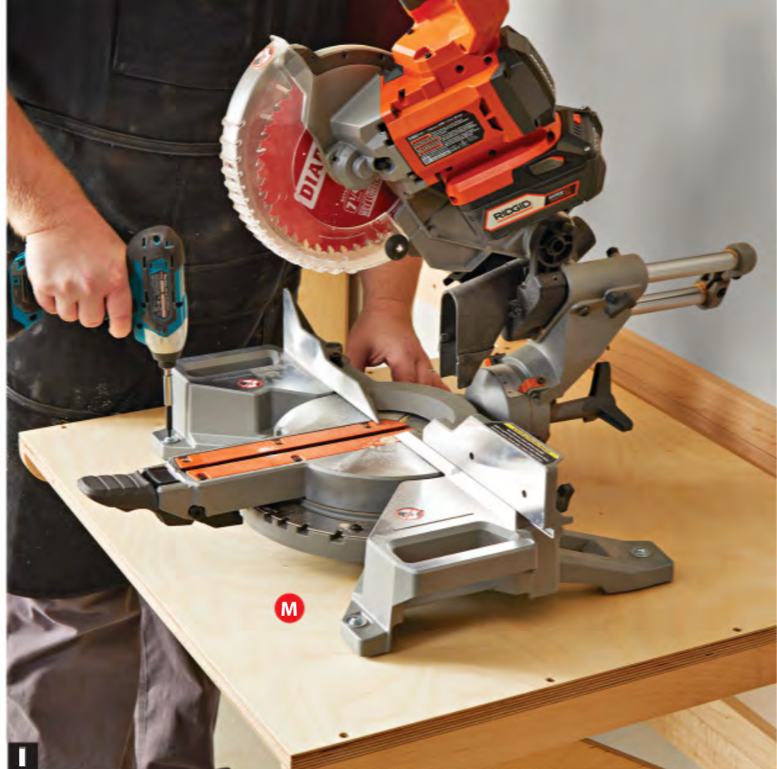
I If the saw-base mounting screws break through the platform (M), raise them slightly using washers beneath the screwheads.
