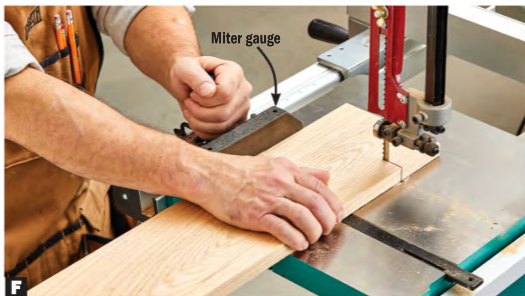
F Guide a workpiece with a miter gauge when crosscutting on the bandsaw. A stand to the side helps support long workpieces.
