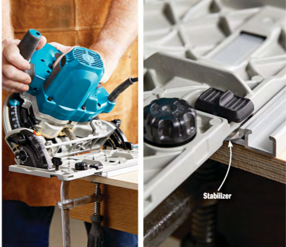
Makita’s slide-out stabilizer slips into a groove to prevent the saw from lifting off the track during beveled cuts.
