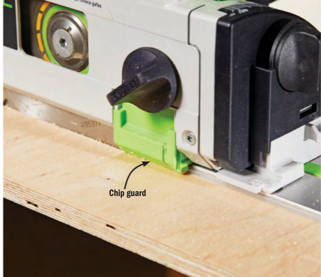
Like a zero-clearance insert on a tablesaw , Festool's replaceable chip guard prevents chip-out by holding down surface fibers at the point of cut.
