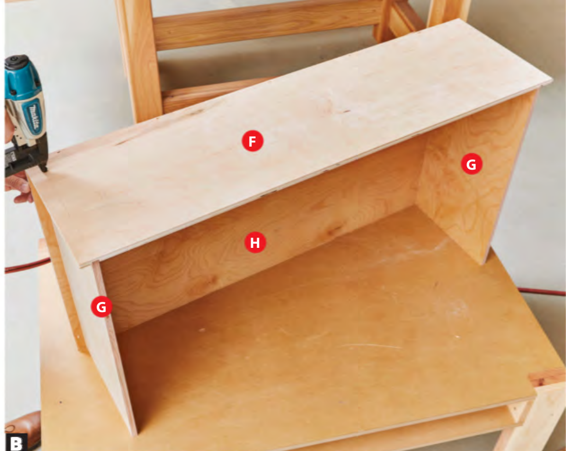
Glue the top and bottom (G) to the back (H), and secure with 1" narrow-crown staples, or #6 screws. A clamping square helps align the pieces while you work. Then glue and staple each side (F) to this assembly.
