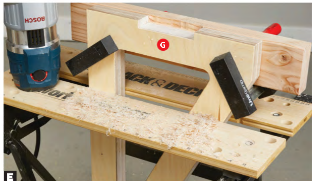
E Clamp a 2x4 to the support (G) to reduce tear-out and provide a wide surface for steadying the router. You can use the flush-trim bit or a straight bit.
