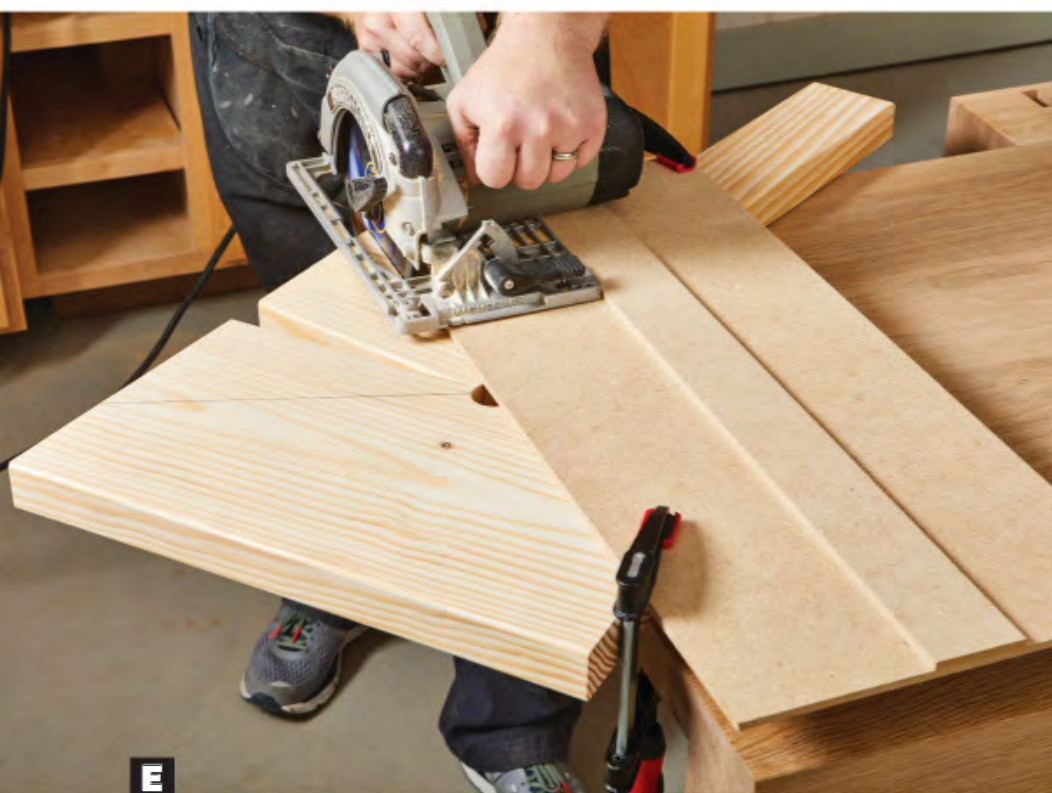
E Use the circular saw and cutoff jig to make the diagonal cuts, stopping when the top of the kerf intersects the hole. Cut away the remainder with a jigsaw.
