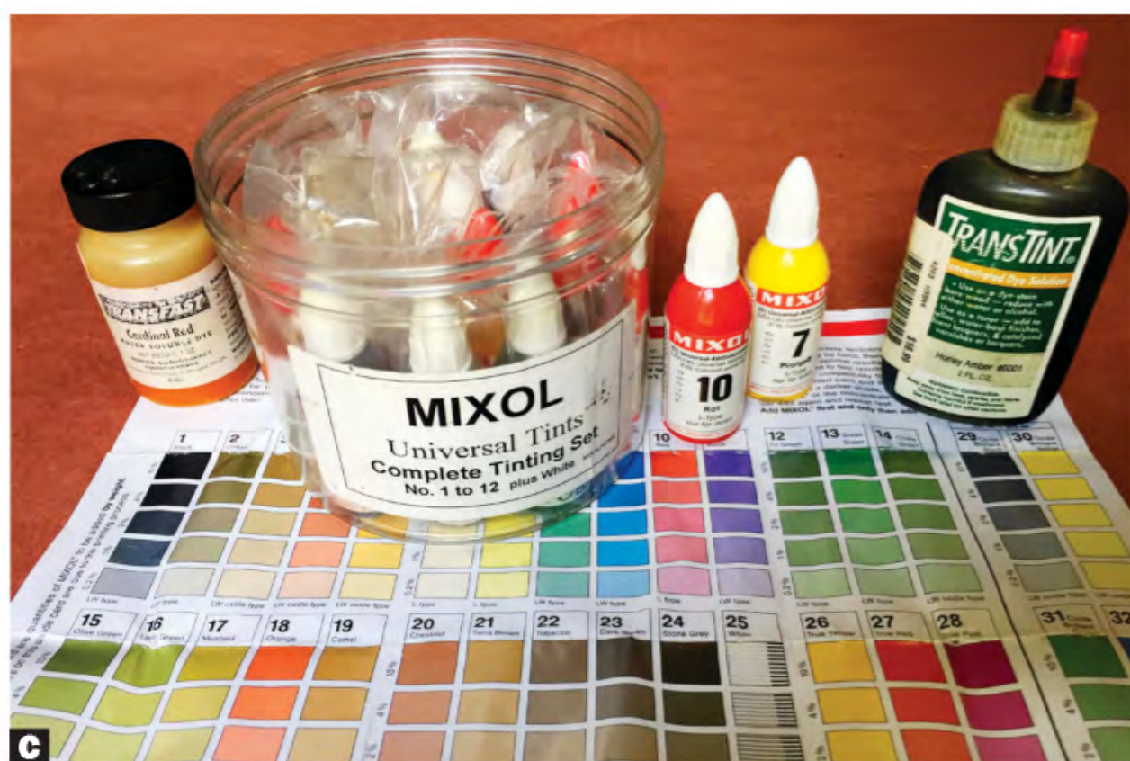
C Measure carefully when using powdered and liquid dyes or universal tinting colors (UTCs), and make more solution than you need. It can be difficult to precisely replicate a color in subsequent batches.
