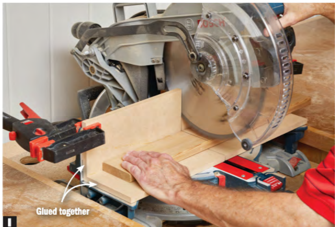
I Add an auxiliary table and fence to keep a miter saw cut clean. Buy or make a zero-clearance table insert and fence for a permanent all-angle solution.
