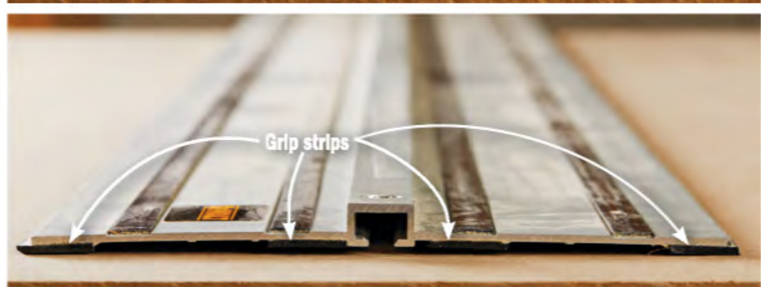
Tracks that lie flat on the workpiece, such as this Festool (top), didn't slip in use, even without clamps. DeWalt's slightly crowned track reduced the grip strips' effectiveness, requiring clamps. (A DeWalt representative said crowned tracks would be replaced under the company's warranty program.)
