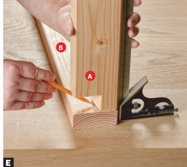
E Transfer the angle from the cut end to the inside face of the mating piece. A square helps ensure the edges stay flush as you mark.
