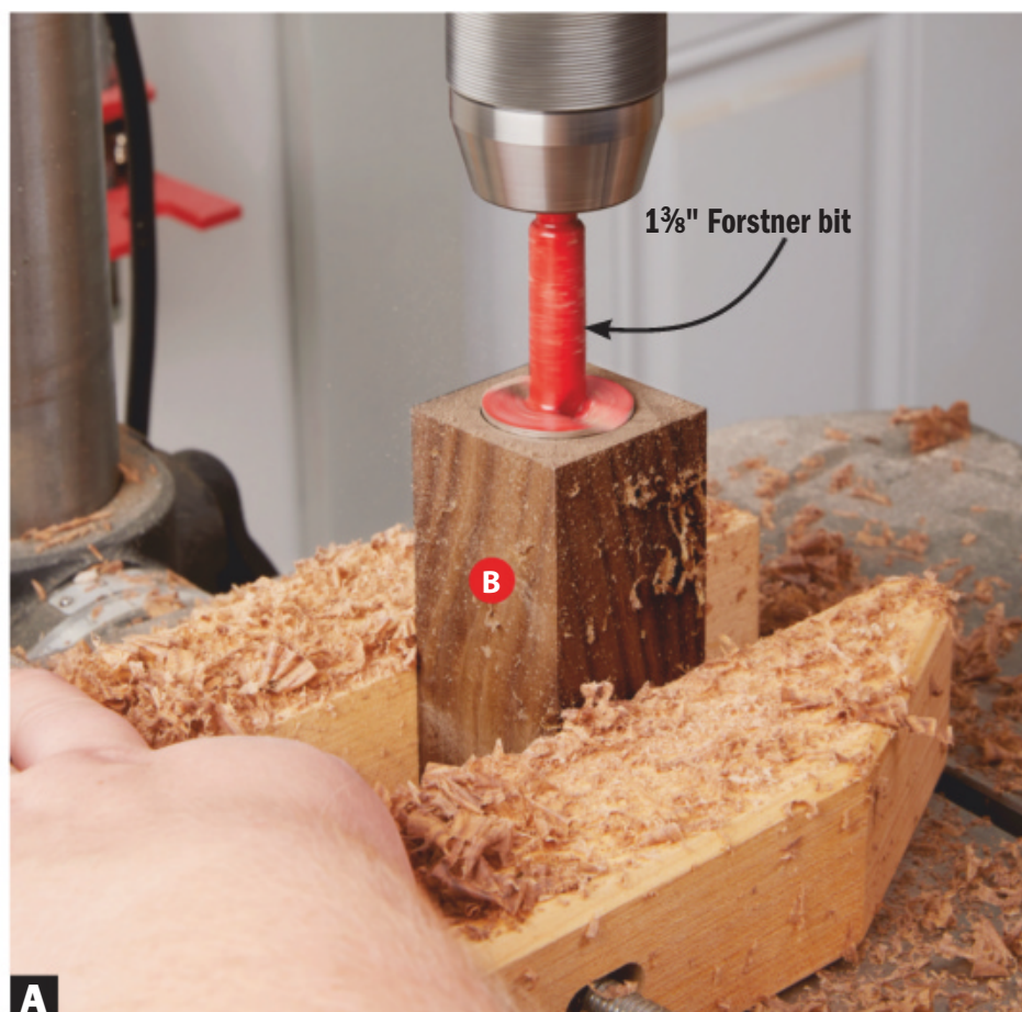
A Drill the counterbore at the bottom of each blank. Secure the blank in a clamp, with the blank aligned precisely with the bit.
