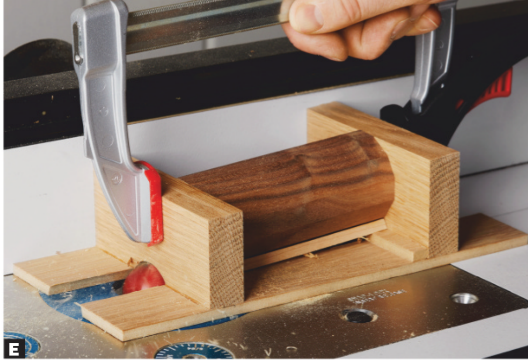
E Raise the bit until it cuts a flute the full length of the shaker blank. The flute should connect two of the 12 points at the shaker bottom.
