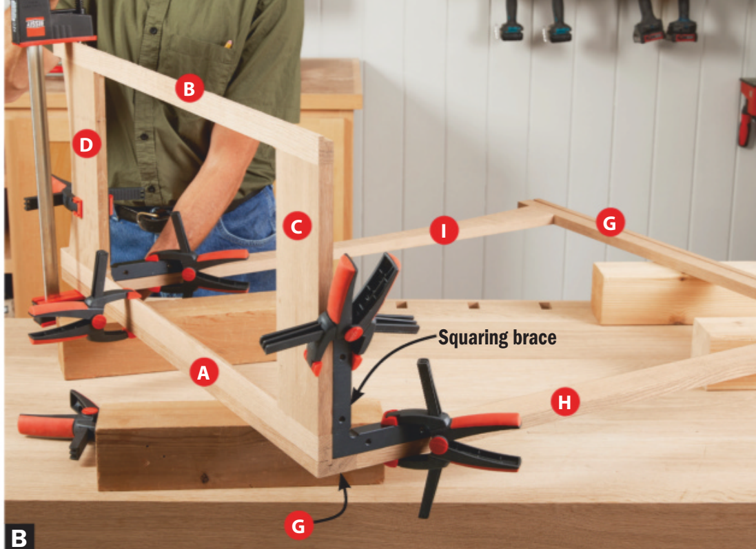
B Squaring braces orient the side and face-frame assemblies while riser blocks make room for bar-clamp heads.
