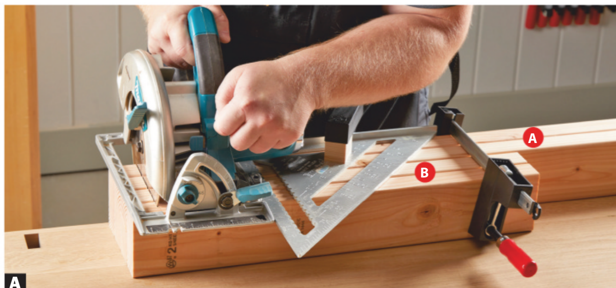
A Align the ends of the box pieces (A, B) for consistently positioned kerfs and a wide, stable surface for the saw base to ride on.
