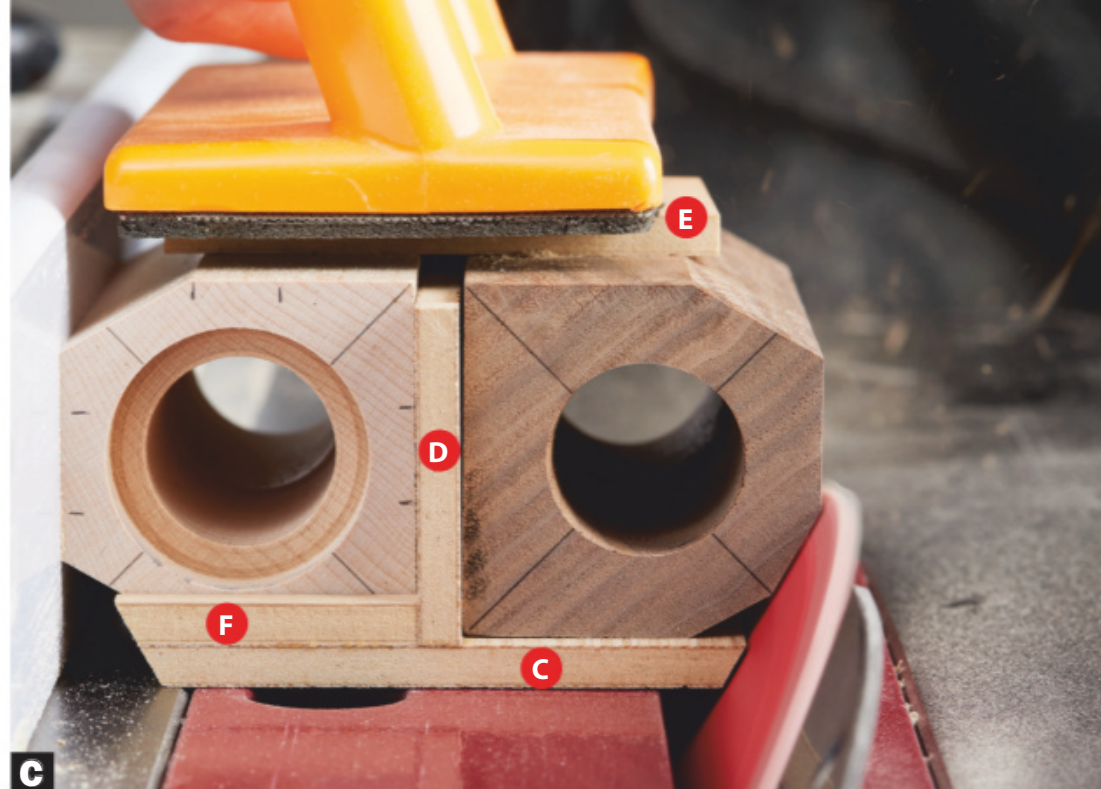
C Bevel-rip each shaker blank by keeping one of the original flat surfaces resting on the jig, and cutting to the lower layout mark on the edge over the blade. Flip the jig end for end and rip the other blank. Reposition the blanks and repeat until finished.
