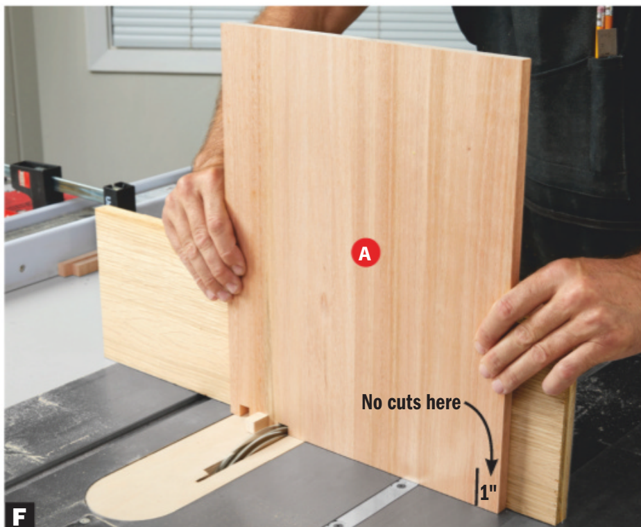
F Work your way across the width of the panel, positioning the most recent cut over the key in preparation for cutting the next notch.
