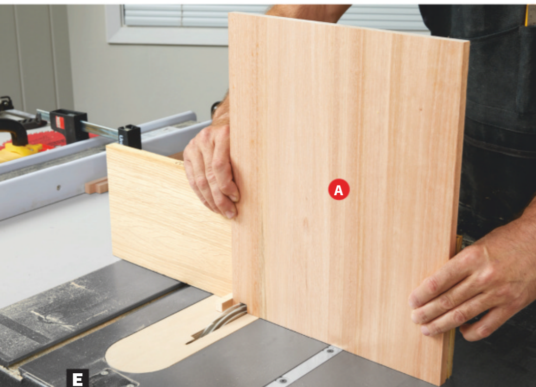
E Hold the workpiece securely against the jig as you make the first box-joint cut.
