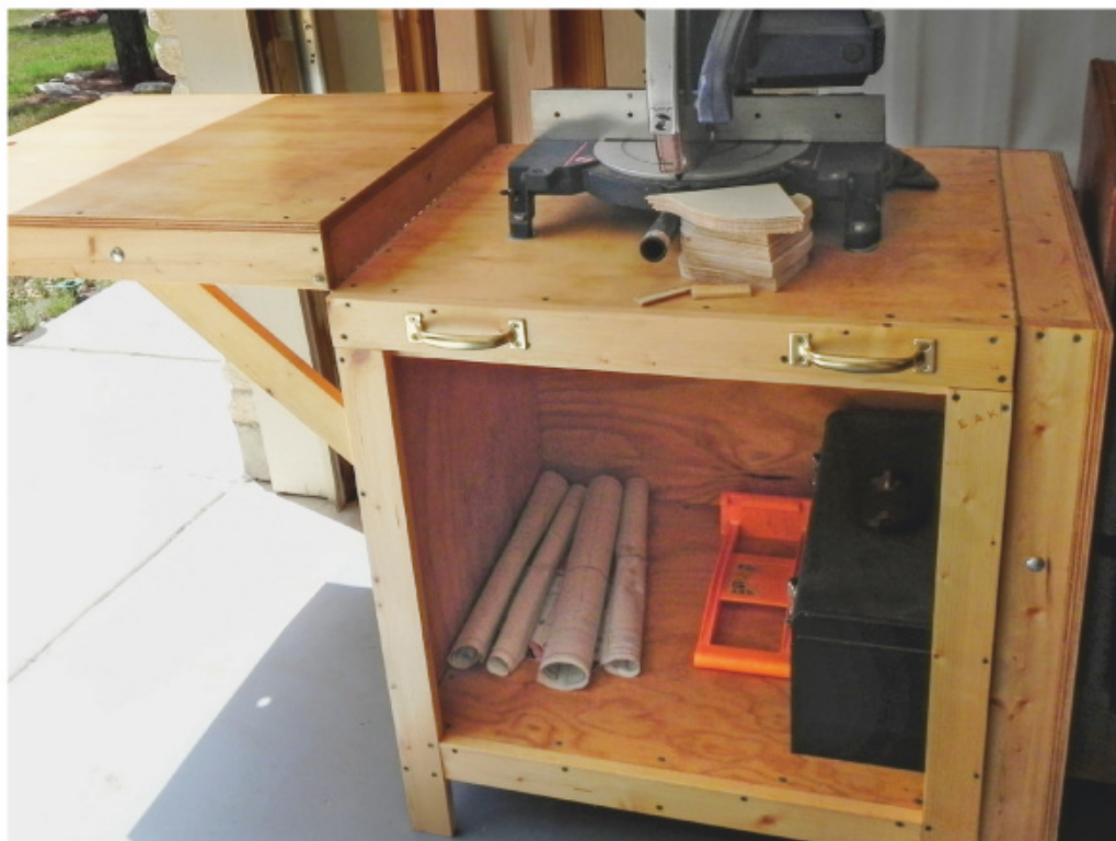
The folding wings on Ed's mitersaw station support long workpieces, then fold down for compact storage. Two casters on the back, and handles up front, make easy work of moving the workstation.
