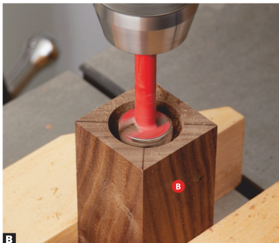
B Switch to a 1" bit and bore each blank fully through. If your bit or drill press won't reach the full depth, simply turn the blank over and drill from that end.
