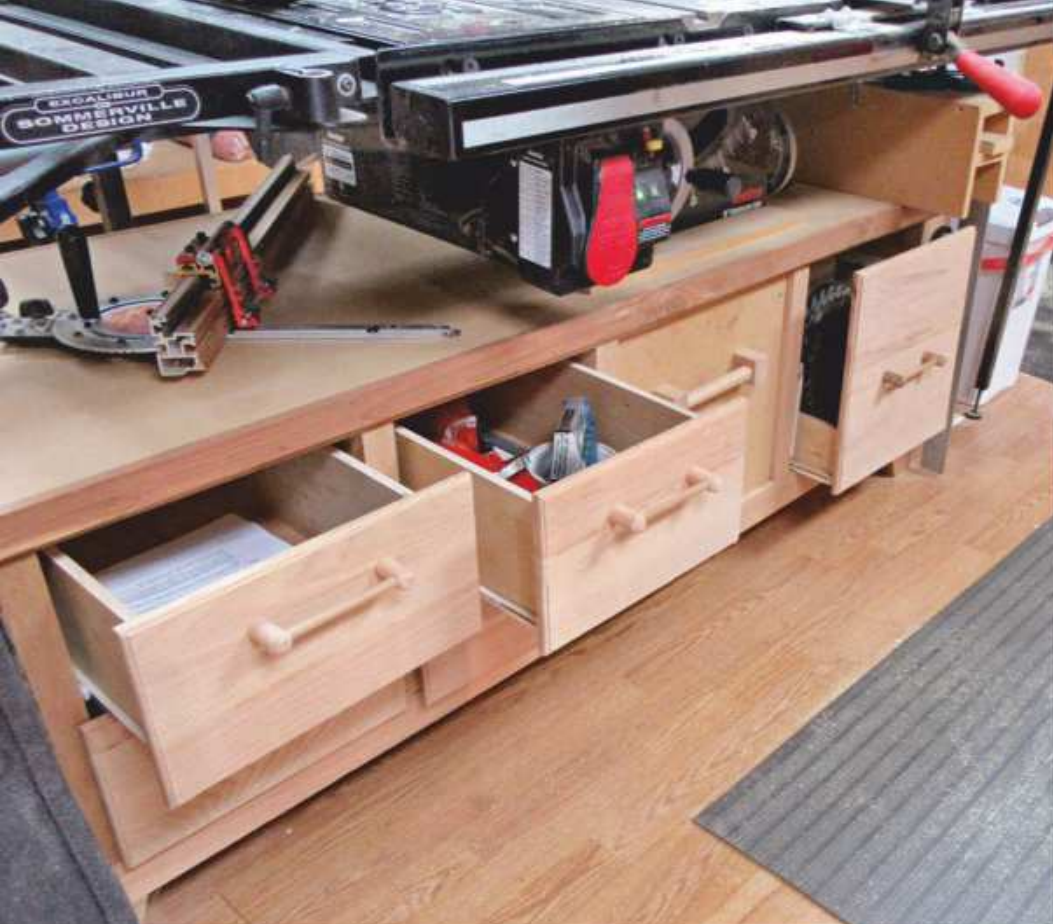
A cabinet surrounding the tablesaw base stores blades and accessories. The cabinet rolls easily on wheels lowered by foot-operated cams.
