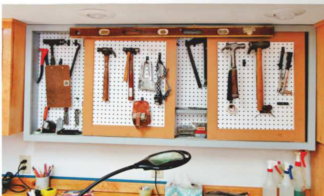
Sliding doors with pegboard panels double the storage of a wall-mounted hand-tool cabinet.
