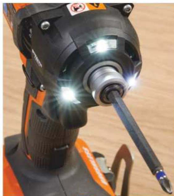
Ridgid's Stealth Force uses three bright LEDs surrounding the chuck to provide shadow-free illumination, best among this test group.
