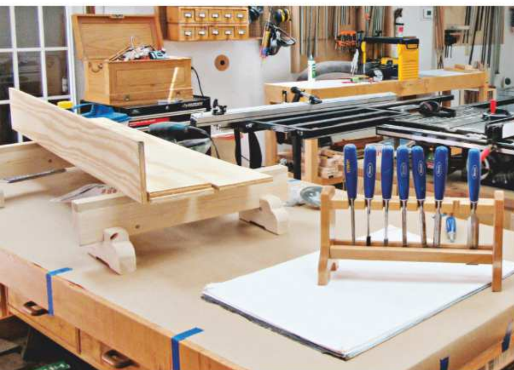
A pair of shop-made risers on Dennis' workbench make project assembly, glue-ups, clamping, and routing easier. The portable chisel rack ensures that his chisels are always at hand.
