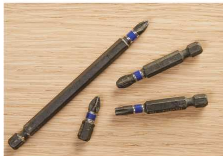
Use impact-ready driver bits with an impact driver to avoid twisting or shearing off regular bits. Impact bits are typically black in color and labeled as impact-ready.
