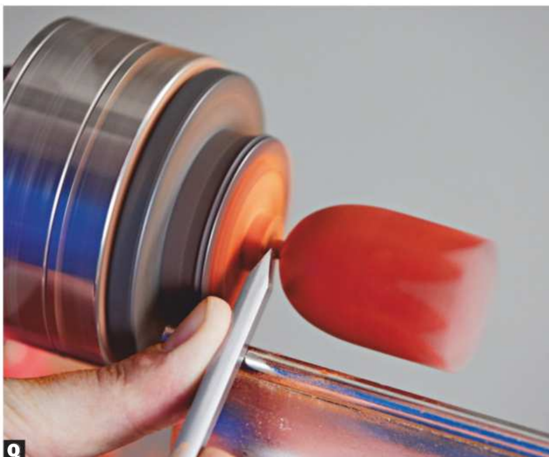
O Shape the cove until the flats disappear from the tips of the petals. Compare the profile to Pattern E .
