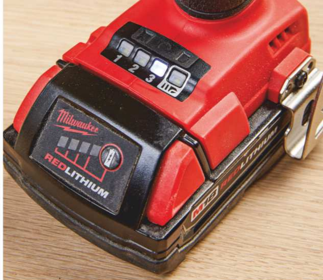
Milwaukee's Surge also has four speed settings , controlled electronically, but the battery gauge is on the battery rather than the tool.
