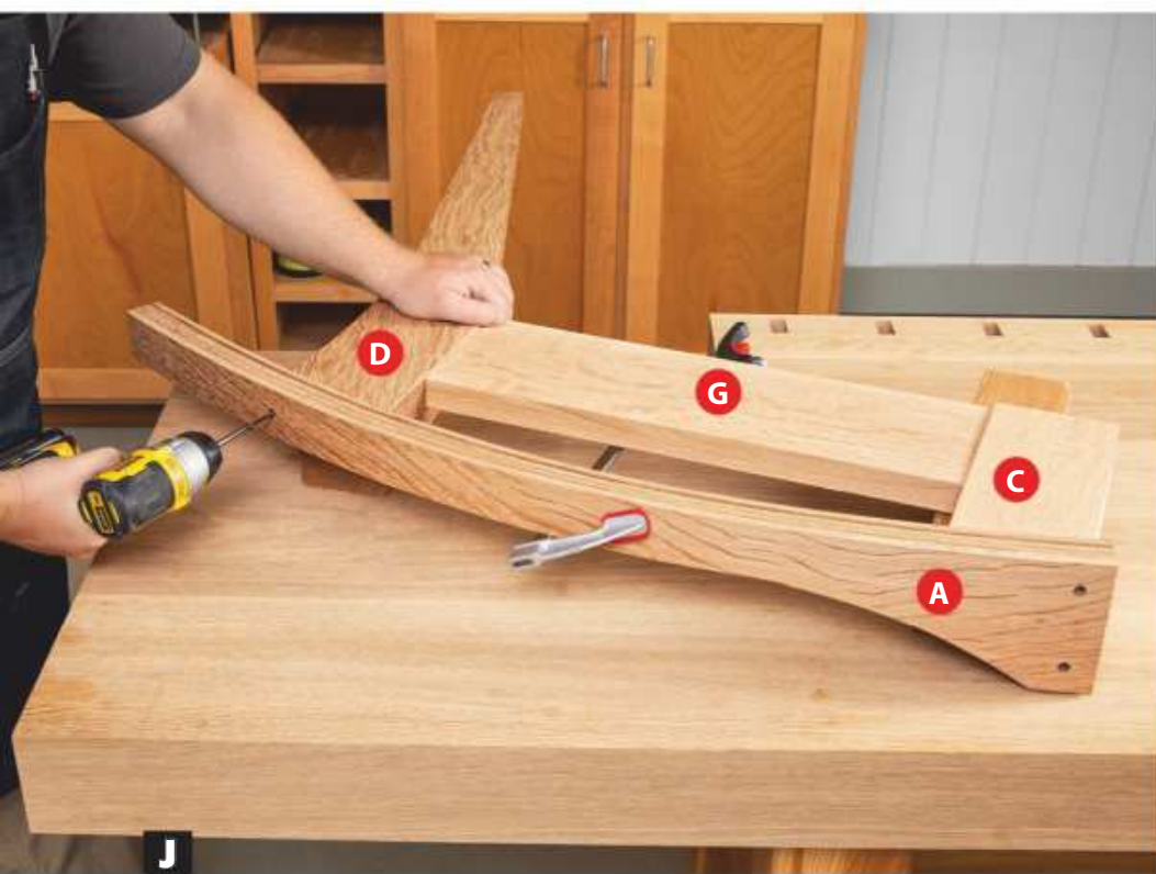
J Lightly clamp a rocker (A) to a side assembly without straightening the curve.
