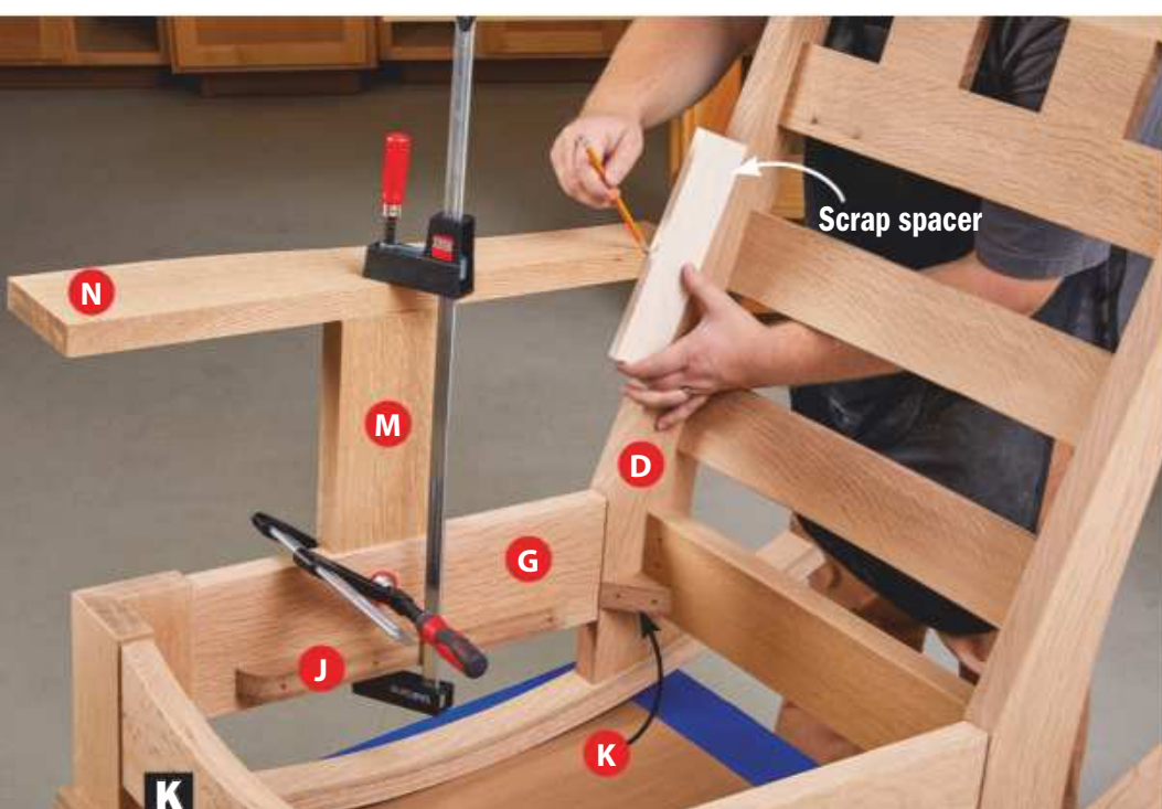
K Butt the end of the arm (N) against the edge of the back leg (D) and use a 3"-wide scrap to trace the angle of the leg onto the edge of the arm.
