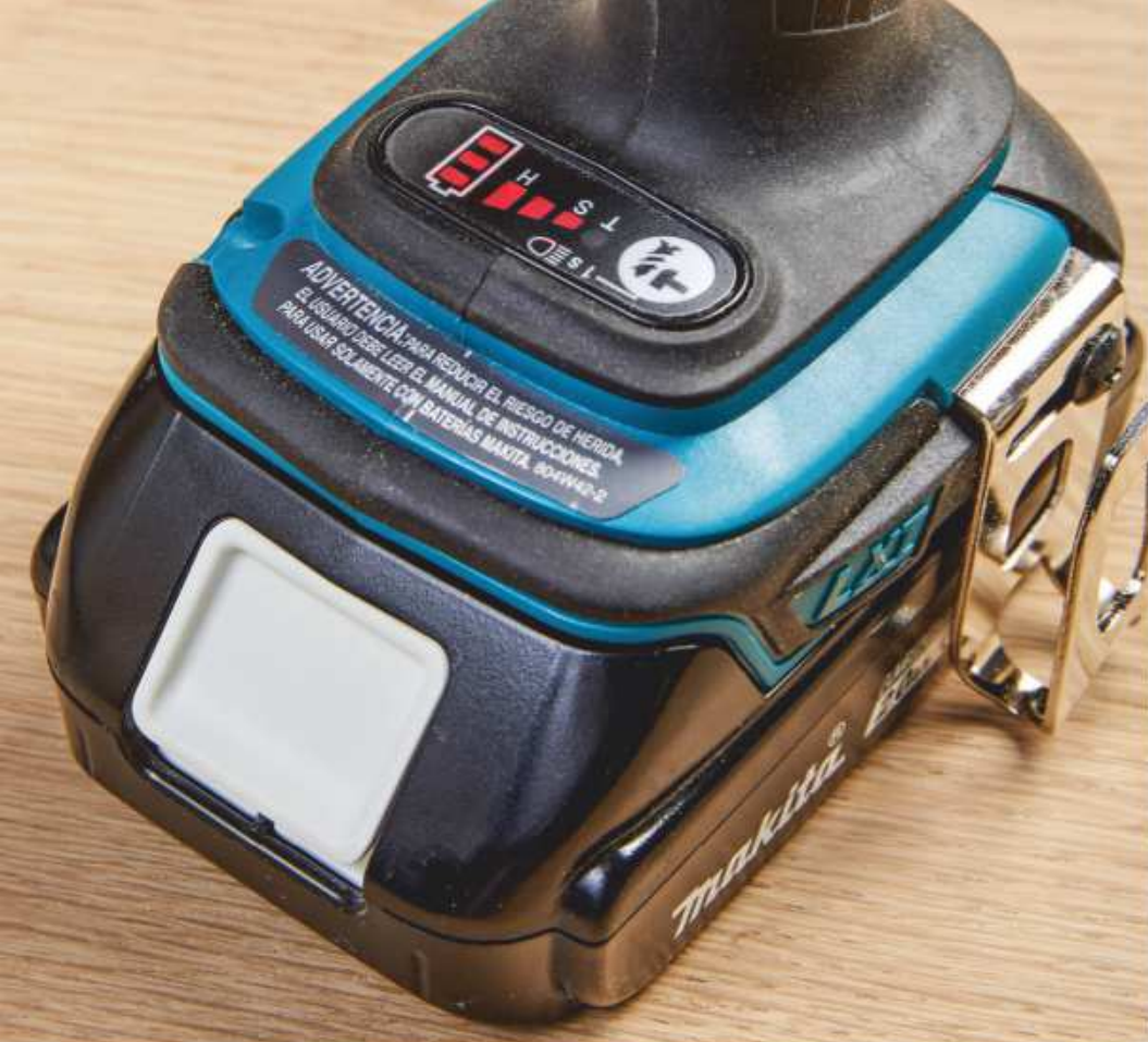
Makita's Oil Impulse driver has four speed settings , a battery-charge gauge, and an on/off switch for the LED, all electronically operated.
