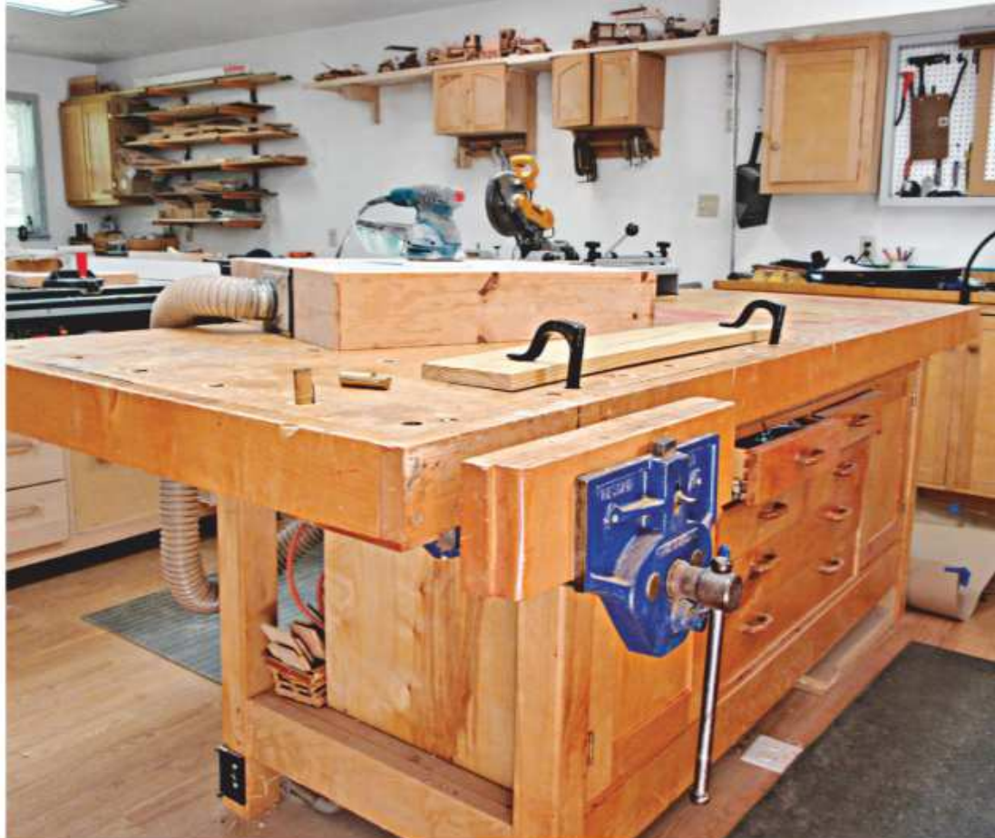
Dennis built two workbenches with solid-maple bases and two layers of MDF for the tops. The box shown on the bench above connects to a dust port in the floor, creating a sanding station. It stores on end under the wing of the bench when not in use. Cabinets and shelves underneath provide plenty of storage. A roll of kraft paper mounted at one end (not shown) allows him to cover the bench, protecting it from glue and finishes.
