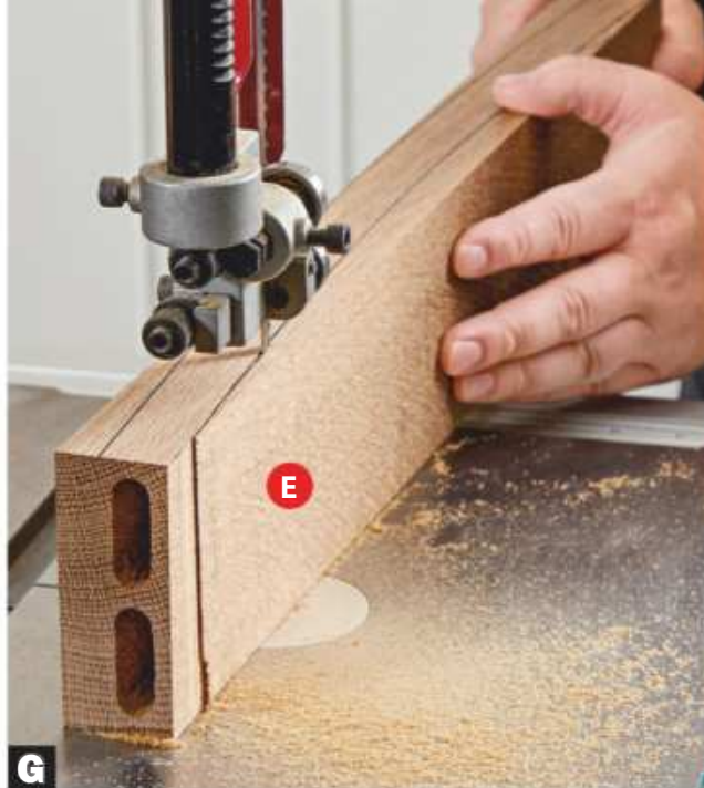
G Contour the back slats (E) after boring mortises for the floating tenons.
