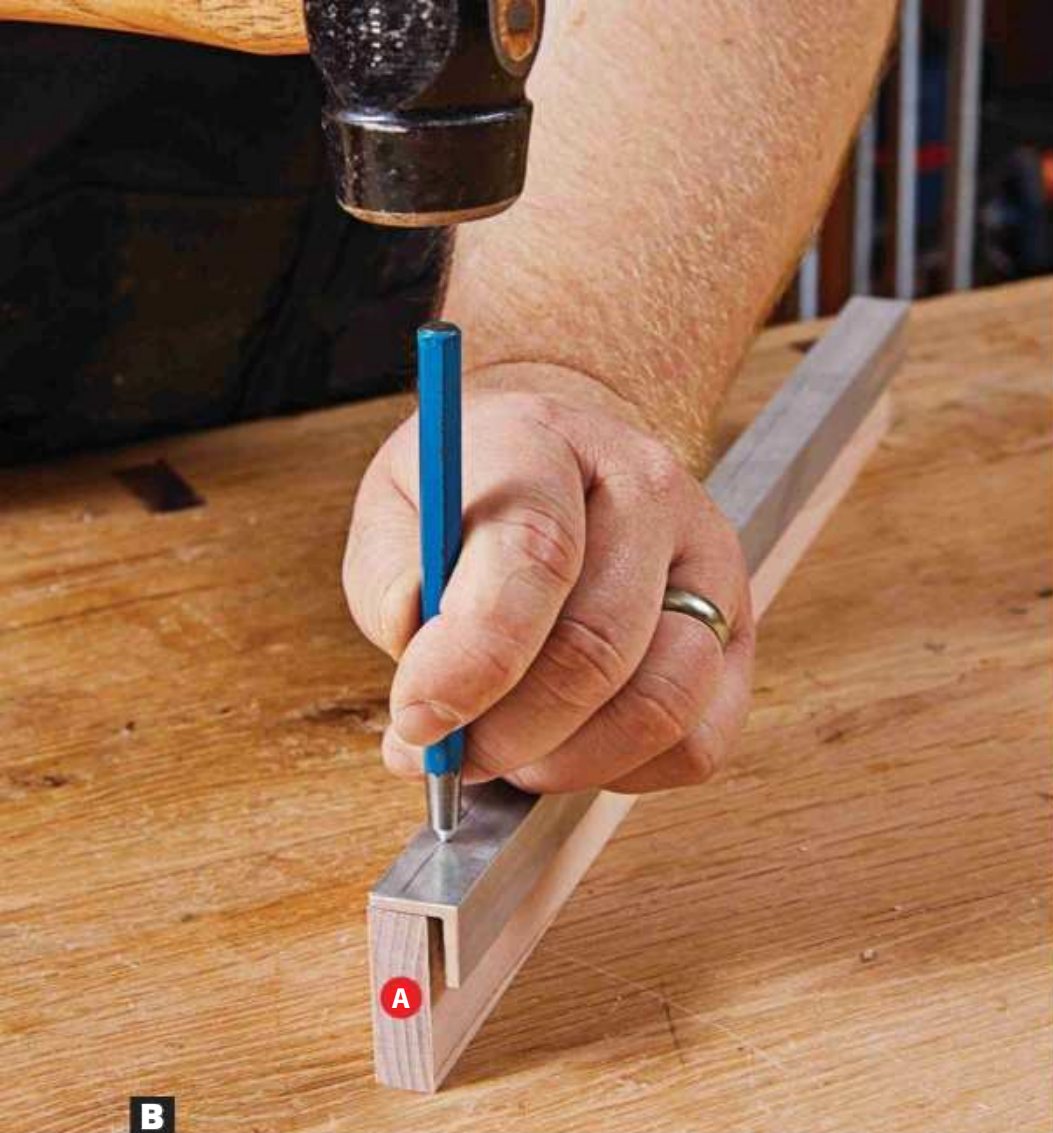
B Punch dimples at each screw location to prevent your drill bit from wandering.
