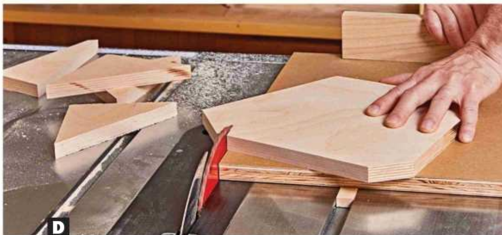
D Repeat this process to cut each of the remaining corners, creating a blank with 16 edges. One more series of corner cuts makes the blank nearly circular.
