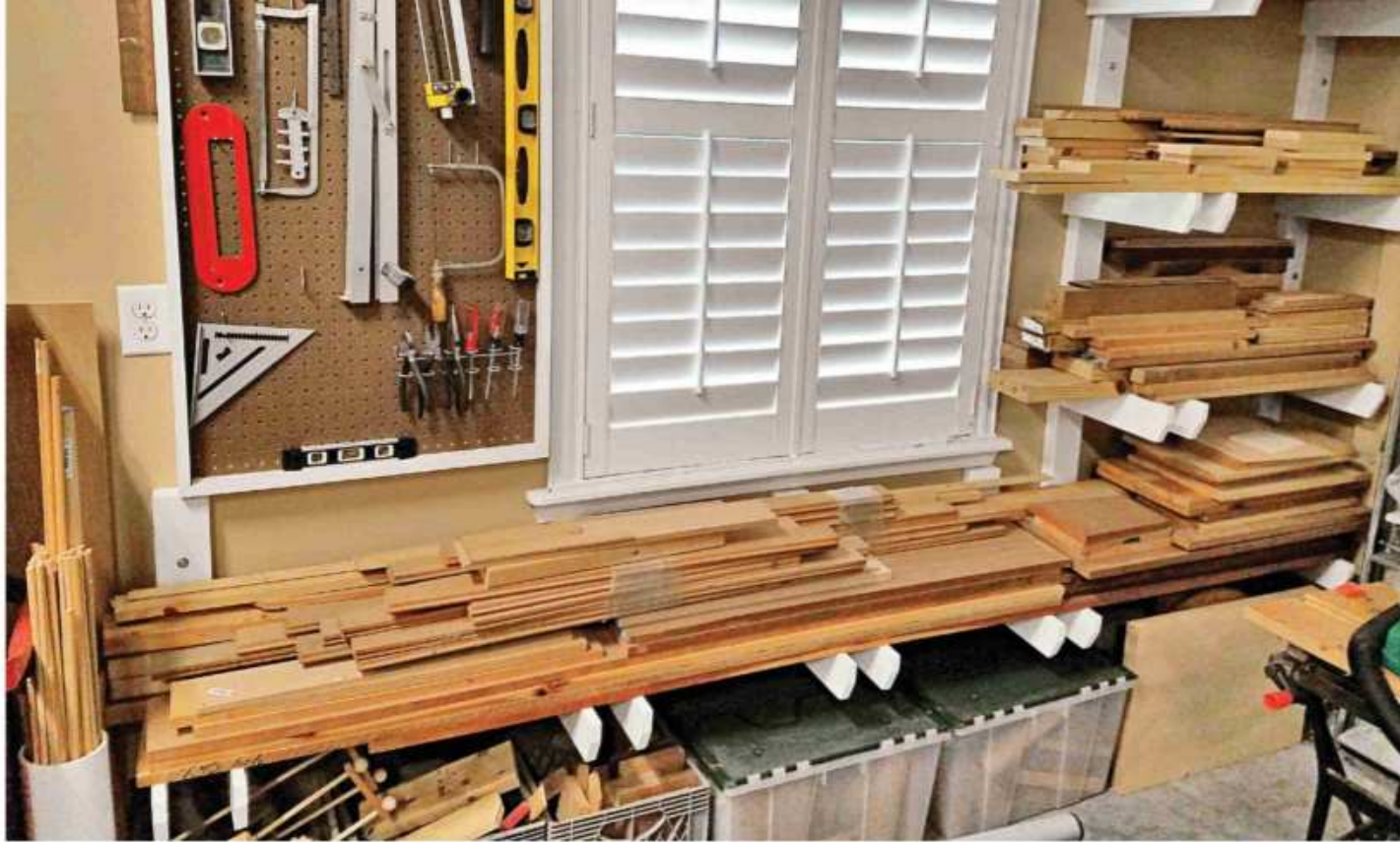
Racks built from 2x4s and 1x4s hold longer boards for Andy's projects. Totes and bins below collect smaller cutoffs. Dowels store in a vertical section of PVC pipe.
