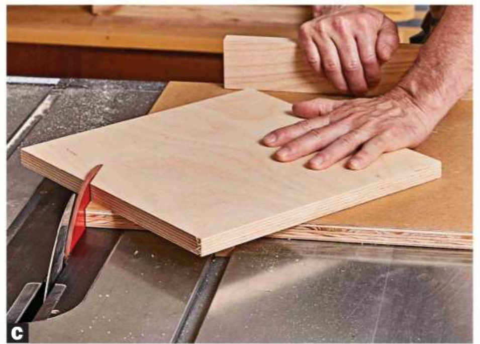
C Cut away a corner, then turn off the saw. When the blade stops, pull the jig back to the start. Rotate the blank 90^\circ and repeat to cut away each of the three remaining corners.
