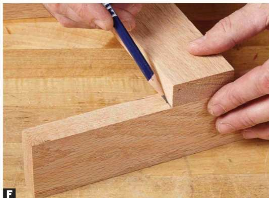
F Mark the dado edges using the mating piece to be rabbeted. If needed, place a center mark on the end of the rabbet part to align with a center mark on the dado part.
