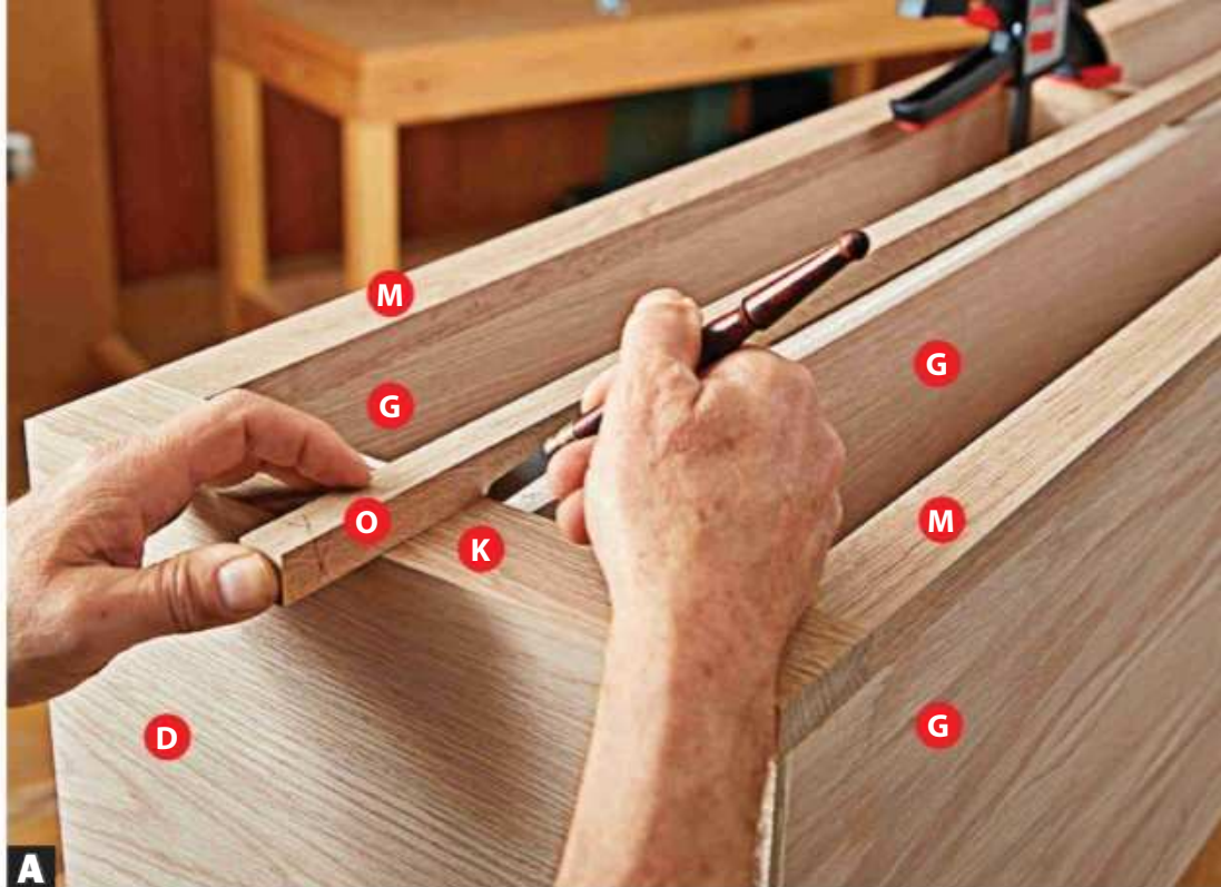
A Position the middle rail across the face frame and mark the length with a knife for maximum precision. Mark the stile for the center cabinet the same way.
