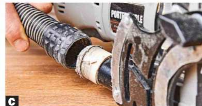
C Go bigger with a few layers of tape. Most any tape will do; we enlarged this biscuit joiner's port with masking tape, applying enough for a good friction fit.
