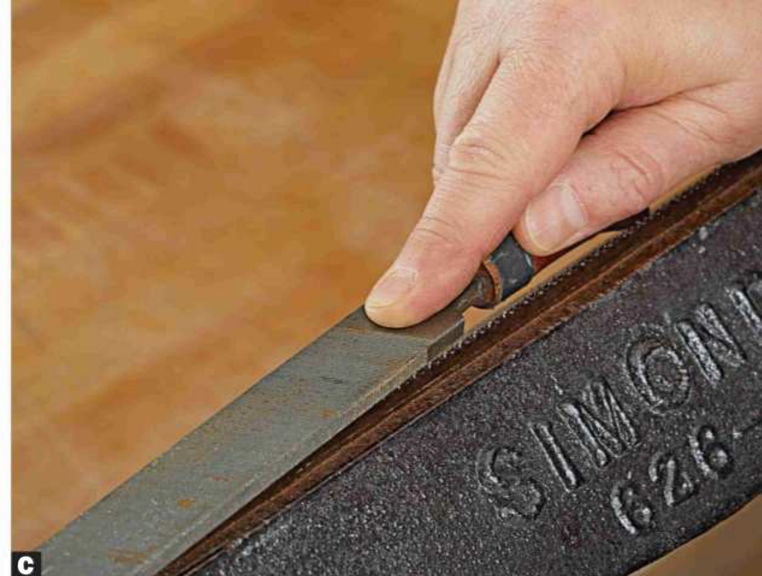
C Make a single light pass from the heel to the toe when jointing the saw. An out-of-joint saw may have been improperly sharpened.
