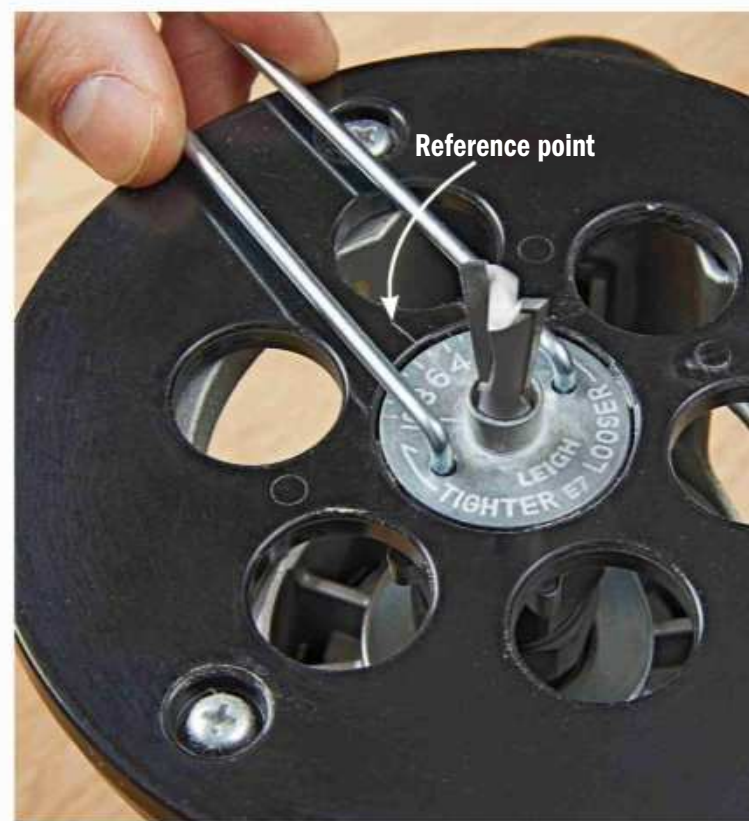
The slightly elliptical guide bushing on Leigh's jigs lets you fine-tune a joint's fit by rotating it a few thousandths of an inch. But you must hold the router in exactly the same orientation with each cut.
