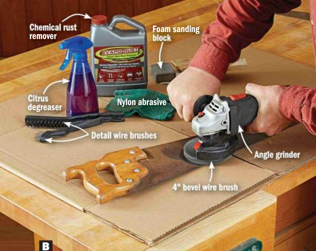
B An angle grinder with a bevel wire brush cleans up a rusty saw quickly. Work in short bursts over large areas to prevent heating the blade and affecting the temper.
