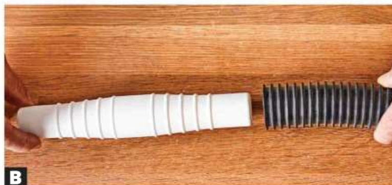
B A pool-hose connector gets the job done. When using a connector that goes inside the hose, cut off any excess at either end to lessen air resistance. Find the connector at swimming-pool suppliers or woodmagazine.com/hoseconnector .
