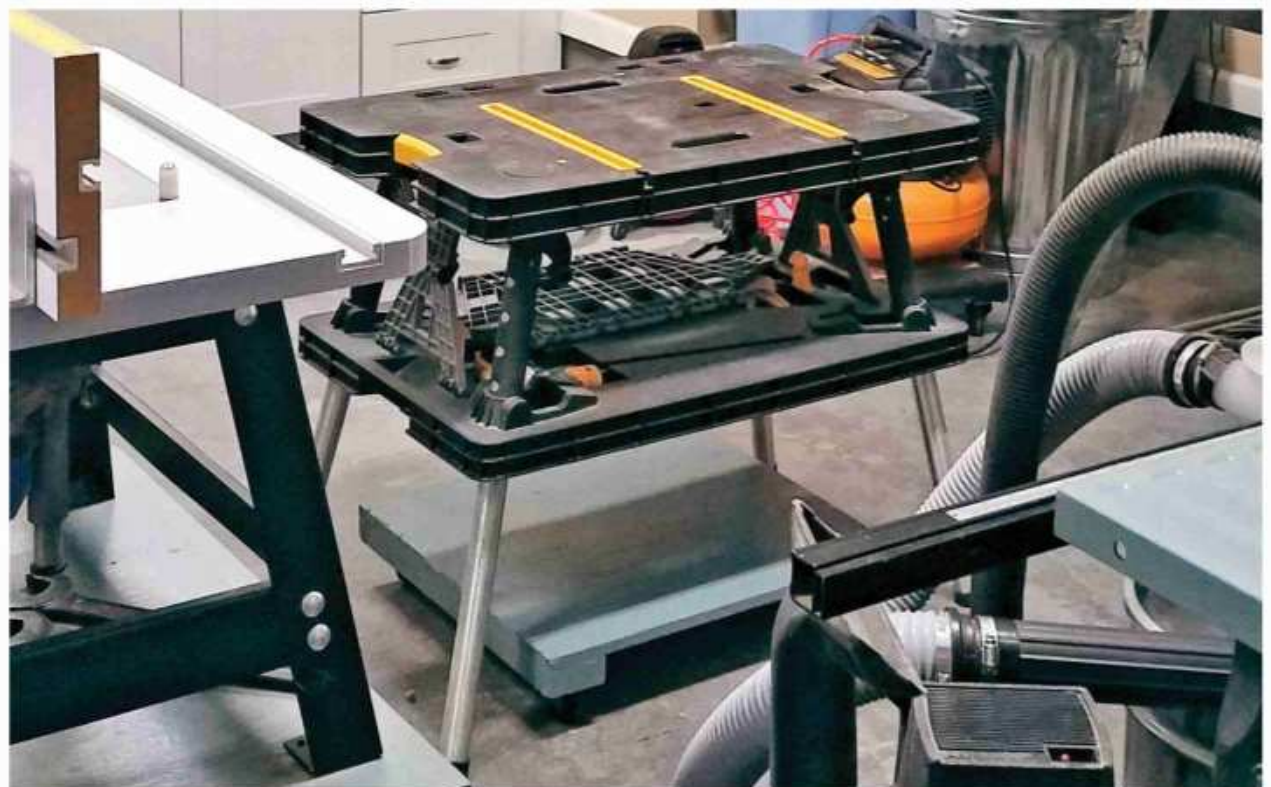
A folding worktable serves as the main worksurface for clamping and assembly. It provides a variety of clamping options for workholding.
