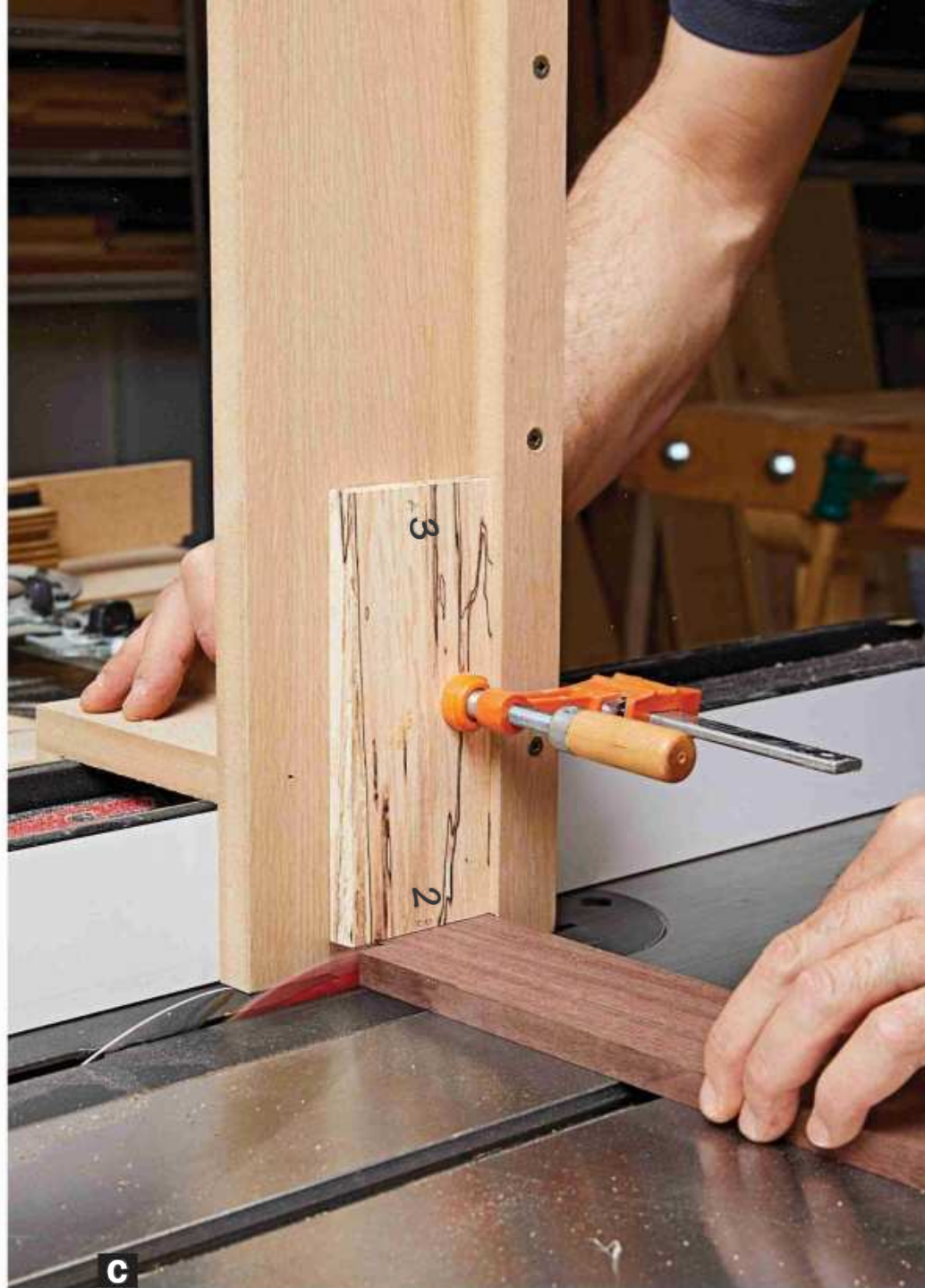
C Clamp the side/corner blank assembly to a rip-fence saddle jig and cut the corner (C) free from the blank.
