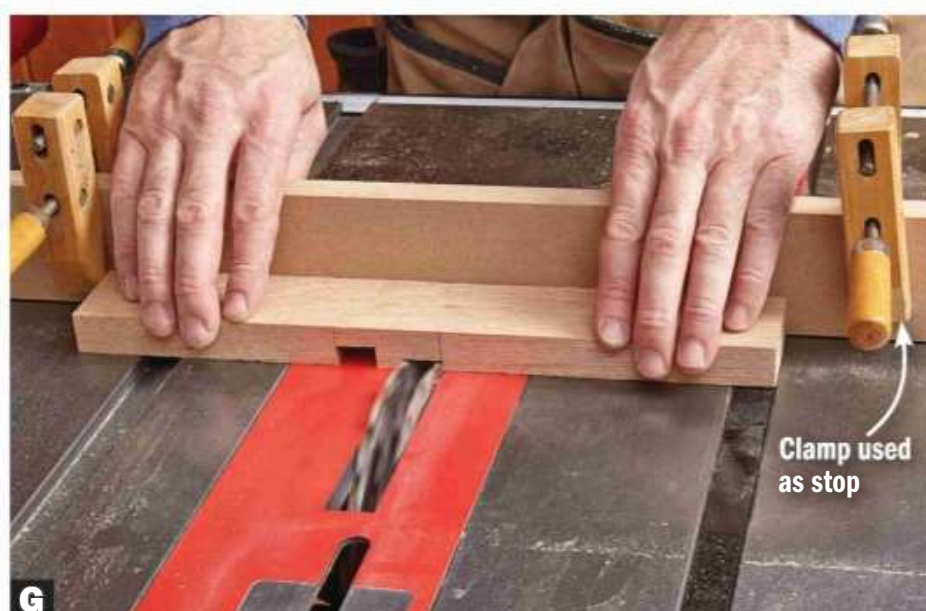
G Stops added to an auxiliary fence simplify duplicate parts, such as the top and bottom rails of a two-door cabinet face frame.
