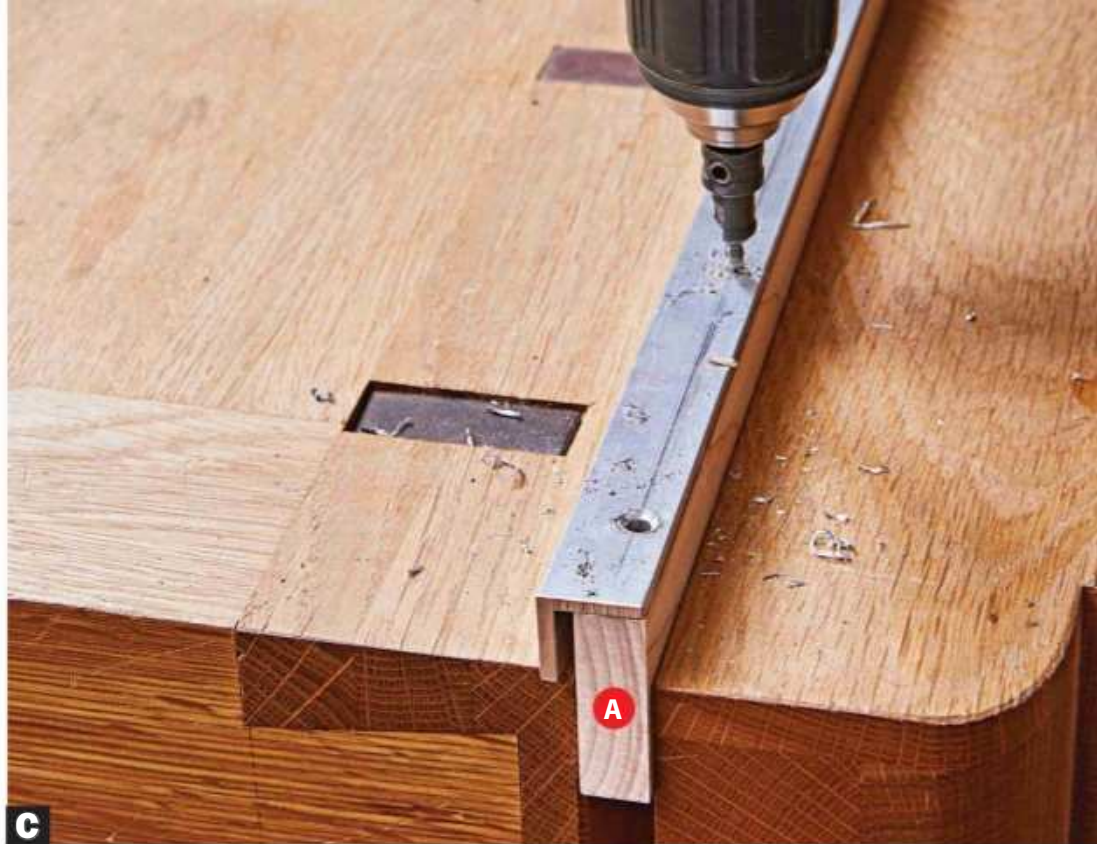
C Countersink each screw hole so the screwheads sit flush with, or just slightly below, the surface of the aluminum angle.
