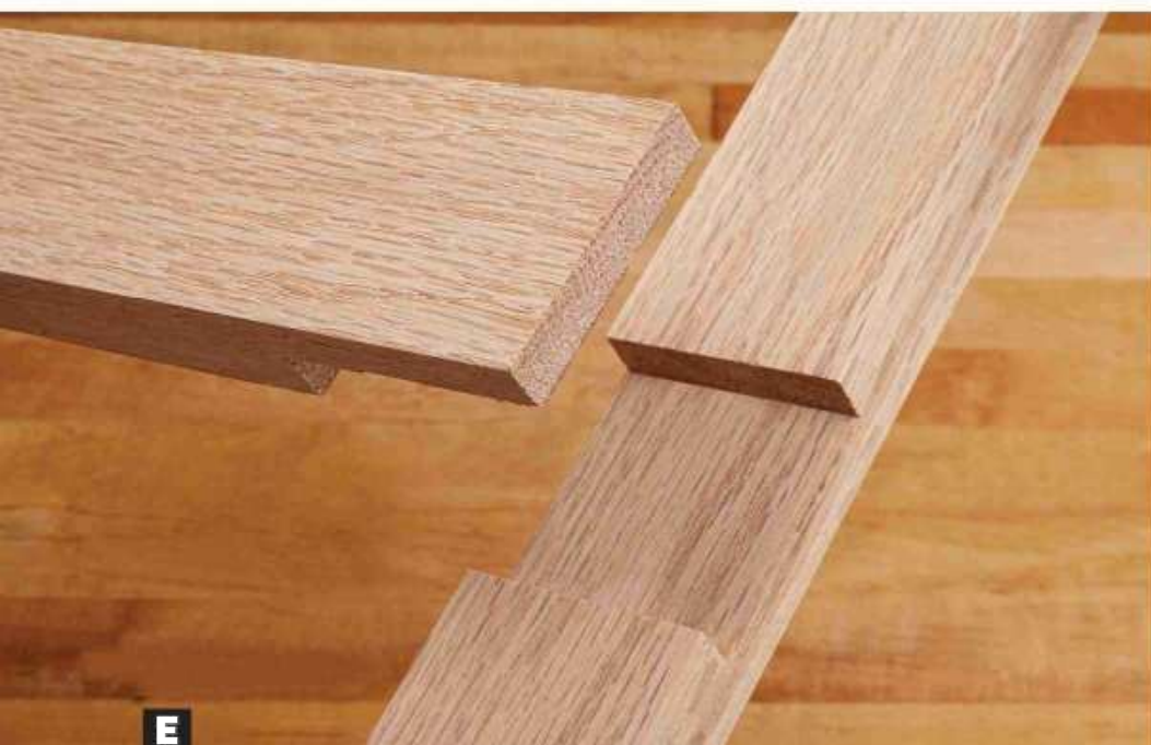
E Half-lap T joints automatically align to form 90° angles when the dado is cut to the width of the rabbeted piece.
