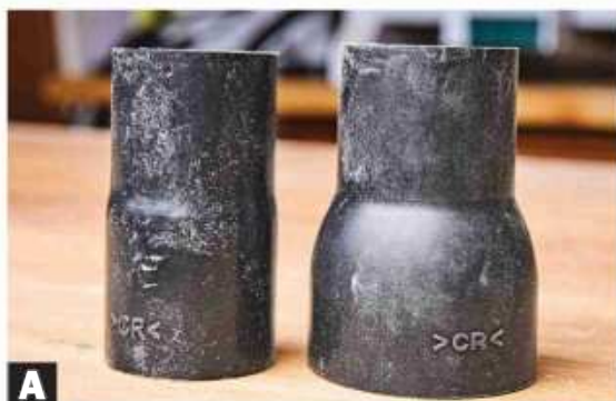
A Rubber adapters stretch to grip tightly. These two adapters (nos. 192407 and 192408, highlandwoodworking.com ), have respective diameters of \frac{19}{32} ×1 \frac{1}{8} " and 1 \frac{11}{16} ×1 \frac{1}{8} ".
