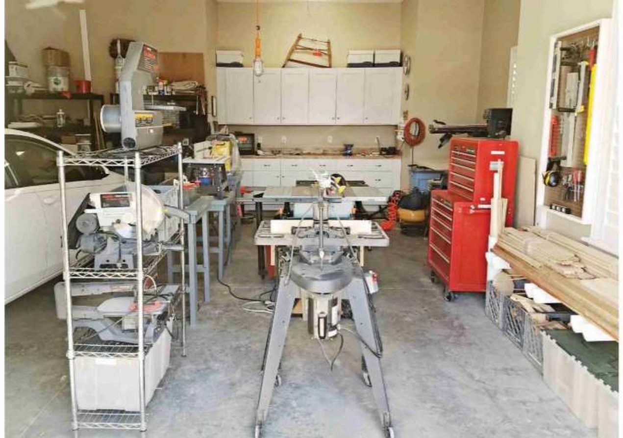
A bumpout in the back of the shop created an ideal location for cabinets and a countertop for additional storage and workspace. The radial arm saw and drill press tuck away in a second bumpout in the side wall.
