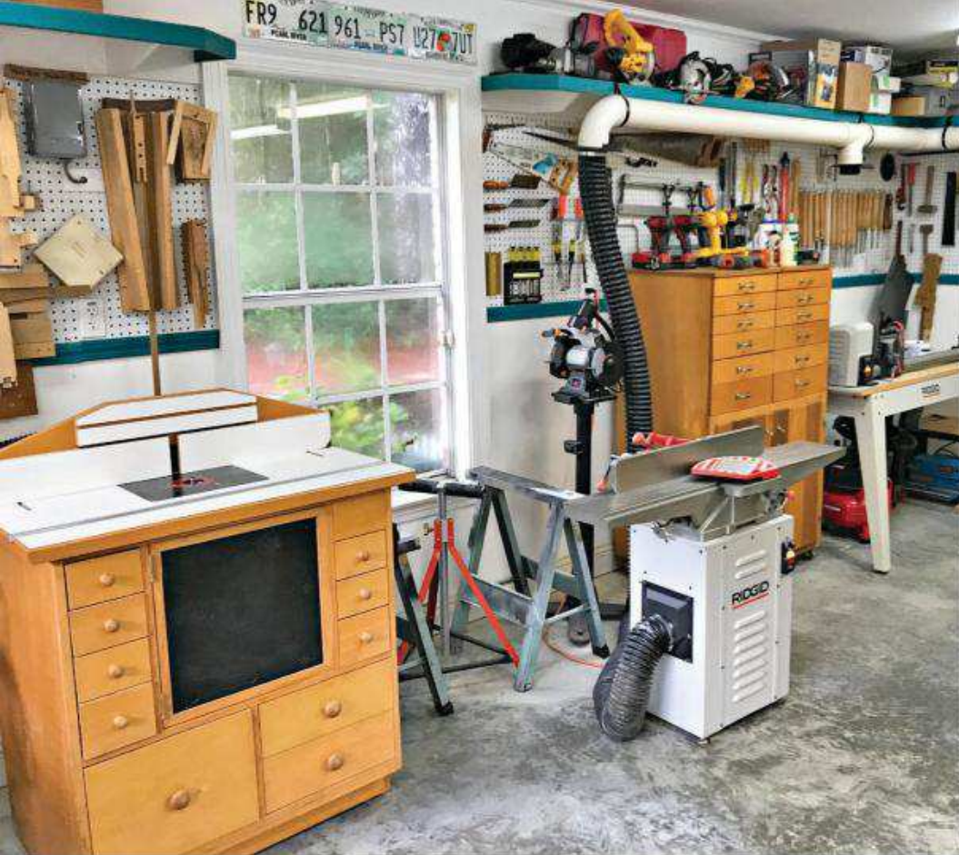
Pegboard running around the perimeter of the shop provides plenty of options for hanging tools and jigs at a convenient height.
