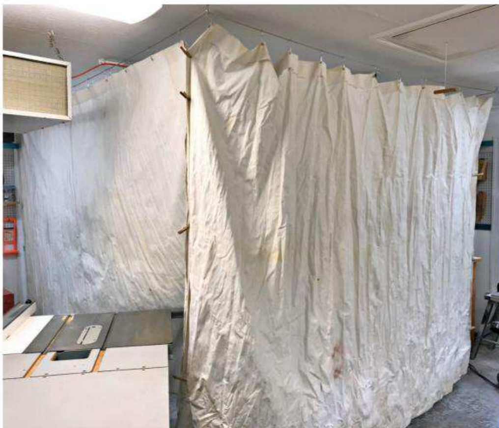
Canvas "walls" form a convenient temporary booth for spraying finish.
