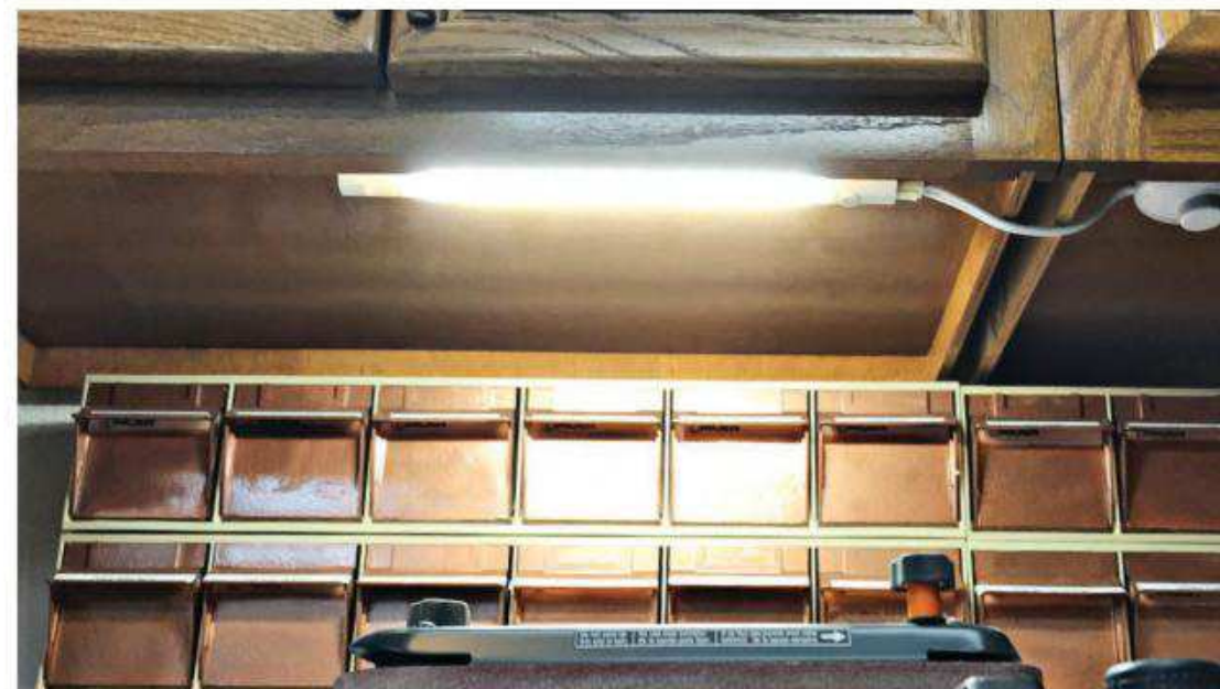
A small LED mounted under a cabinet illuminates storage bins below it as well as a benchtop sander. This light has an easy-on/off touch switch.
