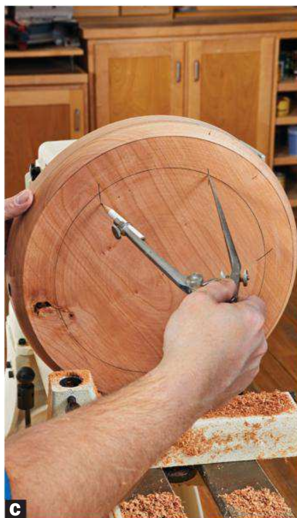
C Lay out a 10"-diameter circle. Without adjusting the compass, place the point on the diameter, and make a mark along the line. Move the compass point to the new mark and repeat until you have six marks. Make an indentation at every other mark with a spring punch.
