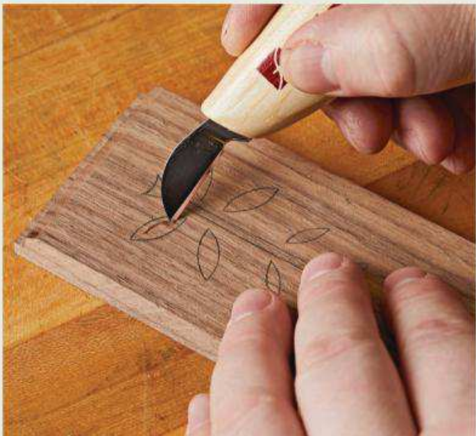
Make a cut inside and parallel to the pattern line. Start shallow, increase pressure to cut deeper in the middle, and finish shallow.
