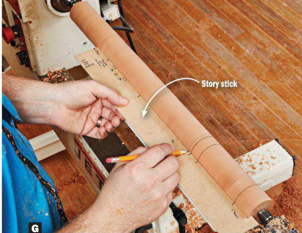
G To mark lines 1–11 , make an 18"-long story stick with a short hook on the right end to register against the end of the leg. Handsaw a short kerf at each of the eleven dimensions shown in Drawing 2 .
