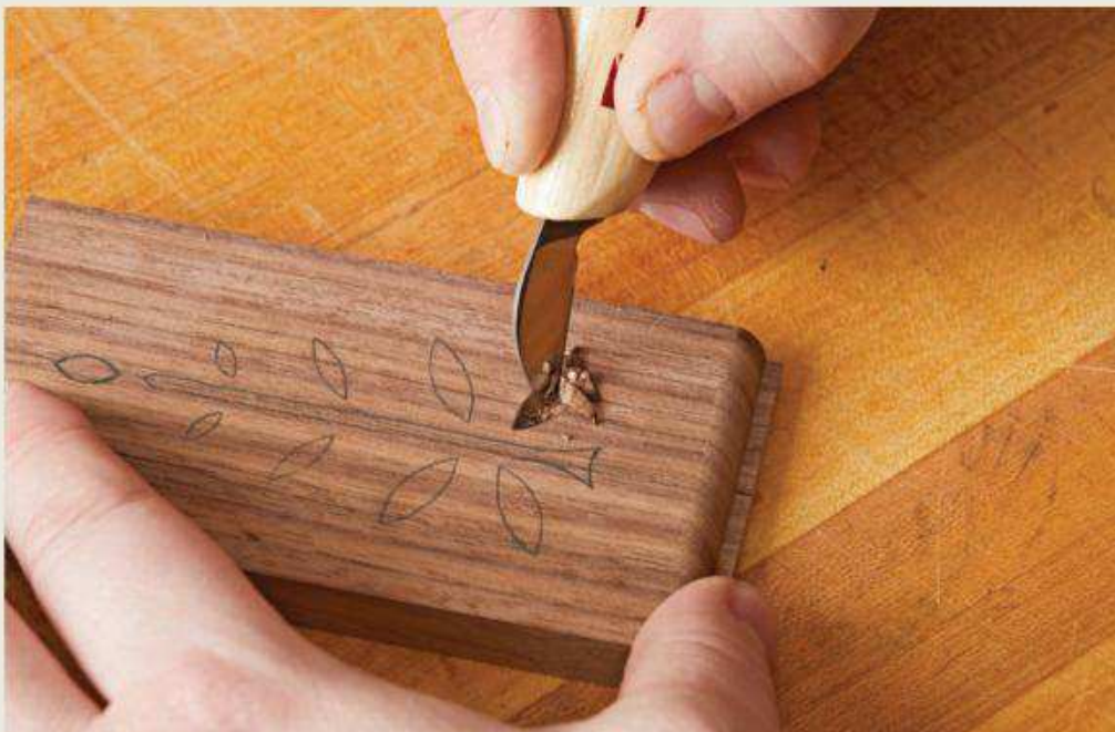
Make multiple concentric cuts, working from the center of the carved element to the pattern line, rotating the workpiece as necessary.
