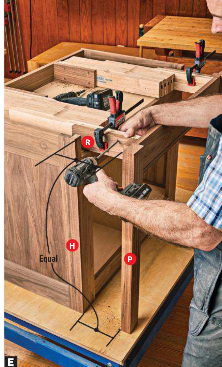
E Fasten the table slides to the slide blocks (R) with a single screw at the top front. Make the space between the stiles (H) and legs (P) equal at top and bottom, and drive the remaining screws.
