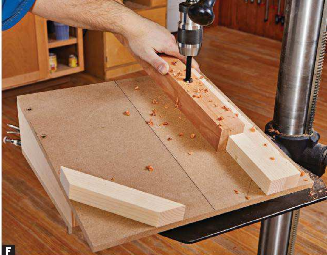
F Reposition the jig. Center each leg under a ¾" Forstner bit, and drill 1" deep, measuring to the deepest portion of the hole.
