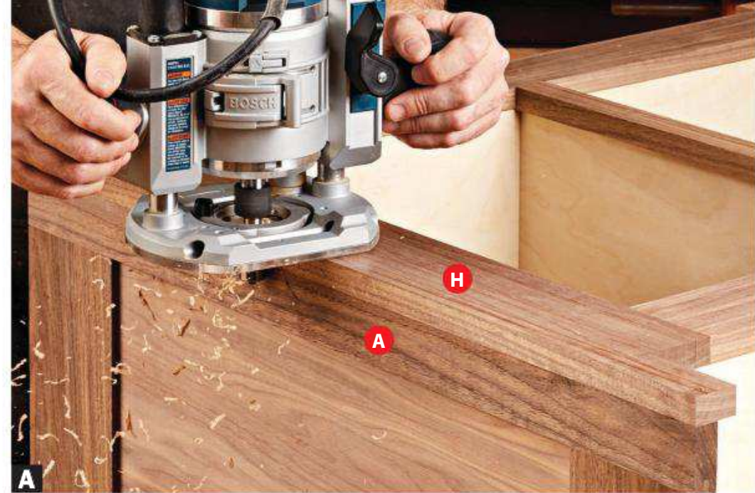
Trim the face-frame stile (H) overhangs flush with the side assembly stiles (A), using a flush-trim bit.
