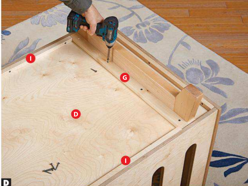
D Butt the extended portion of the base cleats (G) against the side cleats (I). Screw the base cleats to the bottom.
