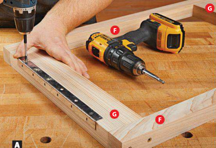
Fold the hinge leaves over the edge of the leg rail (G) for positioning, which is the same on both leg assemblies. The side of the hinge leaf with countersunk screw holes faces up.
