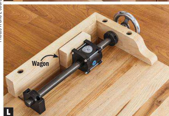
A wagon vise moves within a closed channel to secure workpieces between bench dogs. The wagon attaches to the mechanism that rides along the vise screw, moving the wagon along with it.
