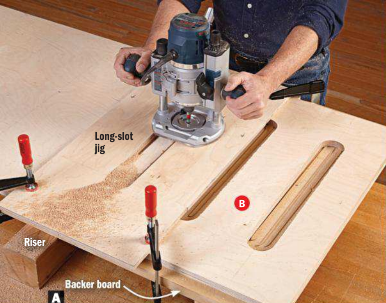
A Clamp the slot jig to an end (B) and a backer board, with the cleat against the bottom edge. Risers create room for the clamp heads.
