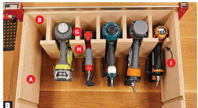
B Position the holders and nail guns so that each gun fits snug enough between them to stay in place, yet still removes and replaces easily.
