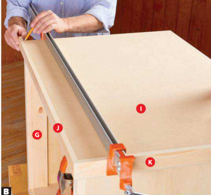
B Miter one end of each molding (J, K) and clamp it in position while you mark where to miter-cut the opposite end.
