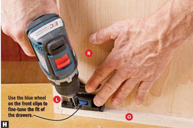
H Position the under-mount drawer-slide clips snug against the drawer sides (L–N) and drill pilot holes.
