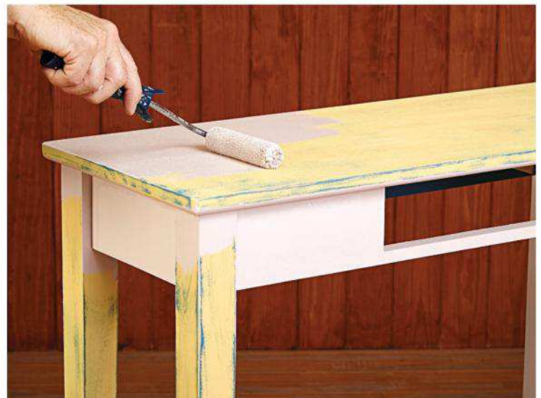
If you like, apply a third color (Sherwin-Williams no. 6043 Unfussy Beige shown), brushing or rolling on, as you would for a typical piece. Sand wear areas again after the paint dries.
