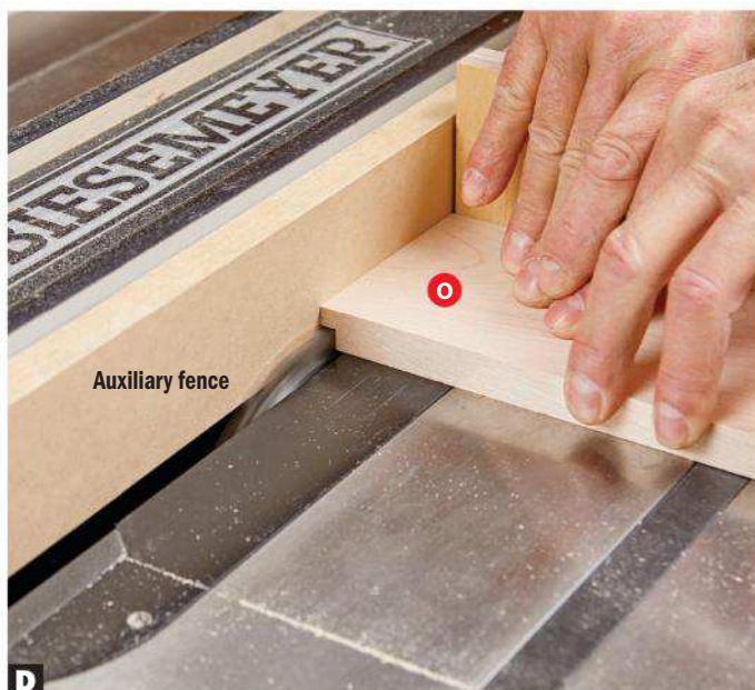
D Attach an auxiliary face to your rip fence with the outside just touching the dado set to rabbet the drawer fronts and backs (O–Q).
