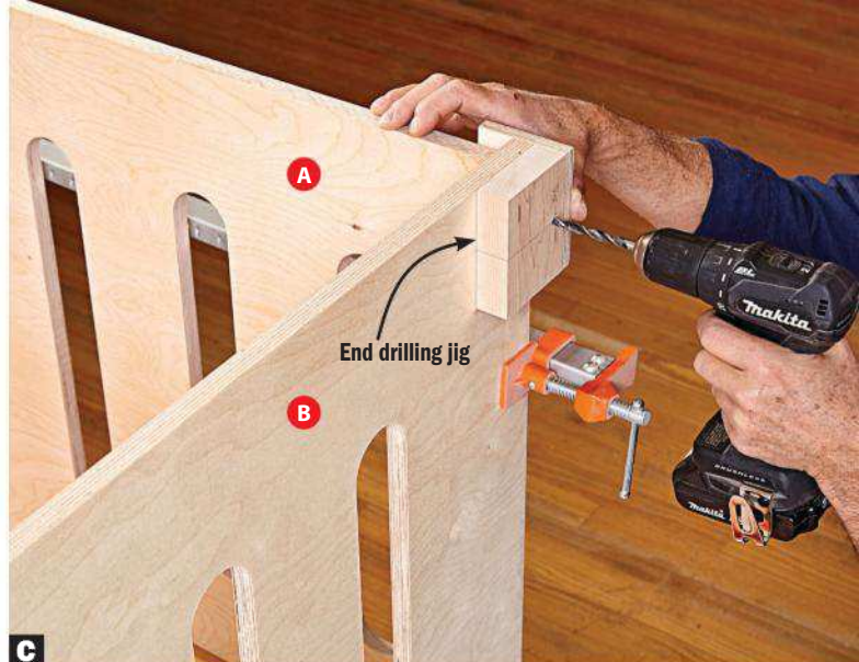
C Clamp the ends (B) to the sides (A) with their bottom edges flush and the sides inset \frac{1}{4} ". Drill holes that intersect the holes in the sides and toddler panel.
