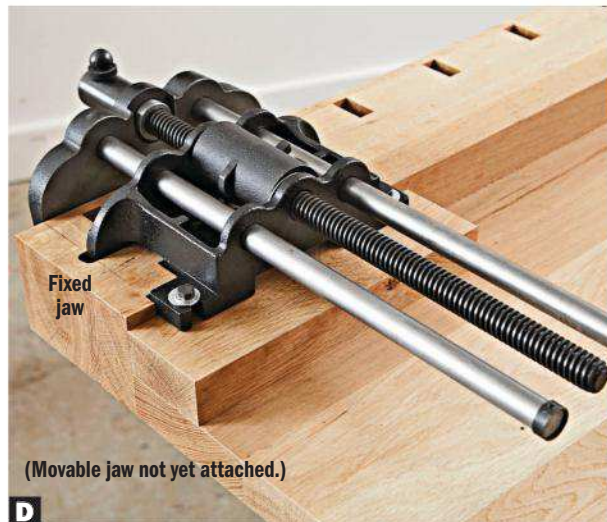
D A cast-iron-jaw vise can be recessed into the bottom of a bench for maximum strength and stability. A thick outer jaw distributes clamping force over a wide surface area. Note how the vise rails fit between dogholes for the tail vise located at the right end of the bench.
