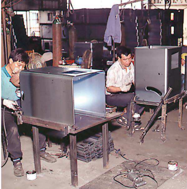
Welding shops, like this one where tablesaw bases are fabricated, have not felt the brunt of environmental enforcement. But heavy polluters that discharge air particulates or chemicals in excess of regulations have had to upgrade their environmental controls or close.
