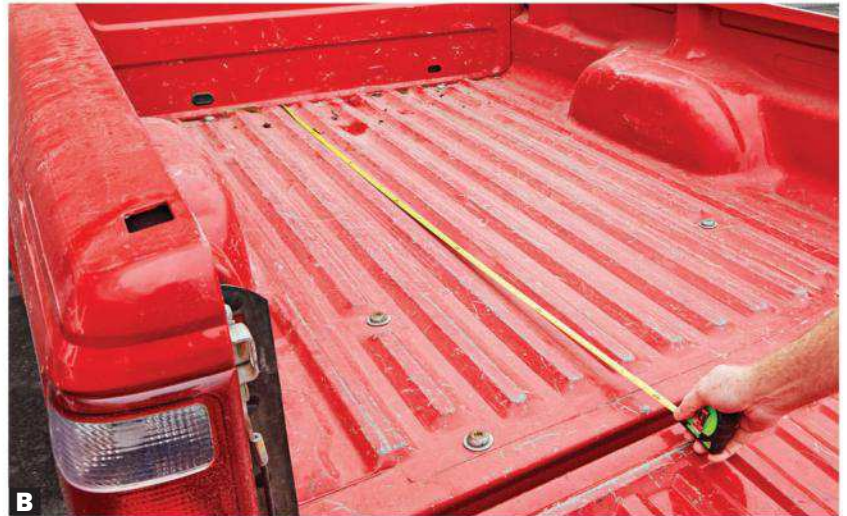
B Measure the length of the bed (not including the tailgate and gap between it and the bed) to determine the length of the side rails (B).
