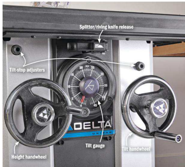
Pull the quick-release lever to remove the guard/splitter from the Delta—no need to remove the throat insert.
