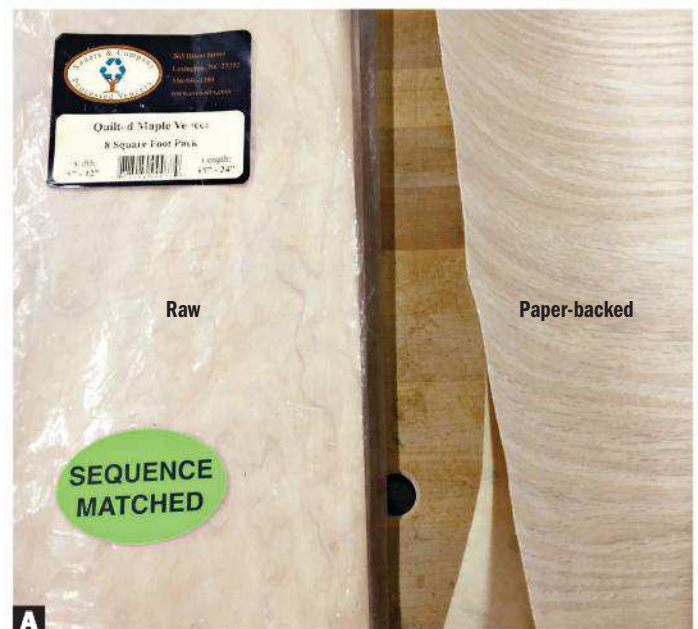
A This sequenced flitch of maple veneer on the left contains eight pieces that will cover 8 square feet. On the right is a single 24×96" sheet of paper-backed oak veneer with a pressure-sensitive adhesive (PSA) backing.
