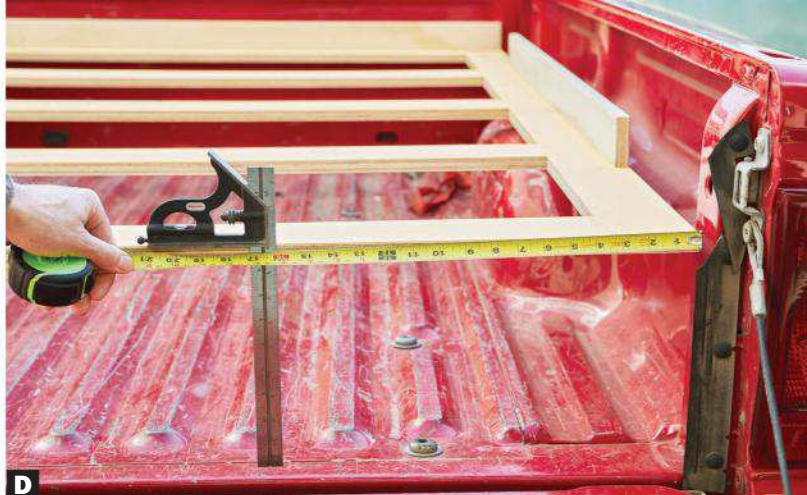
D Determine the width of the vertical supports by measuring from the bottom of the frame to the bottom of the corrugated channels. Now transfer the location of the center of a channel to the frame. This marks the center of one of the vertical supports. Measure from the edge of the frame to the square, as shown, and transfer this measurement to the other end of the frame. Repeat for the other support.
