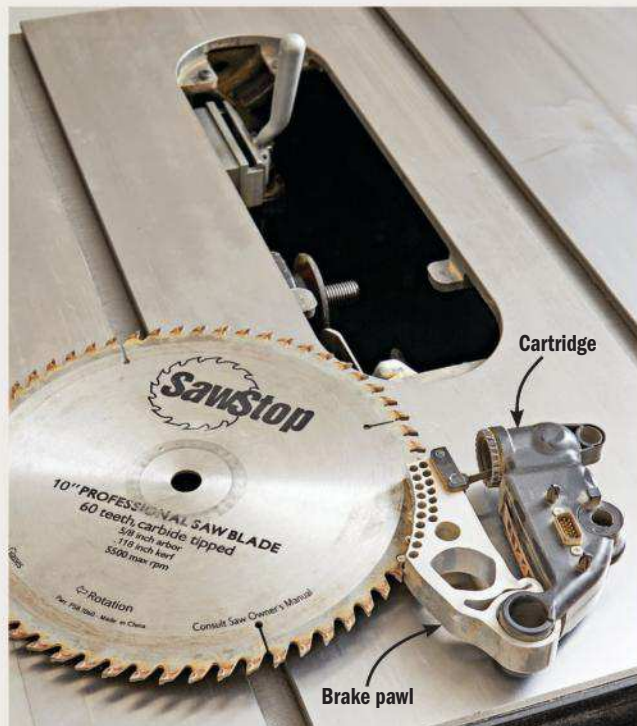
A SawStop blade-brake activation leaves the blade and brake cartridge unusable, but your fingers completely usable.
