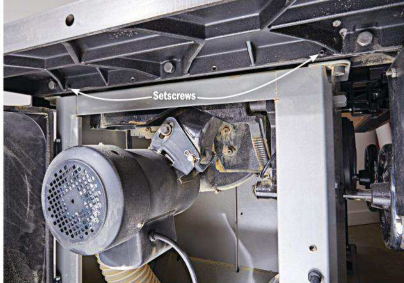
Setscrews make it easy to level the wings on the Delta Unisaw. You simply attach the wings to the top by loosely securing the bolts, adjusting the setscrews until level, and then tightening the bolts.
