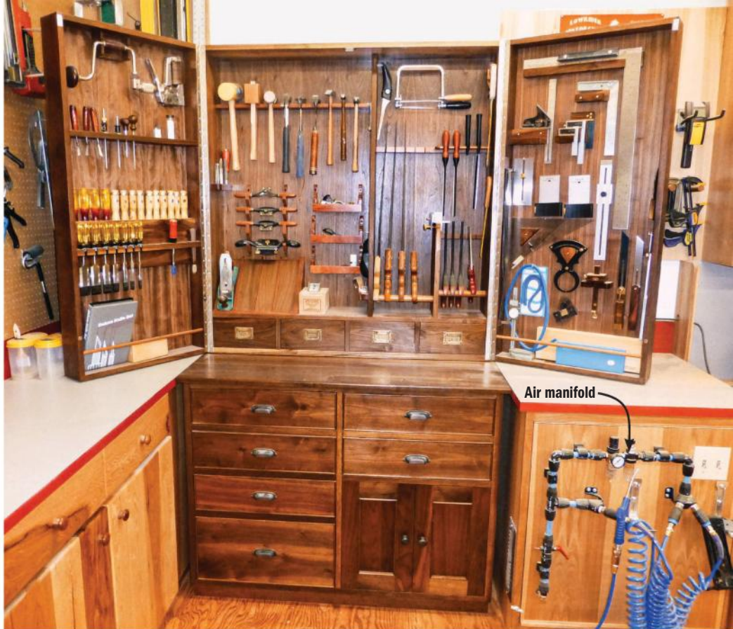
Wayne built this walnut tool cabinet with customized holders for his hand tools. Beside it, a manifold distributes air to three separate lines. The manifold panel is hinged at the top, allowing Wayne to remove the compressor for site use.
