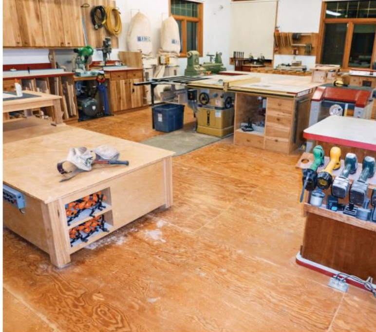
The central work triangle consists of a tablesaw with sliding cutoff table, backed by a large outfeed table, and a multipurpose workstation, all at the same height.
