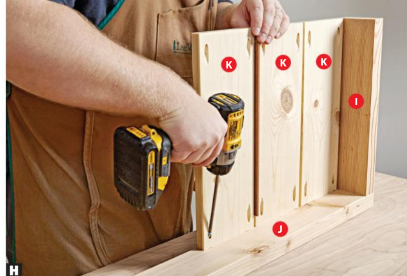
H Pocket-screw the slats (K) to a long rail (J). With all of the slats screwed on one long rail, attach the other long rail to the slats and short rails.
