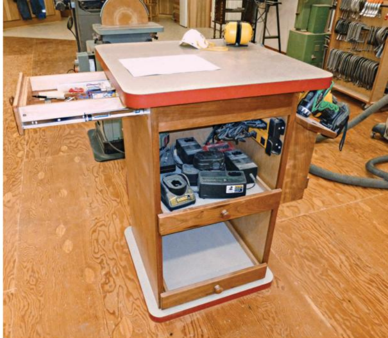
This stand-alone workstation resides at the hub of Wayne's workspace. Drawers hold common layout and measuring tools. The plastic-laminate top "eliminates coffee rings," Wayne quips.
