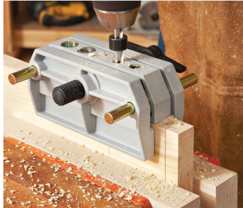
Drill out a mortise with a series of overlapping holes made with a doweling jig.
