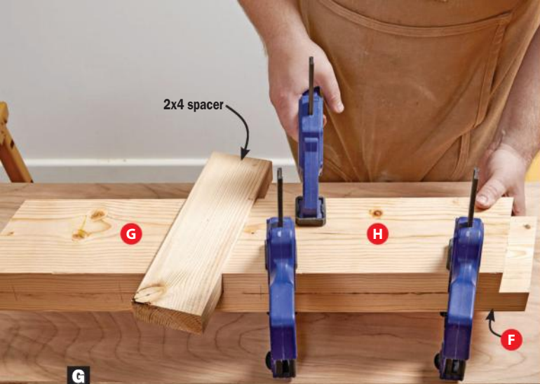
G Glue and clamp the upper leg filler (H) to the F/G assembly using a 2x4 spacer for correct positioning.
