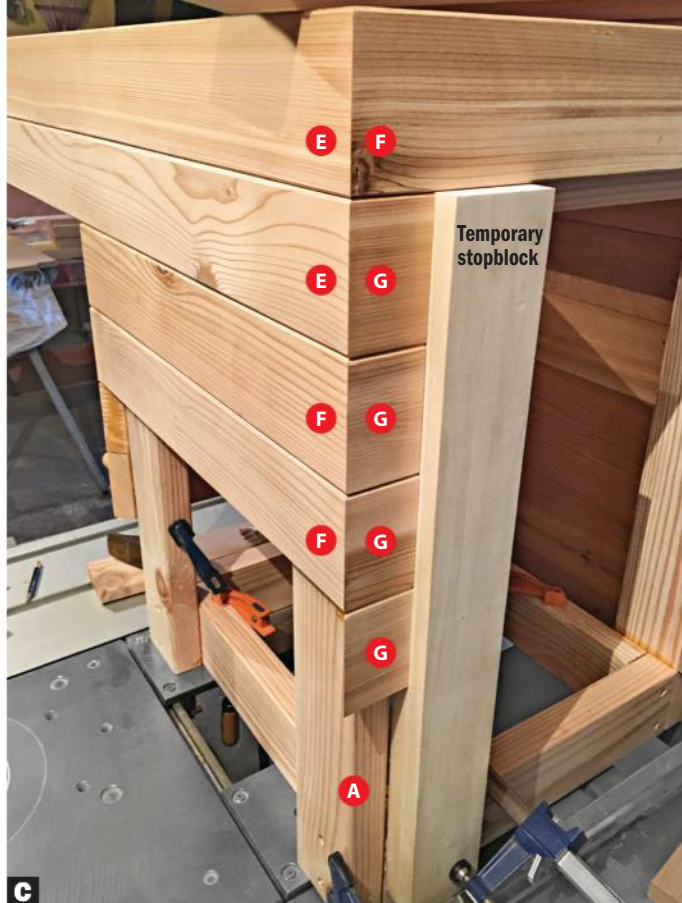
C Clamp a spare board as a stopblock for the end siding (G) flush with the long stile (A). Cut the piece to length, with a miter at one end and square cut at the other, align it against the stopblock, and secure it in place.
