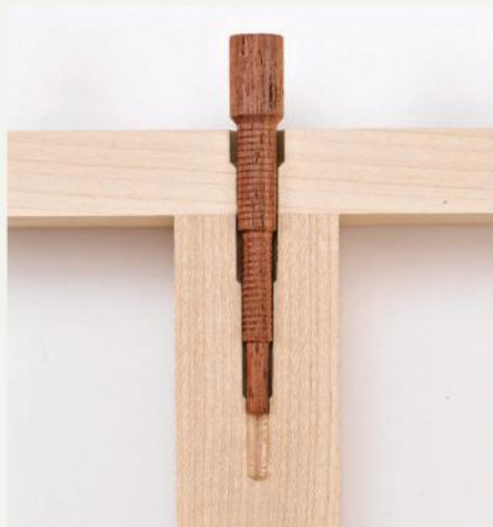
Here's a stepped Miller dowel ready to be driven home in its matching hole. During assembly, seat the dowel as deep as it will go, then trim the end flush.
