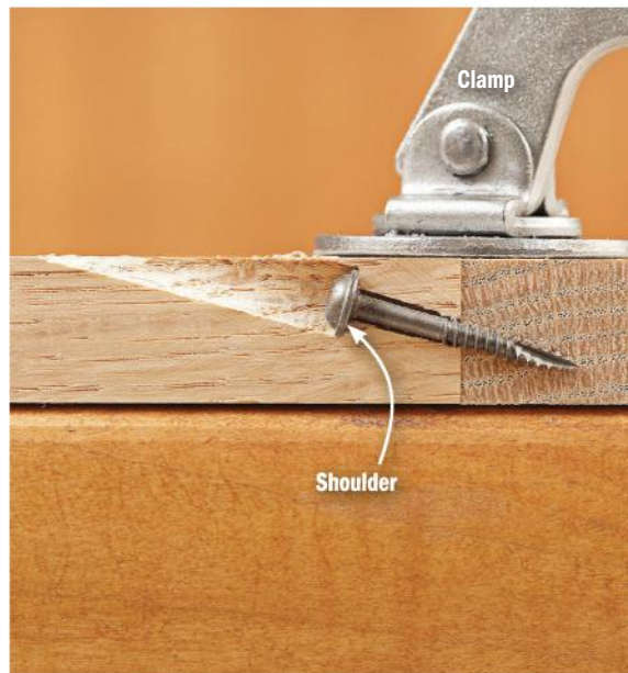
A cutaway view of a pocket hole shows the angle the screw takes into the mating workpiece. The shoulder stops the panhead screw at the proper depth.
