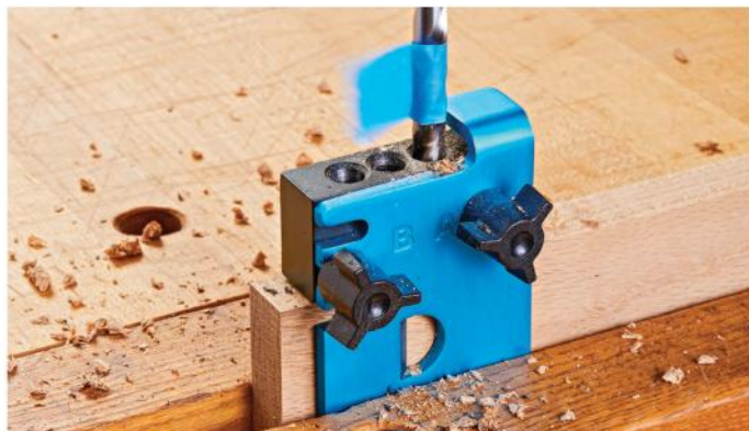
Drill the Beadlock mortise with a series of overlapping holes using the jig and included bit. Repeat for the mating workpiece.
