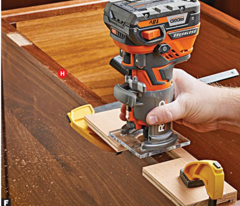
F Set the pattern bit cutting depth to equal the thickness of the hinge leaf.
