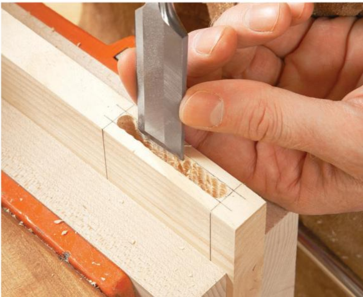
Flatten and smooth the mortise walls with a chisel. Take care to hold the chisel 90° to the workpiece to ensure a mortise with square walls.
