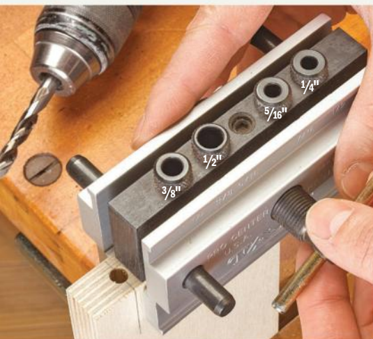
This self-centering doweling jig locates precisely positioned dowel holes and can drill holes of four different diameters.
