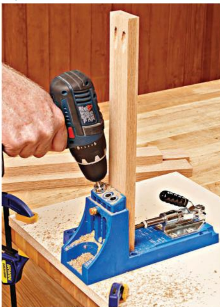
A pocket-hole jig guides the bit to create angled pilot holes. The best jigs either hold the workpiece or clamp to it for drilling.
