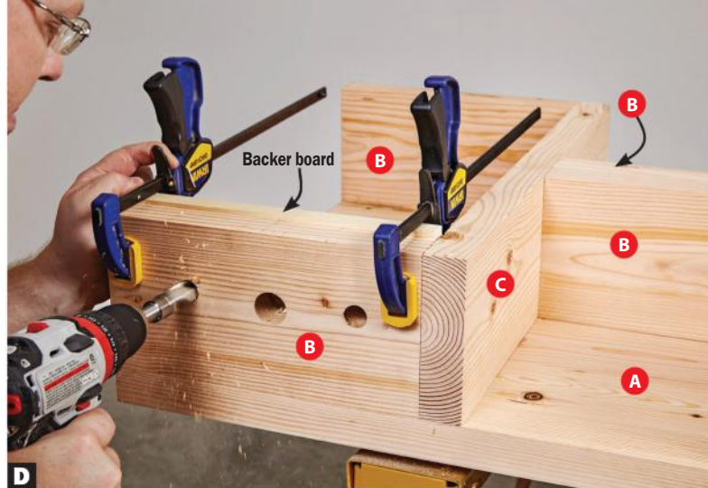
D Drill the vise holes using a clamped-on backer board to prevent blow-out on the exit side.
