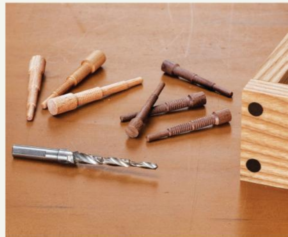
A finished Miller dowel joint, crafted with the stepped bit and walnut dowels (oak dowels also shown).
