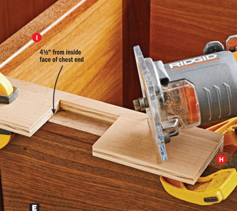
E Clamp the hinge-mortising jig to the chest back (B) and back molding (H) to create a stable platform for your trim router.
