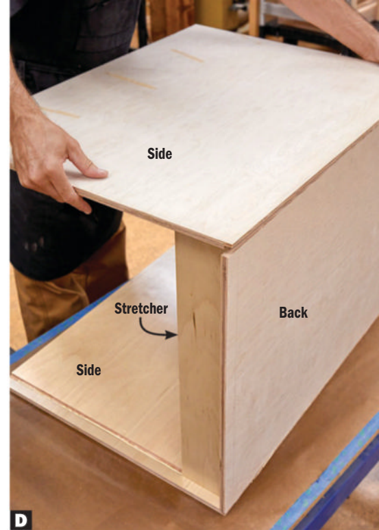
D Add the stretchers and remaining side. Then glue the face frame to the carcass (no staples).
