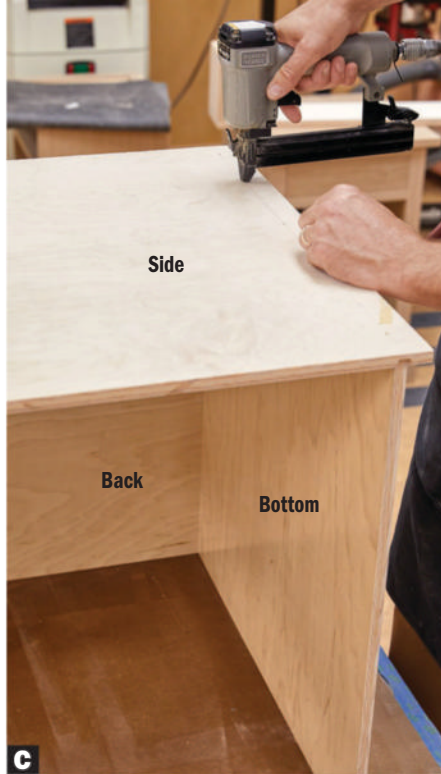
C Attach a carcass side to this assembly. The sides protrude ¼" beyond the bottom to fit into the grooves in the face frame.
