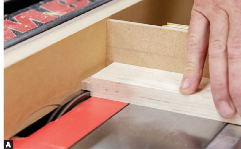
A Adjust the blade height and rip-fence position to cut ⅜"-long tongues on each end of the door rails. Sneak up on the final blade height to get a snug-fitting tongue.
