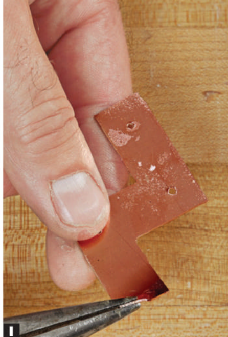
I Form the hinge barrel, working from the outside edge, by folding the copper upward [Photo I] at the bottom of the hinge tab. Similarly fold the copper at the top of the tab [Photo J]. Work back and forth folding until you can slide a length of \frac{1}{8} " rod into the roughly shaped barrel [Photo K]. Complete the barrel by working it around the rod.
