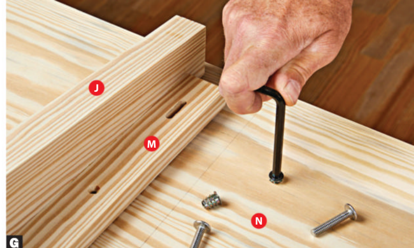
Drive the threaded inserts into the headboard (N) with a hex wrench.
