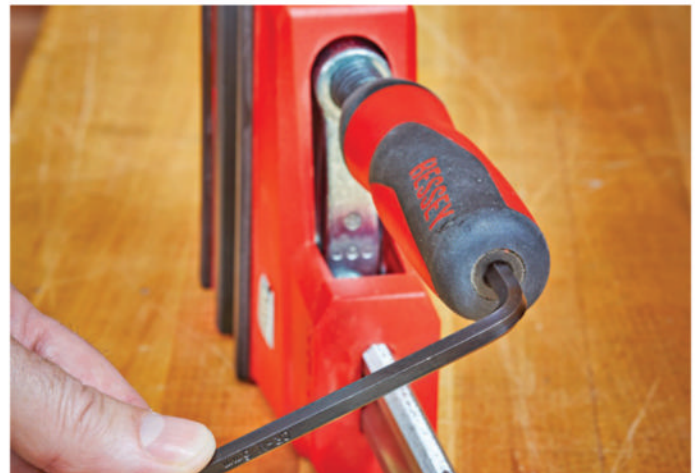
Gain clamping force with the Bessey K Body Revo clamps by inserting a 6mm hex wrench into the socket in the handle end and cranking it.
