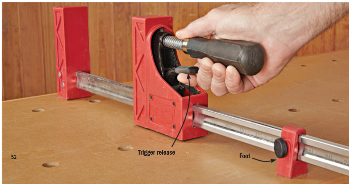
To keep the sliding jaw from dragging on the workbench , you can reposition the foot on the Jet and Irwin clamps, helpful when the clamp is longer than your worksurface.
