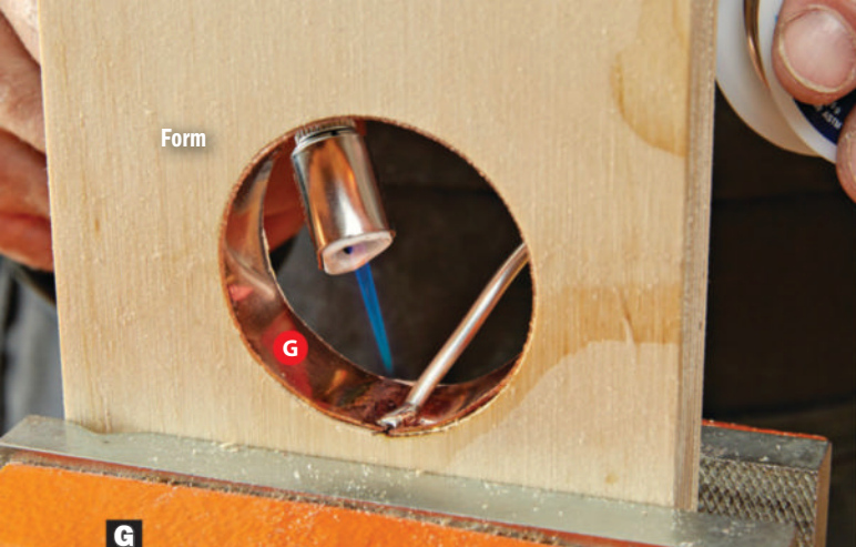
G Solder the butted chimney (G) ends together inside the form hole. A slight solder bead on the inside of the chimney ring is OK.
