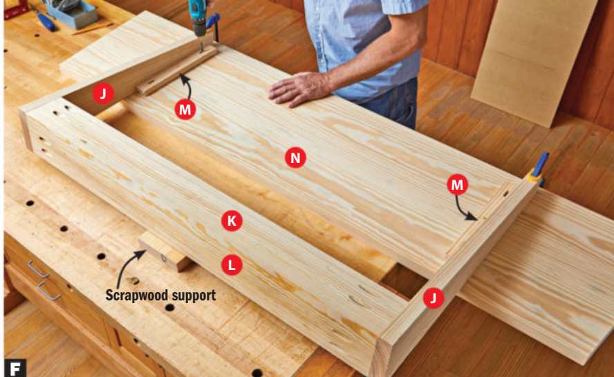
F Center a \frac{1}{4} " drill bit in the flange (M) slots and drill into the headboard (N) only enough to make a mark. Drill pilot holes into the headboard at the flange center-hole locations.
