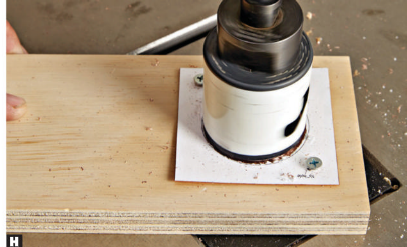
H Bore the chimney plate using a drill press and holesaw. The screws prevent the copper from spinning—do not attempt to hold the metal by hand.
