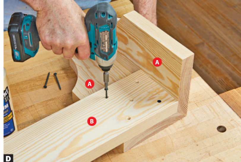
D Glue and screw the feet (A/A) to the ends of the end rails (B) with the top ends and edges flush and the rail ends tightly butted into the inside corners of the feet.
