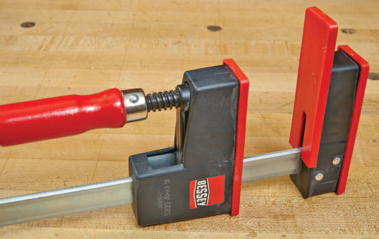
Jaw sleeves help prevent workpiece marring and provide a more glue-resistant surface compared to the actual jaws. You can replace these or remove them for cleaning.
