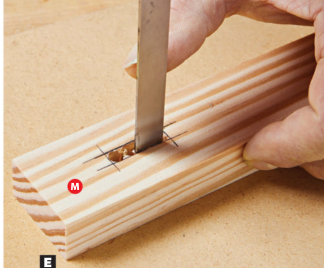
E Lay out the slots and drill overlapping \frac{1}{4} " holes. True up the edges of the slots with a chisel.
