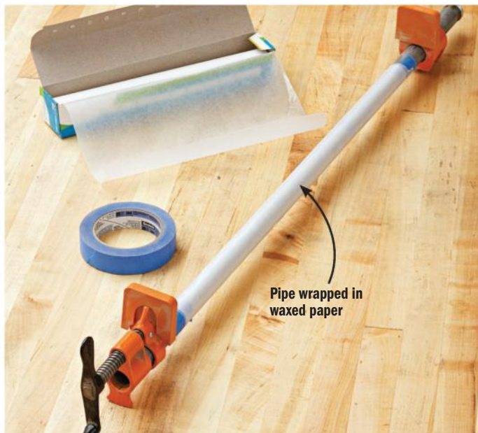
Apply a waxed-paper or tape barrier. Keep the ends of the paper or tape a couple of inches away from the jaws so the jaws have room to move in during clamp-up.
