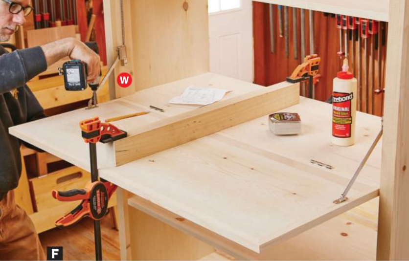
F Clamp a dead-flat scrap to the shelf and drop leaf, then screw the Stopmatic Supports to the drop-leaf stops (W).
