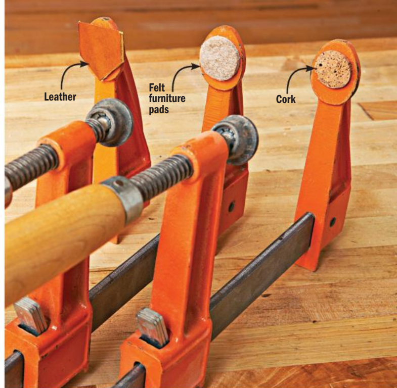
Add materials that cushion jaws. Scrap leather, self-adhesive furniture pads, cork, or even scraps of hardboard all prevent crushing the edges of panels during a glue-up.
