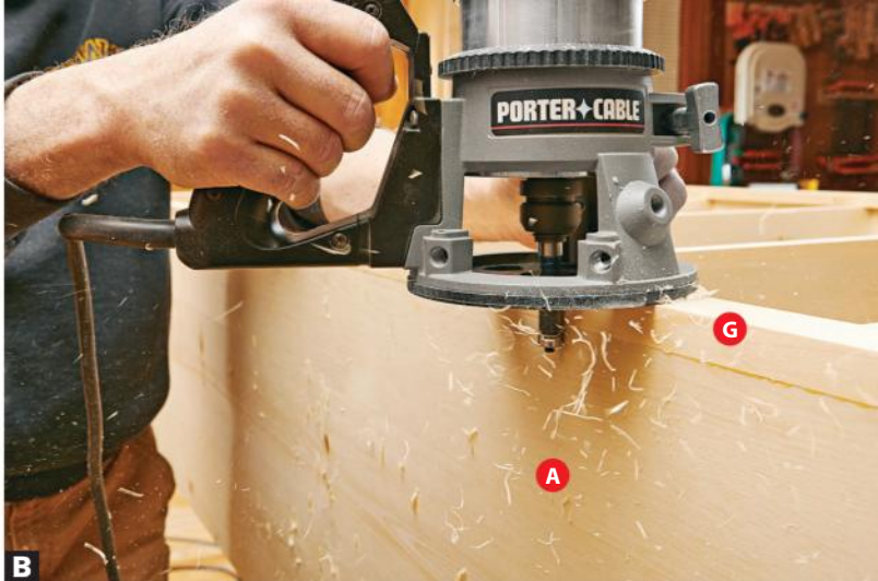
Rout the stiles flush to the sides using a bottom-bearing flush-trim bit.
