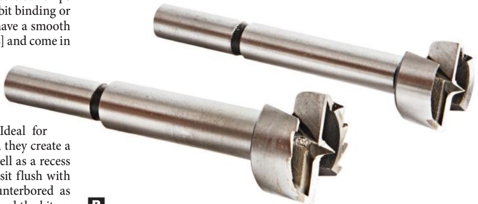
B Saw-tooth rims dissipate heat better than smooth rims, so larger-diameter bits typically use this design.
