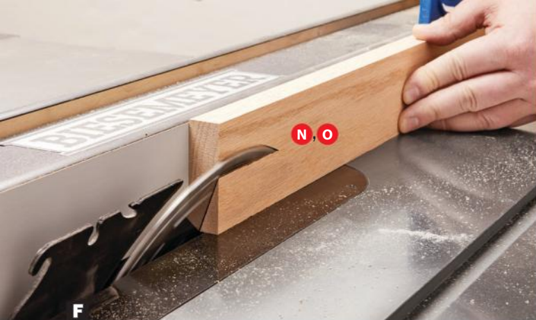
F With the tablesaw blade tilted to 20°, rip the molding face (left) and edge (right). Allow enough extra thickness and width to sand out saw marks as these moldings show prominently on the installed project.
