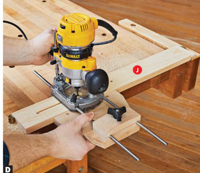
D Align the bit to one side of the starter hole and lock in your router edge guide. Rout one side of the slot from hole to hole. Rotate the leg and rout from the opposite edge to center the slot. Flip and repeat from the opposite face to complete the slot.
