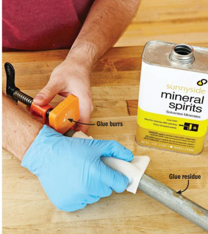
Clean clamps don't ding wood surfaces. Mineral spirits cleans most debris from clamps. Scrape off dried glue with a putty knife. Soften stubborn glue with heat and a damp rag.
