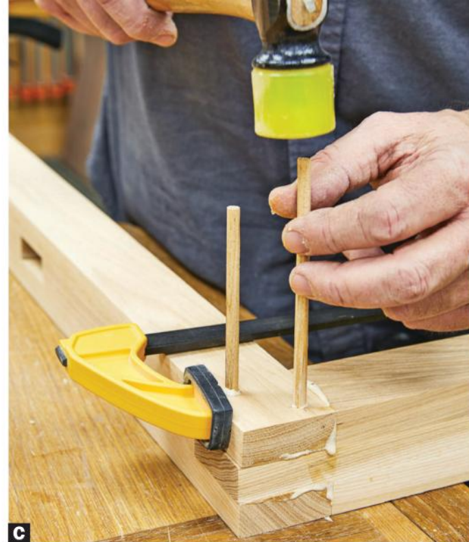
C Apply glue, reassemble the parts, and drive in 1/4" dowels. Trim the dowels flush.
