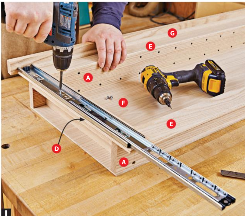
I Attach the slides to the wall box tight against the stop (G) and flush with the outer edges of the rails (D). Make sure the slides are parallel.
