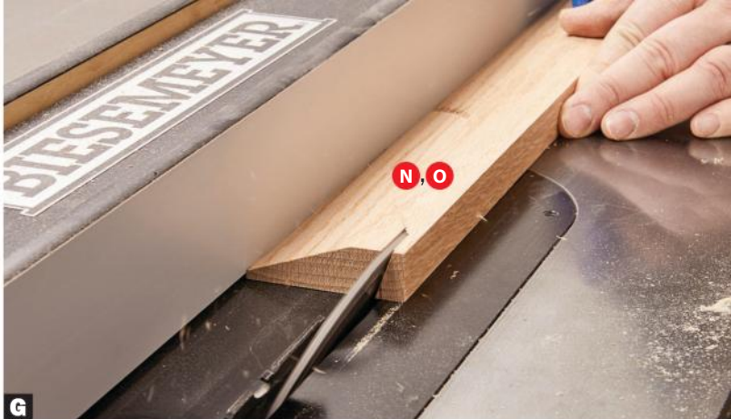
F With the tablesaw blade tilted to 20°, rip the molding face (left) and edge (right). Allow enough extra thickness and width to sand out saw marks as these moldings show prominently on the installed project.
