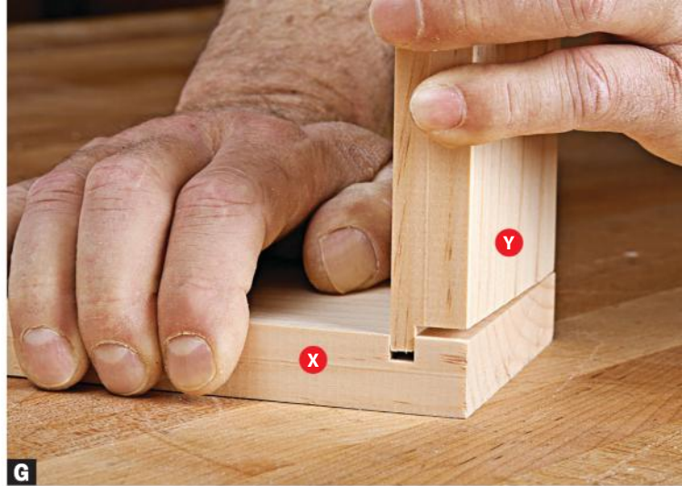
G The tongues on the ends of the tops, bottoms, and dividers (Y) fit into the side (X) dados. The joints are exposed so make them a snug fit.
