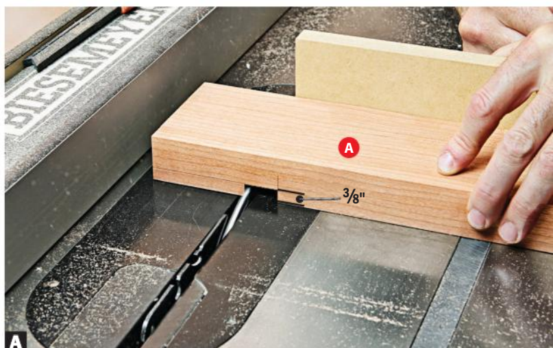
Set the rip fence for the innermost cut , then move the blank away to widen the rabbet for the helicopter platform. Use a dado blade if you have one to work faster.
