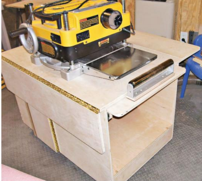
Flip-up wings on a planer cart provide a place to set boards between planing passes, then fold down for storing the cart. The roller extends on a sliding platform to support long boards.
