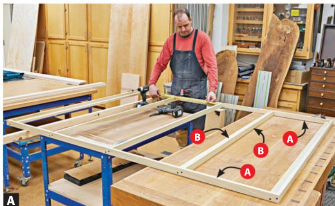
A Glue and screw the frame sides (A) to the strut assemblies (B/B). Ensure the assembly is square, then allow the glue to dry.
