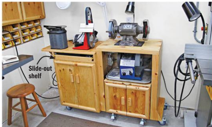
No sharpening system is perfect for every tool , so John has five, including a horizontal abrasive wheel, vertical sanding belt, bench grinder, and a water-cooled slow-speed grinder on a roll-out cart. Waterstones and a lapping plate rest on a locking slide-out shelf.
