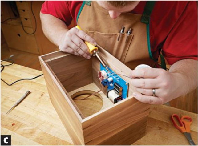
C Connect leads to the crossover first. Solder the wire to a pair of terminals, then cut the wire to length so that you can easily solder to the woofer, tweeter, and speaker-wire terminal [Photos D and E].
