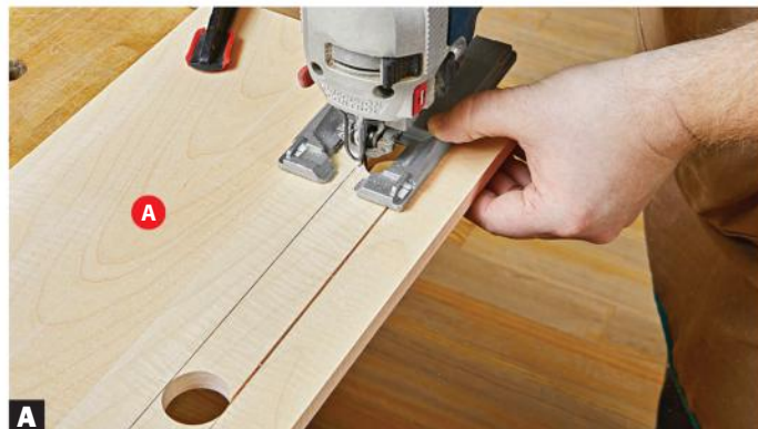
Create the handhold slot by drilling 1\frac{1}{4}" holes at each end of the marked slot, then connecting them with jigsaw cuts. Sand the edges smooth when finished.
