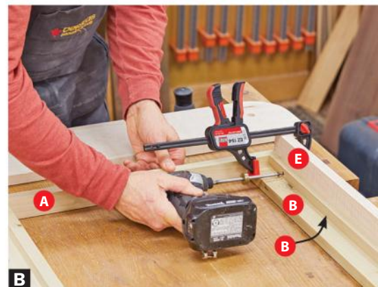
B Glue and screw the foot rail (E) to the frame, flush at the bottom and ends. Repeat with the head rail (D).
