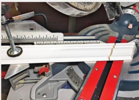
F Find the two inside corner (IC) mated templates and mark them left and right. Do the same with the two mated outside corner (OC) templates. Placing the templates in their intended position provides a visual cue of how to place your workpieces on the saw.
