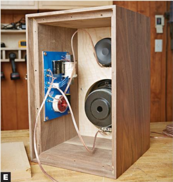
E Solder the wires to the woofer and tweeter, then mount the speakers in the box [Exploded View]. Solder the last lead to the speaker-wire terminals, and test the speakers before screwing the back in place.
