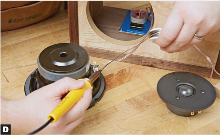
E Solder the wires to the woofer and tweeter, then mount the speakers in the box [Exploded View]. Solder the last lead to the speaker-wire terminals, and test the speakers before screwing the back in place.
