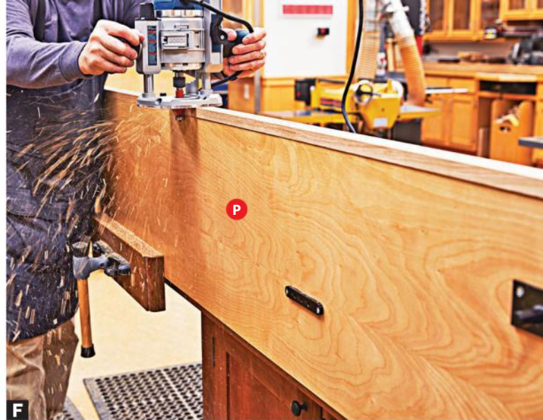
F Trim the stile (R) flush with the face of the inner side (P) using a bottom-bearing flush-trim bit.
