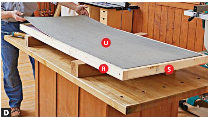
Glue the cement board into the frame rabbets and secure it with screws around the edge.
