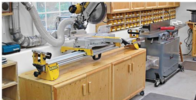
A window recessed in a knee wall provides 14" of clearance behind the sliding compound mitersaw, reducing the depth of the workstation's footprint. As the owner of a hardware store, John knows how to keep fasteners organized, using a 10' run of bins and cabinets above the jointer.
