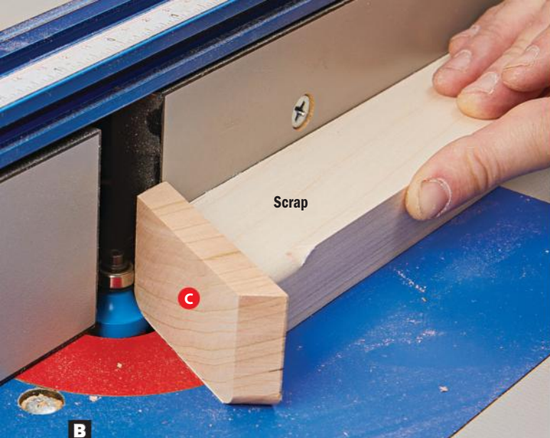
B Rout \frac{1}{4} " round-overs on the top edges of the cowl (C), aligning the mitered edge of the cowl flush with the edge of the scrap.
