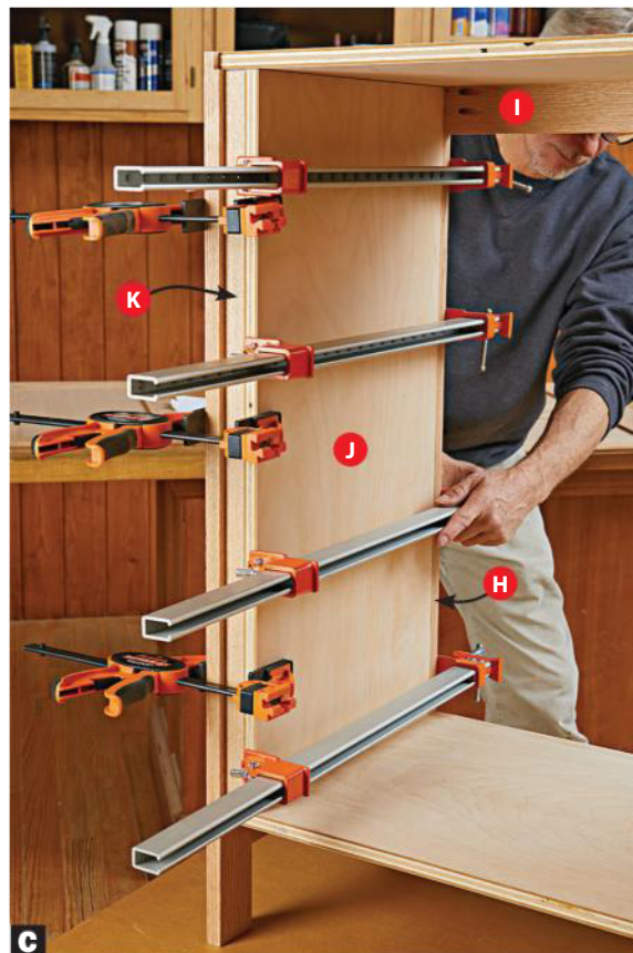
B Glue and clamp the face frame to the carcass, flush at the top and with the stile edges equally overhanging the sides. The lower rail protrudes 1/8" above the carcass bottom (G).
