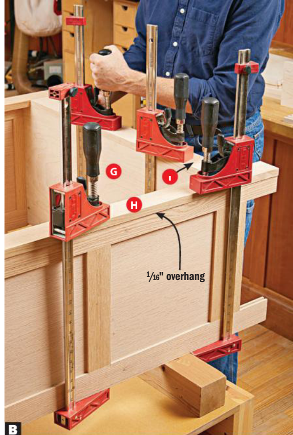
B Glue and clamp the face frame to the carcass, flush at the top and with the stile edges equally overhanging the sides. The lower rail protrudes 1/8" above the carcass bottom (G).
