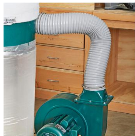
The connector hose on some models adds resistance under pressure by forming a sharper bend. To maximize airflow, trim the hose as short as possible.
