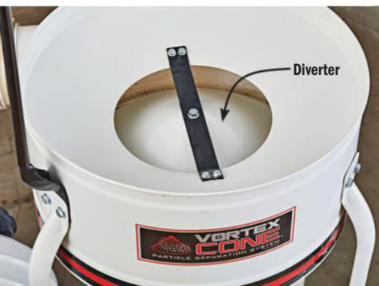
A cone-shaped diverter inside the Jet and Powermatic collectors forces debris toward the outer rim as it enters the separation chamber, better slowing down and settling heavier particles into the collection bag, rather than clogging the filter.
