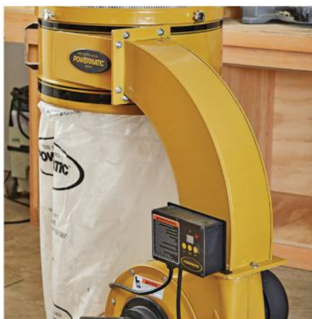
Powermatic's metal chute streamlines the path to the separation chamber for debris. We believe this helped this unit produce the highest airflow of the group.
