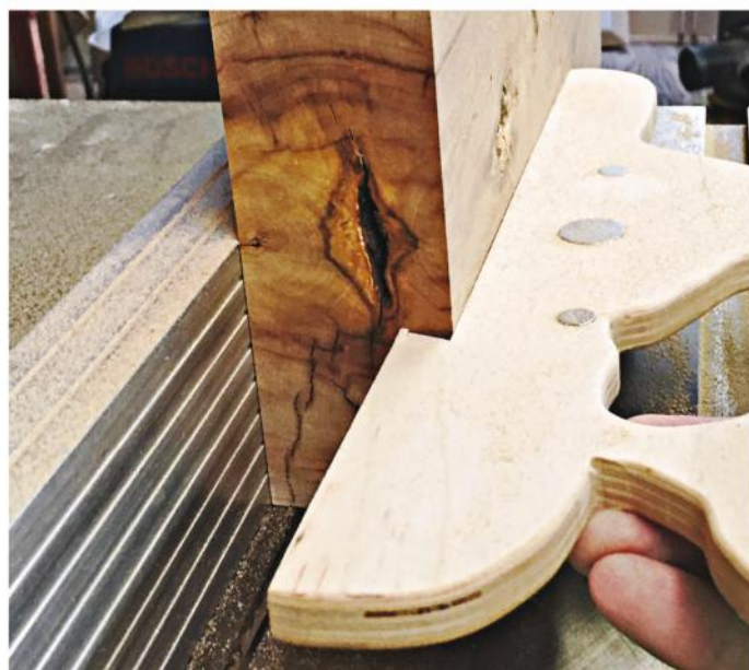
Keep the stock firmly against the fence and the tabletop. A pushstick keeps needed pressure against the fence, and your hands away from the blade as it exits the cut.
