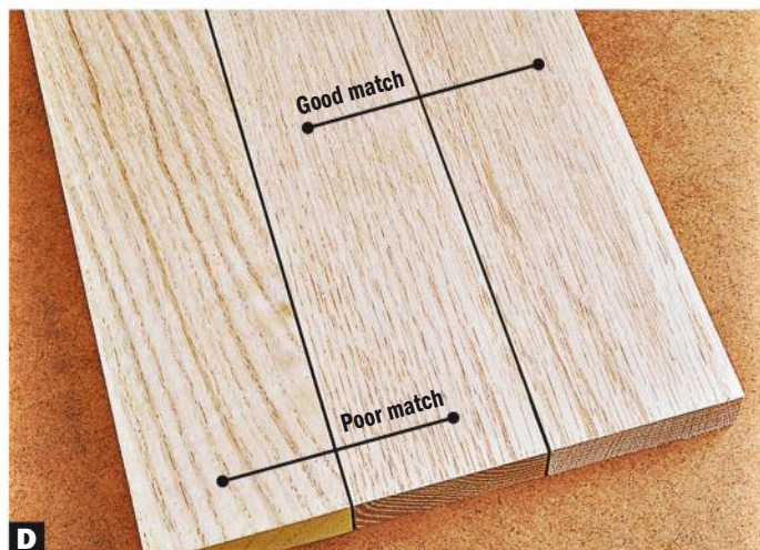
D Joint lines disappear when you arrange boards so the grain pattern and color appears continuous. The seam between the two boards on the left will be obvious. The line between the two on the right will be nearly invisible.
