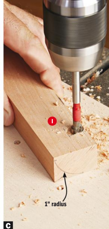
C Use a \frac{3}{8} " Forstner bit to rough out the flat-bottomed mortises that later accept the struts (J, K). Chisel the edges of the slots straight.
