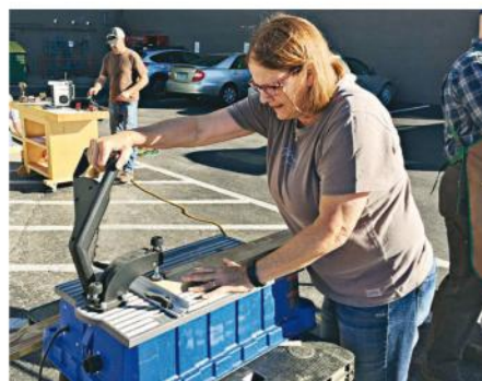
Illustrator Lorna Johnson drilled more than 400 pocket holes (using a Kreg Foreman) to assemble the inside frames.
