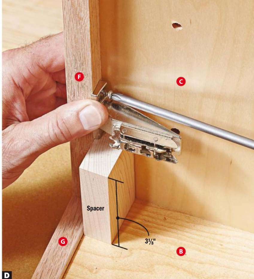
D To attach the hinges, first rest the lower hinge-mounting plate on a 3 1/8"-tall spacer and then screw the plate to the face-frame stile.
