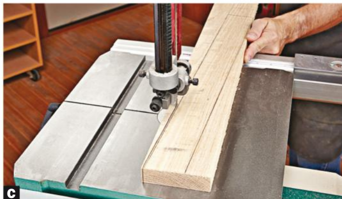
C Lay out a line parallel to the grain, then bandsaw as close to the line as possible. Joint the edge before ripping the piece to width at the tablesaw.
