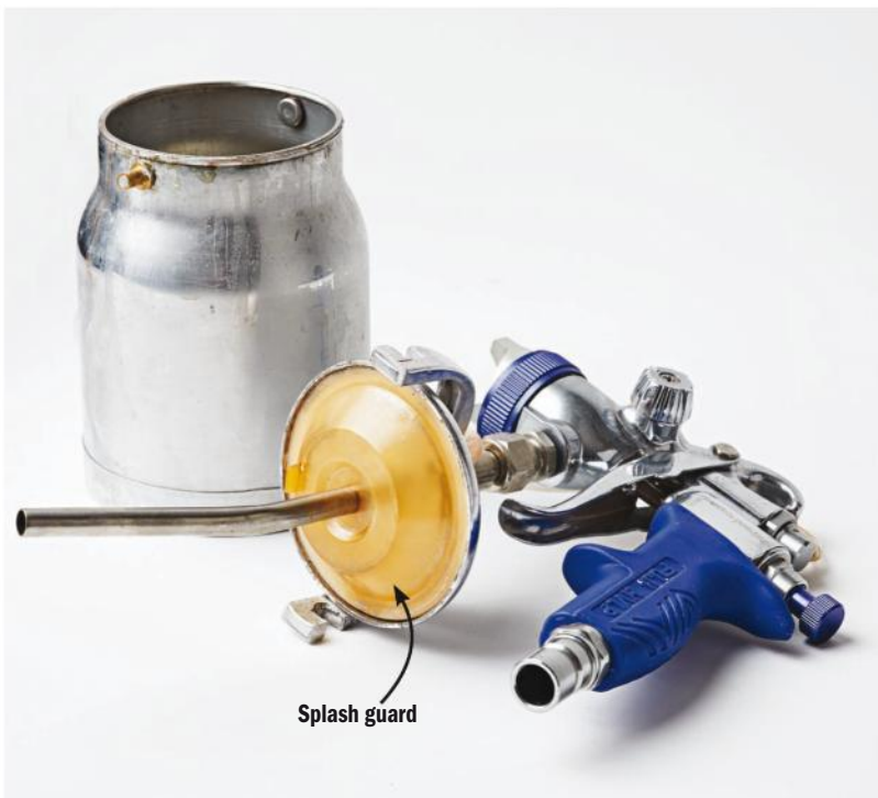
The Fuji T-70 spray gun has a plastic splash guard on the underside of the cup lid to prevent finish from getting into the nooks and crannies of the cast lid, making cleaning easier.
