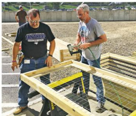
Digital content manager Lucas Peters (right) and I filled each frame with wire-mesh fencing held in place with narrow crown staples. (Note the stack of completed panels behind Lucas.)
