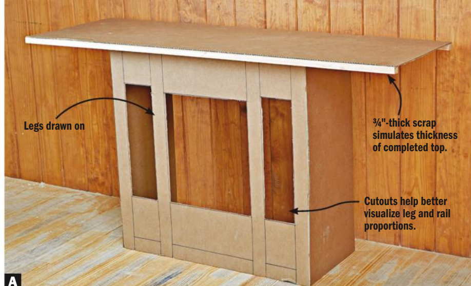
A Cheap will do. Use cardboard, plywood, hardboard, or foam sheets to create full-size or scaled mock-ups.
