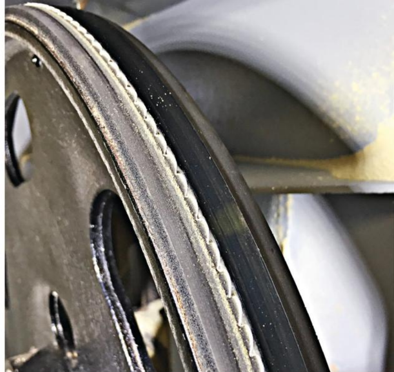
A blade too far back on the wheel , such as this one, tends to make the cut drift toward the fence. A blade that runs too close to the front edge of the wheel does the opposite.
