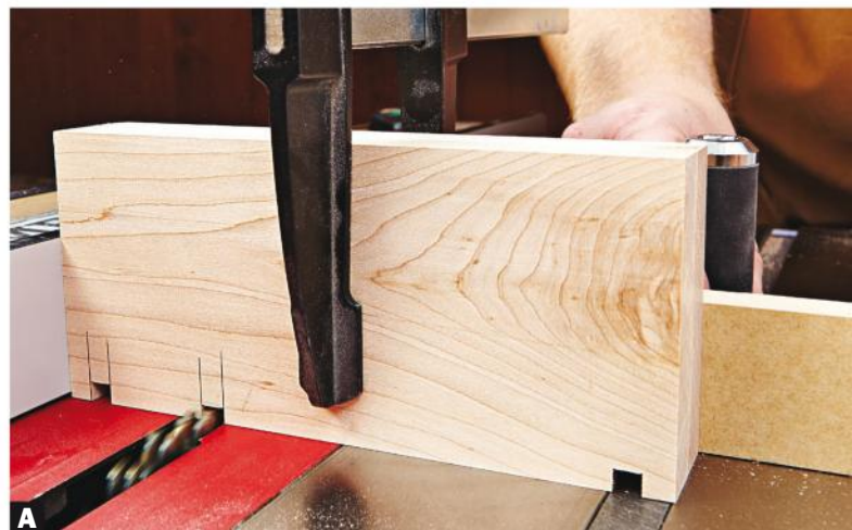
Cut the notches in both blanks , using the rip fence as a stop. After cutting the first notch, rotate the boards to cut the same for the other end. Repeat for the middle notches.
