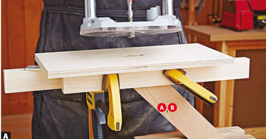
A Cut the mortises. Clamp each seat rail (A) and leg (B) in a vise with its mitered surface positioned horizontally. Align the mortise centerline with the witness mark on the jig and plunge the router to make the cut.
