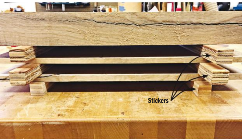
Sticker ing allows rebalancing the moisture content so stock stays flat. The stickers (scraps of plywood in this case) should be evenly spaced and a weight placed atop the stack to reduce warping.
