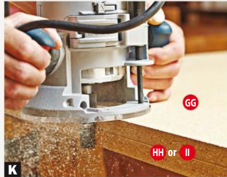
K Trim the countertop rails (HH, II) flush with the panel (GG) edges using a top-bearing flush-trim router bit.
