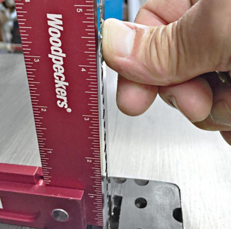
Stand a square ¼" from the blade (you may have to raise the blade guard to accommodate the square), and press the center of the blade. Moderate pressure should deflect the blade to touch the square.
