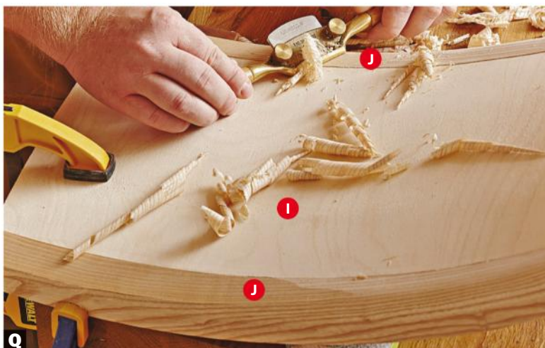
Q Take fine control of stock removal using a spokeshave to bring the back trim flush with the front skin. Work from the ends toward the center.
