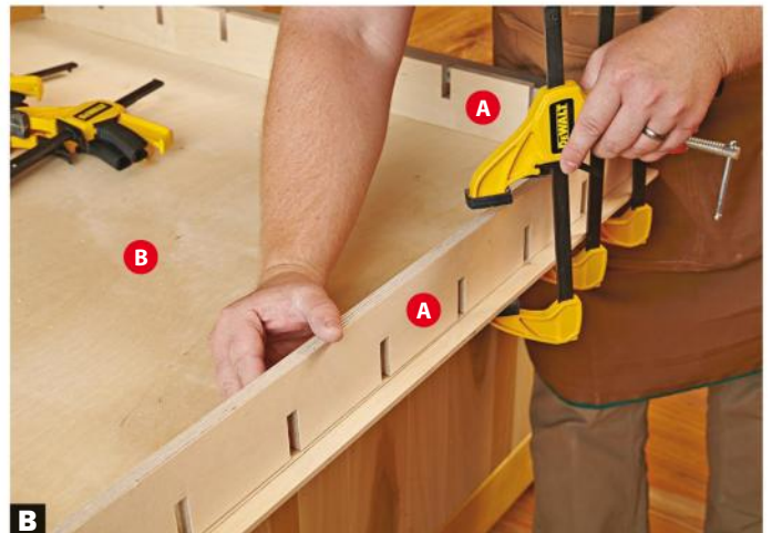
B Glue and clamp two adjacent frames just inside the marked lines. This provides a square and solid start to the frames' glueup.
