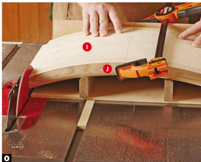
O Crosscut the ends of the seat back with its center aligned with the center of the jig. Apply masking tape to the exit side of the cut to reduce tearout.
