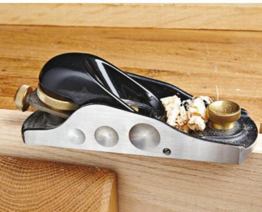
Low-angle block plane Use it to fine-tune part dimensions, cut chamfers, smooth joint lines, and remove tool marks.
