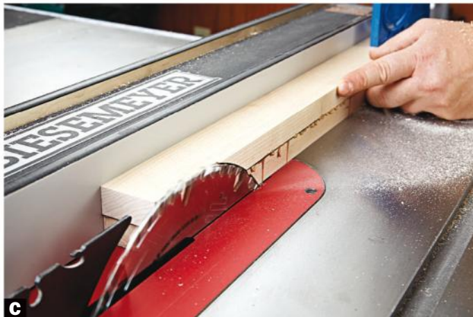
C Rip 1/16" from each face of the key blanks, smoothing the surfaces and bringing them to a finished thickness of 1 1/2".
