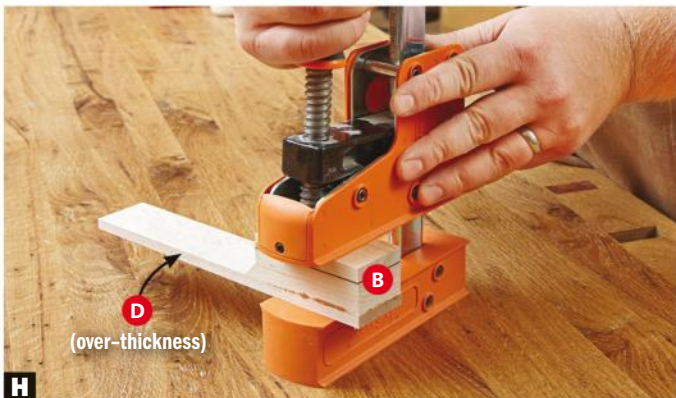
H Glue and clamp the short white key (B) to the over-thickness spacer (D), keeping the ends and edges flush. Remove excess glue from the bevel area.
