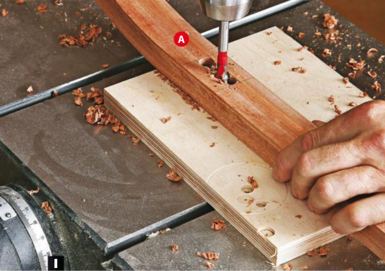
I Drill centered through-mortises at the drill press, using a 1/2" Forstner bit. Then square up each mortise with a chisel. Switch to a 3/4" Forstner bit to drill the rung mortises.
