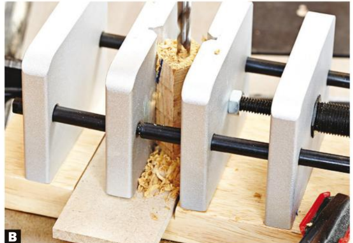
B Secure a pen blank between the jaws of a drilling center vise, clamp the vise to the drill-press table, and bore through the blank. (Or, hold blanks with a wooden handscrew clamp.)
