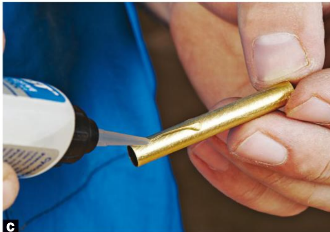
C Glue fast. Evenly space three thin lines of instant glue along half the length of the barrel. Insert the barrel fully into the blank, twisting it as you go. Work quickly, as most instant glues set up in 15 seconds or so.
