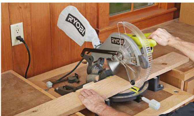
Miter saw You'll find this tool especially useful for crosscutting stock to rough length, and for cutting miters and bevels on boards too long to handle on the tablesaw.
