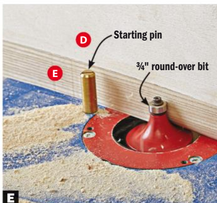
E Round over the seat-trim edges. For best results use a starting pin and be careful to hold the assembly as vertical as possible; it can tip slightly forward, but not backward.
