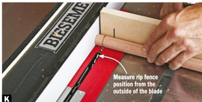
K Raise the blade 1/16" above the table, push the rung over the blade's highest point, and rotate the rung. Repeat, working your way out to create the tenon.
