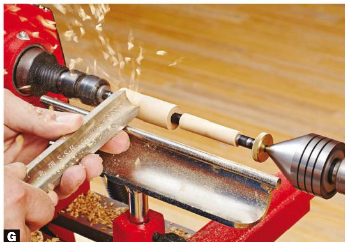
G Turn 'em round. Using a roughing gouge, turn both blanks to cylinders slightly larger in diameter than final size. Then fine-tune the diameter by lightly paring away shavings, using your fingers to support the blanks on the back side to prevent flexing. Continue until each cylinder reaches the desired diameter and shape. After turning several pens, your bushings might become slightly smaller in diameter through contact with the chisels and sandpaper. Instead of relying on the bushings as your depth guide, measure the diameter of the wood so it matches the pen components.
