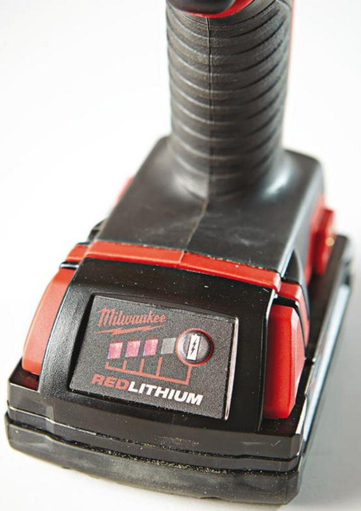
Get a quick read on a battery's charge level by pressing the indicator button. The Milwaukee battery shown here has about three-quarters of a charge remaining.
