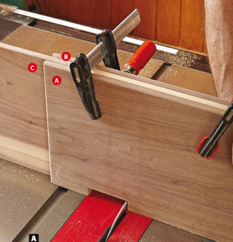
A Line 'em up and make the cut. With a tall fence on your table saw's miter gauge, pass the clamped shelf stack repeatedly through the blade to cut a notch in each shelf.
