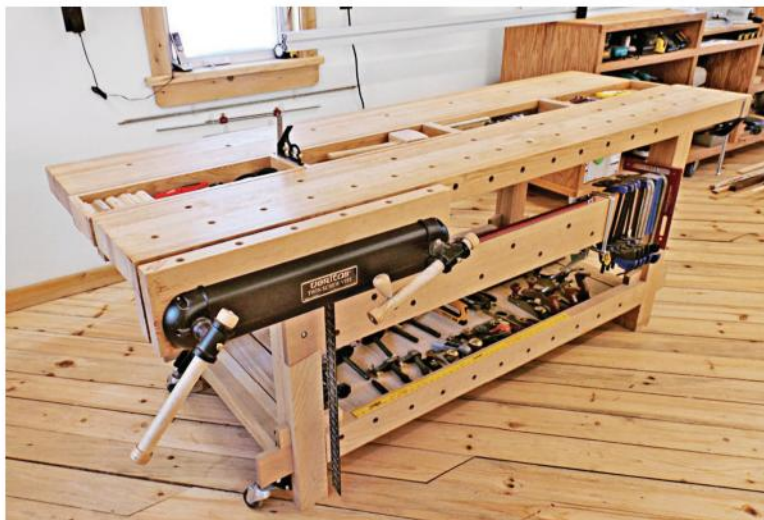
A 30×90" workbench built three years ago was Bill's first project. The ash top disassembles, allowing him to resurface the 12"-wide sections in his planer.
