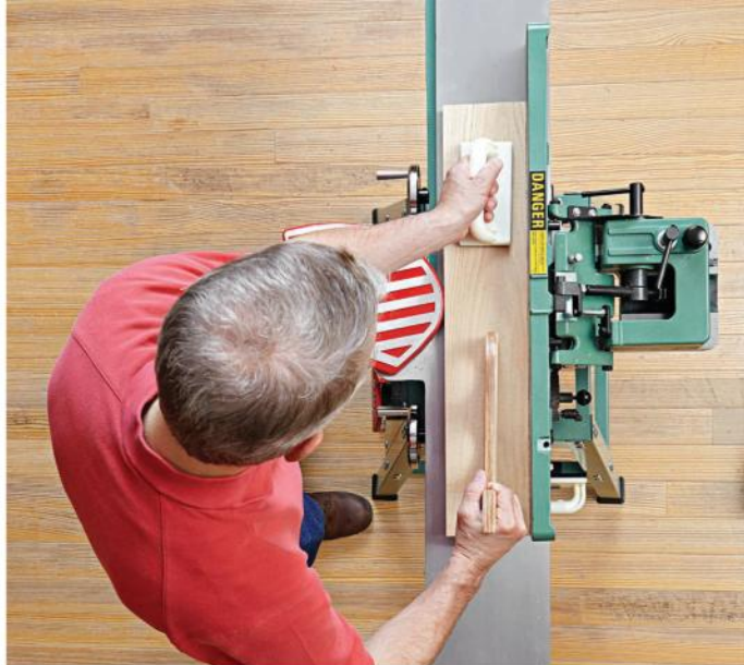
Move the board forward with your right hand, keeping the left hand near the cutterhead.
