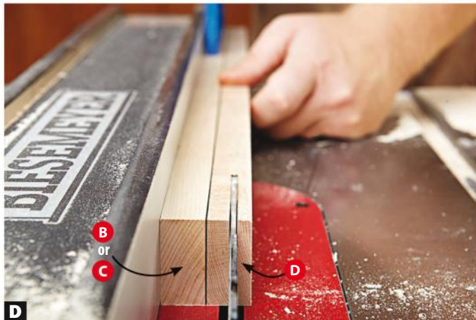
D Flip the key blanks upright and rip one edge to bring them to the finished width.
