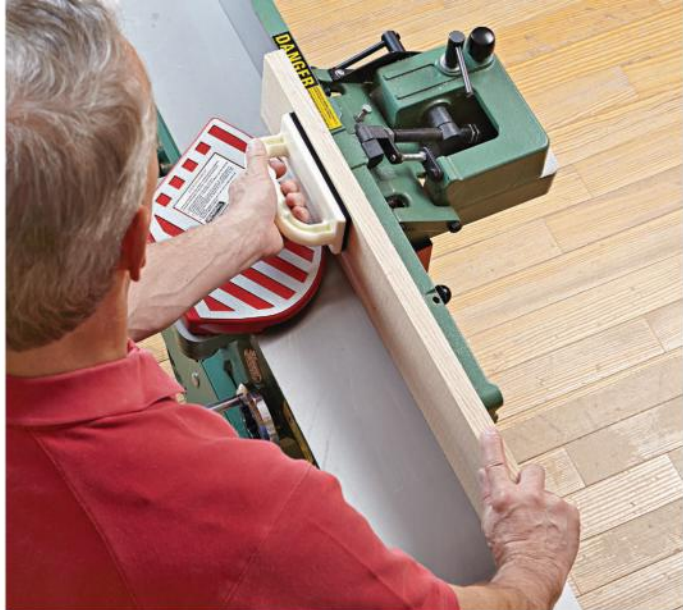
Joint an edge square to the freshly jointed face by pressing that face against the fence with your left hand while moving the board forward with your right.
