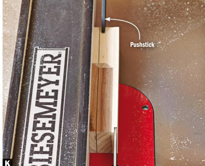
K Rip the six Assembly #1s to 1\frac{3}{16} " wide after scraping away excess glue. Rip only the spacers (D).
