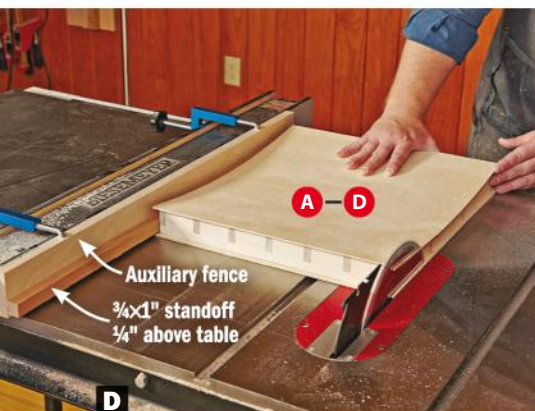
D Trim the excess skin. For accurate trim cuts, clamp an auxiliary fence with a standoff to your tablesaw fence.
