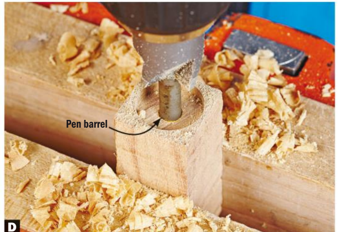
D Trim flush. Using a drill press and the barrel-trimming shaft that matches your barrels' inside diameter, counterbore the wood blank flush with the end of the barrel. This squares the ends and cleans the barrel of any stray glue.
