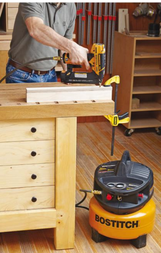
Air compressor A blast of air will clear away dust and debris. Add a brad nailer for quick assembly of project parts.
