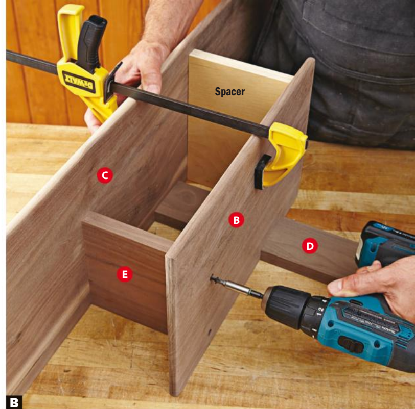
B A spacer and clamp ensure manageable and precise assembly when attaching the middle shelf (B) and short side (E) to the C/D assembly.
