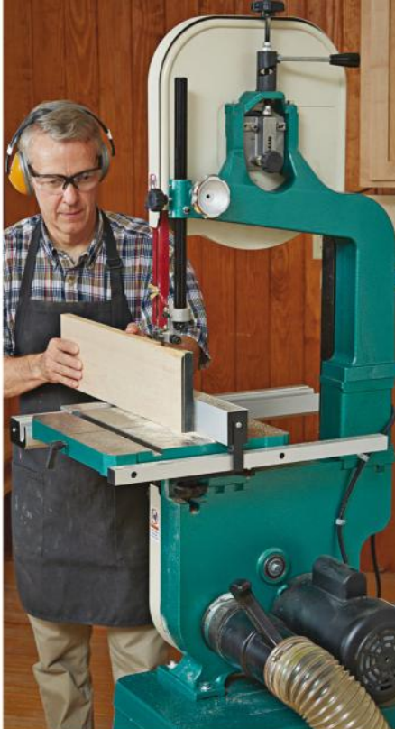
Bandsaw With a narrow blade, it cuts curves. Change to a wider, stiffer blade and use it to resaw boards into thinner workpieces. It can rip stock, too.
