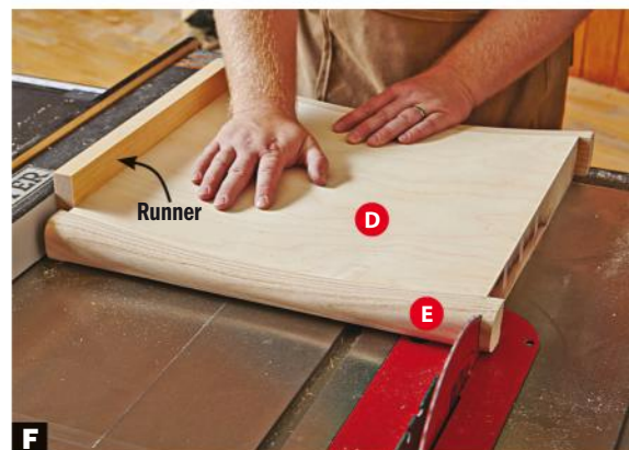
F Trim the trim. Using double-face tape, secure a runner to one end of the seat assembly before flush-cutting the seat-trim ends.
