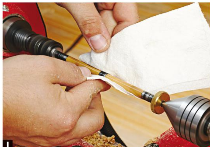
I Make it shine. After sanding smooth, apply a polishing wax, such as Mylands friction polish, to the wood, and buff it with a clean paper shop towel. Note: Do not use cloth towels, as they can wrap around the spinning components. Paper towels will tear away instead.
