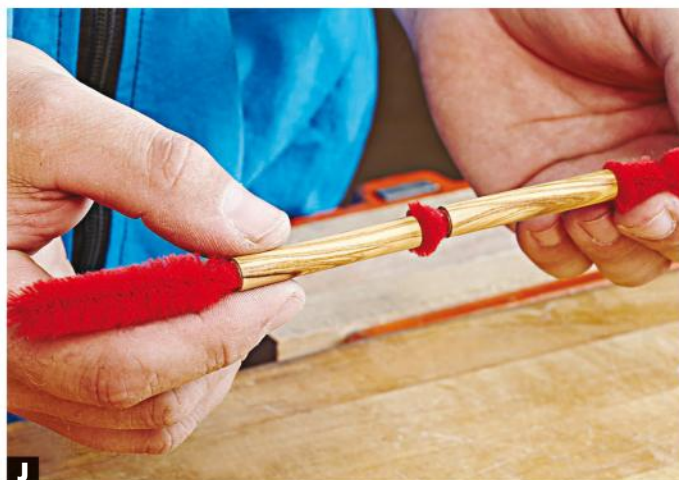
J Keep in line. When finished polishing, remove the wood cylinders from the mandrel and place them onto a pipe cleaner in the same orientation. This keeps the pieces properly oriented as you move to assembly.
