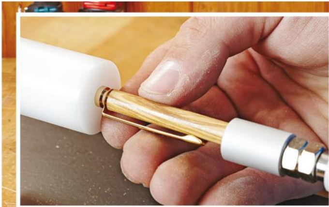
K Start with the tip. Press the pen tip into the front end of one cylinder; seat it fully against the shoulder.
