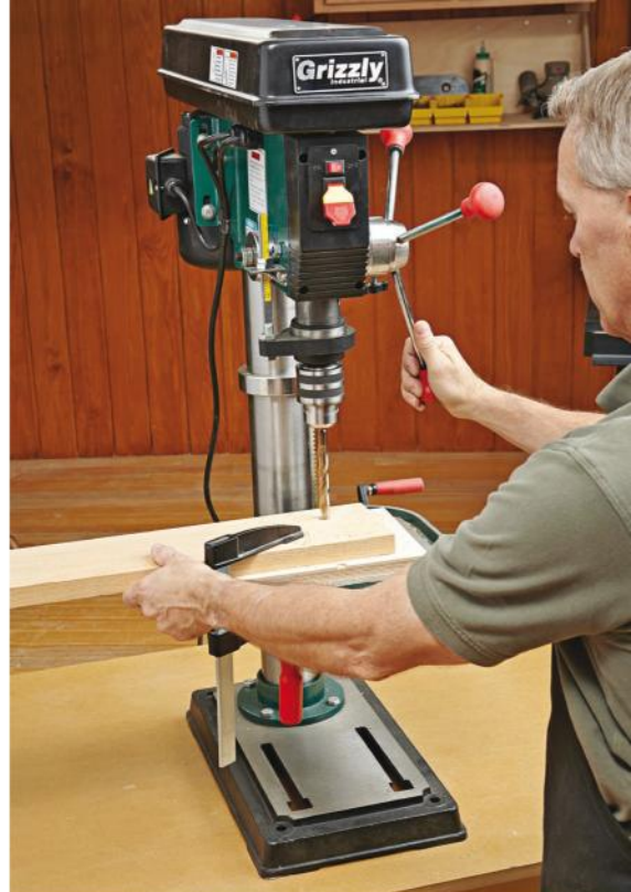
Drill press This helps you drill holes accurately, and can also be outfitted with a drum sander or mortising attachment.
