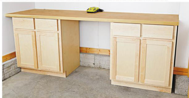
A countertop bridging two cabinets creates another shop worksurface. Plywood door panels rest in frames joined by stub tenons and grooves, a joint you easily can cut on the tablesaw.
