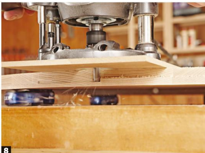
8 Continue plunge-cutting. Elevate the workpiece on riser blocks tucked inside the circle (to avoid contact with the bit). Rout the shape in \frac{1}{8} "-deeper passes, stopping with about \frac{1}{8} " of material left to go.
