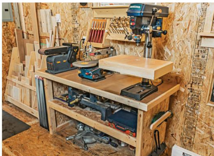
A 26x71½" bench provides space for Mike's drill press, scrollsaw, and 4" belt sander. He stores a mini-lathe and other tools below.
