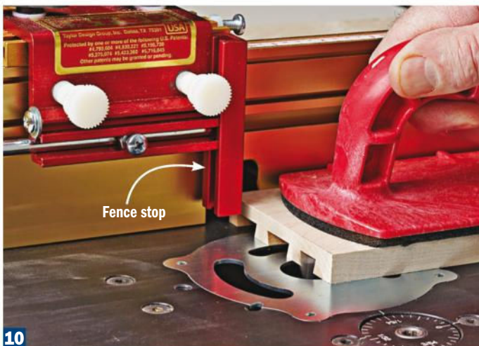
10 Rout the final pins. Retrieve the pin boards and rout tail sockets in each end, using the "D" settings left of zero. Use the fence stop to limit the depth of cut—typically equal to the diameter of the dovetail bit. Sneak up on this depth by extending the stop about \frac{1}{32} " over the bit, then moving it away as needed.
