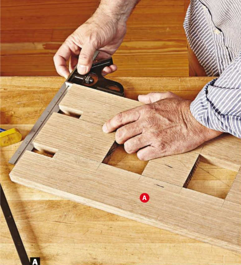
A Square the top ends of the leg boards. Align the center-board segments with the layout lines to form the cutouts.
