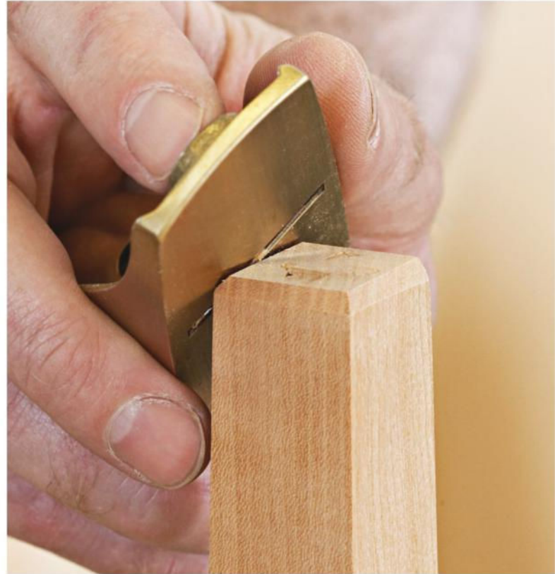
Quick and easy chamfers. Use a low-angle block plane to chamfer the bottoms of table legs to prevent grain splintering. Cut upwards at about a 45° angle.
