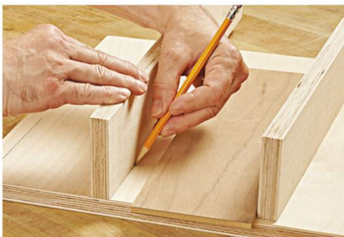
Gauge, measure, repeat. After marking the first dado location, repeat the process to determine the placement of the remaining dividers.
