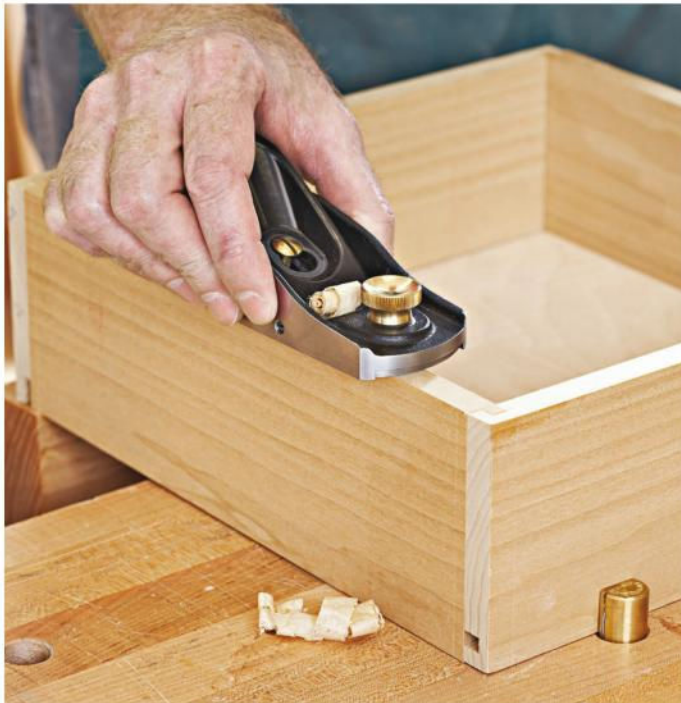
Perfect flush trim. Clean up uneven drawer sides with a few swipes of a block plane. Reverse the cutting direction if you tear out the wood.
