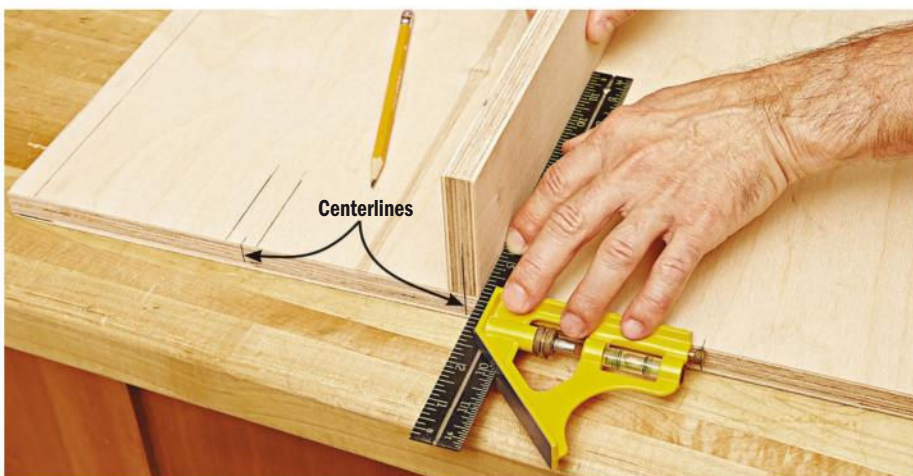
Align centerlines. Mark a centerline on one end of a scrap of the divider stock. Align the mark with each mark on the carcass side, square the scrap with the edge, then mark the dado location.
