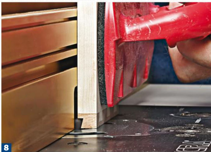
8 Rabbet the tails. Holding each tail board upright against the fence, rout a \frac{7}{32} "-deep rabbet on the inside face. Rout this in three or four incremental passes to avoid tear-out. This reduces the tail thickness to match the depth of the pin board sockets.
