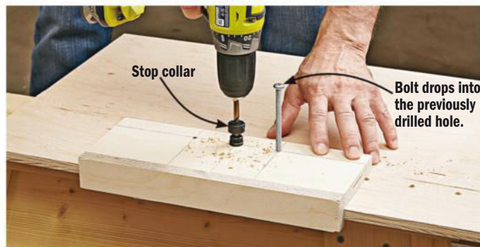
Fabricated from a couple of scraps , this jig automatically spaces the next shelf-pin hole by indexing from the hole you just drilled. A stop-collar on the bit limits the hole depth so you don't drill through the workpiece.
