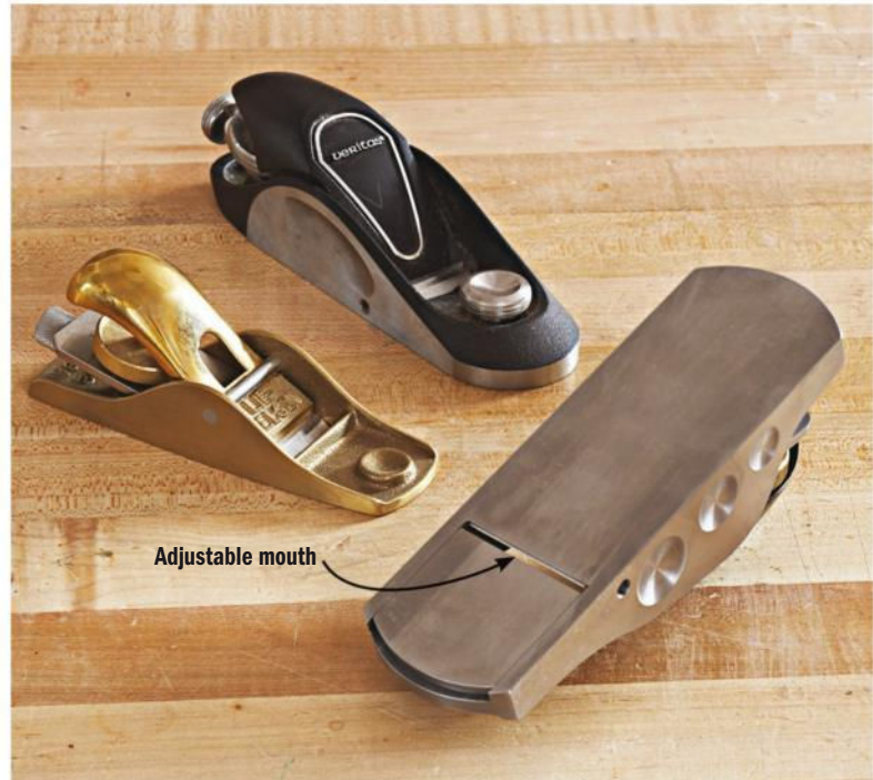
A mouth you can control. Some block planes feature an adjustable mouth, allowing you to better control the depth and smoothness of the cut.
