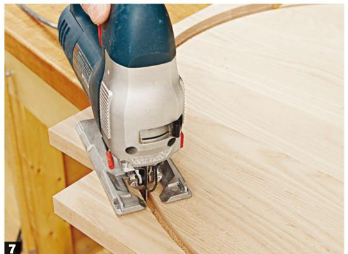
7 Cut away the excess. With the router trammel still attached to the workpiece, cut through the middle of the groove. Rotate the router out of the way as you cut around the circle.
