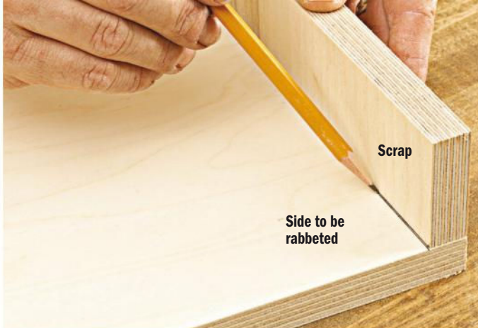
Rabbet hunt. Hold a finish-sanded scrap of stock flush with the top edge of the cabinet side and mark the exact thickness of the plywood top with a sharp pencil or marking knife.
