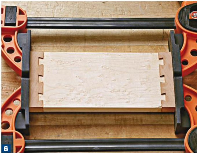
6 Glue your first pins and tails. Apply glue to the inlay pin pieces and slide them onto the ends of the tail boards, centering them on the tail board's thickness. Clamp securely and allow to dry.
