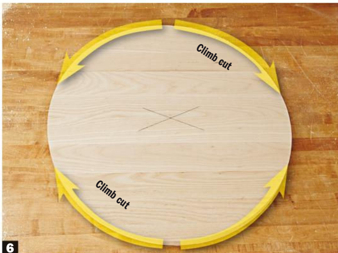
6 Back up for straight bits. If you use a straight bit rather than a spiral, you must climb-cut (routing backwards) the areas of the circle prone to grain tear-out. Do this in \frac{1}{8} "-deep increments.
