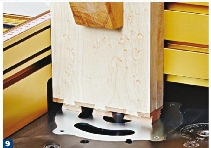
9 Rout the tails, Round II. Sandwich the tail boards against the fence and right-angle fixture with the rabbets to the front and rear. This eliminates tear-out on the outer faces of the tails. Using the "C" settings on the joint template left of zero, rout new tails across the boards.
