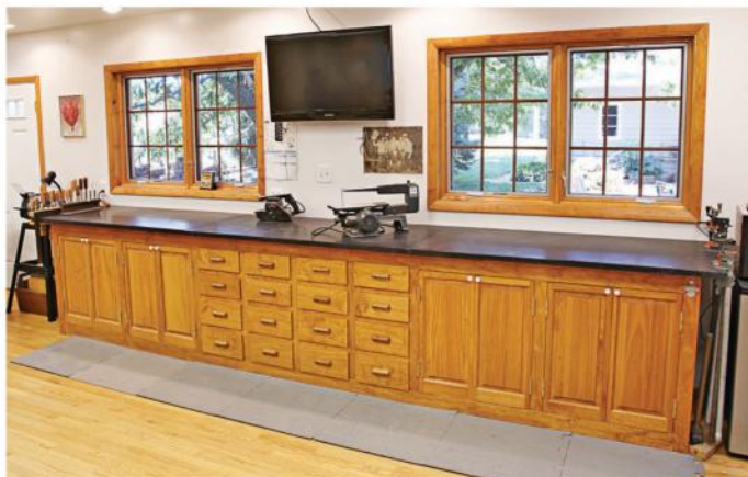
A 15'-long slate countertop, salvaged from a school science lab, tops shop-made cabinets. The raised panels on the doors were reclaimed from interior entry doors.
