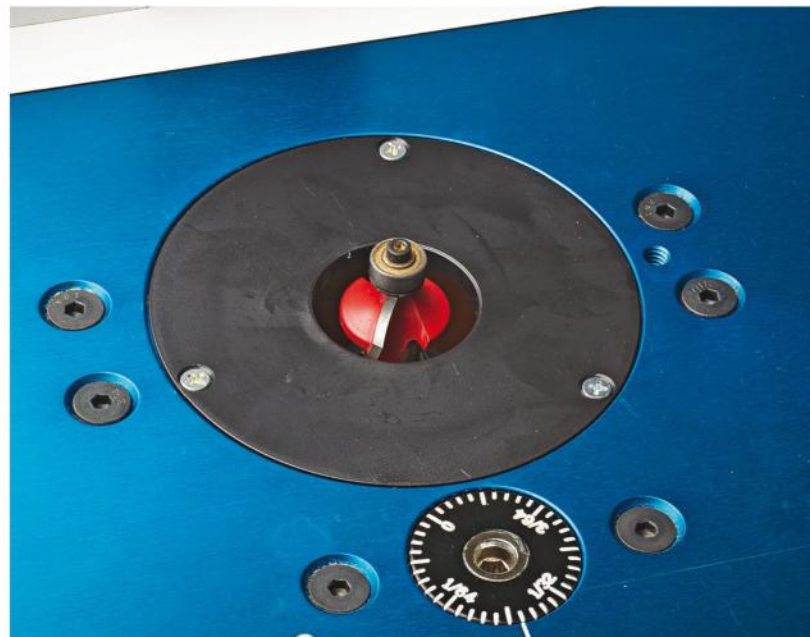
A little more tedious. To remove this insert (shown on the Rockler lift, but also on the Bench Dog) you must first back out three tiny screws.
