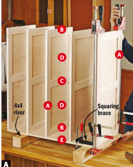
A Install the dust panels one at a time for easier assembly. A squaring brace holds the panel perpendicular to the side while the long bar clamps force it into the side dado.
