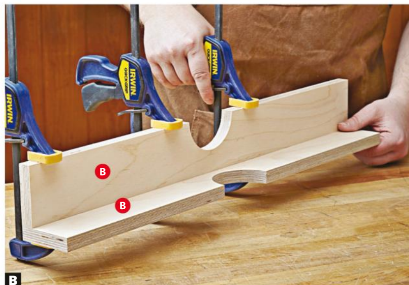
B Clamp up the fence. It will square itself if the edges were cut square to the faces.
