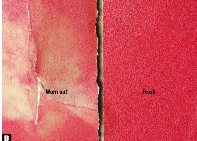
B Sandpaper doesn't last forever. The species of wood and the quality of the paper determine how long a sheet lasts. When a paper's grit no longer has a "catch" when you rub your finger along it, the paper has lost its sharp cutting edge and will only burnish the surface. Replace it.
