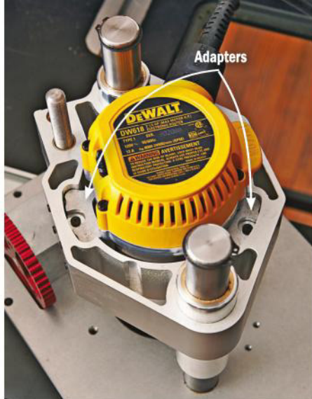
A custom fit. Adapters, such as these shown on the Woodpeckers lift, are sized to fit specific-diameter motors.
