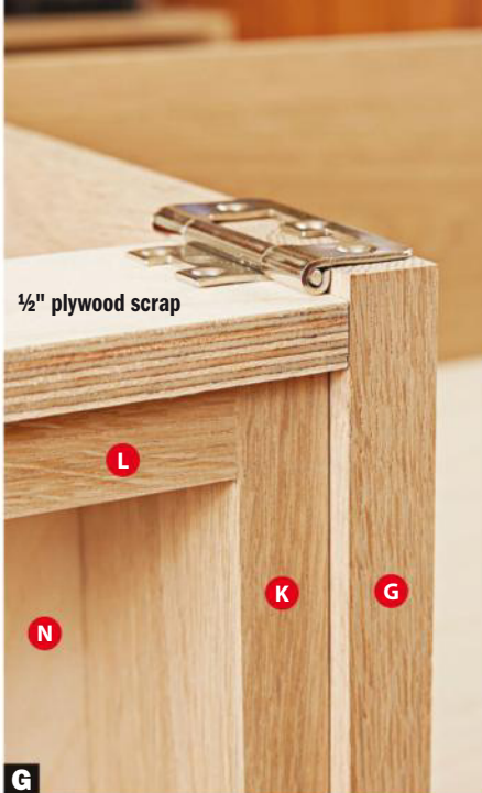
G Check the vertical position of each door by placing a scrap of \frac{1}{2} " plywood on top of the door and a hinge [Source] on top of the case side stiles (G). If there's a gap between the hinge barrel and scrap then shim the door up. If the hinge barrel prevents the hinge leaves from lying flat, then sand down the door top and/or bottom.
