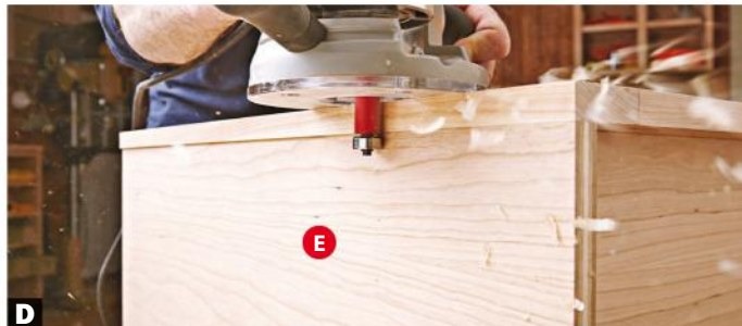
D A router with a flush-trim bit helps you level the stile edges with the sides (E). Set the guide bearing close to the joint between the parts and don't let the router tip on the narrow stile.
