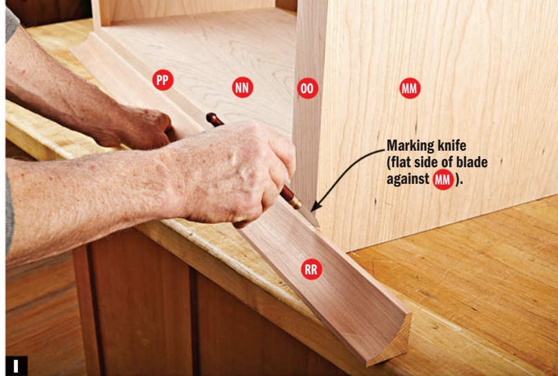
I To fit the front cove trim (RR) precisely, miter-cut one end and mark the location for the opposite miter with a marking knife. Fit the top and bottom trim pieces individually.
