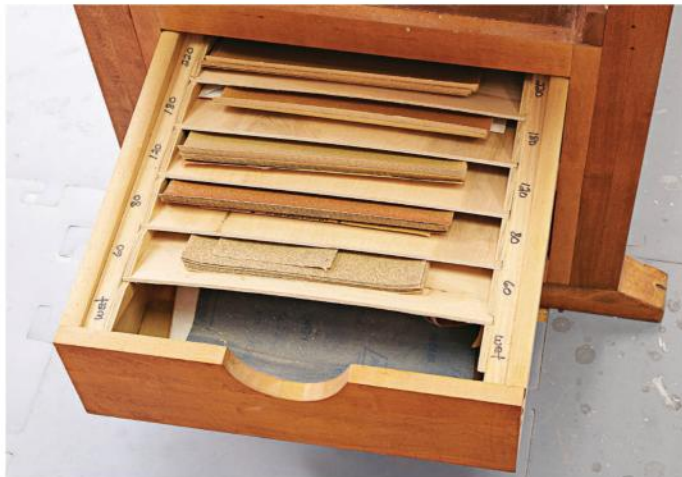
Angled slots provide easy access to sandpaper sheets and make efficient use of drawer space. Labels along each edge help Larry find the right grit quickly.
