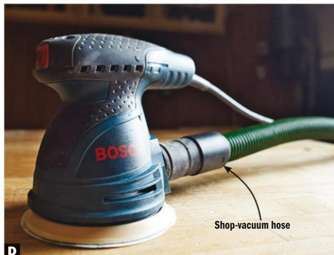
D Hook up a vacuum to protect your lungs from inhaling fine dust and also to remove the minute pieces of loose grit from between the sander and the workpiece. Those pieces, if not collected, can create irregular scratches that stand out on your workpiece's surface.
