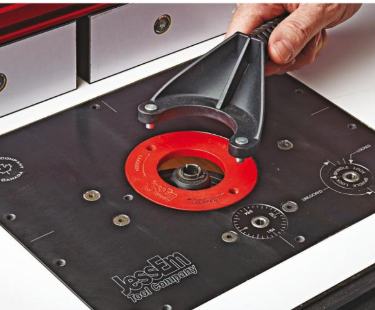
Easy on and off. Insert the spanner wrench's prongs into this insert ring and rotate for quick removal.
