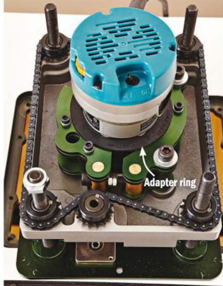
Put a ring on it. Some lifts, such as this Excalibur, use reducing-ring adapters to fit different routers.
