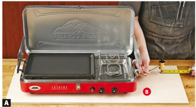
A Mark a hole for the fuel canister by aligning the regulator about 3–4" from the side and back edge of a shelf. Center the hole under the regulator.
