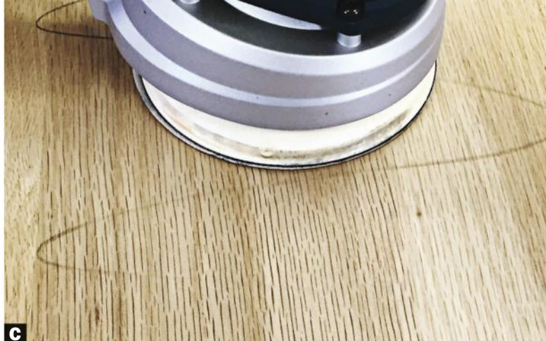
C Pencil-in this sanding trick. Removing a light pencil mark on a board's surface indicates uniform sanding. This method also shows when to switch to the next grit.
