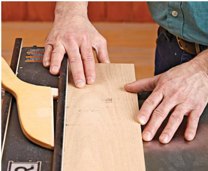
Hooking a couple of fingers over the fence helps keep all digits away from the blade.
