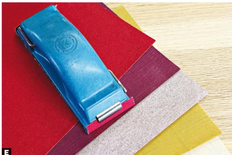
E Sand by hand. Just as there are a number of sandpaper manufacturers, there are also many types of hand sanders. Your choices can range from a simple shop-made pad to a commercially made one like this.
