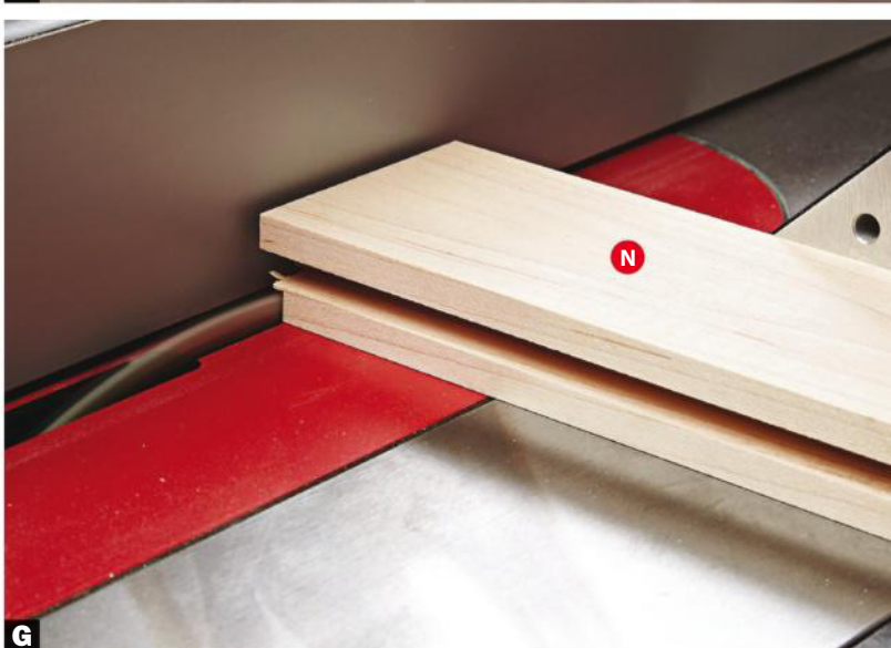
Set your blade height so the highest tooth just touches the groove [Photo F]. After doing so, cut \frac{3}{8} "-long tenons on the drawer rails (N) [Photo G]. Check for fit and square by dry-assembling the frames.
