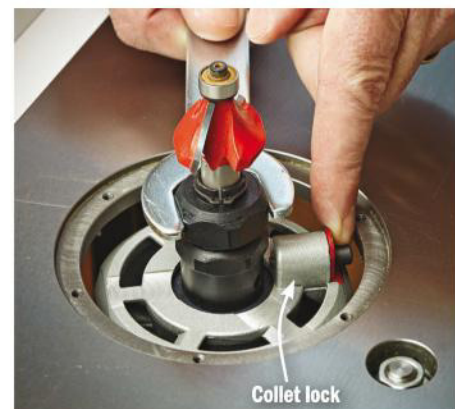
A tight squeeze. This router's collet lock becomes difficult to reach with a finger within the lift opening. We had to use a screwdriver to engage the slide-style lock on some models.
