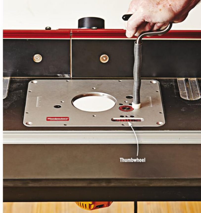
Up and down in a hurry. With the Woodpeckers lift, you compress, twist, and lift with the wrench to disengage the lift system for large adjustments. You then fine-tune the setting with the thumbwheel.
