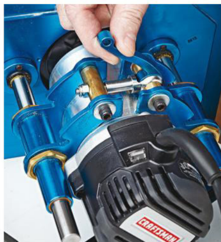
Quick release. Rockler's Router Lift FX uses a simple cam lock to secure a router motor, providing a quick way to free up the router for handheld use.
