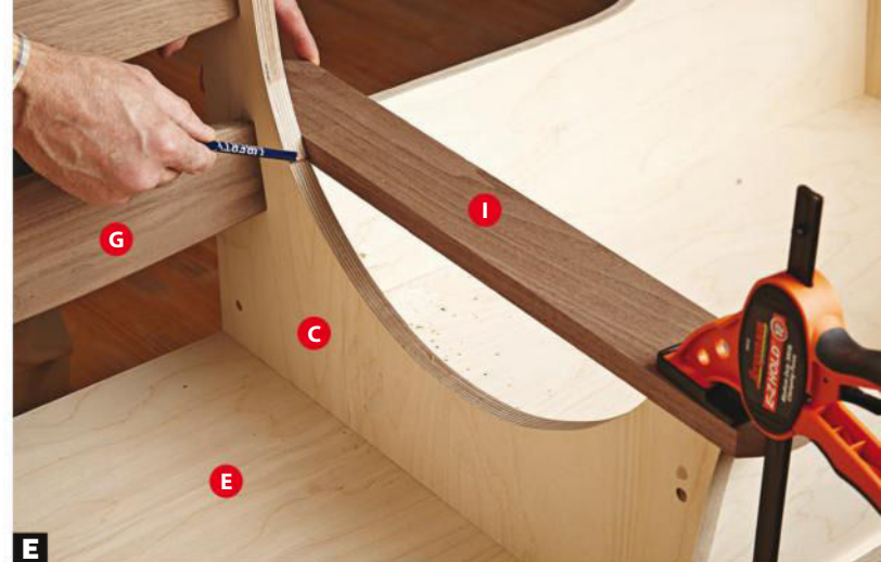
E Mark the armrest notches. Clamp an armrest (I) to the front of the divider (C), with that edge flush with the chair face, and mark where it intersects the divider. Repeat for the chair end (A).
