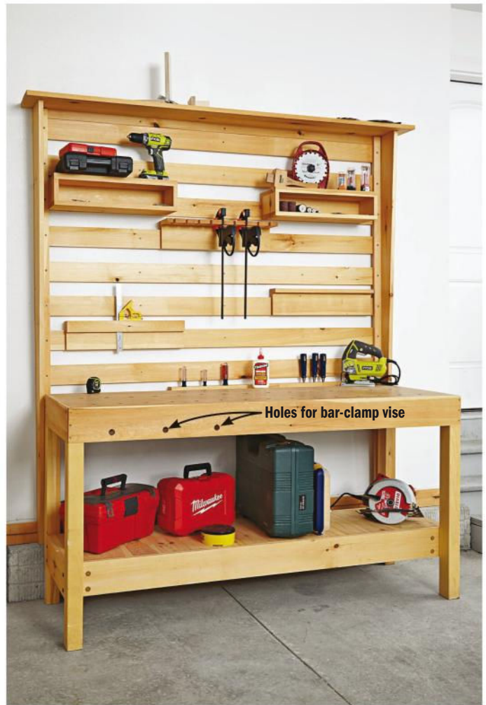
Customize racks and their positions to suit your storage needs. Holders with through-holes trap chisels, squares, and screwdrivers, a slotted hanger keeps clamps close at hand, and boxes serve as two-tiered shelves.
