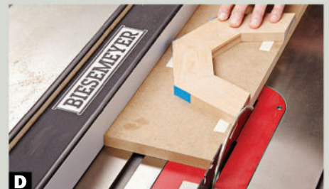
D Mount the half-octagon to a carrier board with double-faced tape with the ends overhanging the edge just slightly. True up the end miters.
