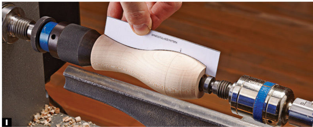
I Turn the spindles to shape, checking the profile with the pattern template.
