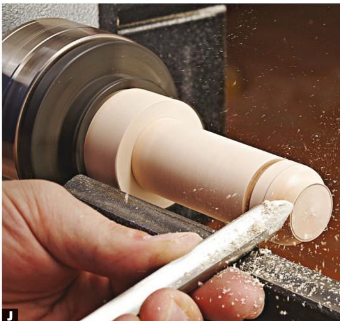
J Use a spindle detail gouge to form an ogee from the \frac{1}{16} " mark on the side of the blank to the \frac{7}{8} "-diameter circle scribed on the end.
