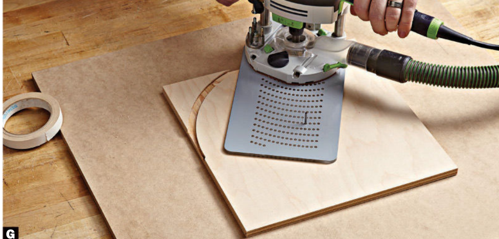
G Mount each plywood disk blank to a spoil board with double-faced tape. Use a plunge router and circle jig to cut the disks.
