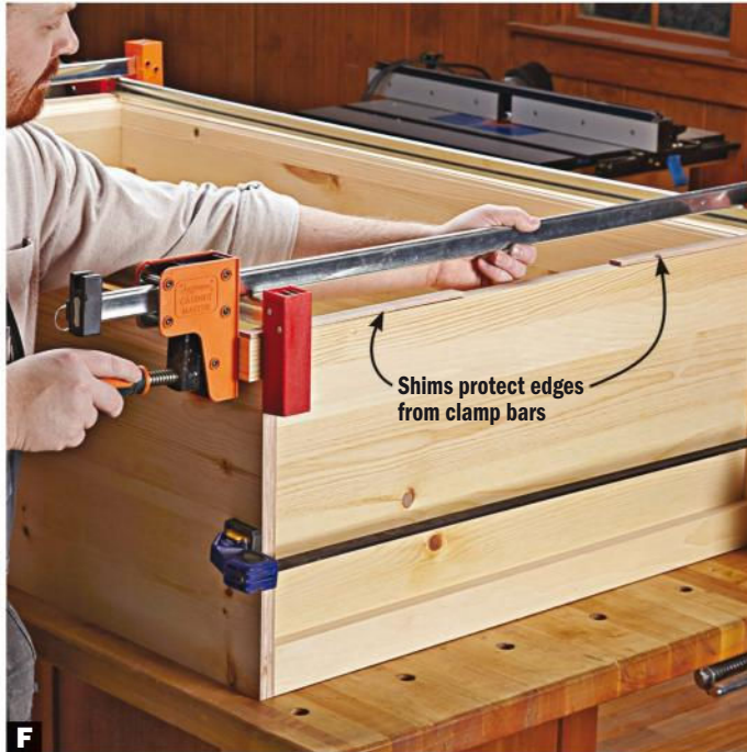
F Watch your corners. When gluing up the case assembly, focus on tightly pulling together the mitered corners to prevent unsightly gaps.
