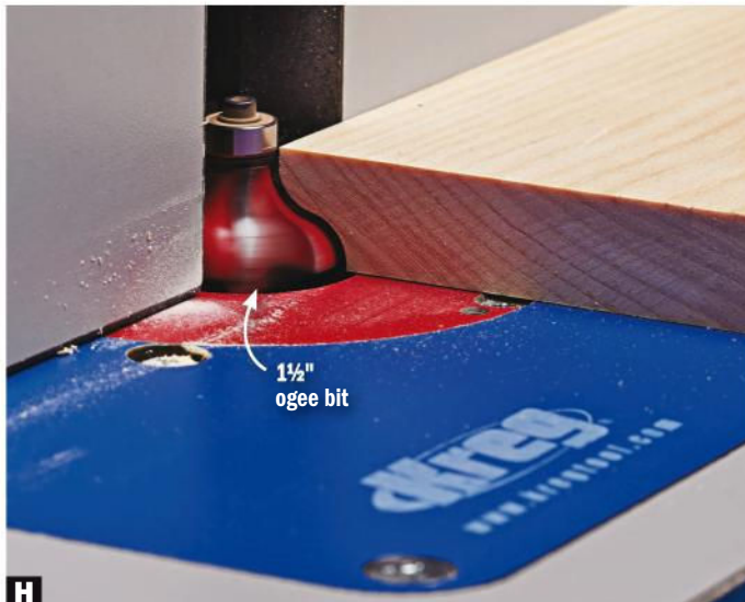
H With the bearing flush with the router-table fence, rout a profile along both edges of the molding (H, I) blank. Doing so in a wider piece like this is safer, more efficient, and yields better cuts than machining a narrow piece.
