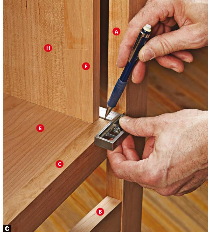
A small square aids in marking the front stile locations on the stretchers (C). These marks indicate the outer edges of the doors for locating the hinges on the stretchers.
