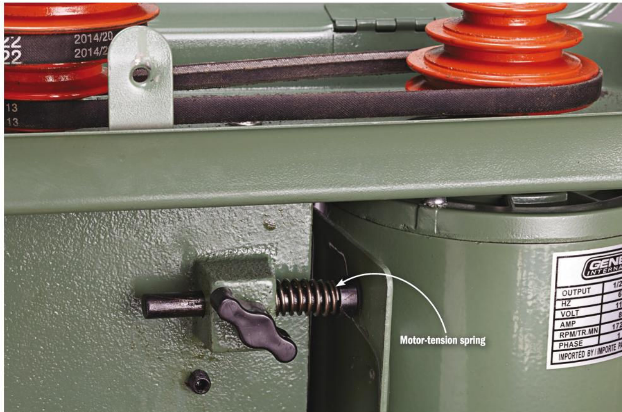
Fully compressing this motor-tension spring proved difficult, making it a chore to change belt position for a different spindle speed.
