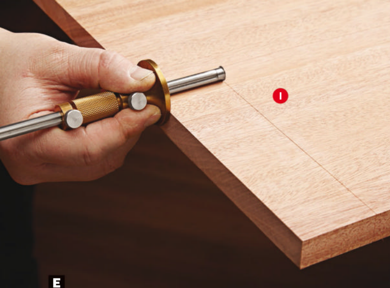
E Score the ends of the top panel with a marking gauge to indicate the length of the tenons. (See Drawing 5.)
