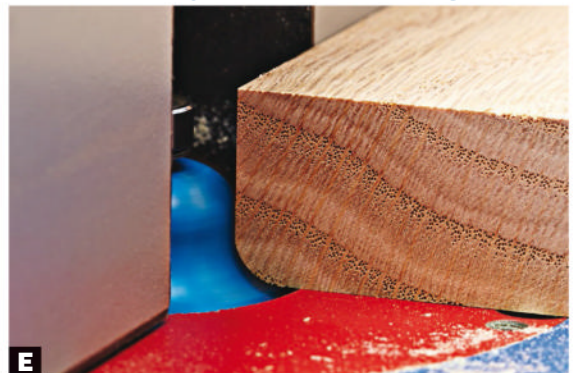
E Break the edge. The round-over softens the sharp edges and corners on projects made with splinter-prone woods such as oak or cedar. The radius of this round-over is \frac{1}{4} ".
