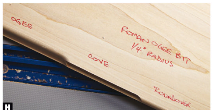
H To instantly recall how you made a profile, keep a storyboard like this one. Mark the bit type and any pertinent details (cutting depth, bit height, etc.) beside each profile.
