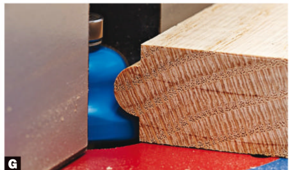
G Create a beaded profile. Rout a round-over with a fillet along both edges of your board. Test-cut a piece of scrap, adjusting the bit height until the two round-overs meet at the center, forming a perfectly round bead.
