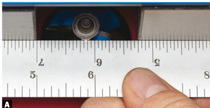
A Set the bearing flush with the fence. Using a straightedge against the fence face helps to locate the bearing correctly. The bearing should just “kiss” the straightedge.
