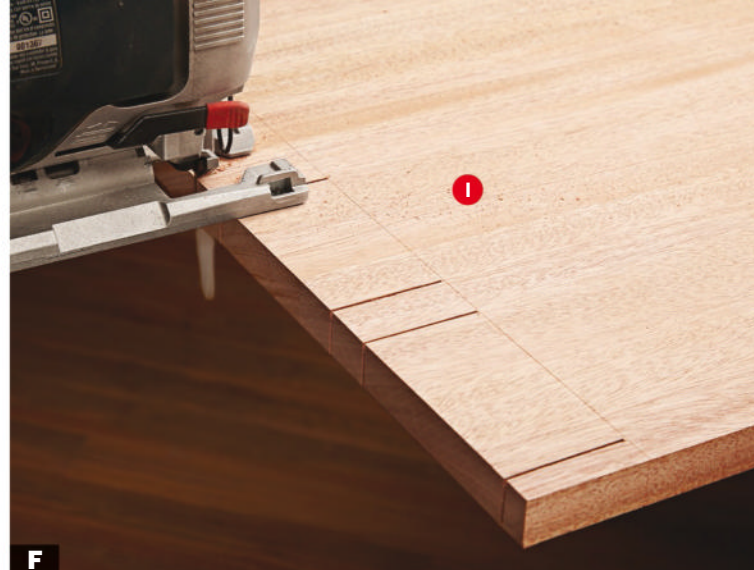
F Separate the tenons by cutting along the layout lines with a jigsaw. Doing this now provides full-thickness support for the jigsaw.
