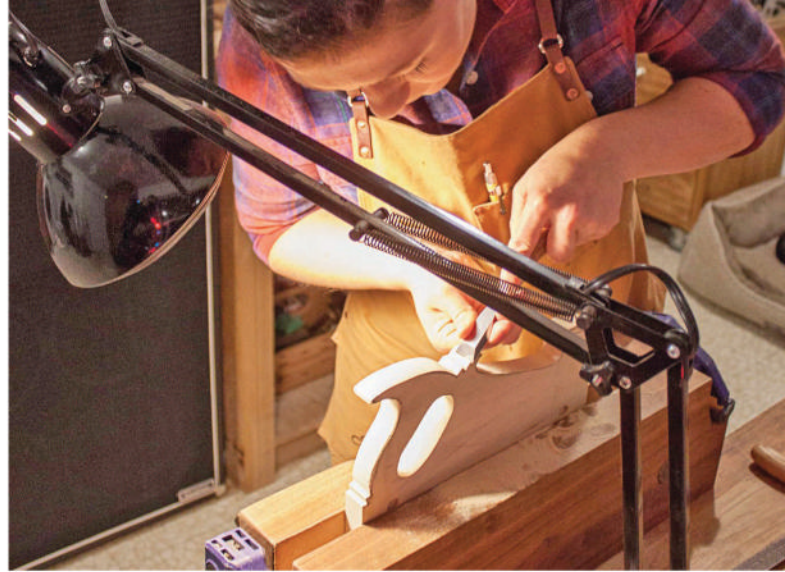
Bench-dog-mounted lighting travels to wherever it is most needed, eliminating the need for an expensive electrical overhaul in the farmhouse.
