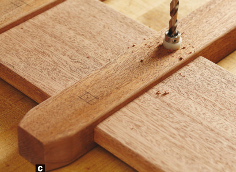
C Drill stopped holes for each plug mortise by attaching a stop collar to a \frac{21}{64} " brad-point drill bit for a \frac{3}{8} "-deep hole. (You can get by with a \frac{5}{16} " bit.)
