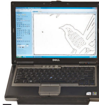
B Create in CAM. A model or drawing created in CAM software can be re-created on any number of workpieces, and scaled up or down easily.
