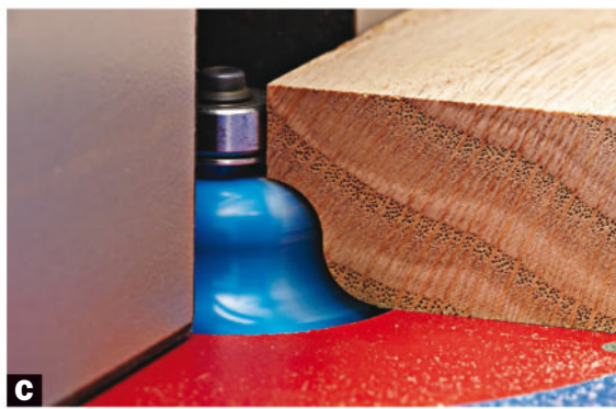
C Classic ogee profile. Lowering the bit removes the fillet, resulting in a more classic-looking ogee profile. This second profile has less ornamentation than the first but provides a smooth transition from a flat surface.
