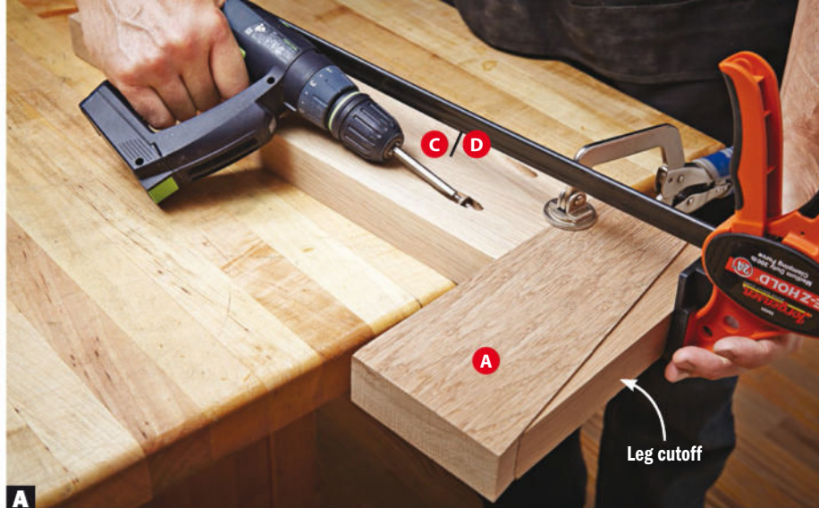
A Attach the rails to the legs using 2½" heavy-duty pocket screws (no glue necessary). Position the leg cutoffs to ease clamping.
