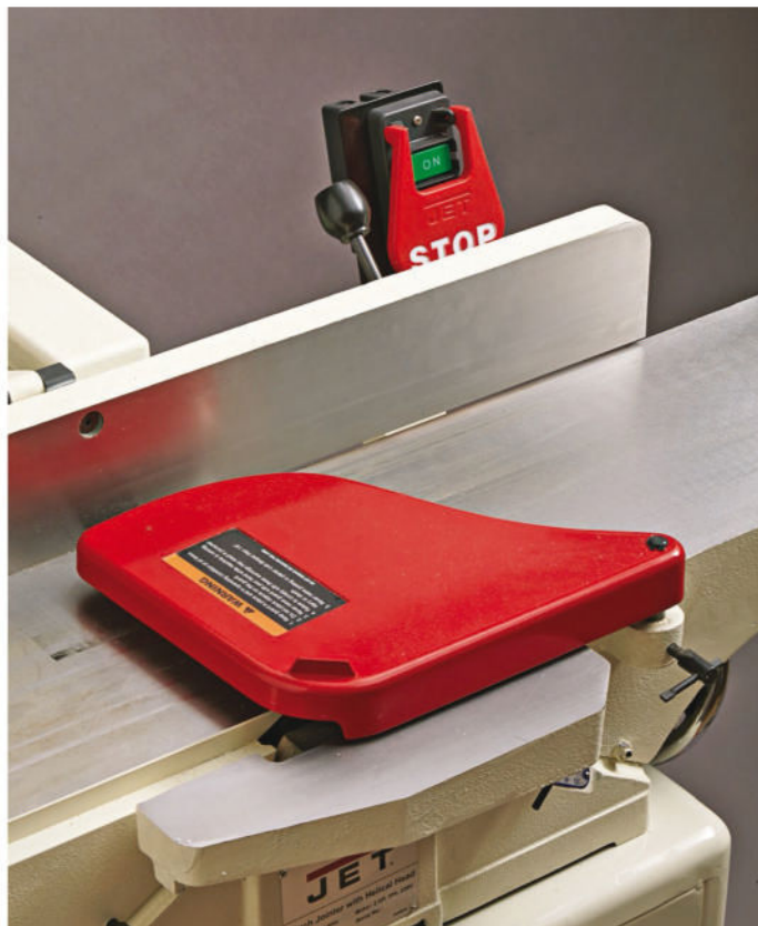
Jet's switch sits behind the fence, making the off paddle awkward to reach in an emergency. You can also mount the switch to the cabinet below, but it's equally awkward.
