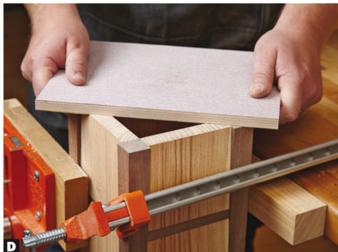
D Make a big sanding block by spray-adhering sandpaper to a scrap of flat plywood or MDF. Sand diagonally in alternating directions until the top and bottom of the box are flat.
