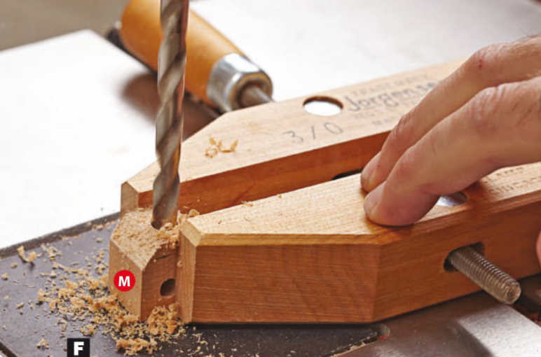
F Drill holes in small parts safely. Use a wooden handscrew to hold the cannon base (M) securely when drilling its holes.
