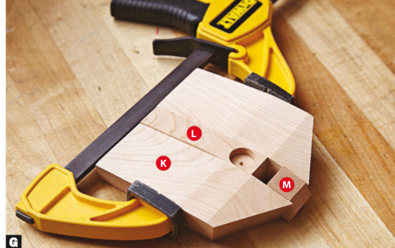
G Clamp down on the turret. Use the bar of a one-handed bar clamp to keep the ends of the turret assembly aligned during glue-up.
