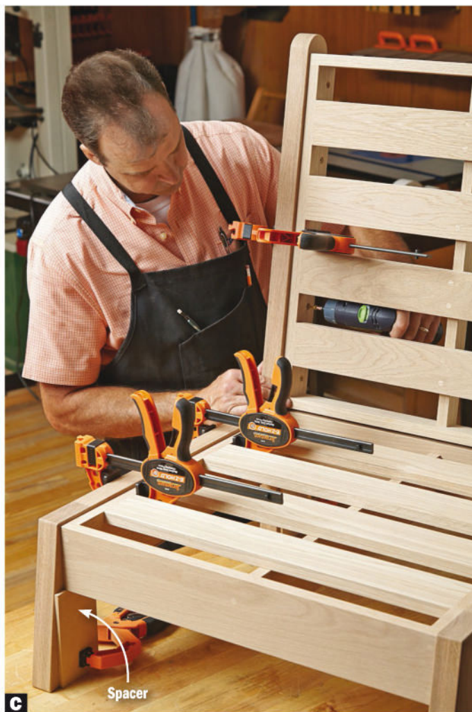
C Use spacers to position the seat frame when attaching the second leg/rail assembly. Check for symmetrical spacing on both sides.
