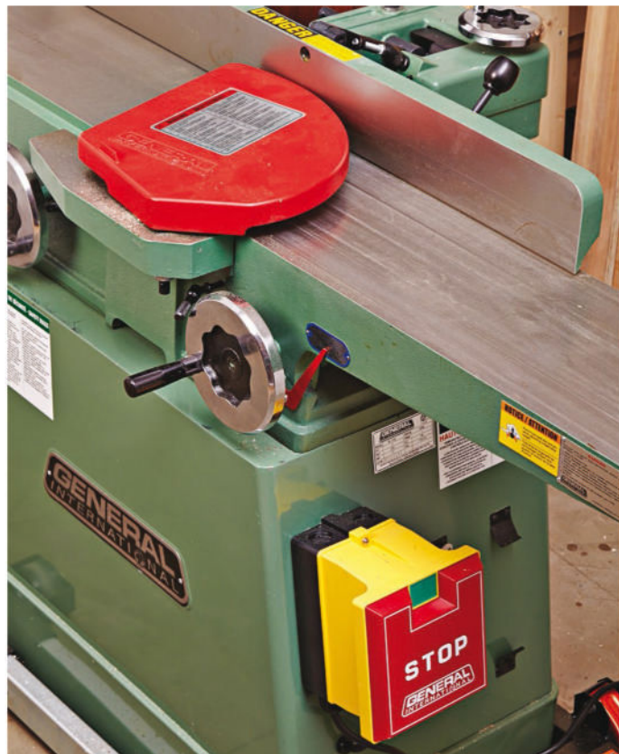
General International's switch mounts below the infed table, and cannot be easily reached if you're working nearer the outfeed table.
