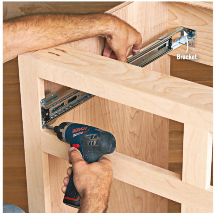
Secure the front of the slide to the face frame. The bracket at the rear slides to reach the back of the cabinet. This requires a stretcher or cabinet back at least \frac{1}{2} " thick.
