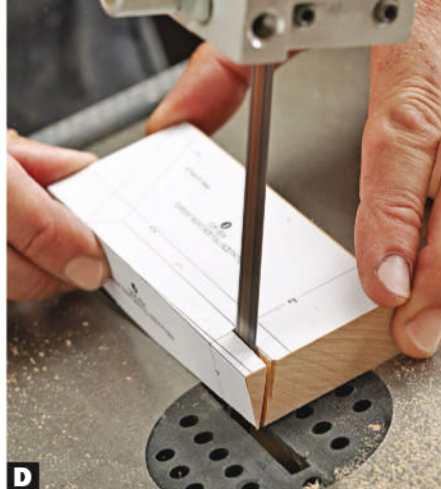
D Tilt the table 15° , then cut along the long edge of the patterns. Keep the flat center portion of the piece resting on the table throughout the cut.
