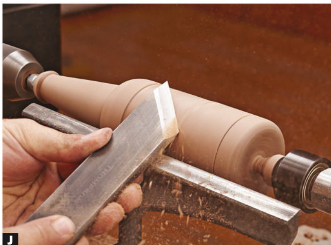
H Using a spindle detail gouge, form a smooth half-bead transition from the barrel to the neck. Leave the pencil line for the label.
