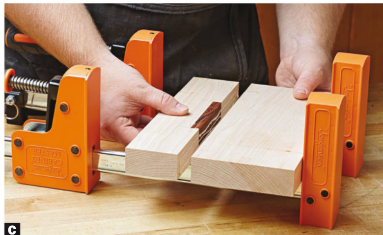
C Reclamp the blank's two sections, being careful to align the ends and faces of the workpieces.
