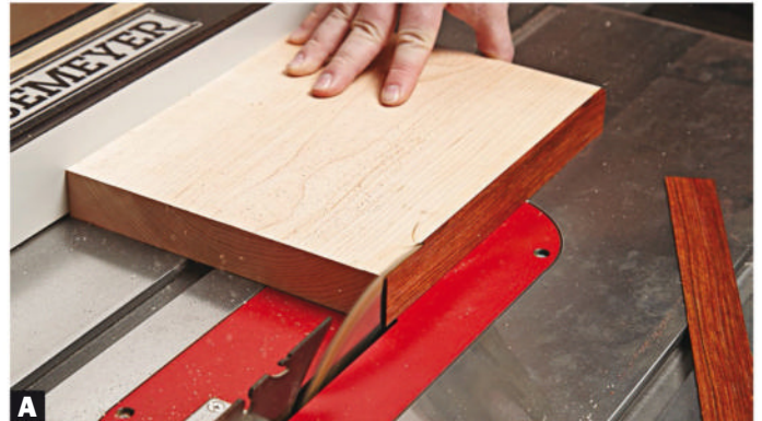
A A large blank makes ripping thin strips safer, so glue the cocobolo to the maple block before ripping the cocobolo and maple strips.
