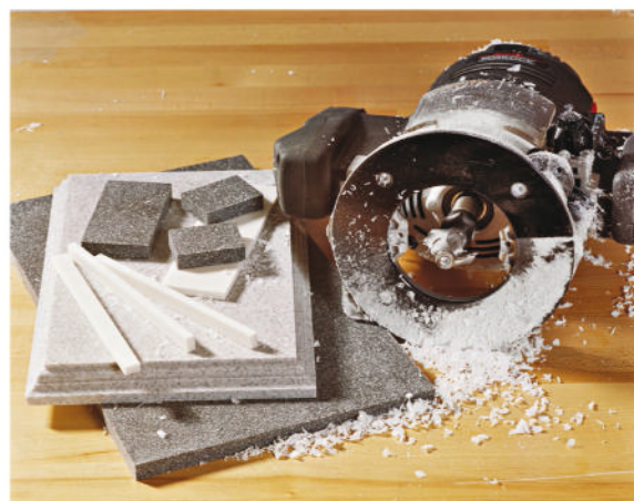
Many woodworking tools and tricks work with solid-surface materials. Cut and rout with sharp carbide blades. You can even sand it like wood.
