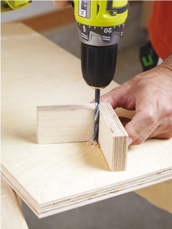
A jig can be as simple as two scraps of plywood glued together to help guide a drill bit perpendicular to a workpiece.
