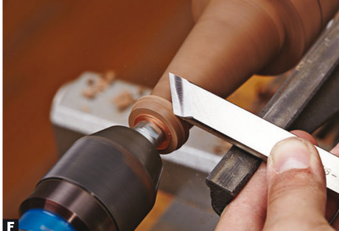
F Chamfer the lip to \frac{7}{8} " diameter at the end with a skew chisel.
