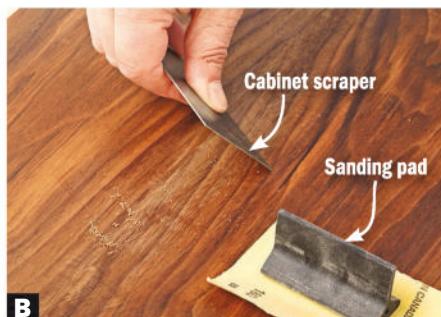
B Remove dried glue to fix a finish. Scrape and sand glue from only the affected area (Photo B) if you can, going down to the bare wood. Test the area as in Photo A, to make sure you've removed all traces of glue. With finish applied and blended into the surrounding area, the flaw nearly vanishes (Photo C).
