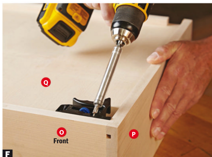
F Place the clip tight against the drawer front (O) and side (P). Drive the furnished screws snugly into the drawer front.
