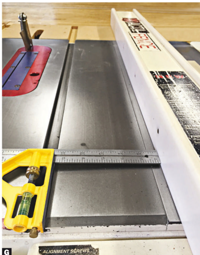
G Slide in the slot. Rest the combination square against the right edge of the right miter slot. The square's rule should touch the fence face at the rear as it does the front edge.
