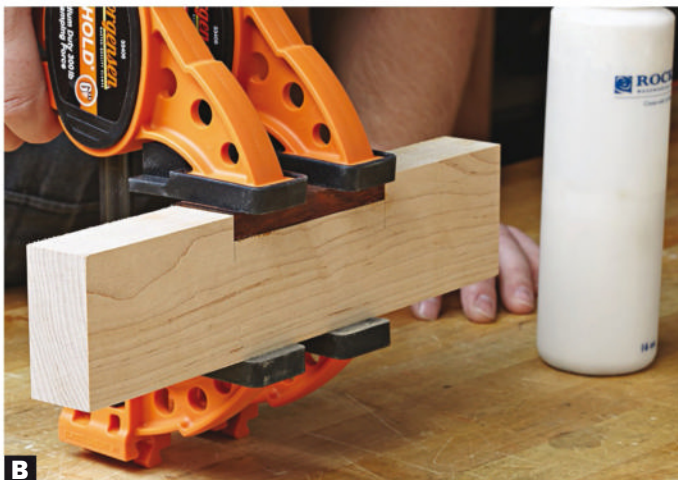
B Make a hard-wearing sole. The cocobolo insert becomes the spokeshave's sole (after all cutting and shaping has been done). Trim it flush to the maple edge when dry.
