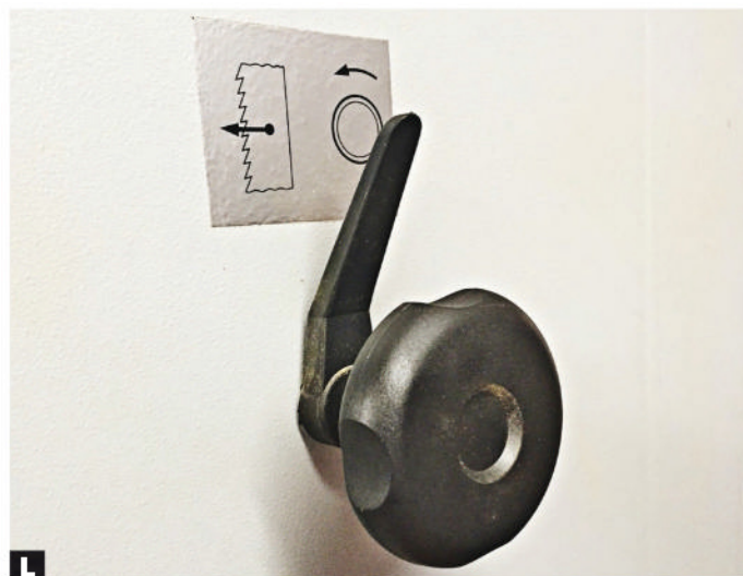
L Keep everything on an even keel. With the bottom wheel's position fixed, use the tilt knob to align the top wheel.
