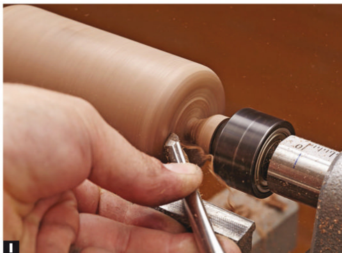
G Make a small half-bead with a detail gouge on the bottom of the lip.
