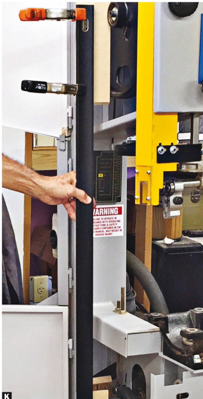
K Here's the long and short of it. A couple of particleboard extensions allow my straightedge to reach the top and bottom of both wheels while clearing the saw frame. I had to remove the table to gain access to both wheels.
