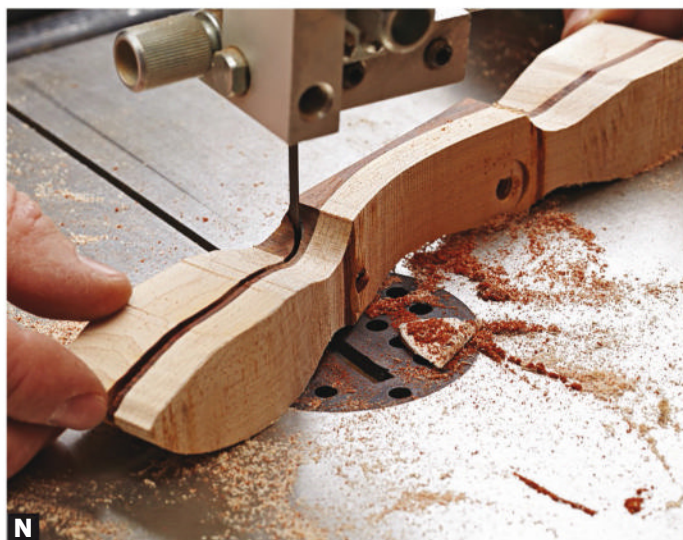
N Now shape it top to bottom. Cut just outside the lamination glue-lines—except for the sole's pattern—to bring the spokeshave to its rough final shape.
