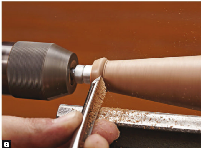
E Make a \frac{1}{16} "-deep V-cut with a skew chisel at the base of the lip. This defines the top of the neck.
