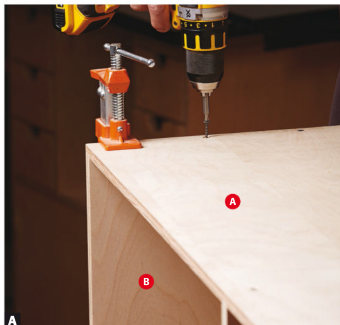
A Keep the edges flush as you glue and screw the sides and divider (B) in place. Drive the screws slightly below the surface.
