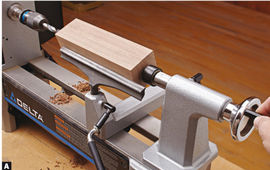
A Position the tool rest against the blank to keep it from turning. With the lathe running at 500 rpm, slowly feed the blank into the bit by turning the tailstock's quill-feed handle.
