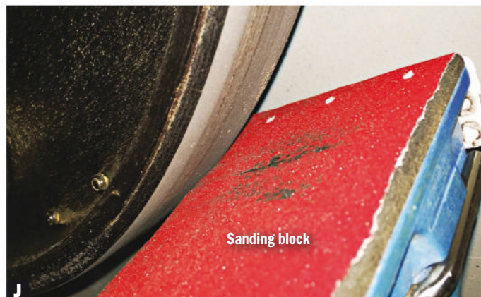
J Get down to the nitty-gritty. While turning each wheel by hand, angle a sanding block with 100-grit sandpaper to restore the radius. I check my progress often using a contour gauge until the tire matches the profile suggested by the manufacturer.
