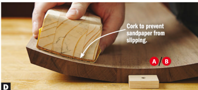
D Add a curve to your sanding block. Use a sanding block, rounded to match the curve of the blanks, and aggressive abrasive, to smooth the inside. It may take longer than using a random-orbit sander, but the curve will be smooth and even.
