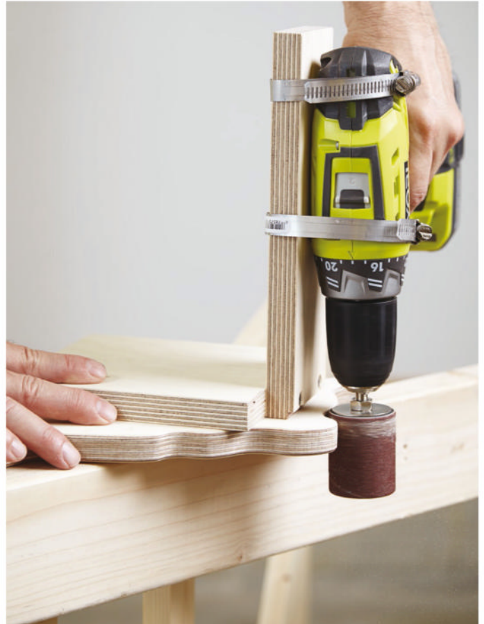
Two more scraps of plywood and two hose clamps create a jig to hold a drill equipped with a sanding drum. Use it to smooth edges without rounding them over.
