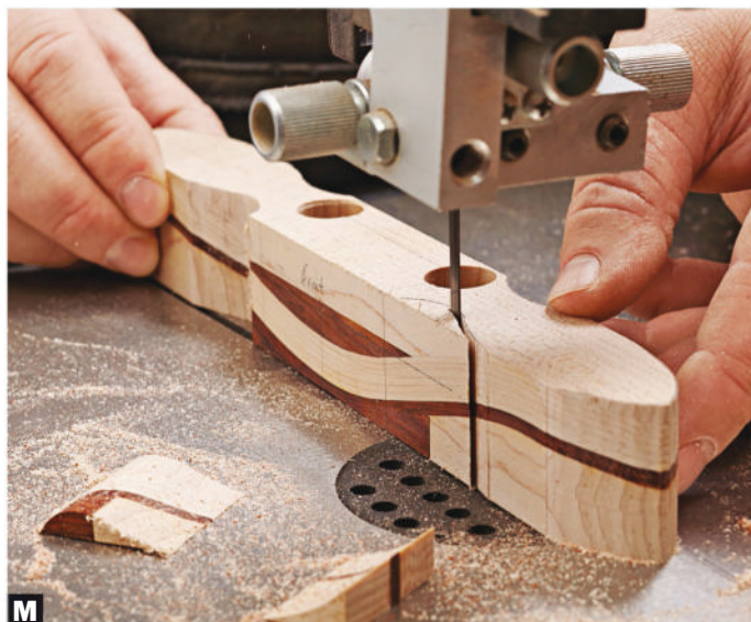
M Shape the body front to back. Bandsaw the handle curves to shape, staying just outside your pencil lines.
