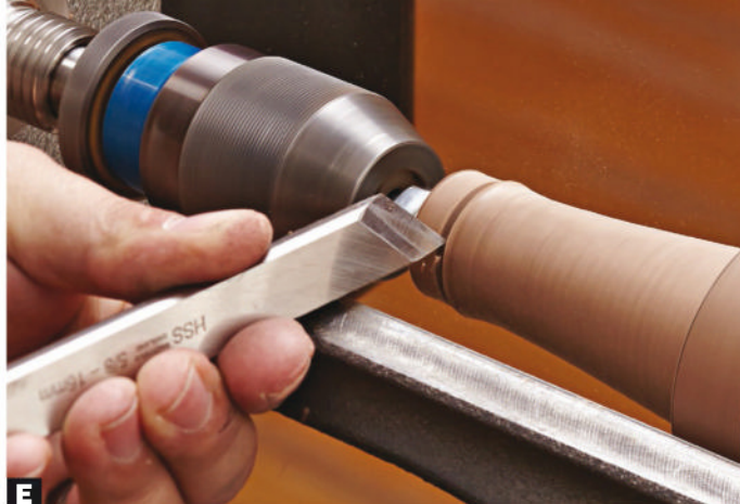
E Make a \frac{1}{16} "-deep V-cut with a skew chisel at the base of the lip. This defines the top of the neck.
