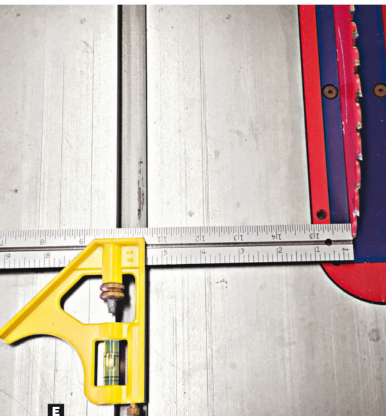
E Slide from front to back. Use care when sliding the square so as not to damage the blade teeth. A gap or binding between the square and tooth means the blade is not parallel to the miter slot.
