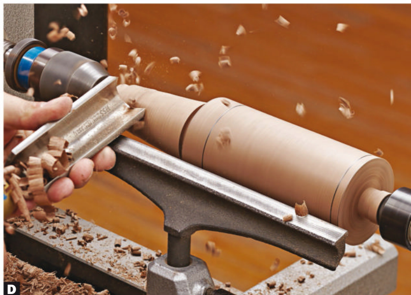
D With your spindle roughing gouge, remove most of the material between the lip and the base of the neck.
