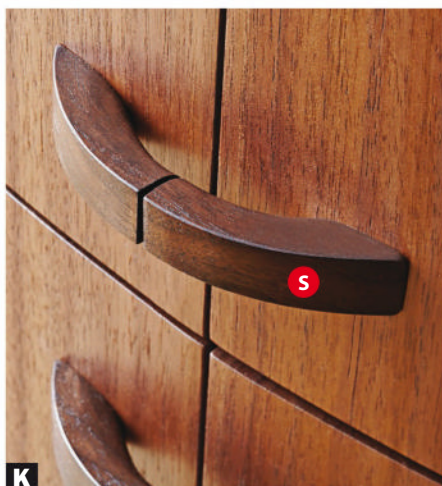
K Round the inside of each handle using a chisel and by hand sanding. Crosscut each handle in half and screw the two parts to the doors.
