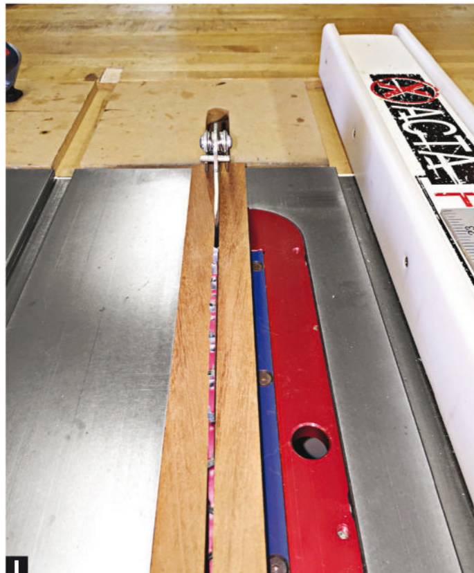
I Now is the time to split hairs. The splitter shown is sized to work with regular 1/8"-kerf blades. If you use both regular and thin-kerf (3/32"), you'll need a separate splitter for each.
