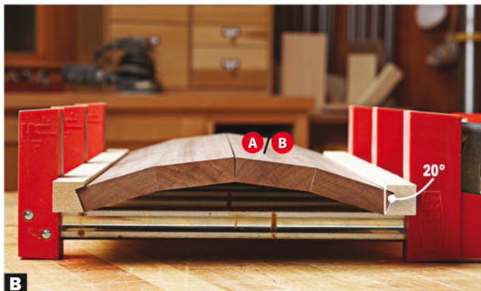
B Mind the gap. The joint between the stave pairs will want to open up during clamping.
