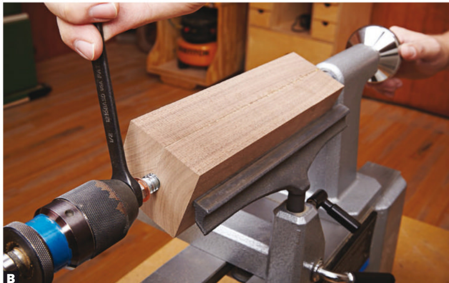
B Without running the lathe, use a \frac{1}{2} " wrench to thread the insert into the blank while also advancing the tailstock quill-feed handle.
