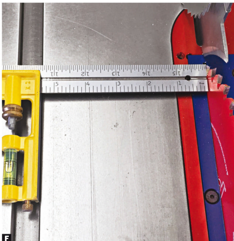
E Slide from front to back. Use care when sliding the square so as not to damage the blade teeth. A gap or binding between the square and tooth means the blade is not parallel to the miter slot.
