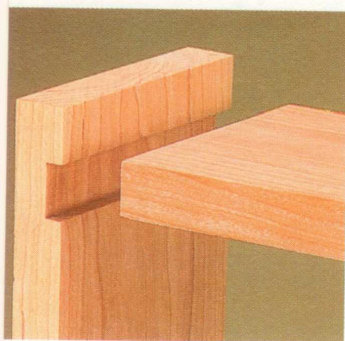
A dado joint can be used to hold a shelf in a bookcase or to join the parts of a cabinet.
