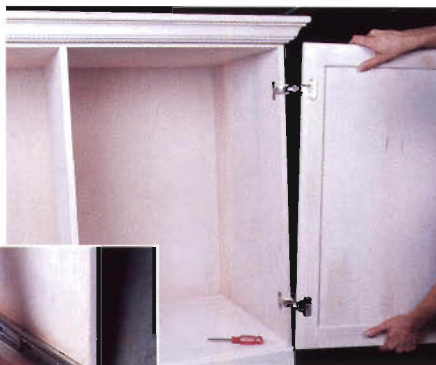
Figure 5: Use 270° Aximat hinges for full clearance. Accuride slides (inset) provide easy access to the printer and keyboard.
