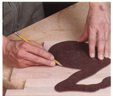
Figure 3: As each leg is made up of two laminations, you can add considerable strength by paying special attention to grain patterns.
