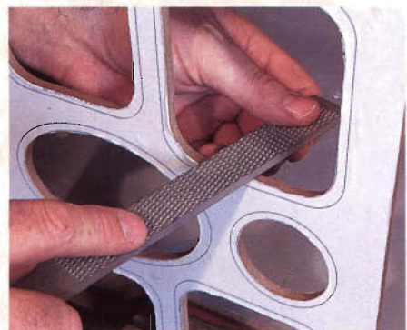
Figure 2: Refine your template with files and sandpaper. Accuracy is very important as any rough spots will be transferred to the project.
