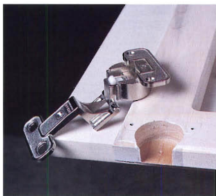
Figure 3: Install the Aximat hinges by boring a couple of 35 mm holes, then screwing the hinges in place.
