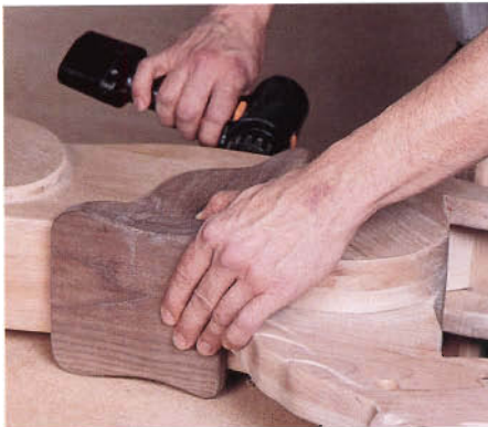
Figure 6: The saddle top is secured to the horse's body with glue and screws driven up through the body cavity.
