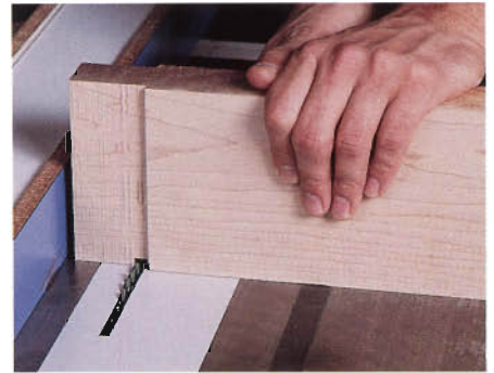
Figure 7: There's only one tenon in this project so it's quicker to nibble away the waste with a regular blade than installing a dado head.
