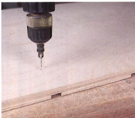
Figure 1: Position the screws that hold the carcass together by drilling pilot holes in the dadoes, then counterbore them from the outside.
