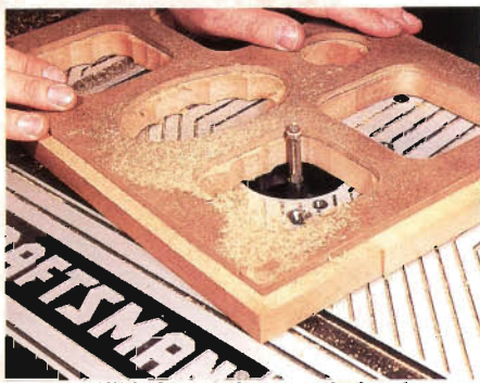
Figure 3: With the template attached to the workpiece with two-sided tape, a laminate trimming bit cleans up the cutouts.
