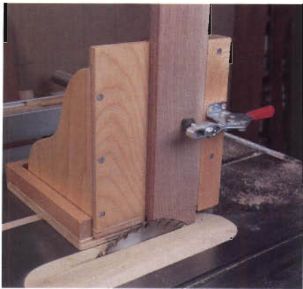
Figure 4: You can make the tenons on the ends of the door rails with a tenoning jig like this one featured in issue 34 of Today's Woodworker .
