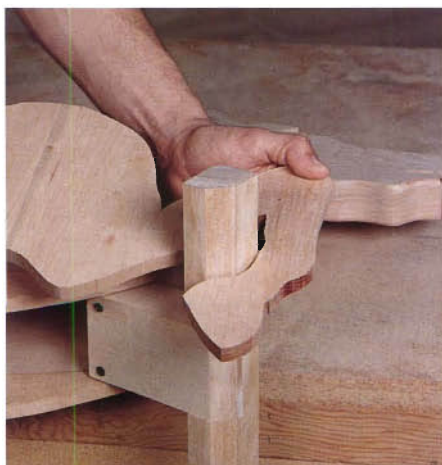
Figure 4: Dry fit the front leg laminations around the foot support and, if necessary, remove a little material from the support for a perfect fit.
