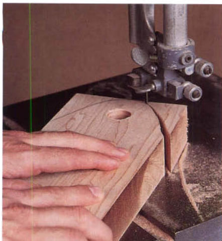
Figure 8: Saw the curve on the top of the riser before cutting the shoulders: it's easier to draw the curved line with the piece still square.
