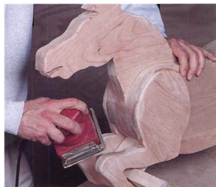
Figure 5: Use a palm sander to add final shape to the horse's legs after they have been installed. Be careful not to over-sand.
